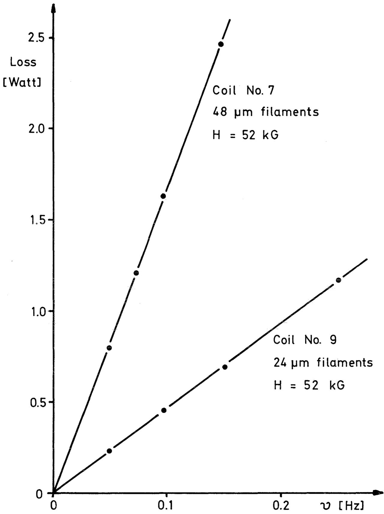
Fig. 5: Variation of ac-losses with filament diameter for twisted Cu/CuNi composites
