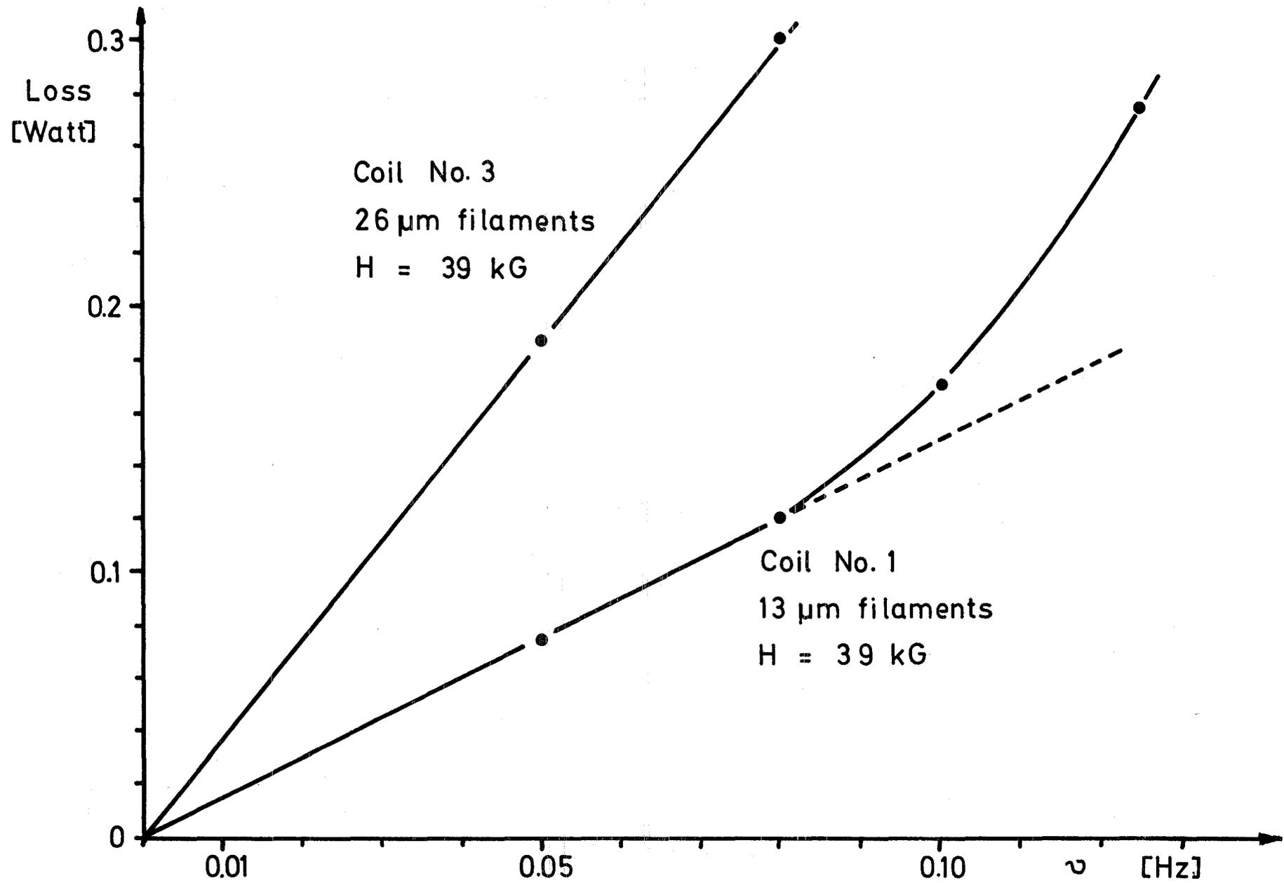
Fig. 4: Variation of ac-losses with filament diameter for twisted copper composites
