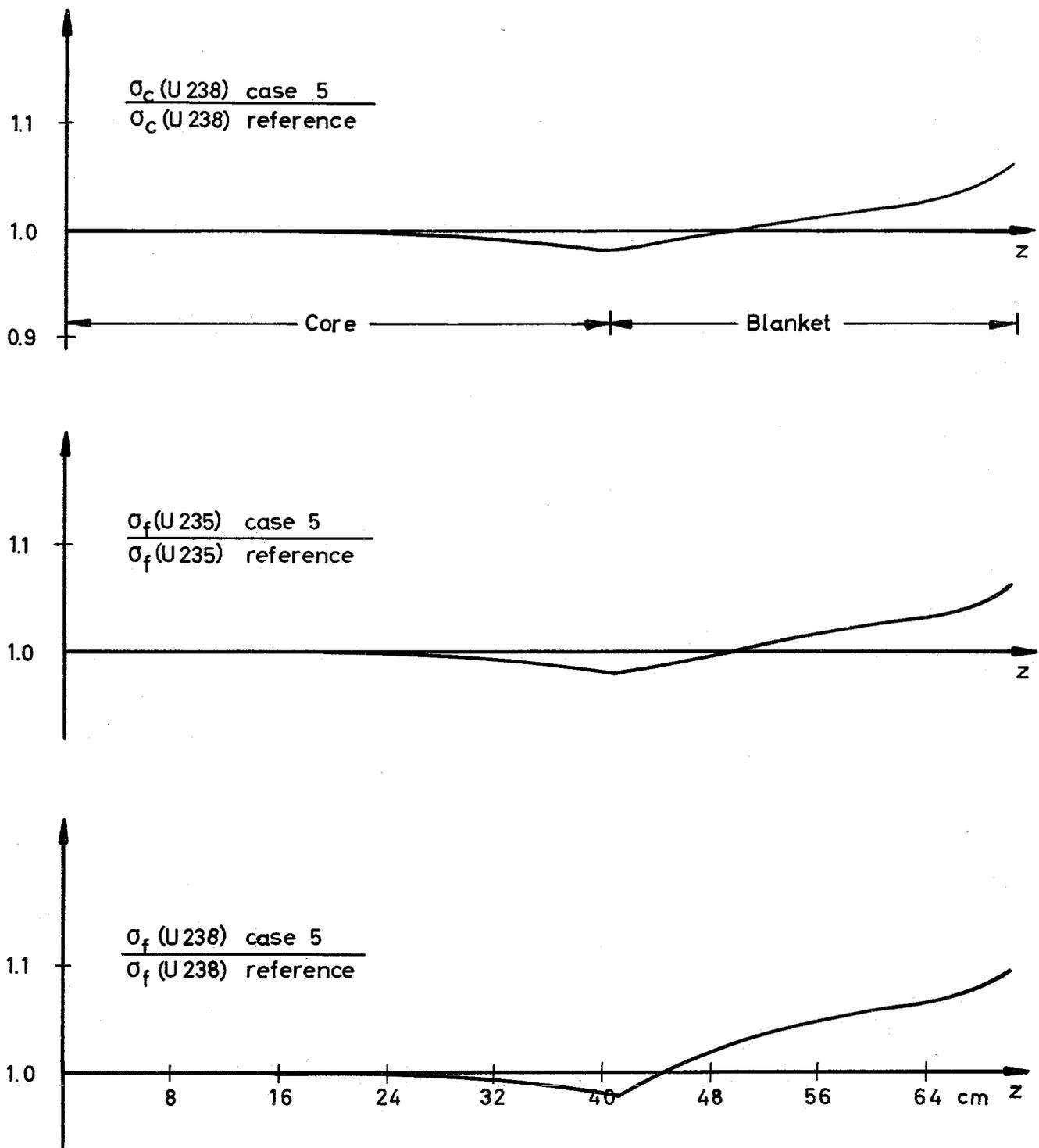
Fig. 5a Case 5: Influence of a 5% reduction of the transport cross section  $\Sigma_{tr}$  for the blanket composition on the reaction rate traverses.
