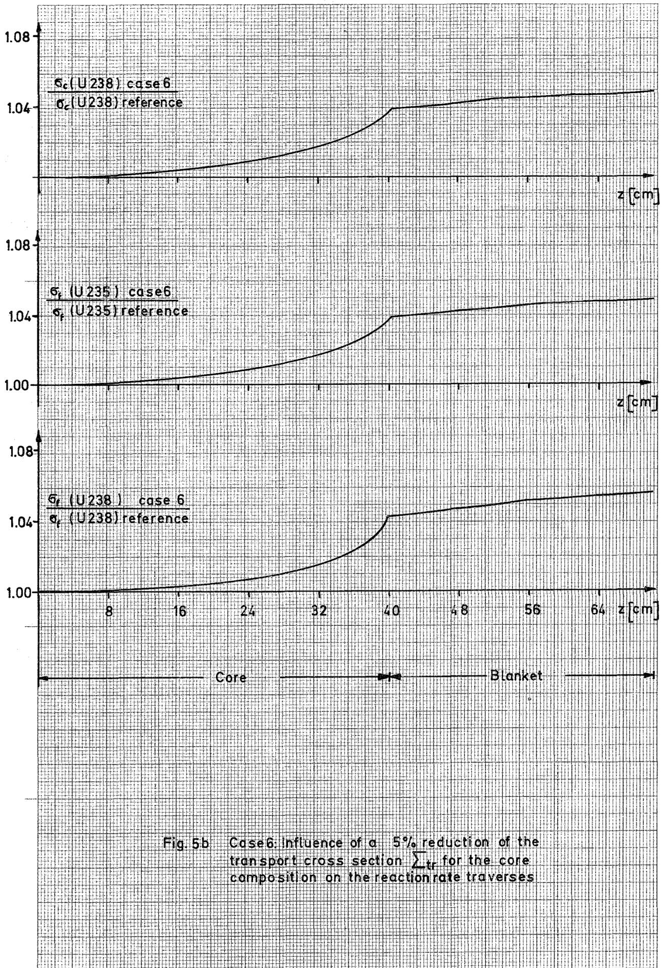
Fig. 5b Case 6: influence of a 5% reduction of the transport cross section  $\Sigma_{tr}$  for the core composition on the reaction rate traverses
