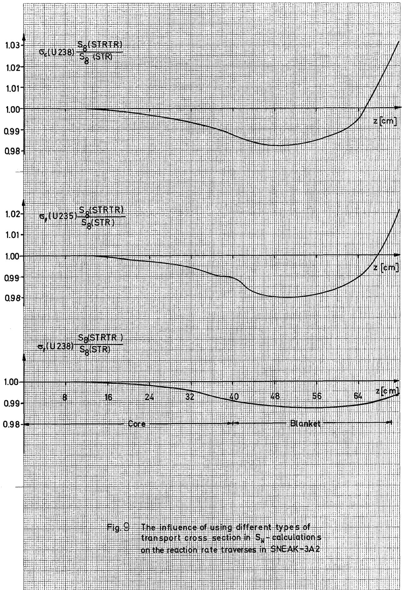
Fig. 9 The influence of using different types of transport cross section in  $S_N$ -calculations on the reaction rate traverses in SNEAK-3A2
