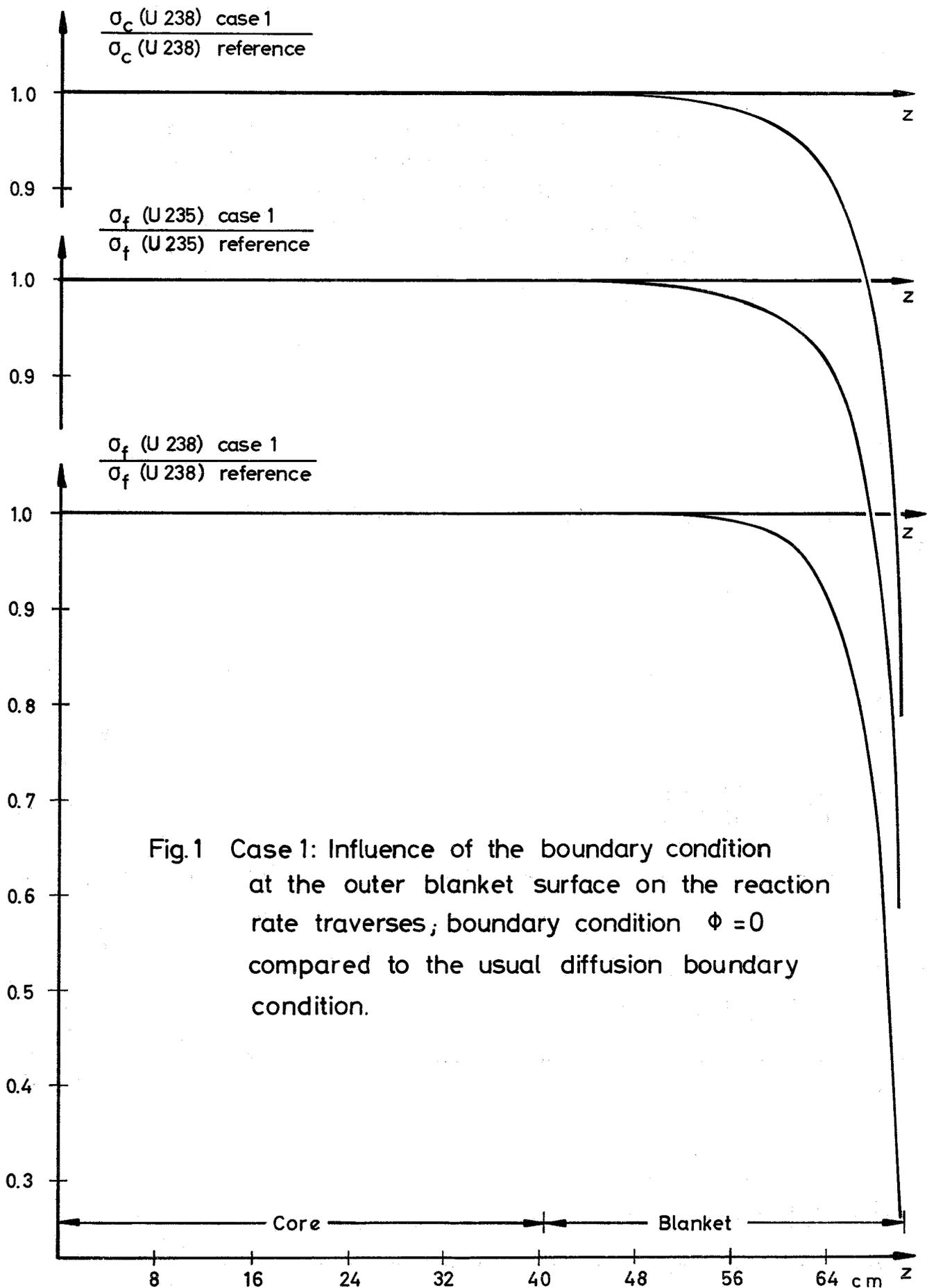
Fig.1 Case 1: Influence of the boundary condition at the outer blanket surface on the reaction rate traverses; boundary condition  $\Phi = 0$  compared to the usual diffusion boundary condition.
