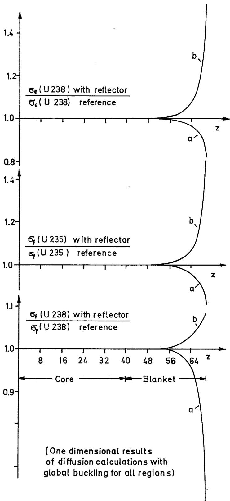
Fig. 13 A : Influence of reflectors on the reaction rate traverses
