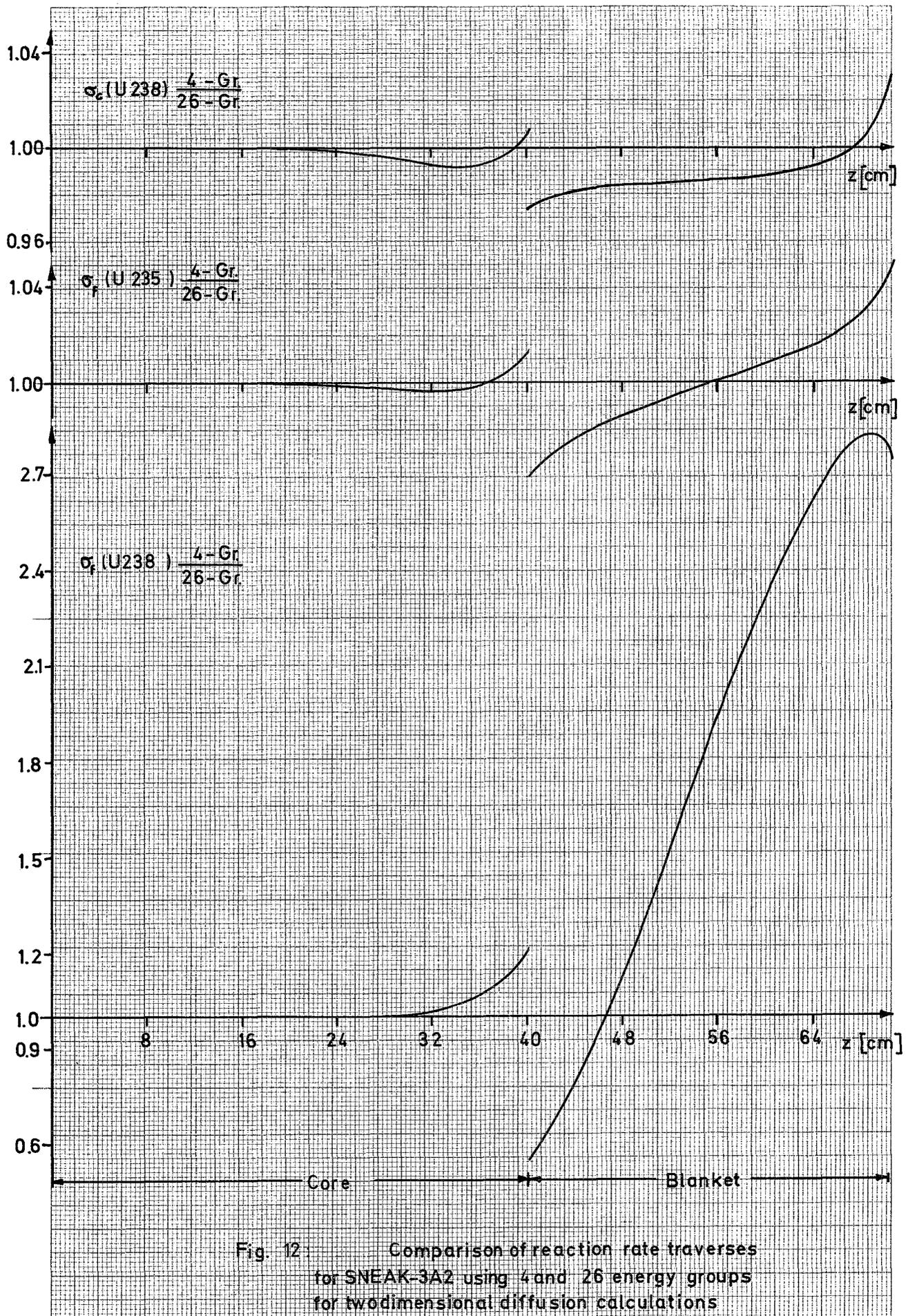
Fig. 12: Comparison of reaction rate traverses for SNEAK-3A2 using 4 and 26 energy groups for twodimensional diffusion calculations
