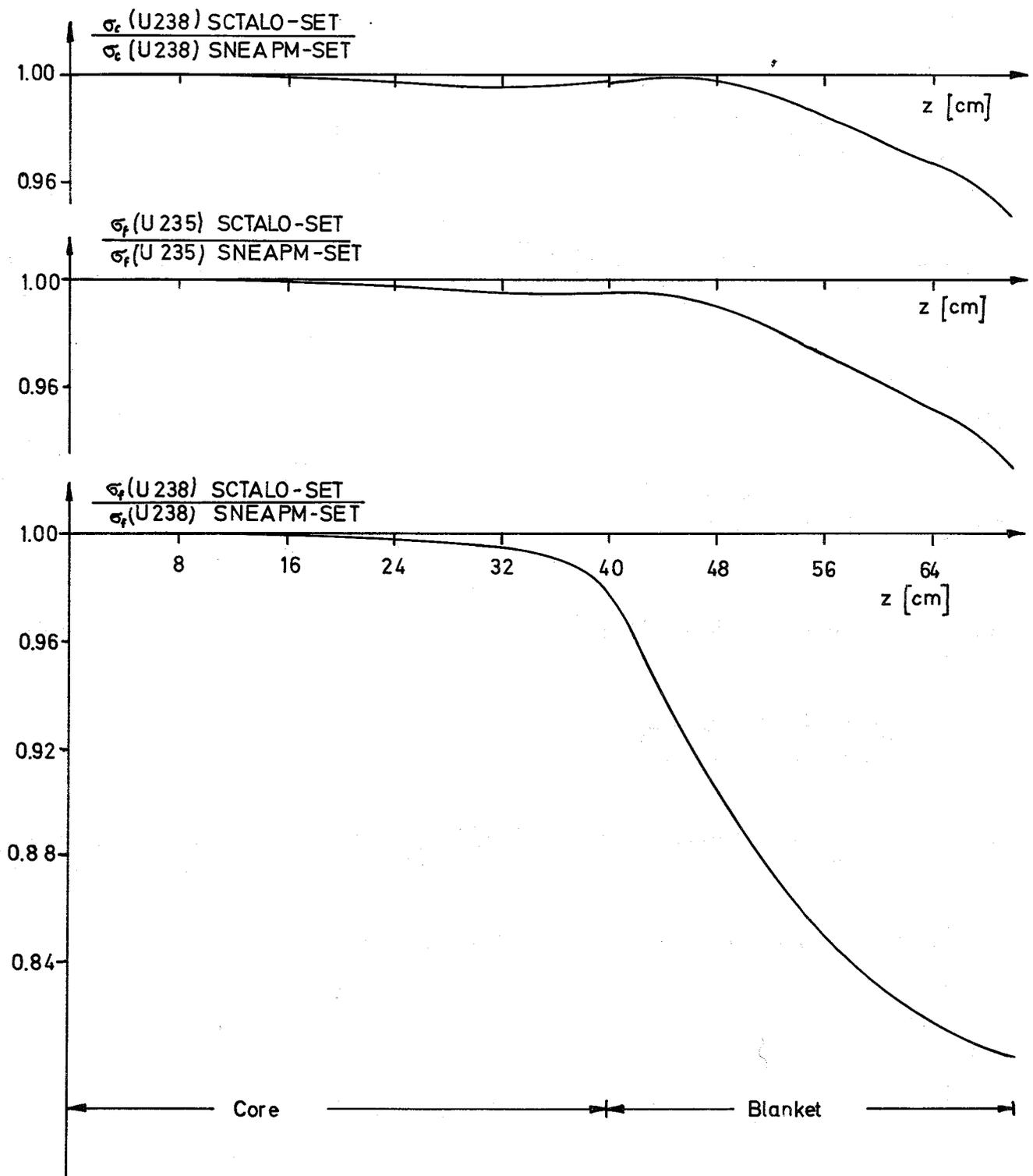
Fig.6b Influence of changes in the inelastic scattering probabilities on the reaction rate traverses in SNEAK-3A2
