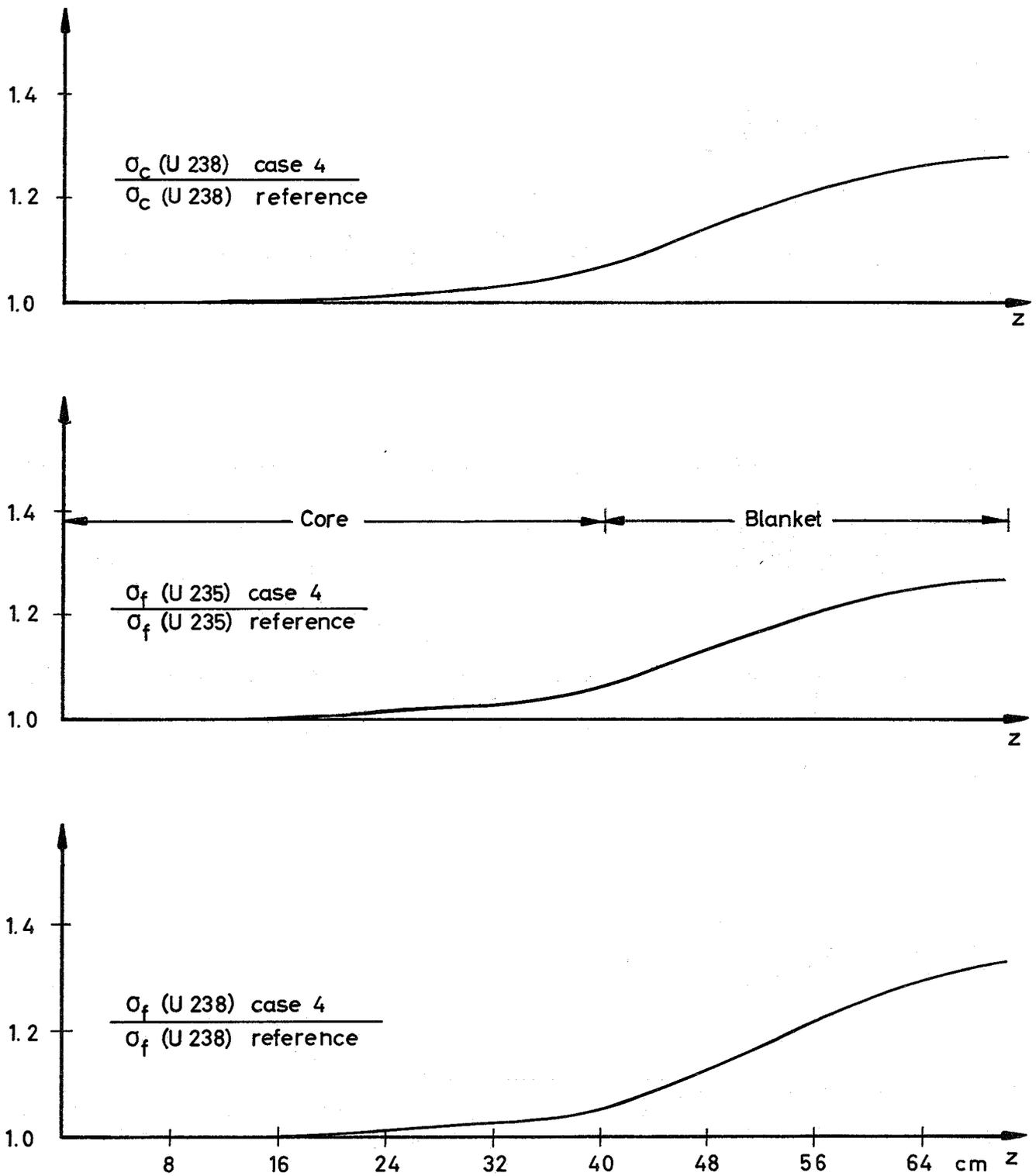
Fig.4 Case 4: Influence of a 5% reduction of  $\Sigma_{rem}$  for the blanket - composition on the reaction rate traverses.
