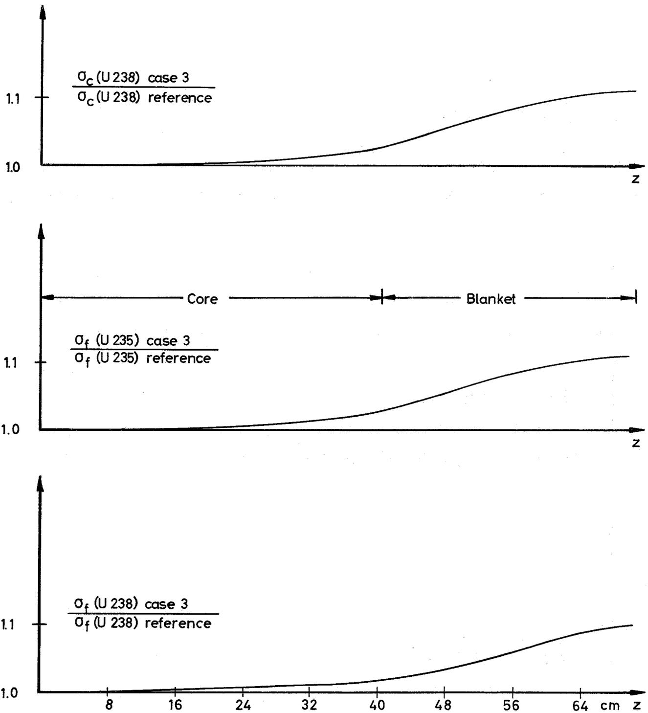
Fig. 3 Case 3: Influence of  $B_{\text{sep}}^2$  in the blanket region on the reaction rate traverses;  $B_{\text{sep}}^2 = 9.0 \cdot 10^{-4} \text{ cm}^{-2}$  for case 3,  $B_{\text{sep}}^2 = 16.949119 \cdot 10^{-4} \text{ cm}^{-2}$  for the reference case.
