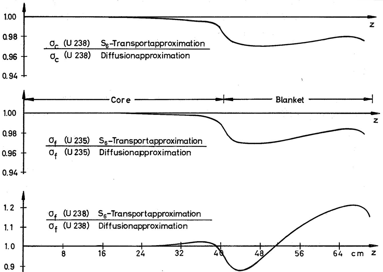
Fig. 8 Case: G4 Comparison of reaction rate traverses obtained by  $S_6$ -transport calculation to those obtained by diffusion calculation (MOXTOT-SET).
