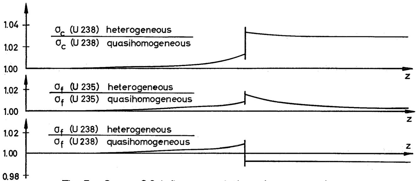
Fig. 7 Case: G2 Influence of the heterogeneity-effect on the reaction rate traverses.
