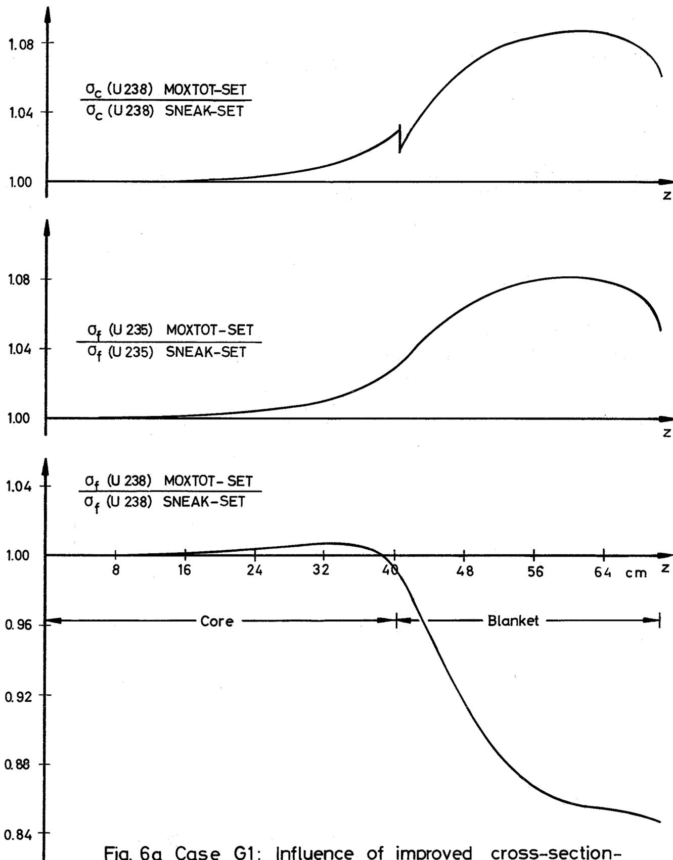
Fig. 6a Case G1: Influence of improved cross-section-set-data on the reaction rate traverses.
