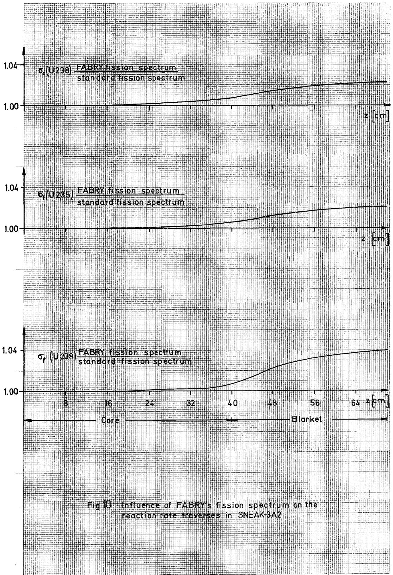
Fig.10 Influence of FABRY's fission spectrum on the reaction rate traverses in SNEAK-3A2
