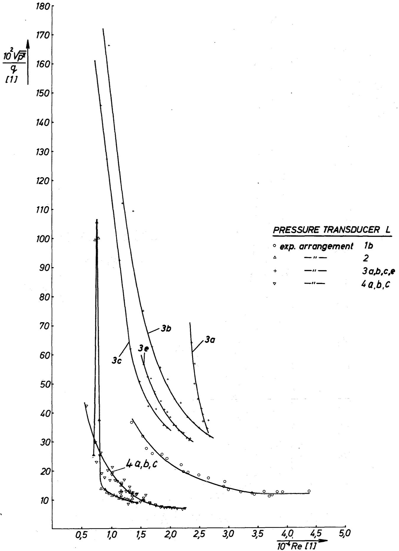
Fig. 6 RMS-values of pressure fluctuations in pin bundle
