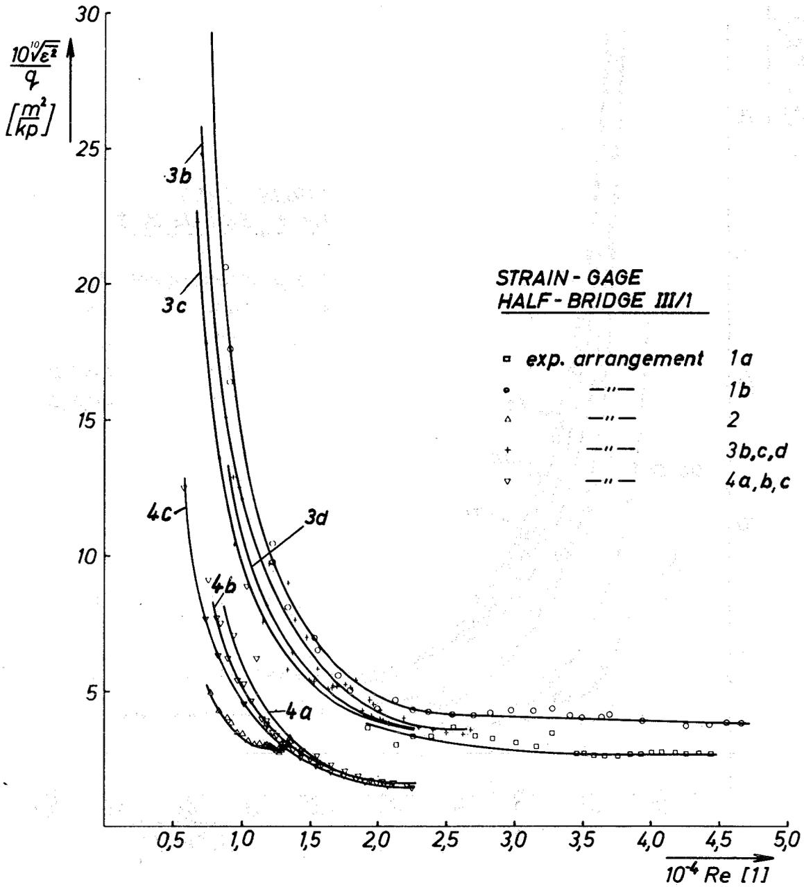
**Fig.7** RMS-values of bending strain of vibrating pin
