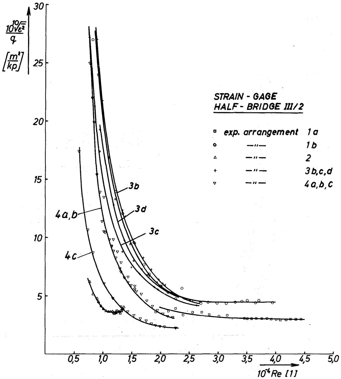
Fig.8 RMS-values of bending strain of vibrating pin No.III.
