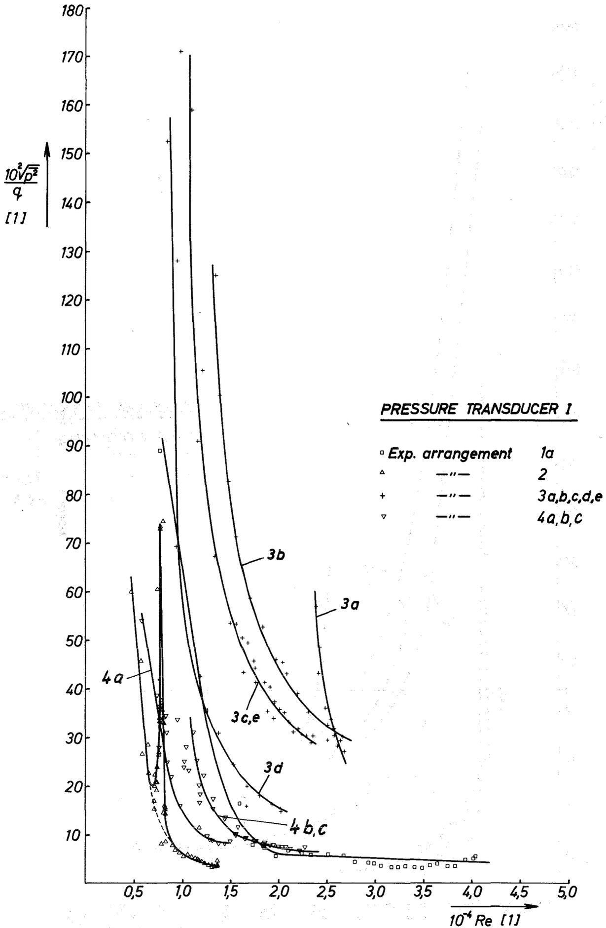
Fig.5 RMS-values of pressure fluctuations at water inlet in subassembly
