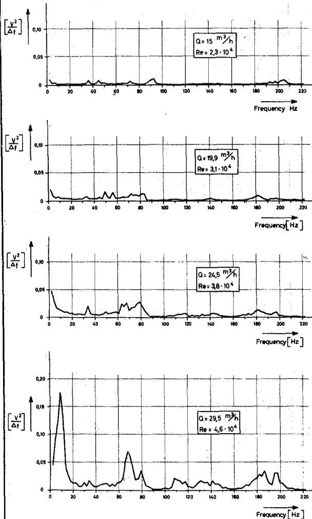
PRESSURE FLUCTUATIONS (DA L), in test section
