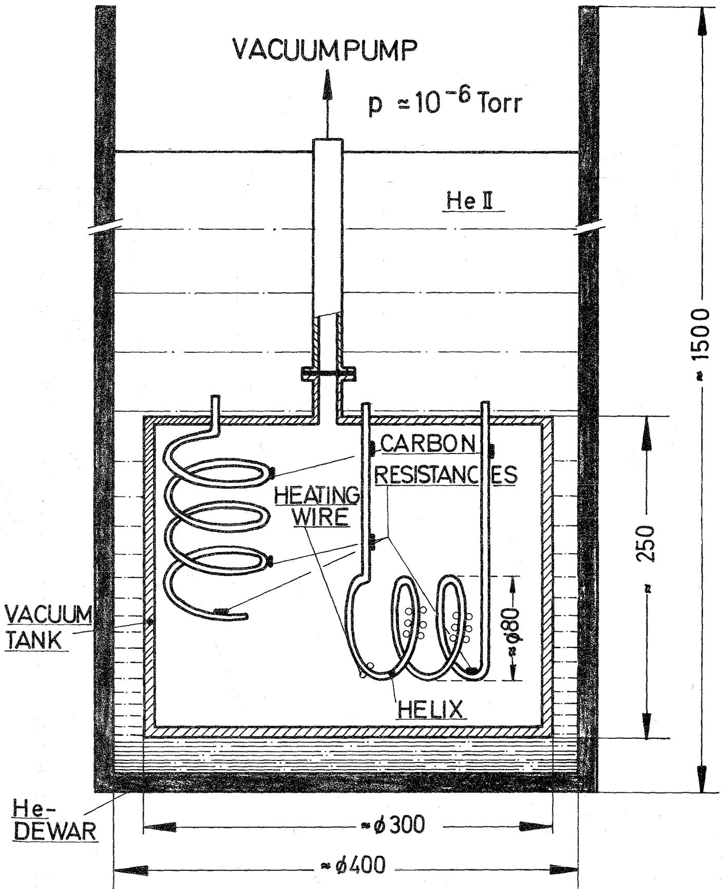
CRYOSTAT WITH VACUUM TANK AND HELICES
