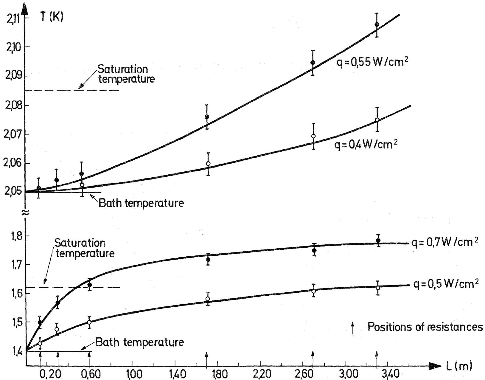
Temperature distribution along the helix ( $d = 0,8 \text{ cm}$ , one end closed) for two bath temperatures and heat-current densities with heater location at  $L = 3,30 \text{ m}$
