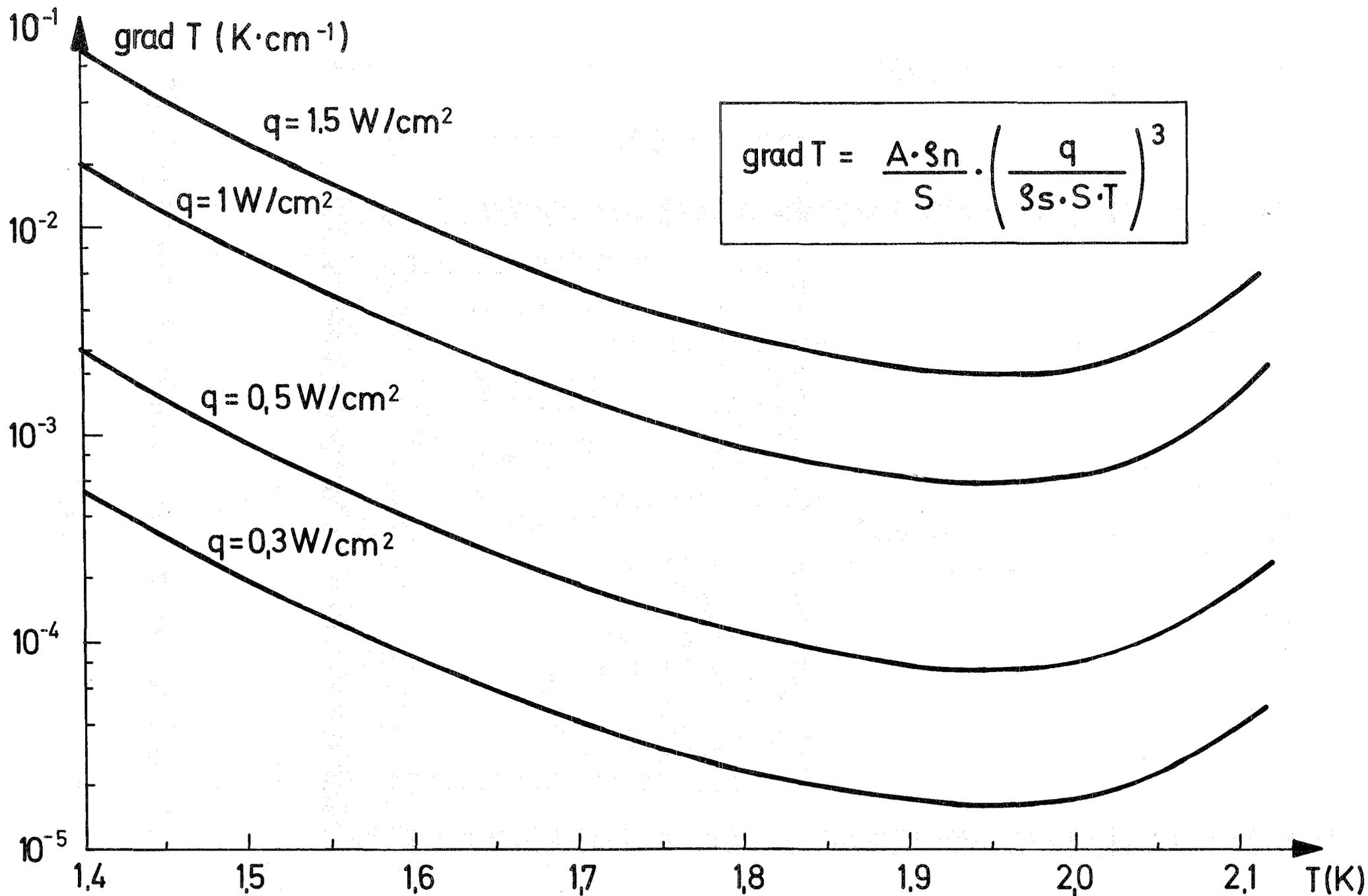
Temperature gradient as a function of heat-current density and temperature
