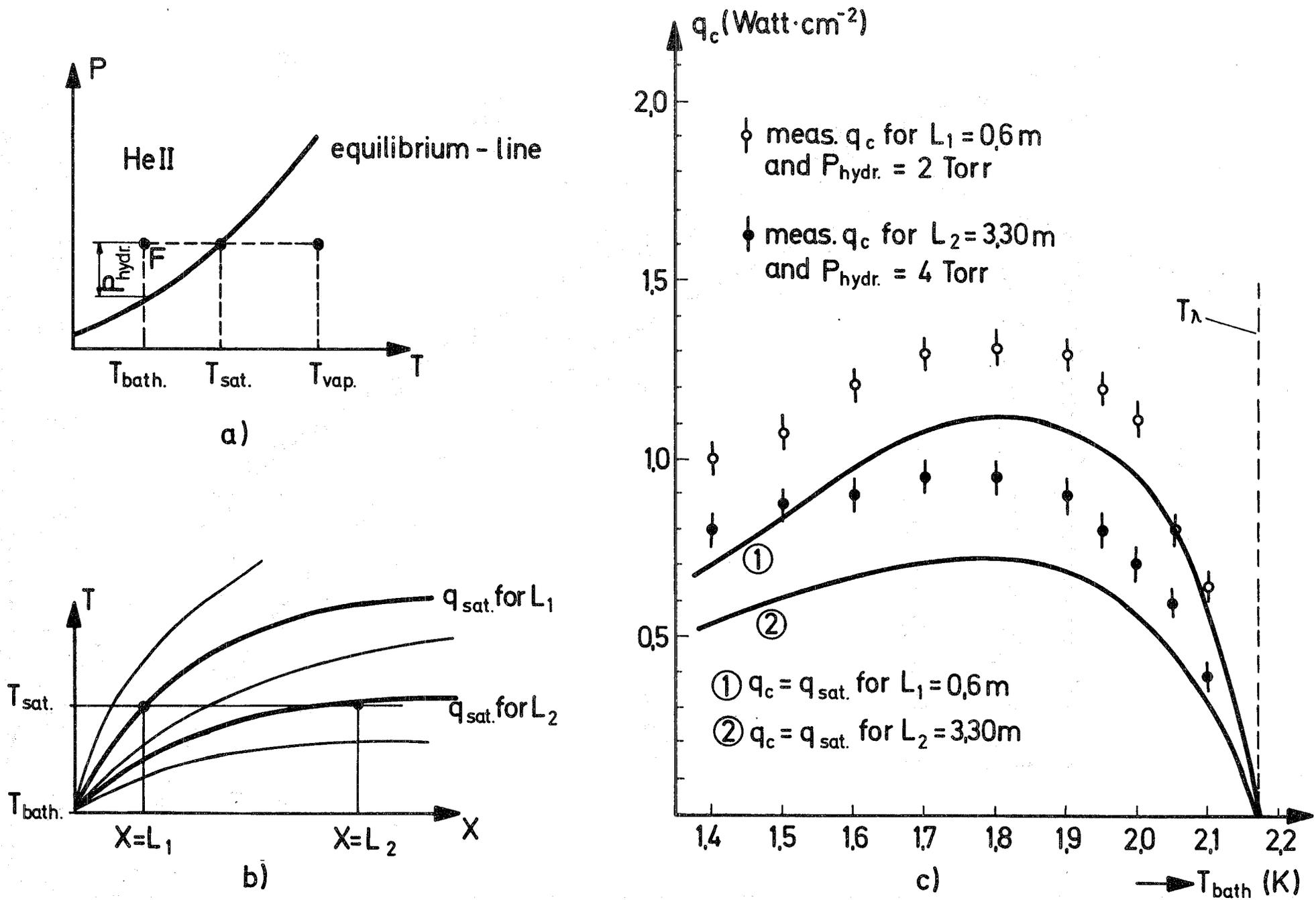
CRITICAL HEAT FLOW DENSITIES FOR DIFFERENT TUBE LENGTHS AND BATH TEMPERATURES
