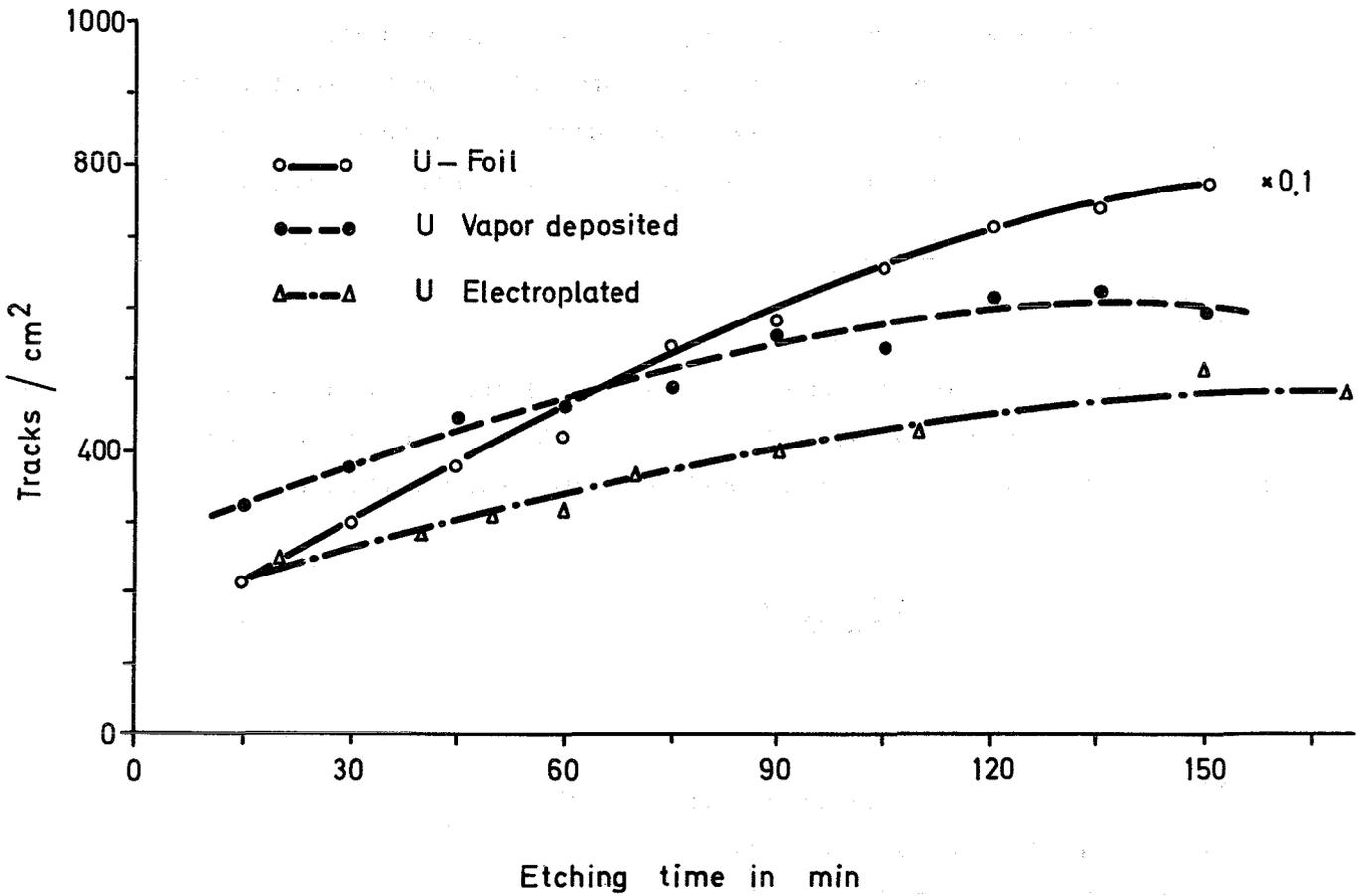
Fig. 4: Number of fission tracks counted in Makrofol with the spark counter as a function of etching time for a electroplated, vapor deposited and metallic uranium
