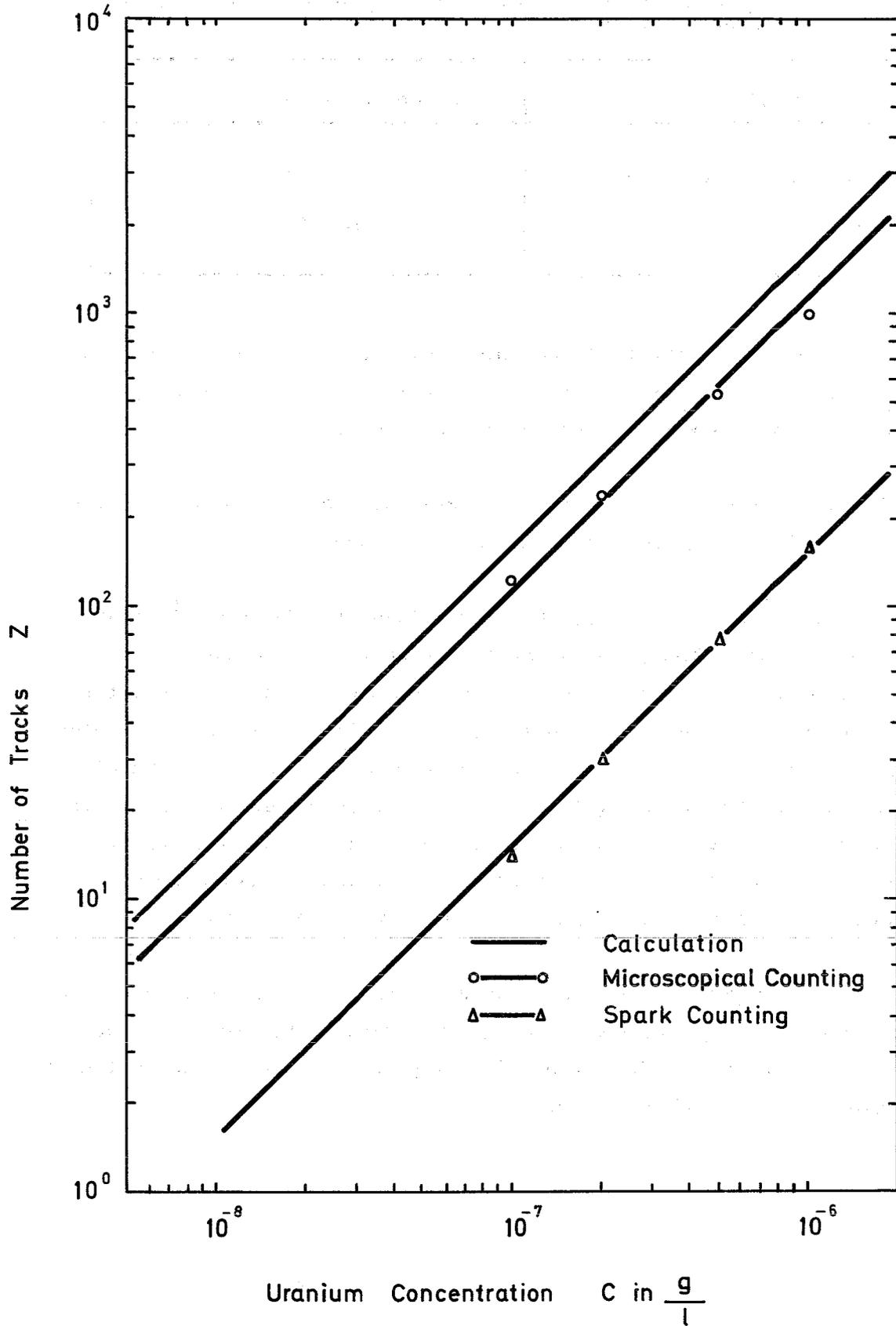
Fig. 5: Number of fission tracks in thick Makrofol foils as a function of the uranium concentration in water from a 0.2 ml sample after reactor irradiation with  $7 \times 10^{14}$  n/cm<sup>2</sup> for microscopical counting and spark counting
