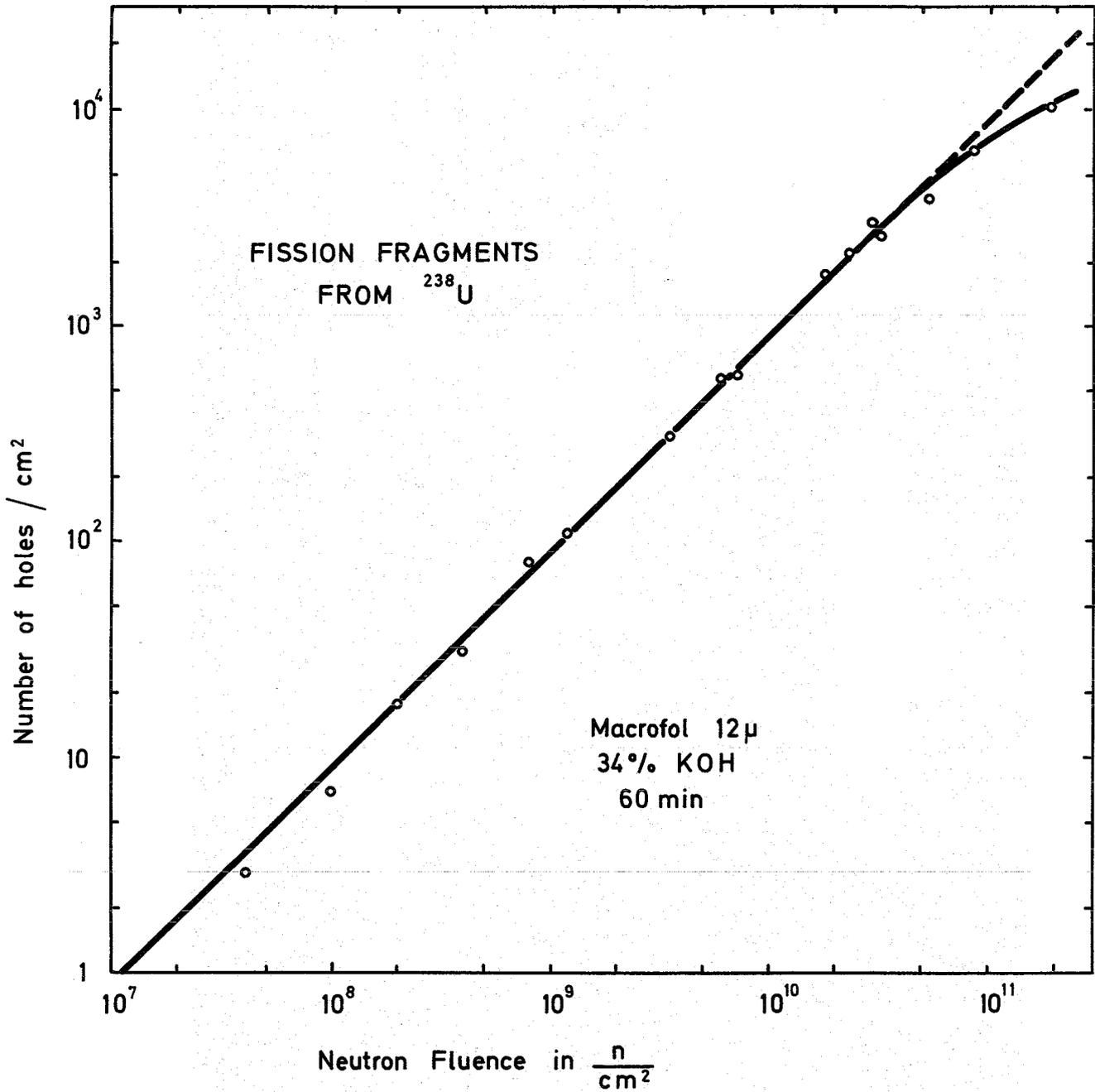
Fig. 3: Number of fission fragments in Makrofol counted with the spark counter as a function of neutron fluence from electroplated uranium
