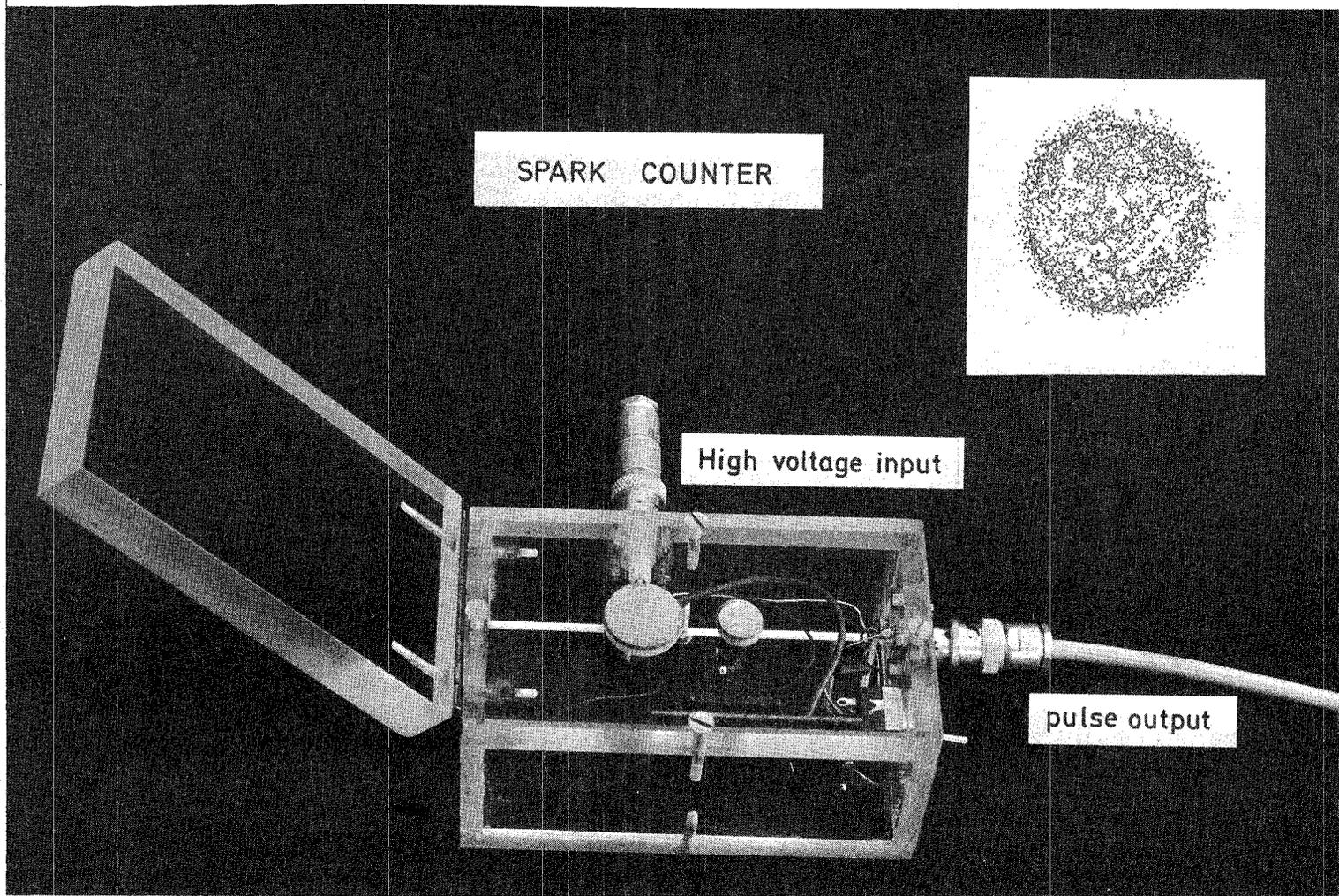
Fig. 2: Spark counter device and replica of etch pits in the mylar foil after spark counting
