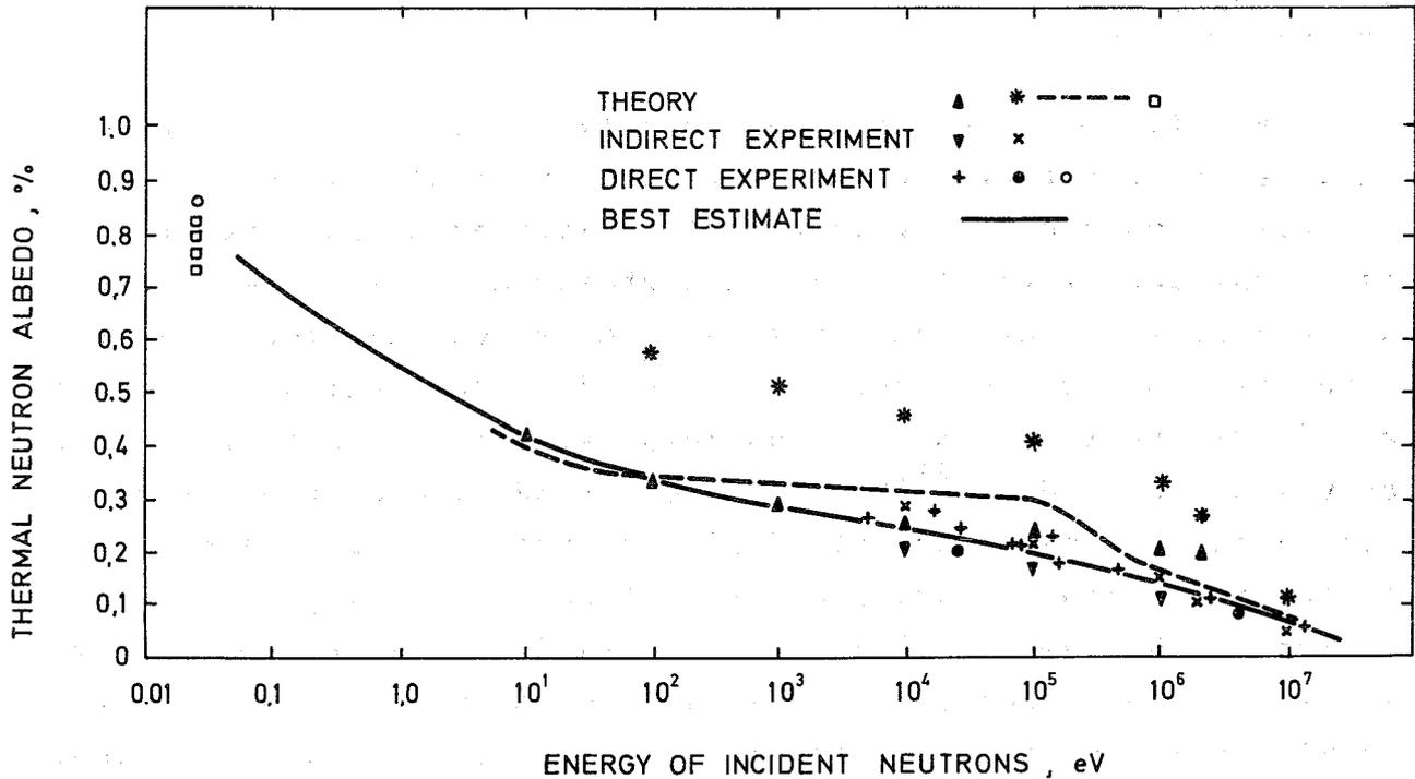
Fig. 1: The thermal neutron albedo as a function of incident neutron energy [3].
