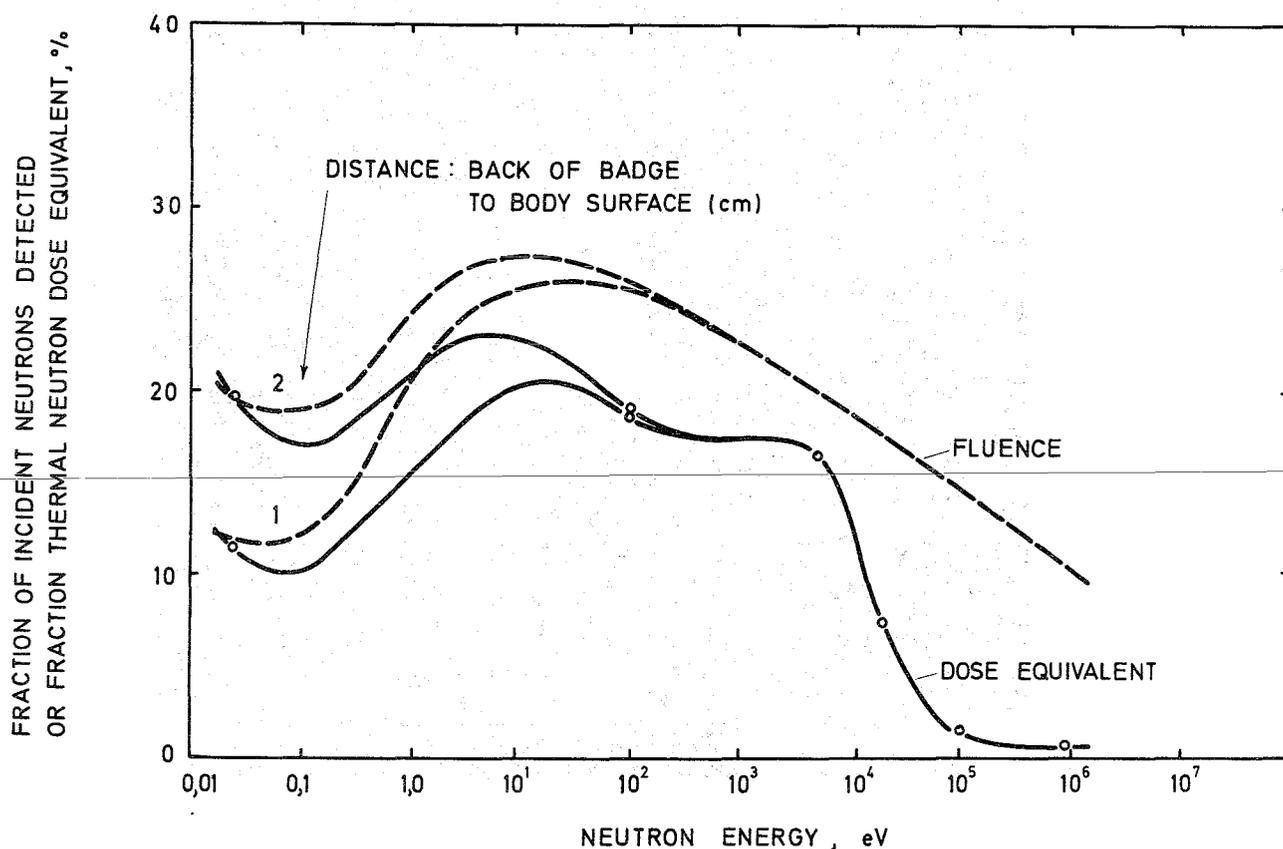
Fig. 6: The response of the LiF albedo dosimeter with the boron shield, worn on the body, as a function of incident neutron energy [3].
