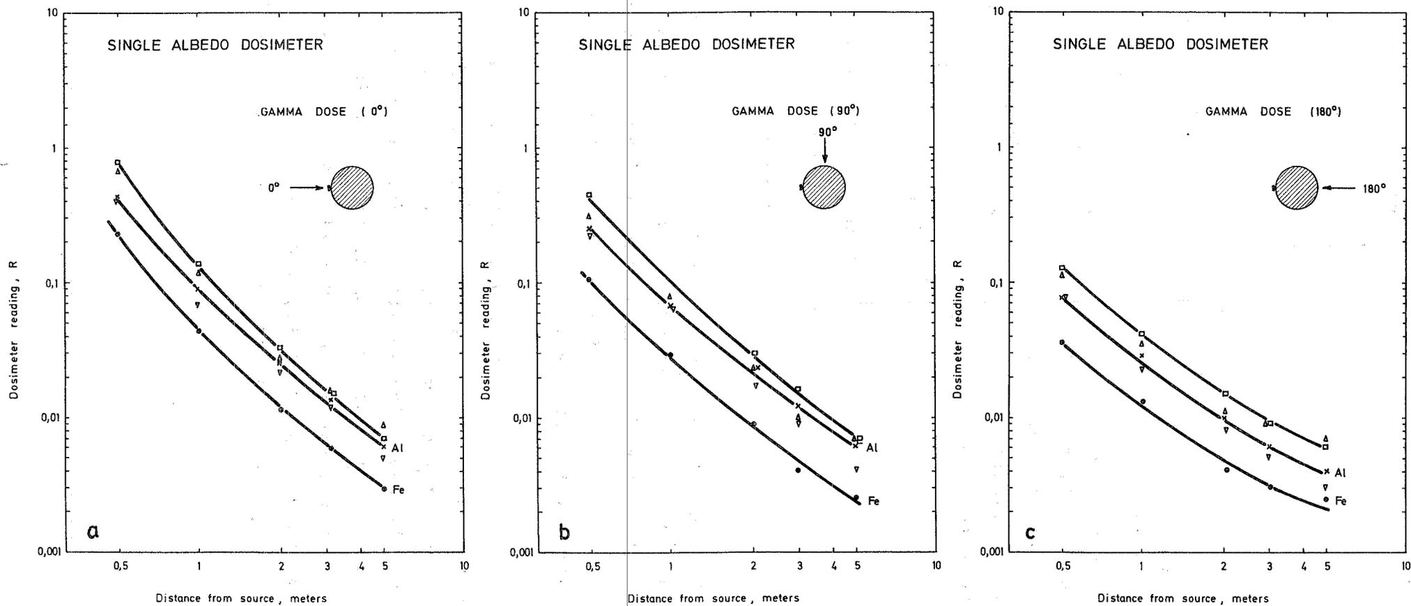
Fig.2o: The gamma-dose reading of TLD 700 on the front of the phantom as a function of distance from the source for radiation incidence angles of  $0^\circ$  (a),  $90^\circ$  (b) and  $180^\circ$  (c)
