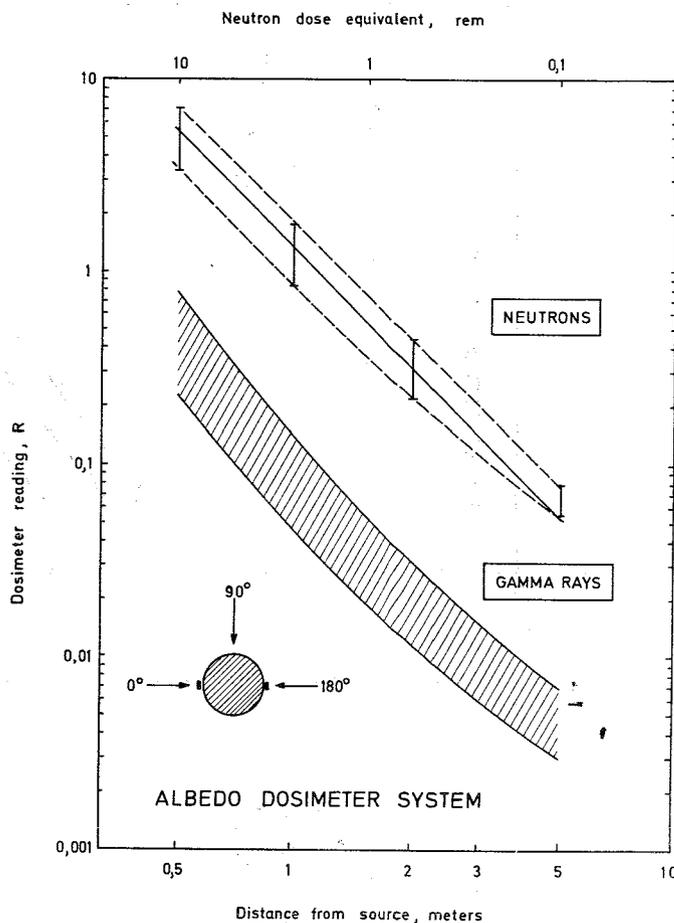
The dosimeter readings per dose equivalent of 1 rem are shown in Fig. 18 as a function of the distance to the  $^{252}\text{Cf}$  source. For distances of more than 1 m from the source we find an average value of 0.54 R/rem, which is 10 % greater than the corresponding value of the single albedo dosimeter.
