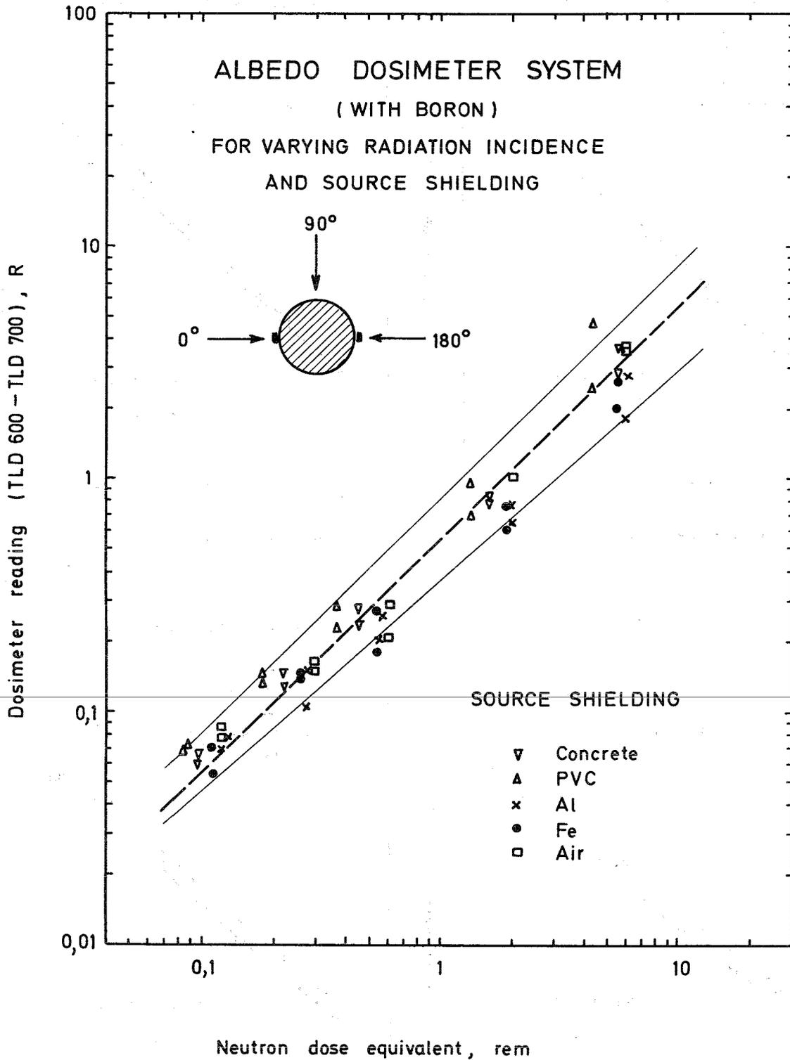
Fig.16: The dosimeter reading of the albedo dosimeter system with the boron shield as a function of dose equivalent for varying radiation incidence angle and source shielding.
