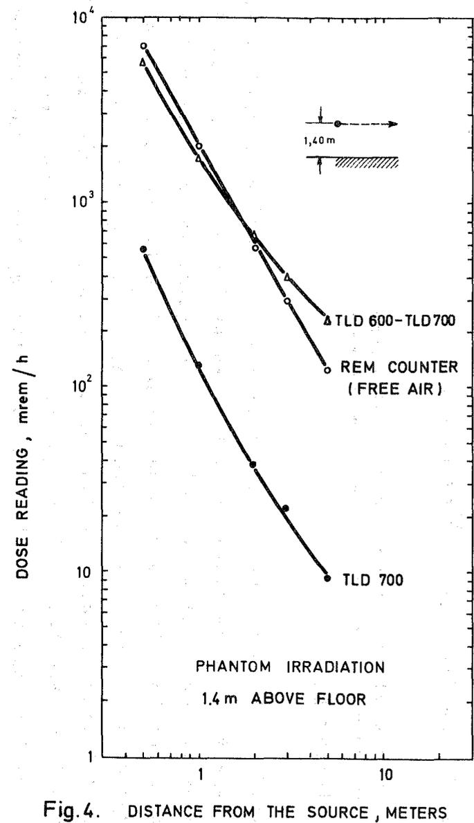
The main purpose of our experiments was to study the properties of a simple LiF albedo dosimeter to monitor the personal neutron dose in the field of a  $^{252}\text{Cf}$ -source.
