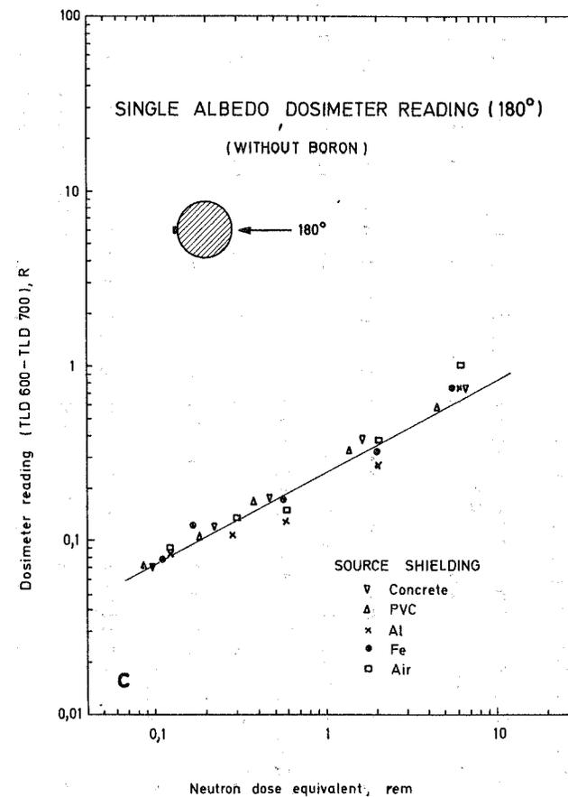
Fig.11: The dosimeter reading of a single albedo dosimeter without boron shield as a function of neutron dose equivalent for radiation incidence angles of  $0^\circ$  (a)  $90^\circ$  (b) and  $180^\circ$  (c)
