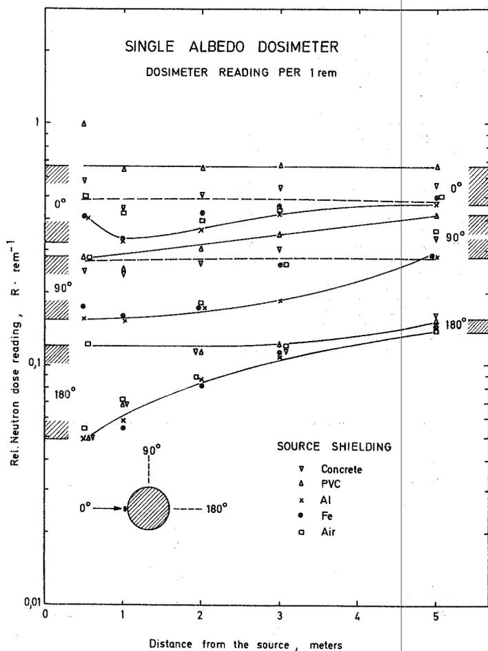
Fig.13: The neutron response of the single albedo dosimeter
