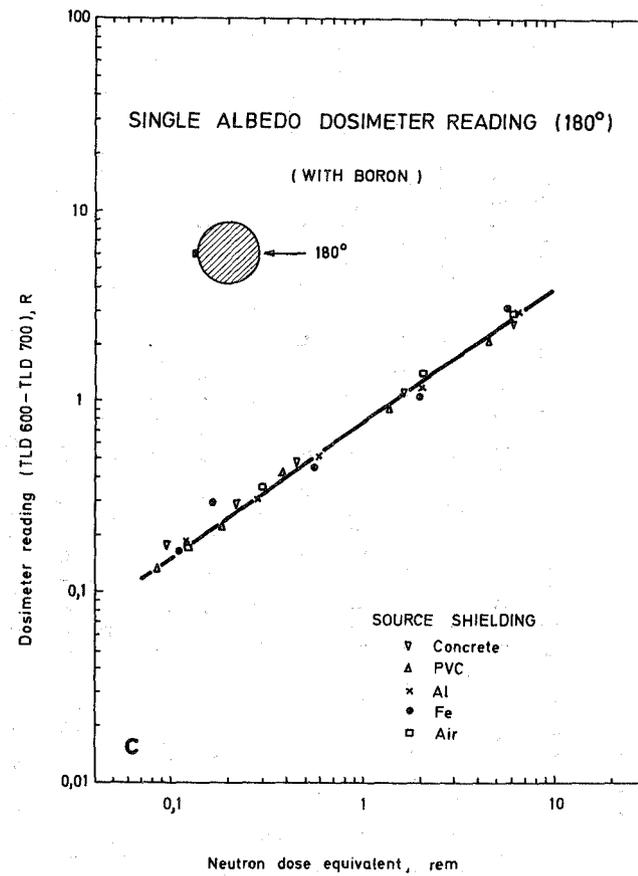
Fig.12: The dosimeter reading of a single albedo dosimeter with the boron shield as a function of neutron dose equivalent for radiation incidence angles of  $0^\circ$  (a),  $90^\circ$  (b) and  $180^\circ$  (c)
