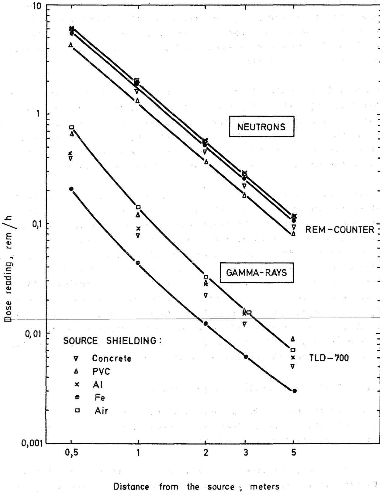
Fig.8: The dosimeter reading of TLD 700 and the Rem-counter reading in the field of the  $^{252}\text{Cf}$  source for various source shieldings.
