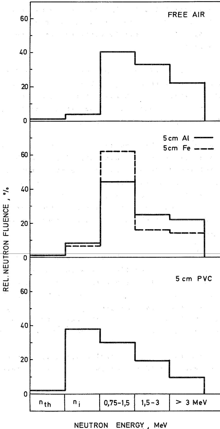
Fig.9: The neutron-energy distribution of <sup>252</sup>Cf-neutrons for various source shieldings of 5 cm thickness
