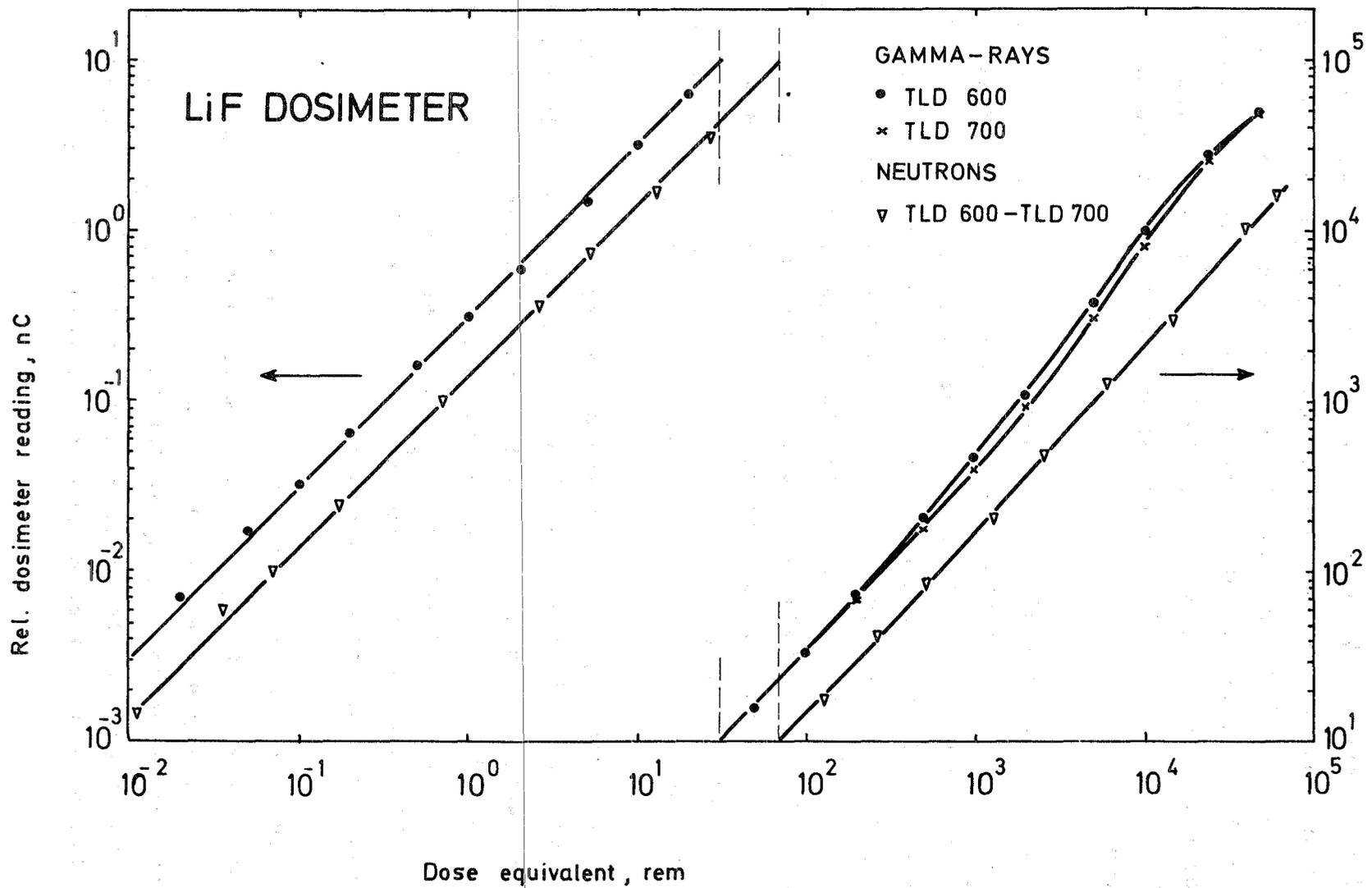
Fig.5: The relative dosimeter reading of LiF dosimeters as a function of dose equivalent for gamma irradiation and of an albedo dosimeter for  $^{252}\text{Cf}$  neutron irradiation
