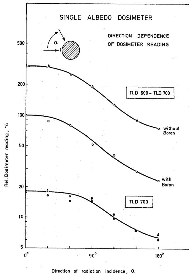
Fig.14: The direction dependence of the single albedo dosimeter reading
