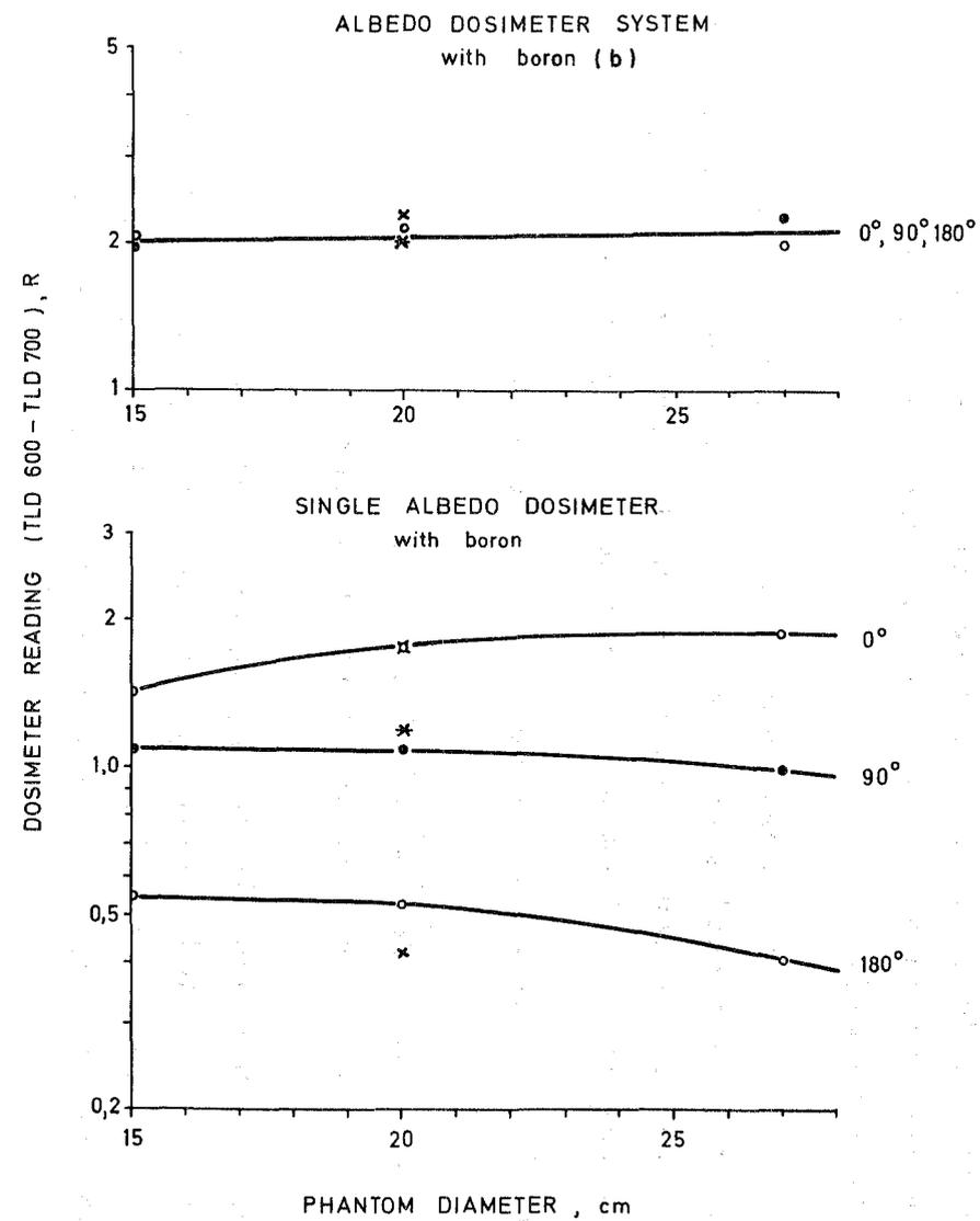
Fig.22: The dosimeter reading of the albedo dosimeter with and without boron shield as a function of phantom size for various radiation incidence angles.
