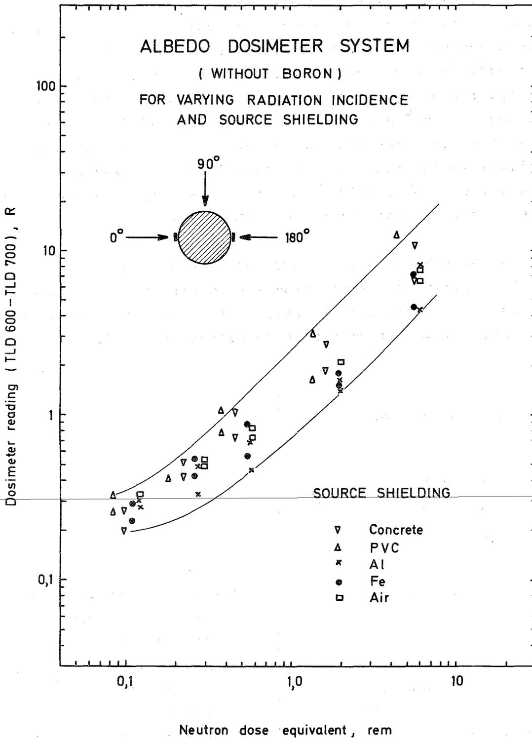
Fig.17: The dosimeter reading of the albedo dosimeter system without boron shield as a function of dose equivalent for varying radiation incidence angle and source shielding.
