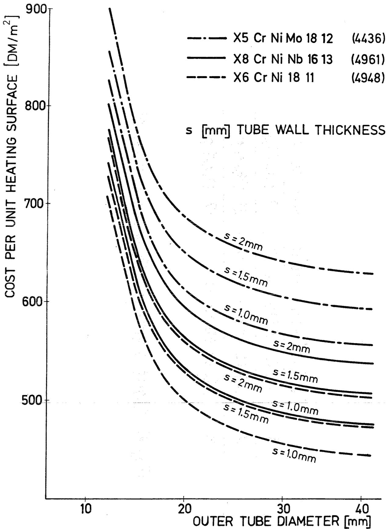
Fig. 5 Cost per Unit Heating Surface Versus Outer Tube Diameter
