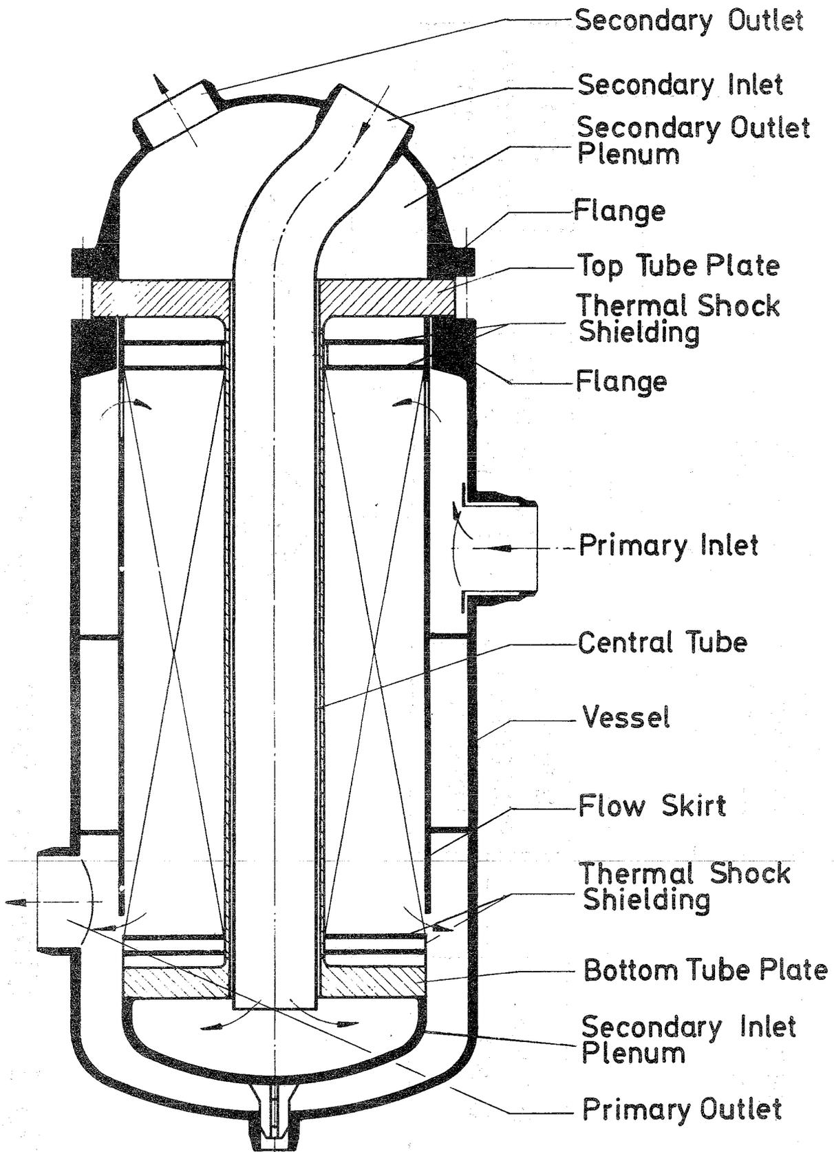
Fig. 1 Sodium/Sodium Intermediate Heat Exchanger Cross Section
