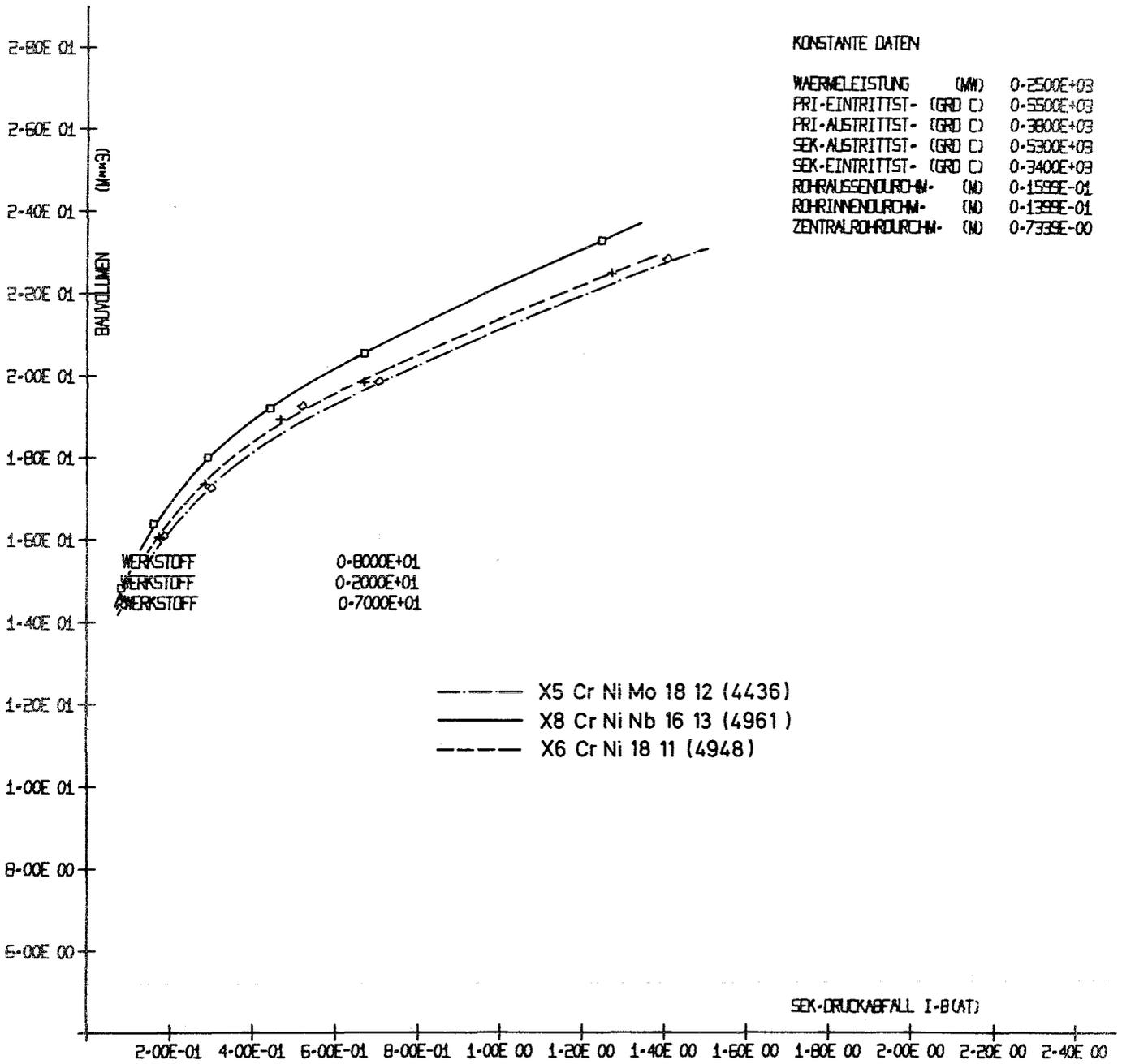
Fig. 15 Total Heat Exchanger Volume Versus Secondary Pressure Drop
