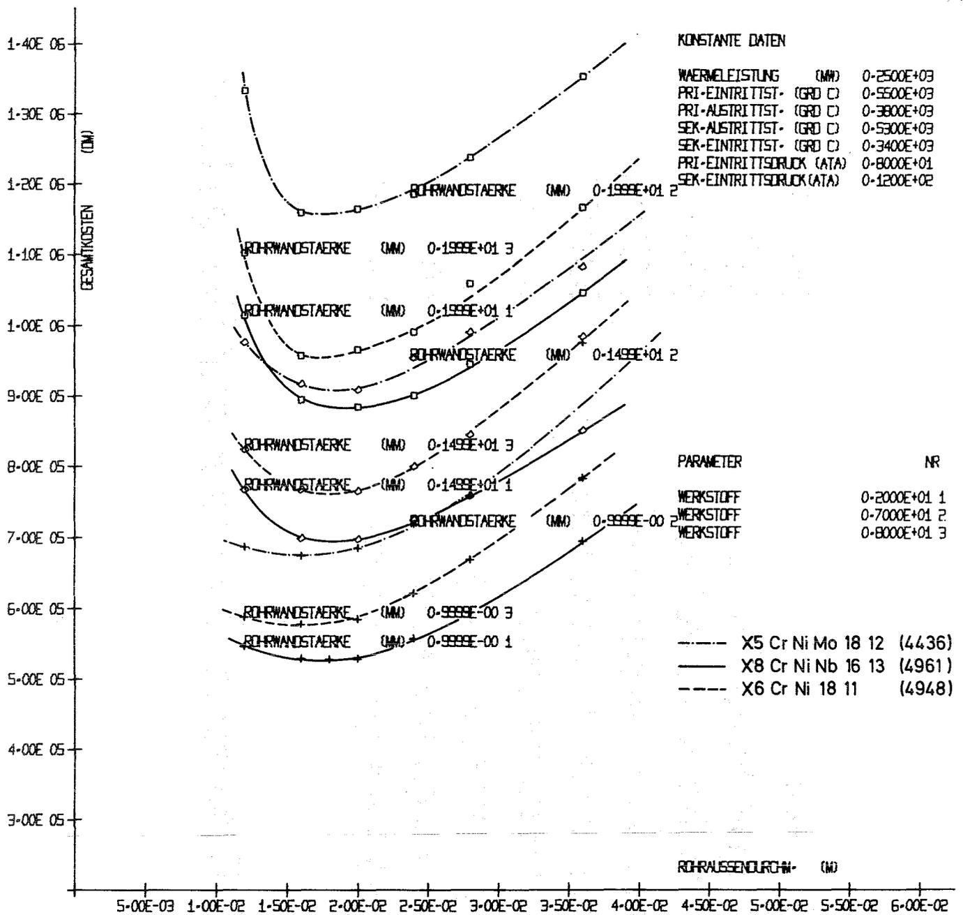
Fig. 8 Total Heat Exchanger Costs Versus Tube Outer Diameter
