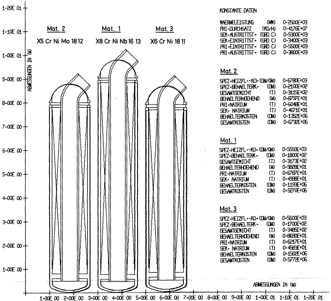
Fig. 9 Comparison of Optimum Heat Exchanger Design for three Different Austenitic Materials
