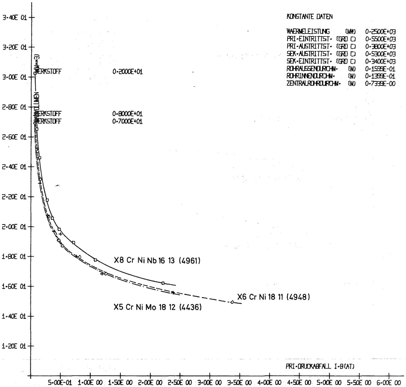
Fig. 13 Total Heat Exchanger Volume Versus Primary Pressure Drop
