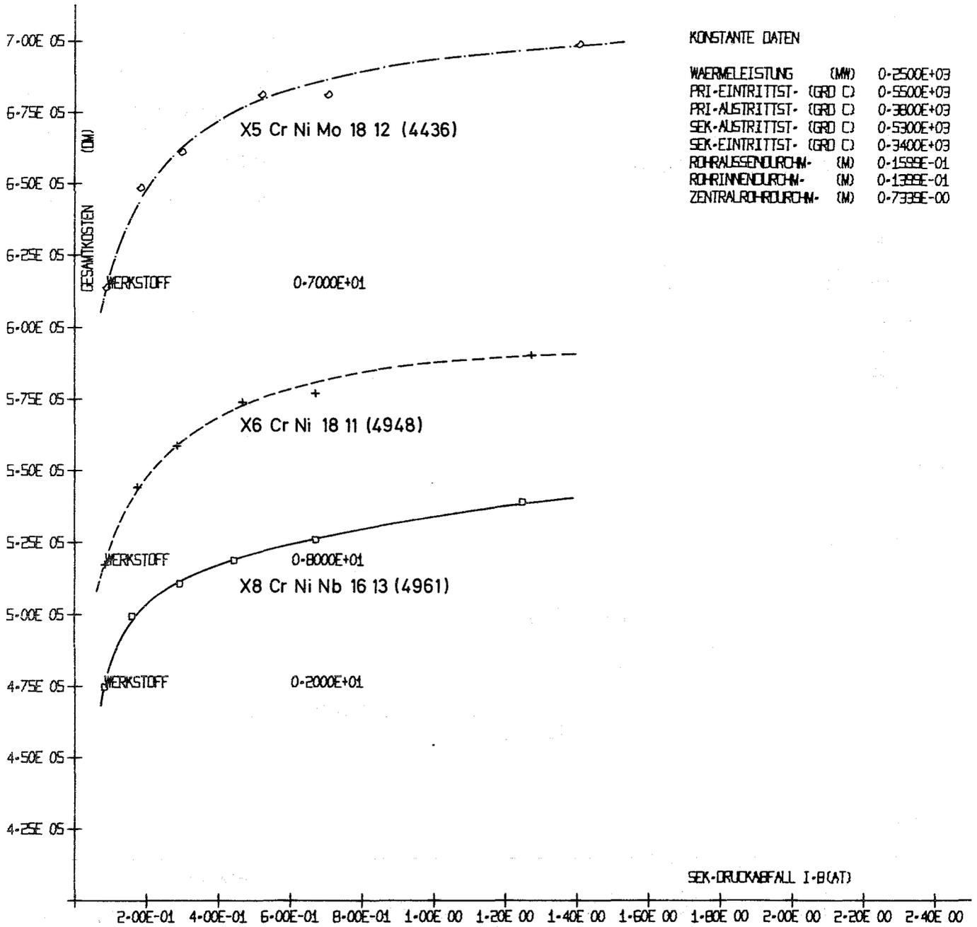
Fig. 14 Total Heat Exchanger Costs Versus Secondary Pressure Drop
