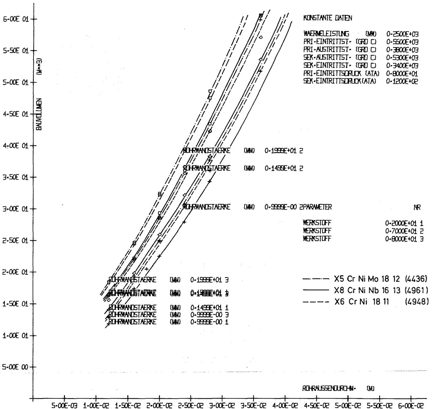
Fig. 11 Total Heat Exchanger Volume Versus Outer Tube Diameter
