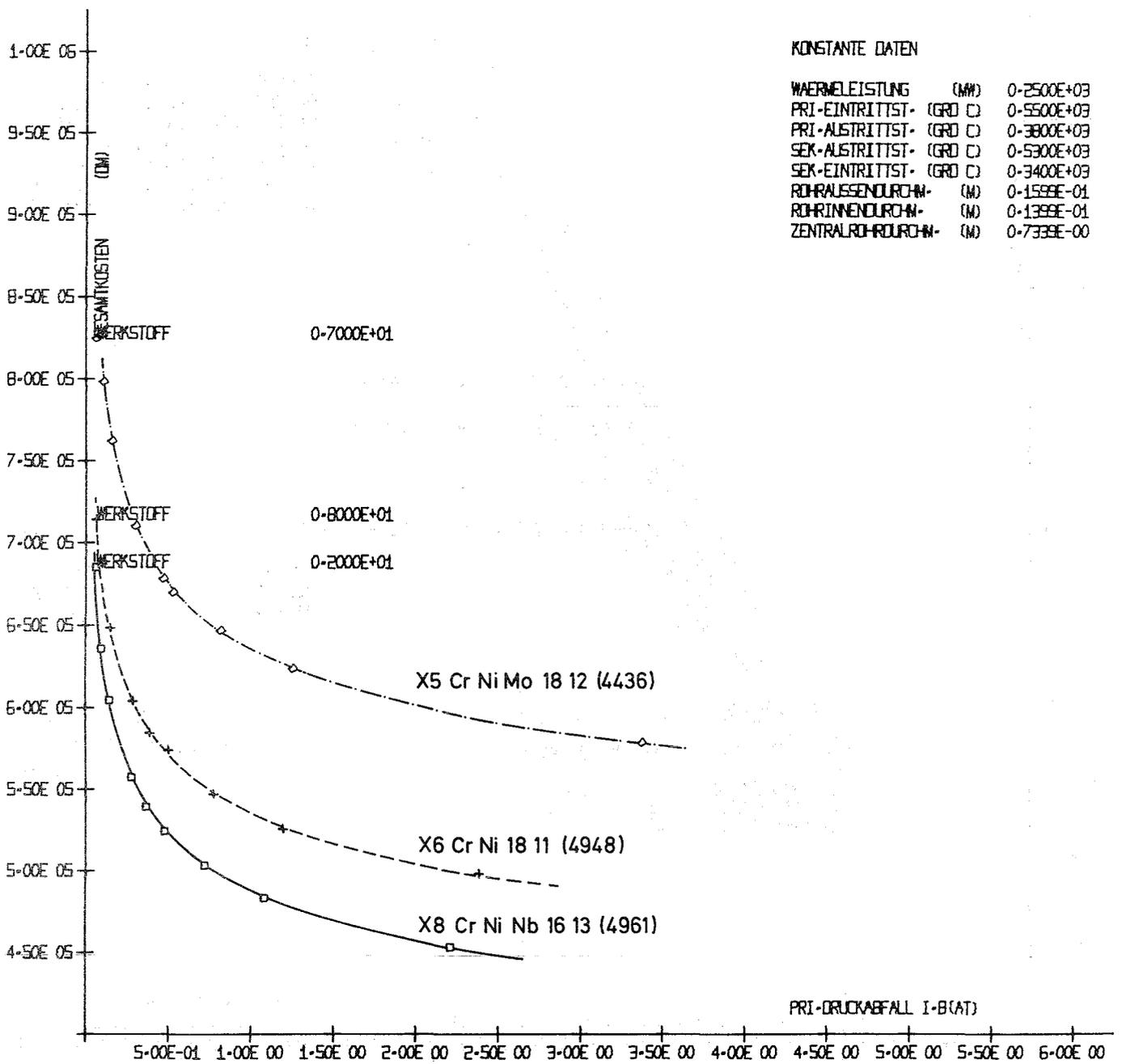
Fig. 12 Total Heat Exchanger Costs Versus Primary Pressure Drop
