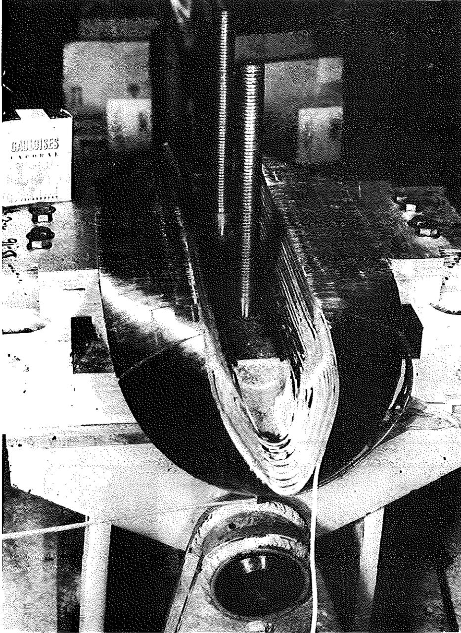
Fig. 9: Completed brass model showing winding technique of MOBY
