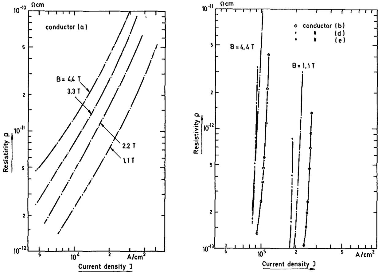
Fig. 2: Short sample characteristics: Resistivity versus current density for some selected conductors
