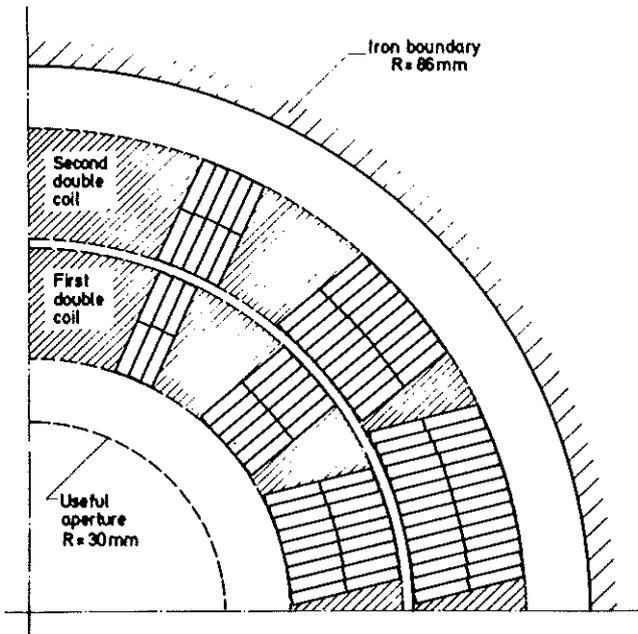
Fig. 11: Cross sections of a two double layer dipole using a flat cable
