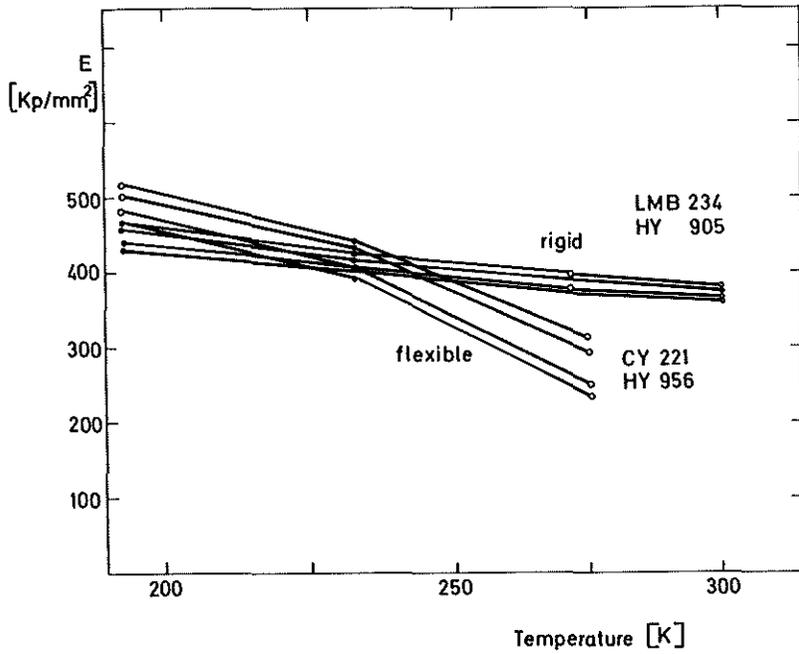
Young's modulus and relative thermal contraction vs temperature of un-filled epoxies. Flexible or rigid refers to their behaviour at room temperature.
