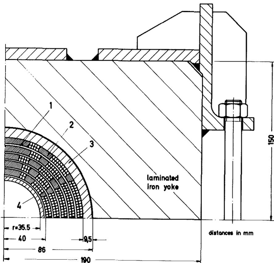
Dipole D2a cross section with conductor configuration (left) and longitudinal section with conductor end configuration (below):
