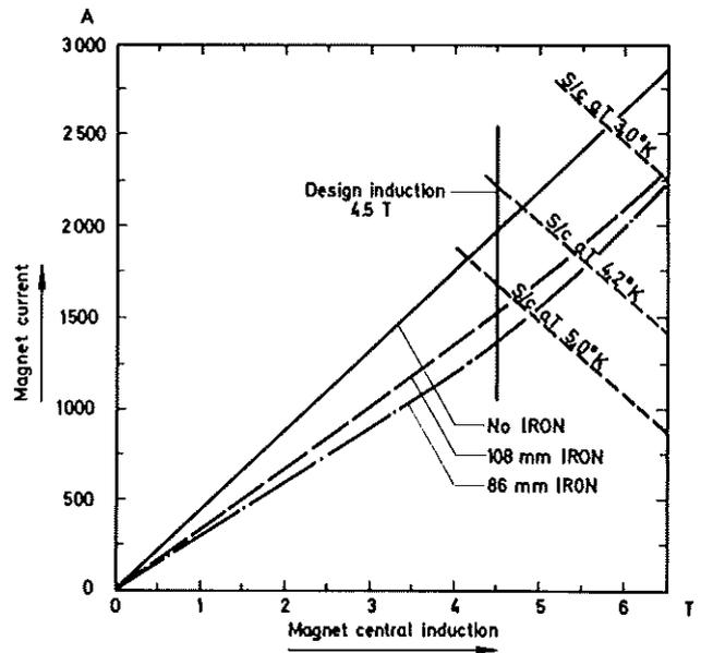
b) Field enhancement factor for saturated (86 mm) and unsaturated (108 mm) iron version
