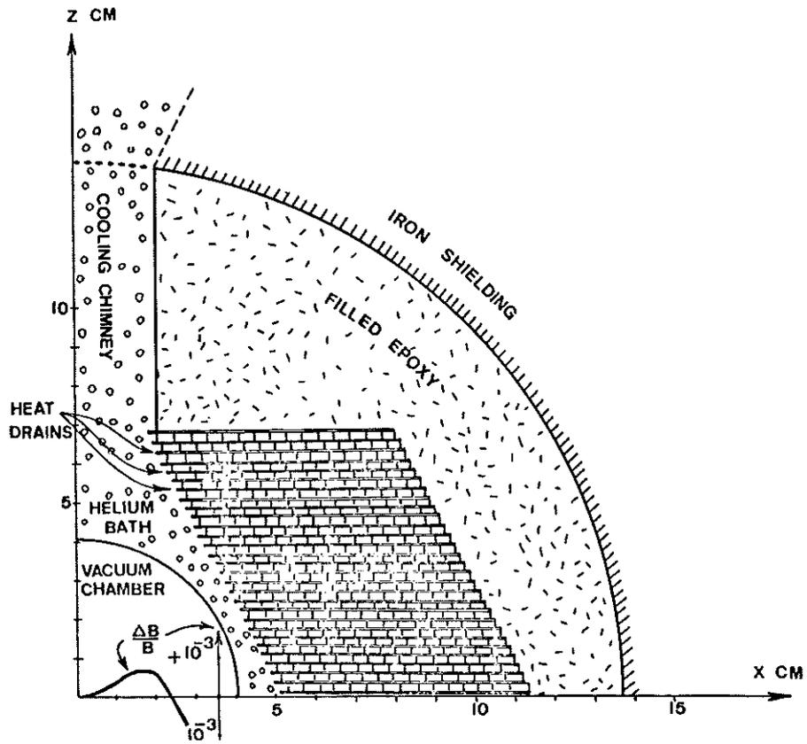
Fig. 8: Coil and iron shielding configuration of MOBY (CEN)
