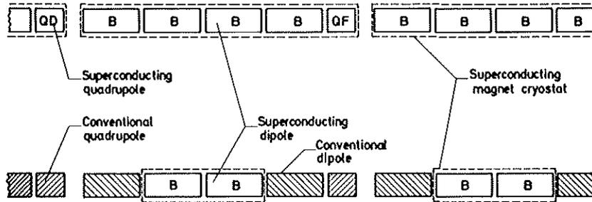
b) Mixed missing magnet ring (400 - 500 GeV with S/C magnets alone)
