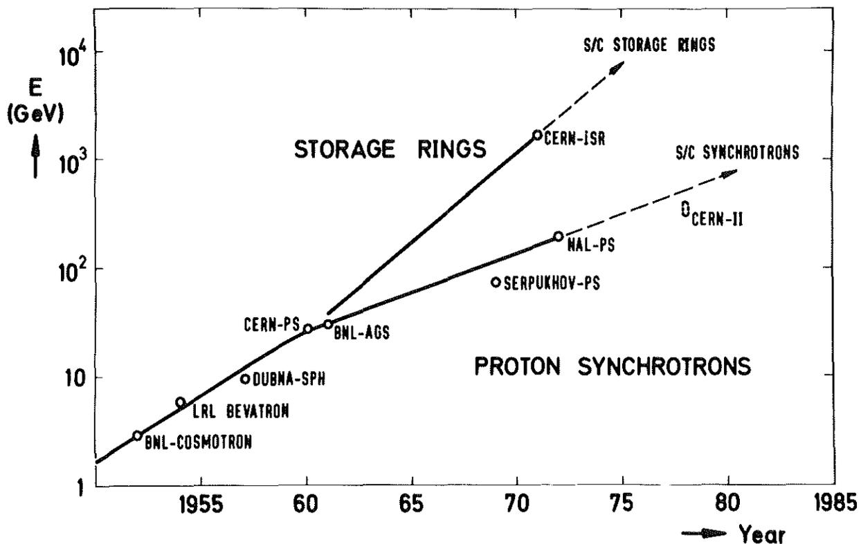
Fig. 1: Maximum energy of various accelerators versus date of first beam obtained
