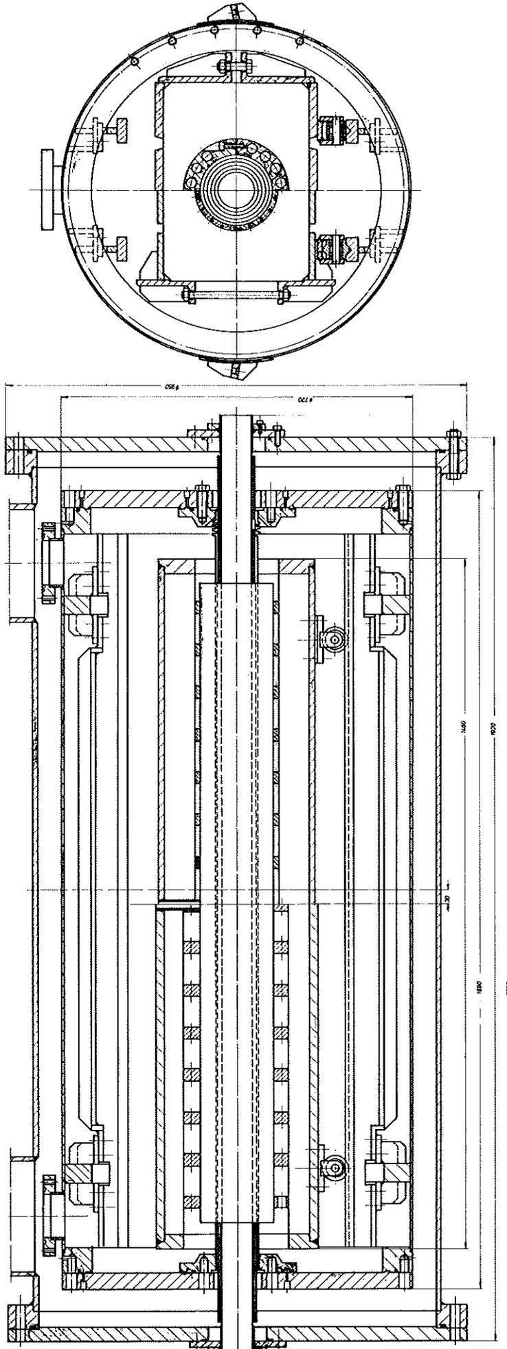
Fig. 16: Axial and radial views of cryostat for D2 (IEKP)
