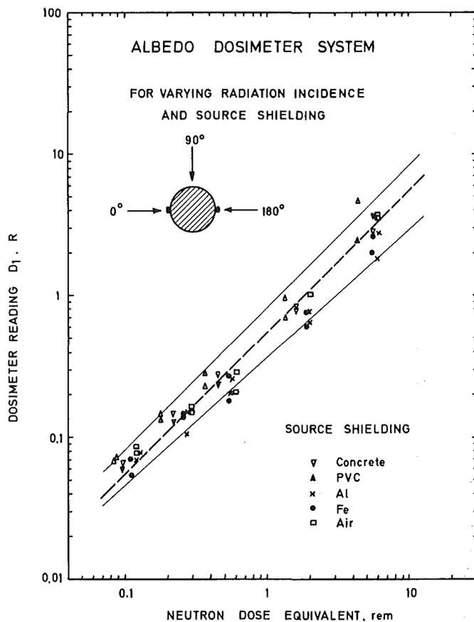
FIG. 4. Dosimeter reading  $D_1$  of the albedo dosimeter system as a function of the dose-equivalent for varying radiation incidence angles and a source shielding of 5-cm thickness.
