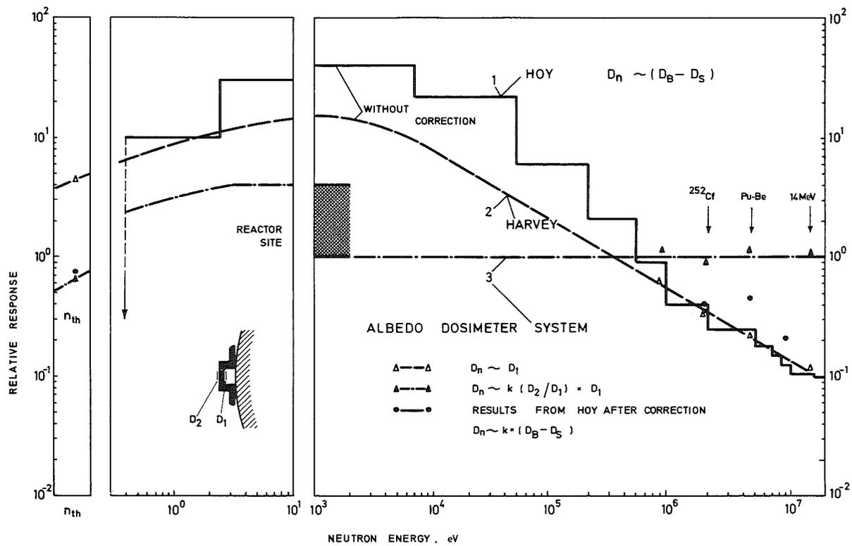
FIG.16. Relative response of different albedo dosimeters as a function of neutron energy, with experimental results for the single albedo dosimeter, the albedo dosimeter system and after J. E. Hoy: (1) albedo dosimeter after J. E. Hoy [ 7 ], calculation after Ref. [ 10 ]; (2) albedo dosimeter after Harvey [ 4 ], normalized to own results; (3) albedo dosimeter system, approximation in the energy range of intermediate neutrons, no calculation.
