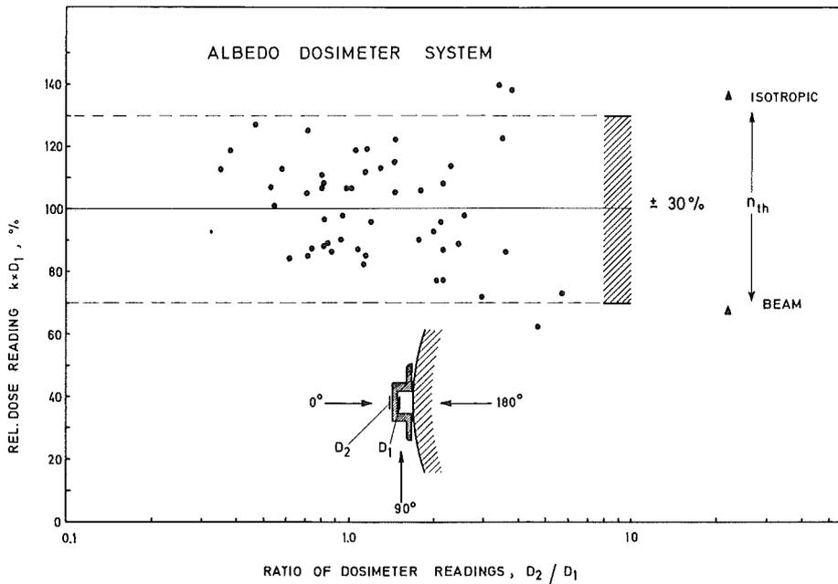
FIG. 12. Relative dose reading  $k \cdot D_1$  of the albedo dosimeter system after correction for the effect of scattered neutrons as a function of the ratio of the dosimeter readings  $D_2/D_1$  for all irradiations with fast neutrons (see Table I) and directions of radiation incidence of  $0^\circ$ ,  $90^\circ$ ,  $180^\circ$ .
