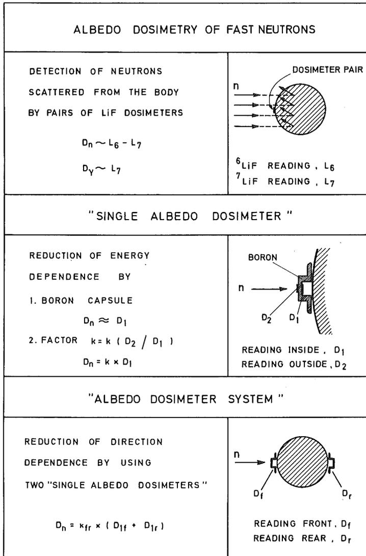
FIG. 2. Application of albedo dosimetry to the measurement of fast neutrons.
