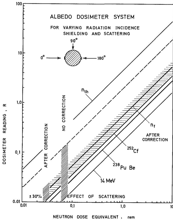
FIG. 13. Dosimeter reading  $D_1$  of the albedo dosimeter system before and after correction for the effect of scattered neutrons as a function of the neutron dose-equivalent for directions of radiation incidence of  $0^\circ$ ,  $90^\circ$ ,  $180^\circ$ .
