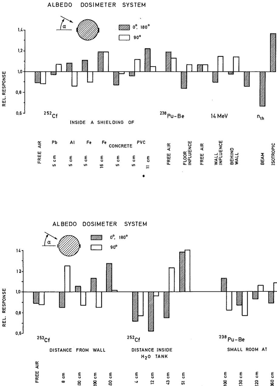
FIG. 11. Relative response of the albedo dosimeter system after correction for the effect of scattered neutrons for various exposure conditions (see also Fig. 12 and Table I).
