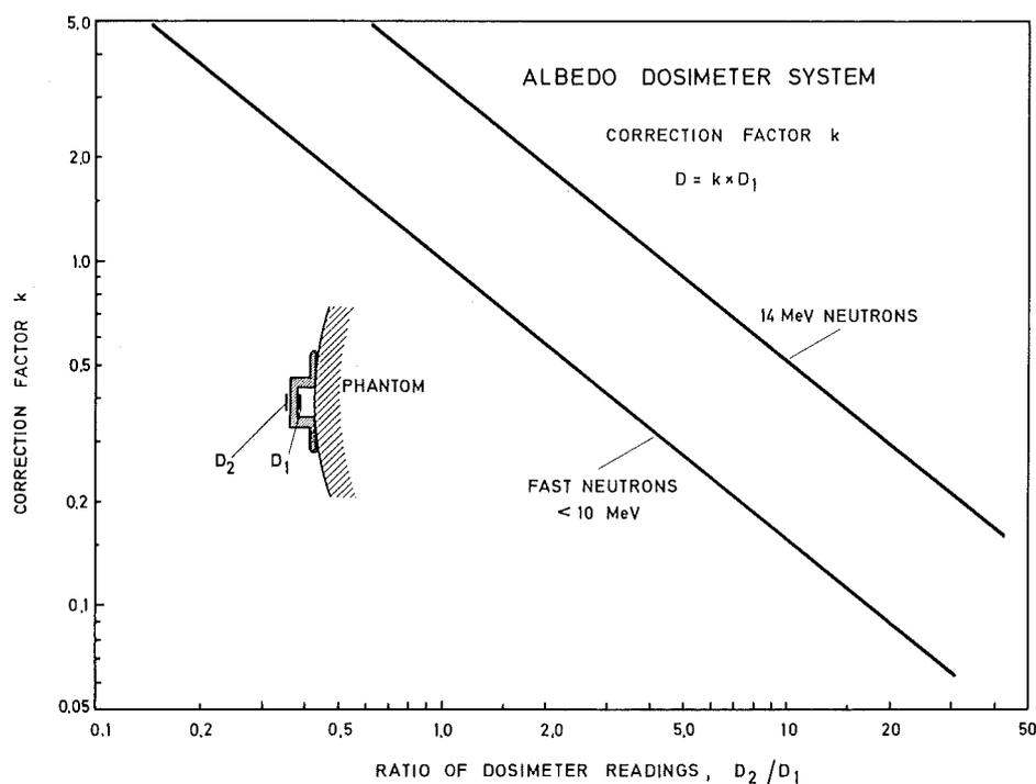
FIG. 9. Correction factor  $k = k(D_2/D_1)$  for the albedo dosimeter system as a function of the ratio of dosimeter readings  $D_2/D_1$  for fast neutrons below 10 MeV and for 14-MeV neutrons.
