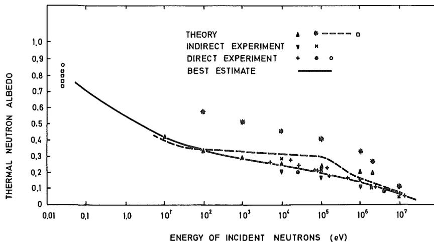
FIG. 1. Thermal neutron albedo as a function of incident neutron energy, after Ref. [4].
