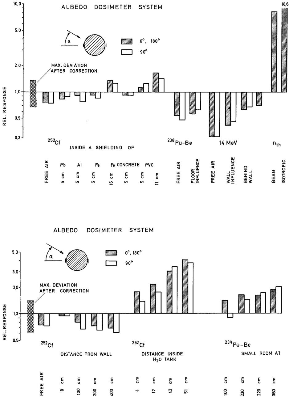
FIG. 10. Relative response of the albedo dosimeter system without correction for the effect of scattered neutrons for various sources and exposure conditions and directions of radiation incidence of 0°, 90°, 180°.
