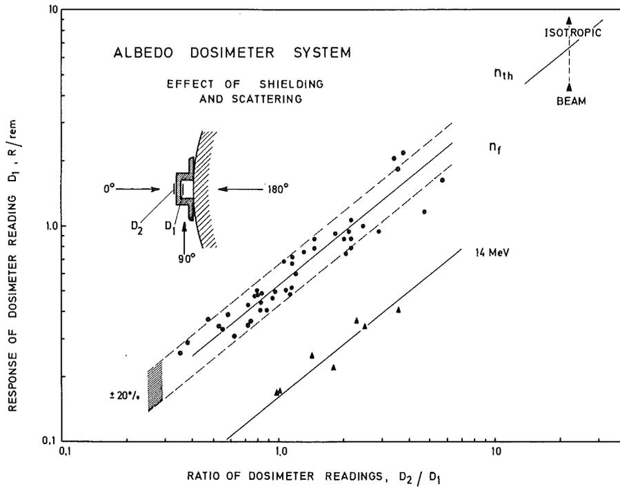
FIG. 8. Response of the albedo dosimeter system reading  $D_1$  as a function of the dosimeter readings  $D_2/D_1$  for irradiation with various neutron spectra, including the effect of shielding and scattering and directions of radiation incidence of  $0^\circ$ ,  $90^\circ$ ,  $180^\circ$ .
