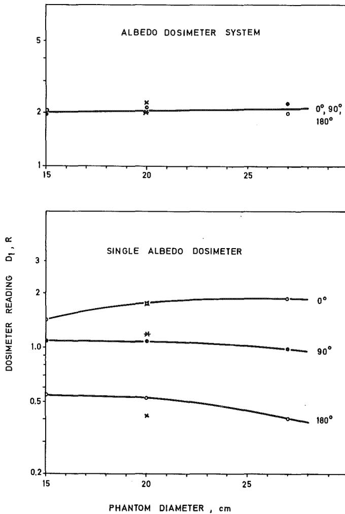
FIG. 15. Dosimeter reading  $D_1$  of the single albedo dosimeter and the albedo dosimeter system as a function of phantom diameter for an irradiation with  $^{252}\text{Cf}$  neutrons.
