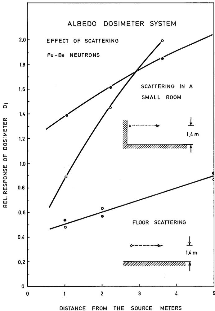
FIG. 5. Relative response of dosimeter reading  $D_1$  as a function of the distance from the source for irradiations with PuBe neutrons in a small room, the source in contact with the walls at the corner of the room and under free air conditions.
