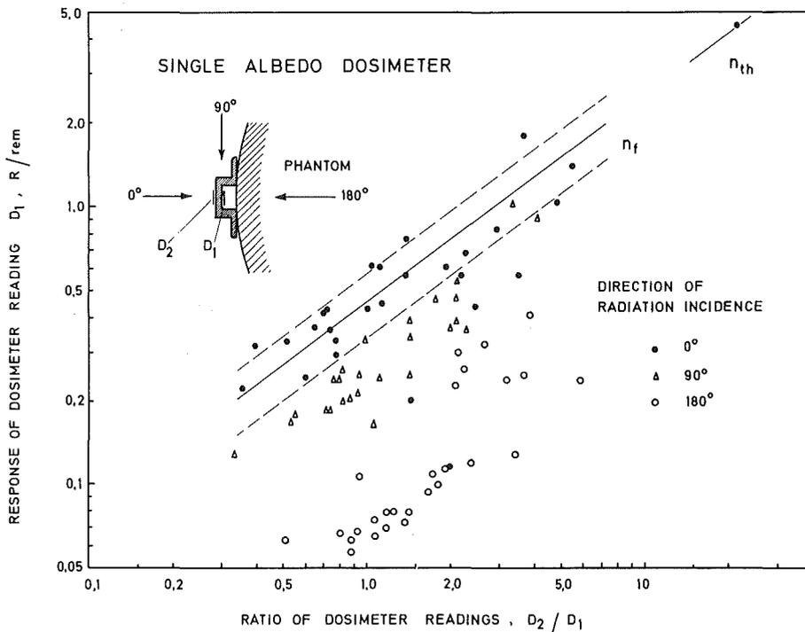
FIG. 7. Response of single albedo dosimeter reading  $D_1$  as a function of the ratio of the dosimeter readings  $D_2/D_1$  for directions of radiation incidence of  $0^\circ$ ,  $90^\circ$  and  $180^\circ$  after irradiation with  $^{252}\text{Cf}$ , PuBe and 14-MeV neutrons.
