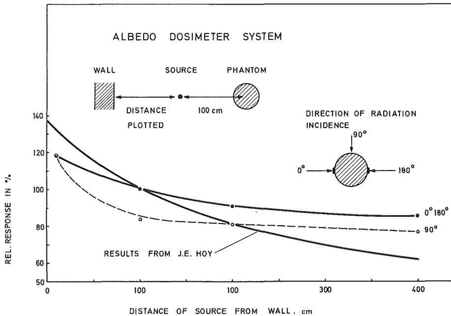
FIG. 6. Relative response of dosimeter reading  $D_1$  as a function of the distance of the  $^{252}\text{Cf}$  source from the concrete wall for the albedo dosimeter system with directions of radiation incidence of  $0^\circ$ ,  $90^\circ$  and  $180^\circ$  and of the albedo dosimeter developed by J. E. Hoy after Ref. [7].
