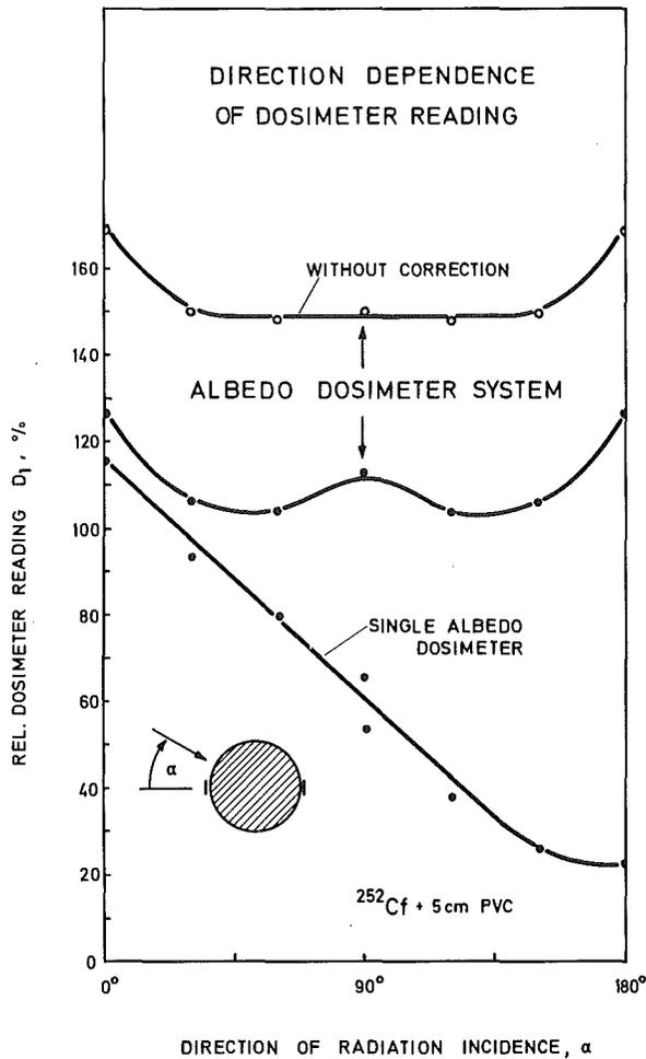
FIG. 14. Relative dosimeter reading  $D_1$  of the single albedo dosimeter and the albedo dosimeter system without and with correction for scattered neutrons as a function of the direction of the radiation incidence angle  $\alpha$  for irradiation with  $^{252}\text{Cf} + 5 \text{ cm PVC}$ .
