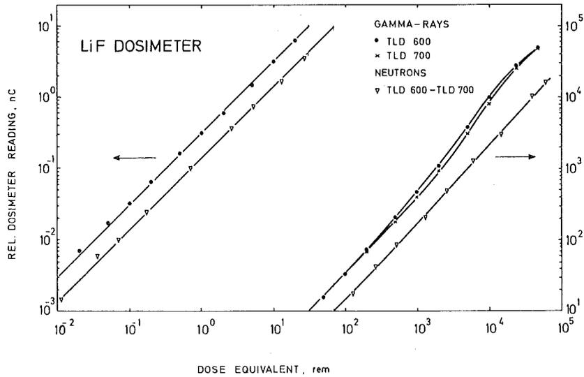
FIG. 3. Relative dosimeter reading of LiF dosimeters as a function of the dose-equivalent for gamma irradiation and of an albedo dosimeter for fast-neutron irradiation.
