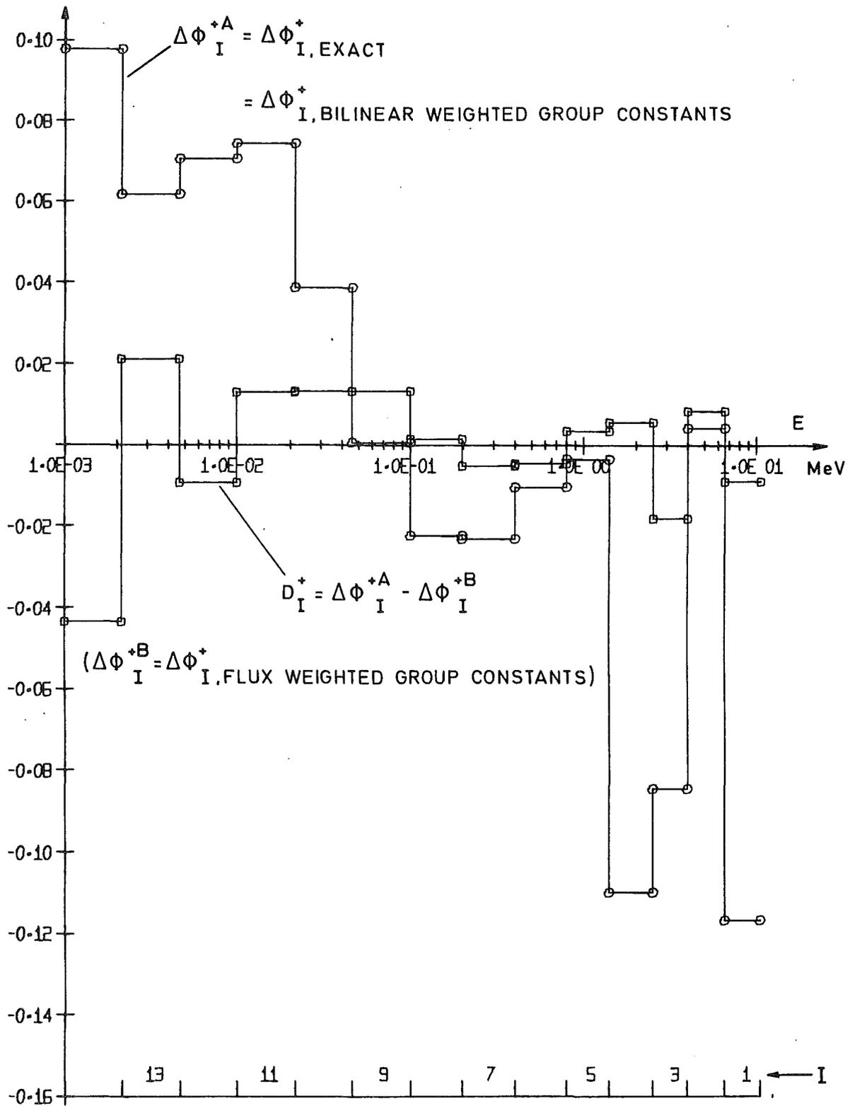
Fig. 4: Comparison of adjoint flux differences
