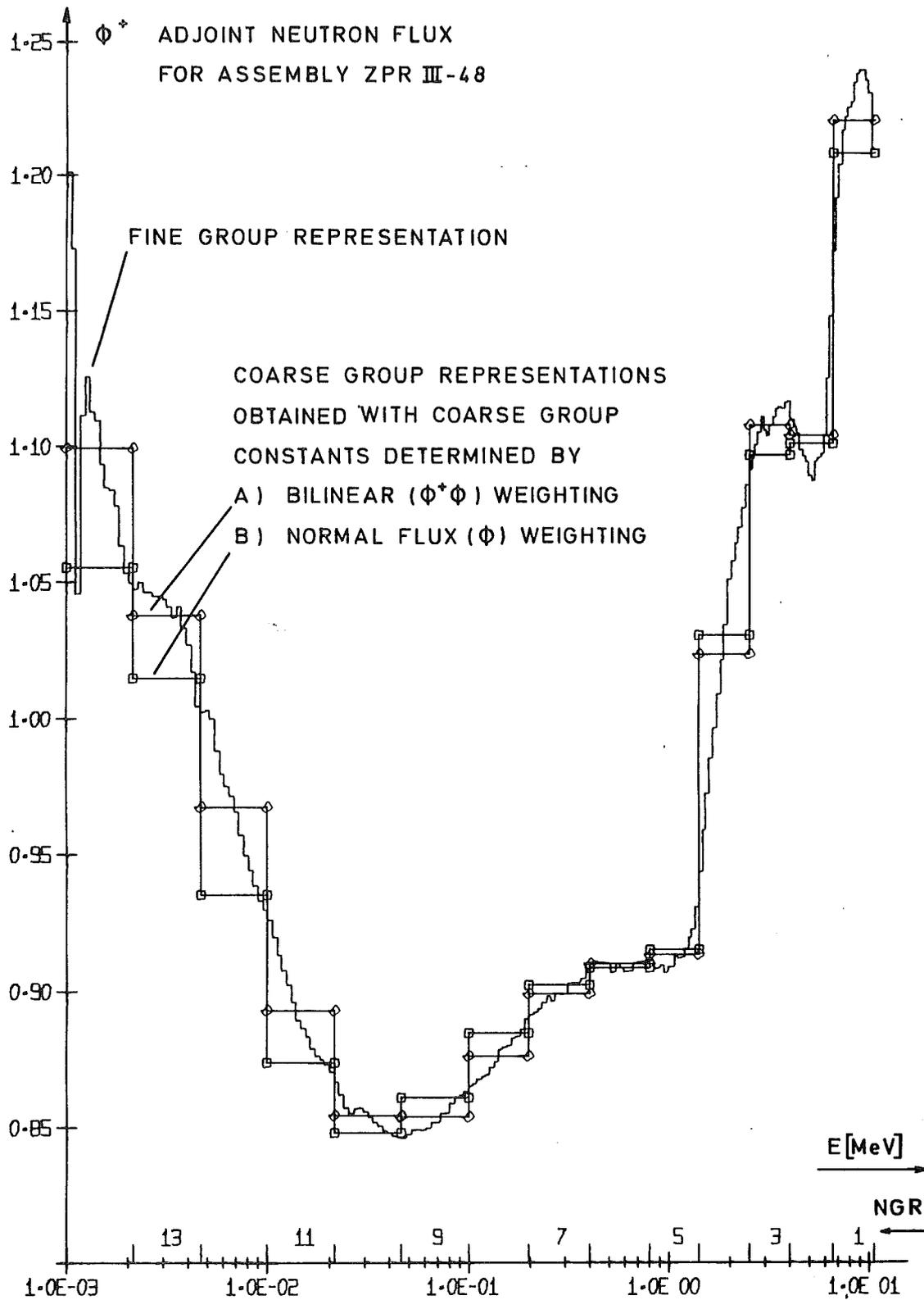
Fig. 2: Energy dependence of adjoint neutron fluxes
