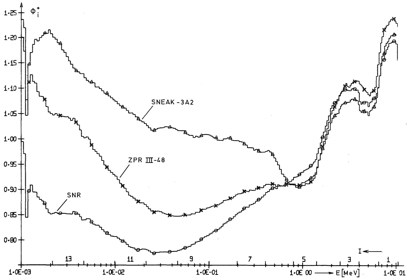
Fig. 7: Fine group representation of adjoint fluxes for SNR, ZPR III-48, SNEAK-3A2
