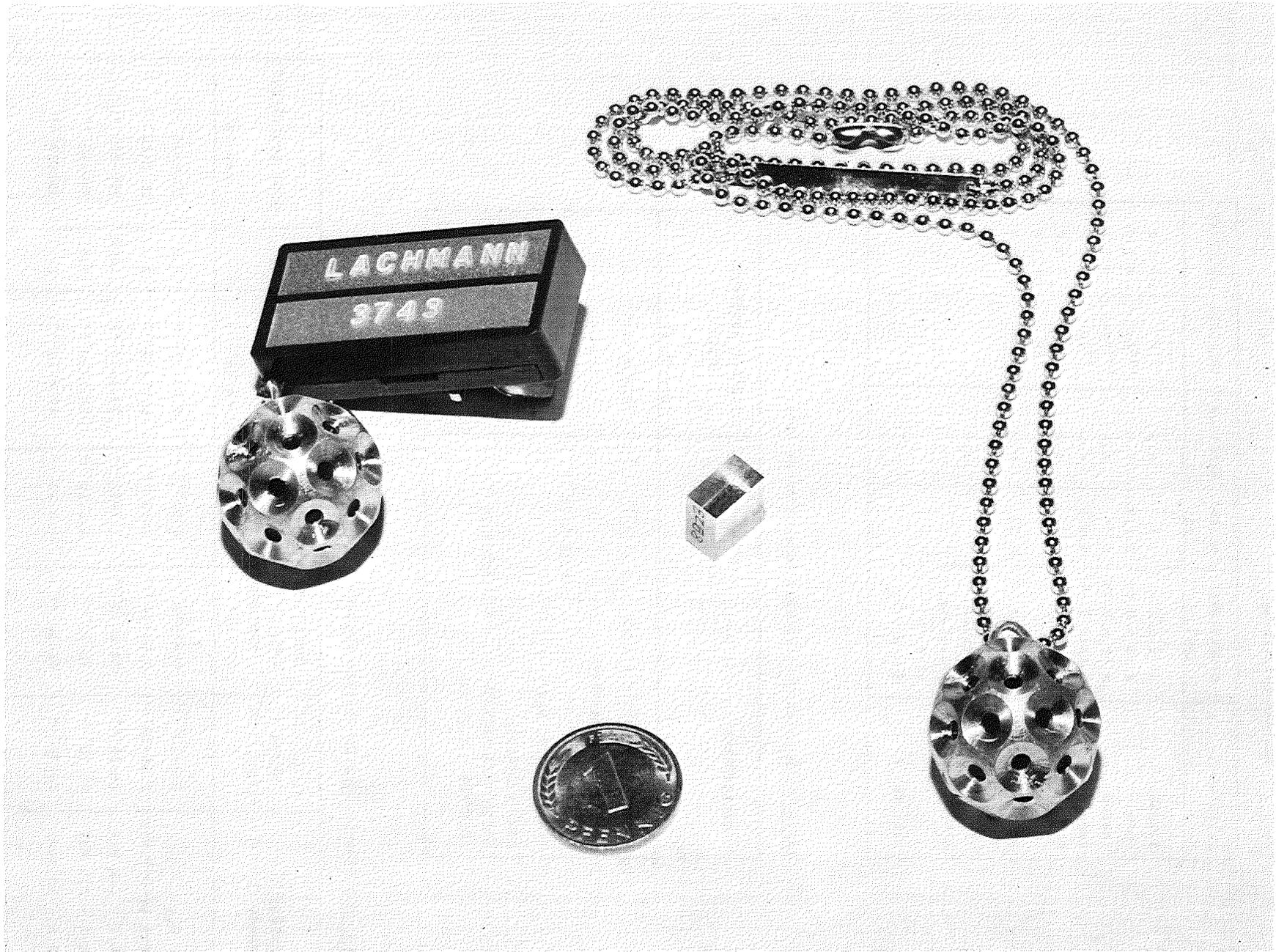
Fig. 1: The Personnel Dosimeter used at the Karlsruhe Nuclear Research Center
