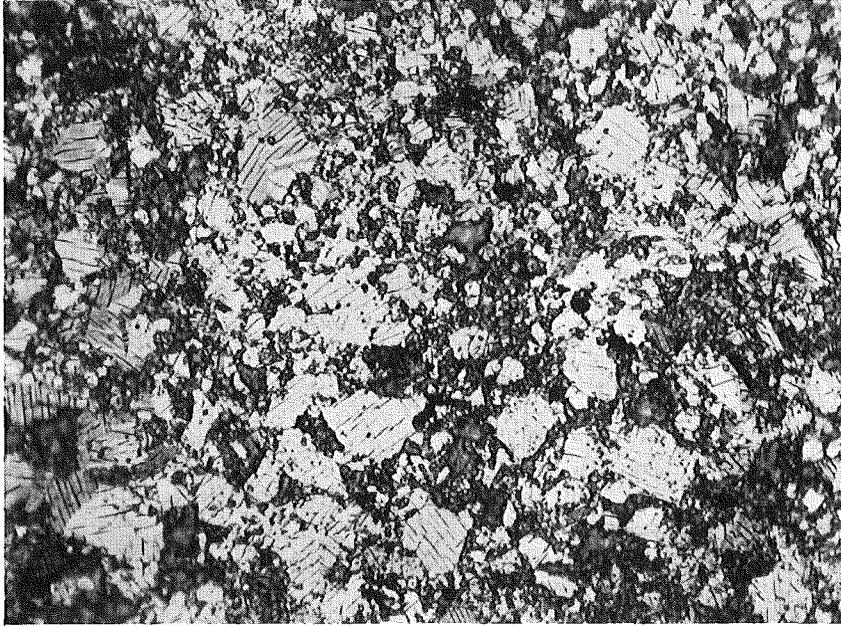
Fig. 3 Uranium dicarbide,
