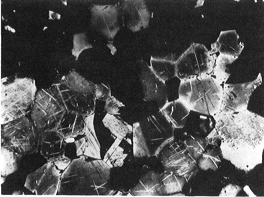
Fig. 1 Uranium monocarbide with dicarbide needles,
