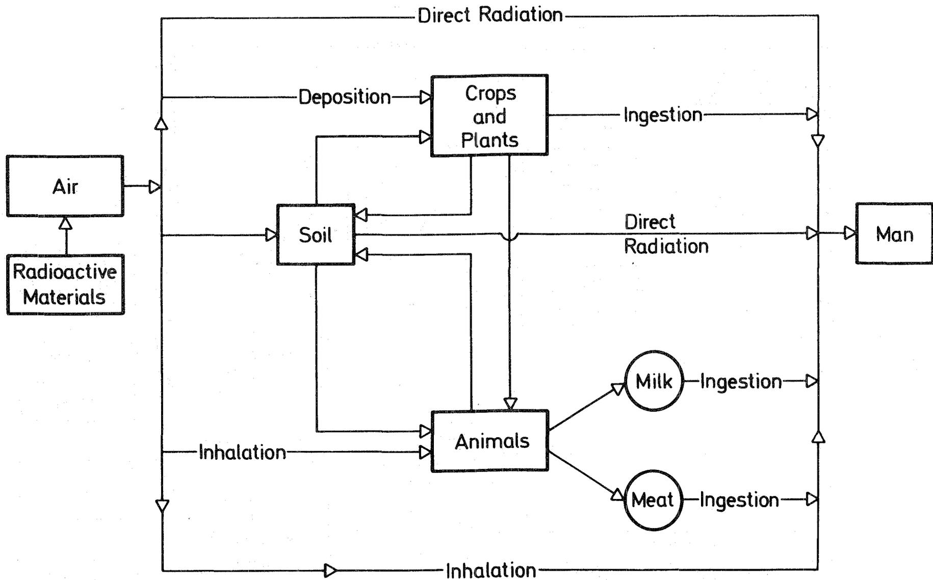
Fig.8 Pathways between Radioactive Materials released to the Atmosphere and Man (Environmental Protection Agency, 1972)
