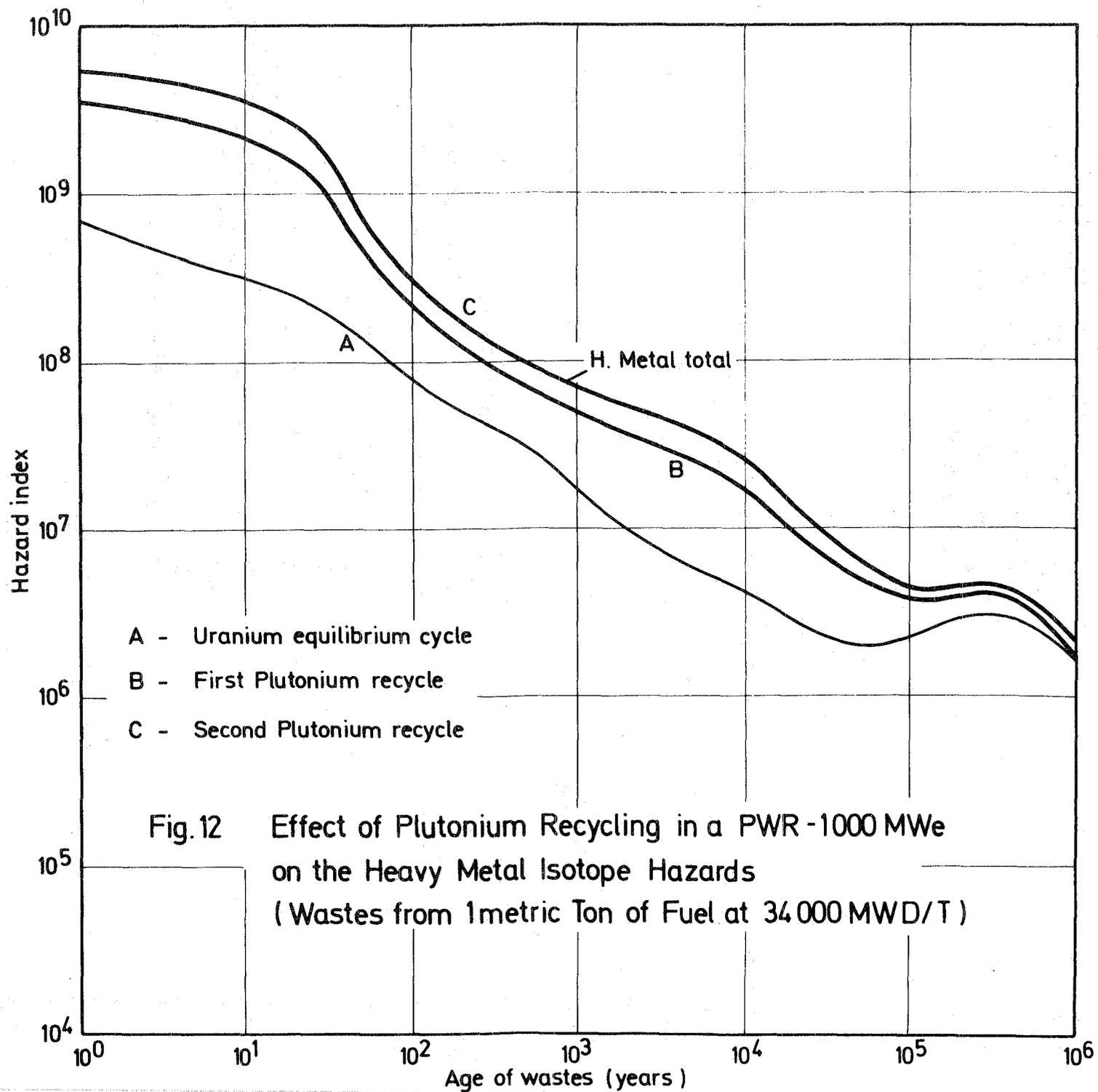
Fig.12 Effect of Plutonium Recycling in a PWR-1000 MWe on the Heavy Metal Isotope Hazards (Wastes from 1metric Ton of Fuel at 34 000 MWD/T)
