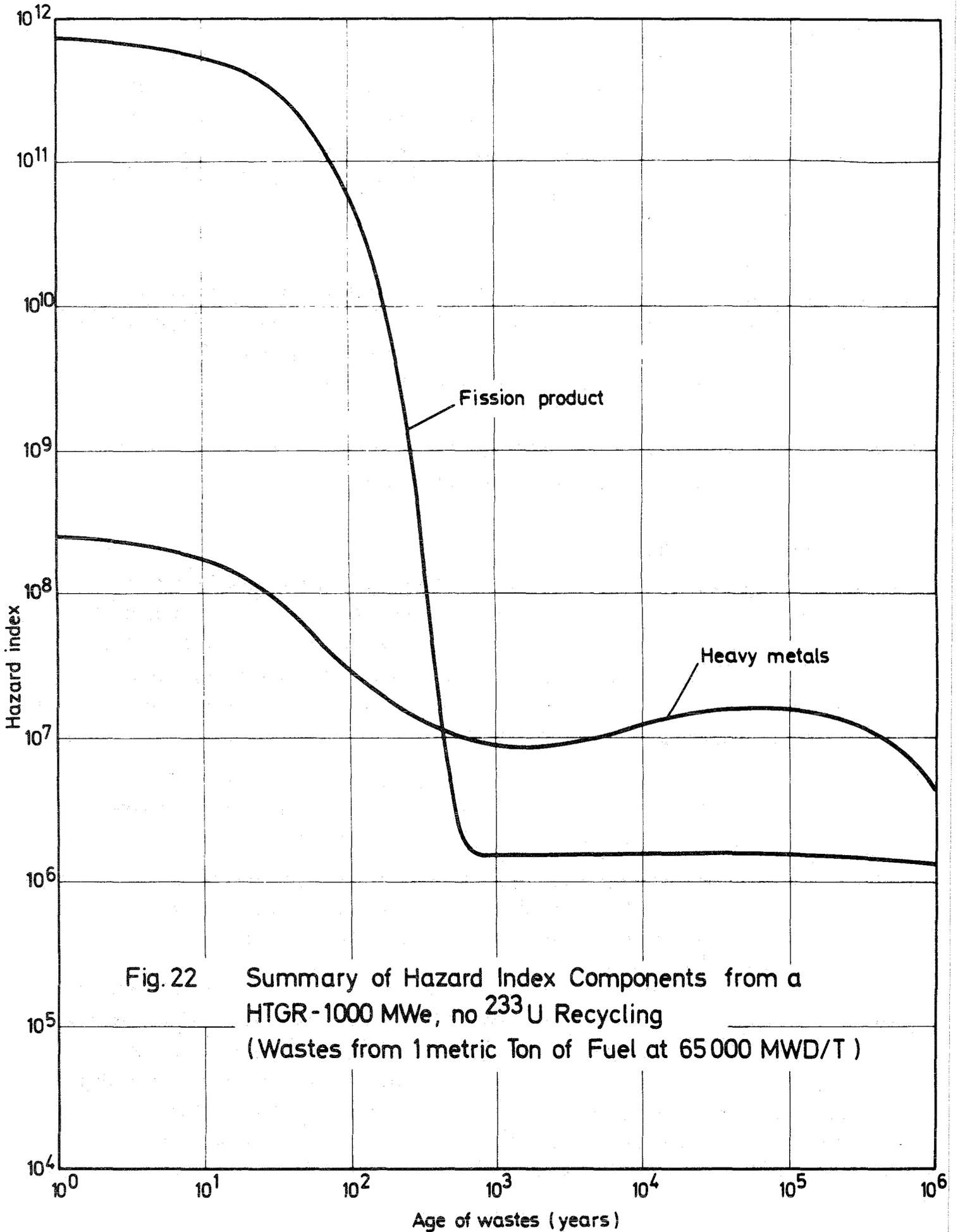
Fig. 22 Summary of Hazard Index Components from a HTGR-1000 MWe, no  $^{233}\text{U}$  Recycling (Wastes from 1 metric Ton of Fuel at 65 000 MWD/T)
