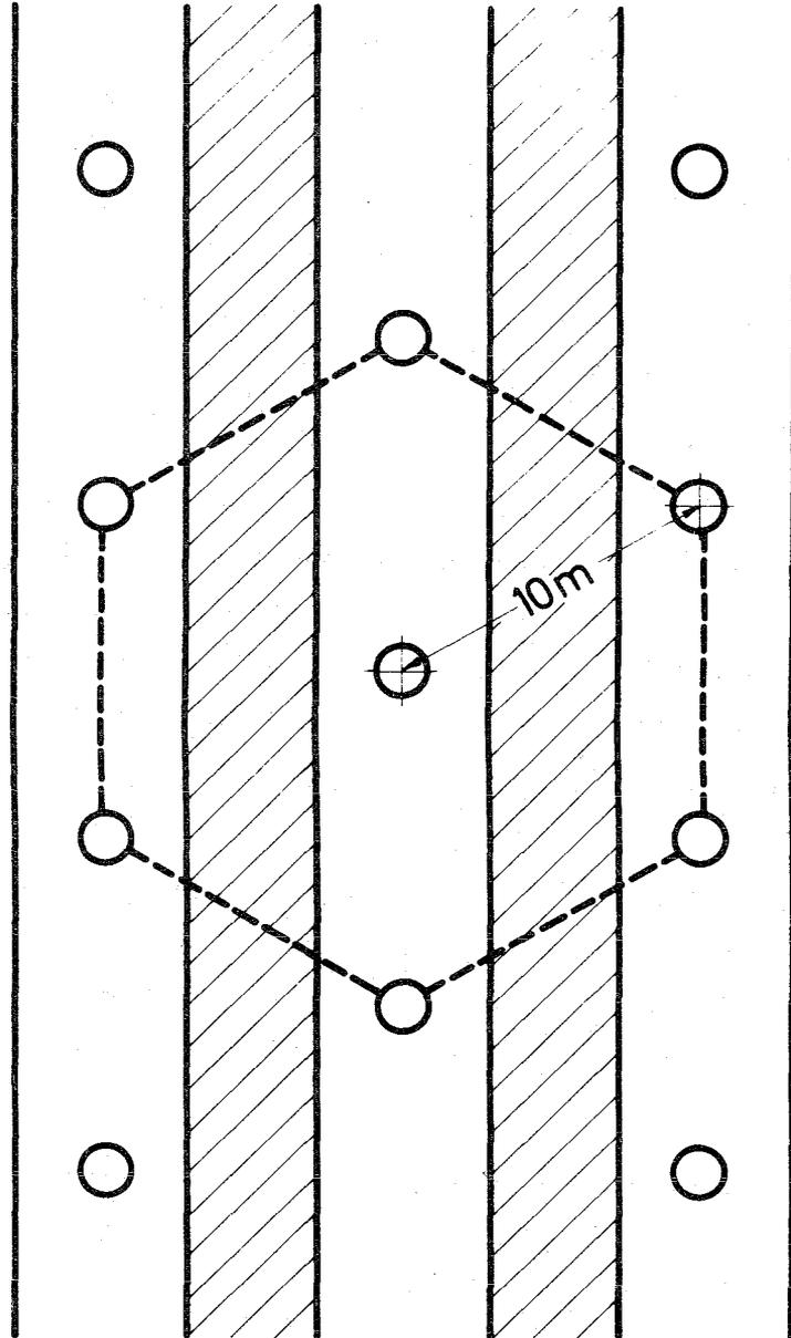
Fig. 25 Arrangement of Waste Cylinders in Salt Deposit
