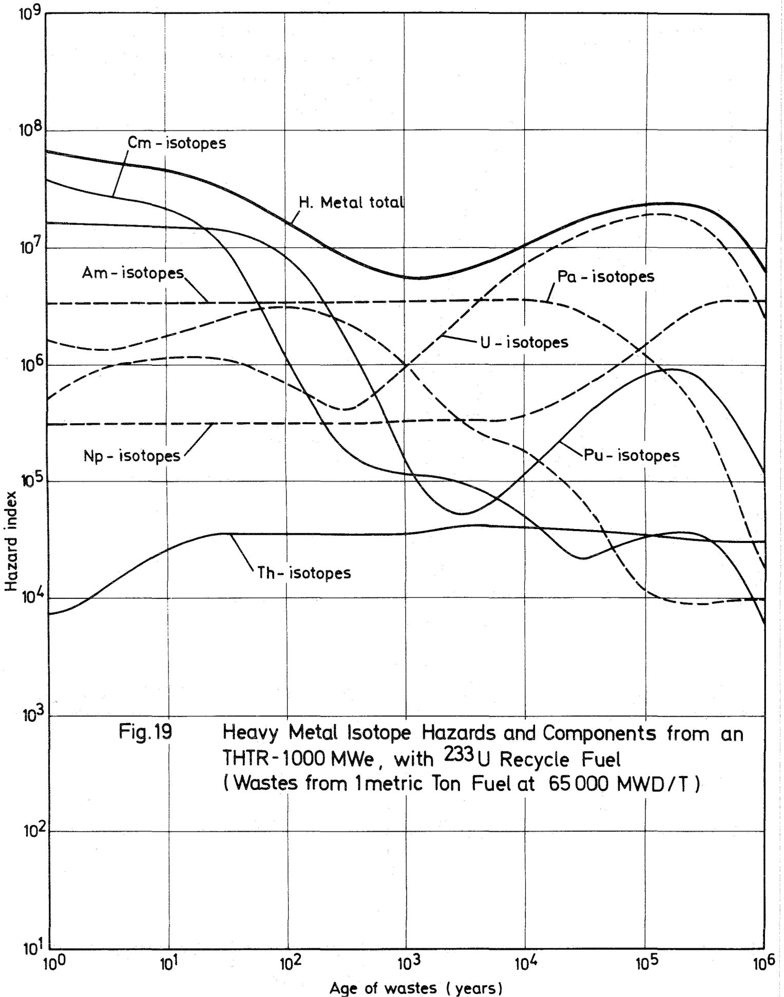
Fig.19 Heavy Metal Isotope Hazards and Components from an THTR-1000 MWe, with  $^{233}\text{U}$  Recycle Fuel (Wastes from 1 metric Ton Fuel at 65 000 MWD/T)
