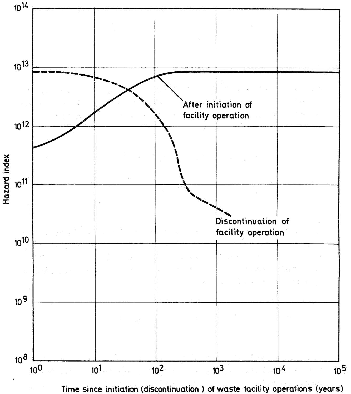
Fig. 29 Hazard Index of Total Waste Storage Facility at a Constant Yearly Rate ( $H_i(t) = 4.14 \times 10^{11} \text{ m}^3$ ) of Addition
