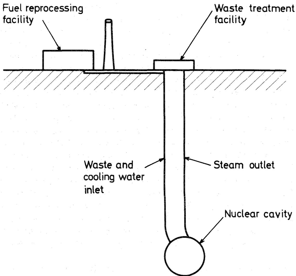
Fig. 28 Waste Disposal in a Nuclear Cavity
