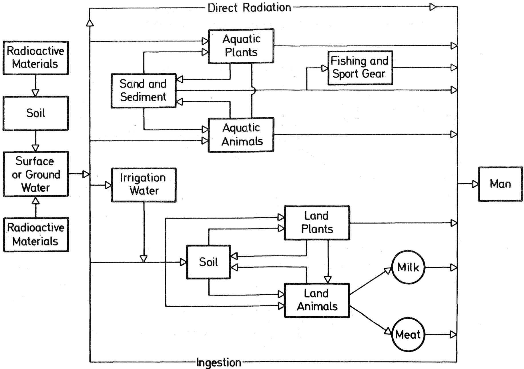
Fig.9 Pathways between Radioactive Materials released to Ground and Surface Waters and Man
