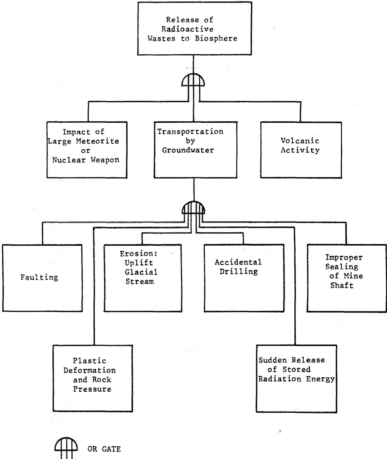
Fig. 27 Fault Tree of Salt Mine Used for Storage of Radioactive Wastes
