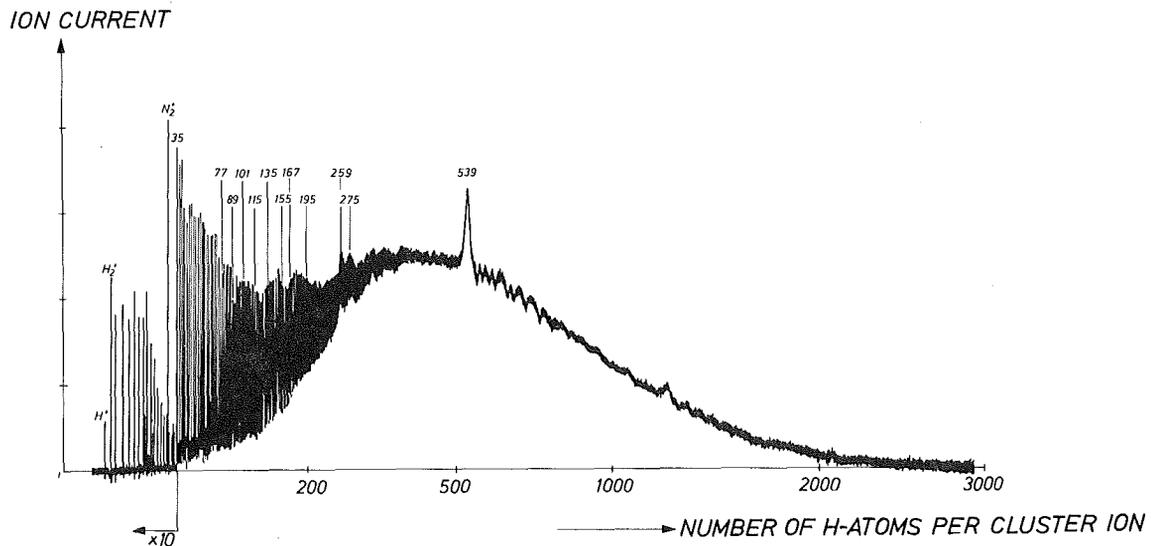
Fig. 1: Cluster ion spectrum generated by electron impact ionization of clusters of approximately  $10^4$  H-atoms. The cluster ions contain on the average 300 H-atoms per charge.
