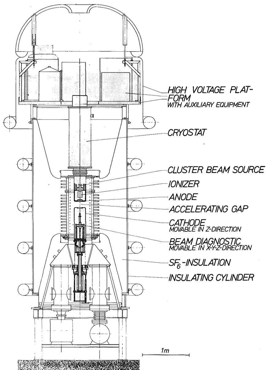
Fig. 4: Schematic diagram of the test assembly on high gradient acceleration of cluster ions to an energy of 1 MeV at Lyon. The shaded areas indicate the amount of alterations of the existing accelerator necessary for the experiment. The high voltage generator and the motor generator supplying the cluster ion beam source are not shown on the diagram.
