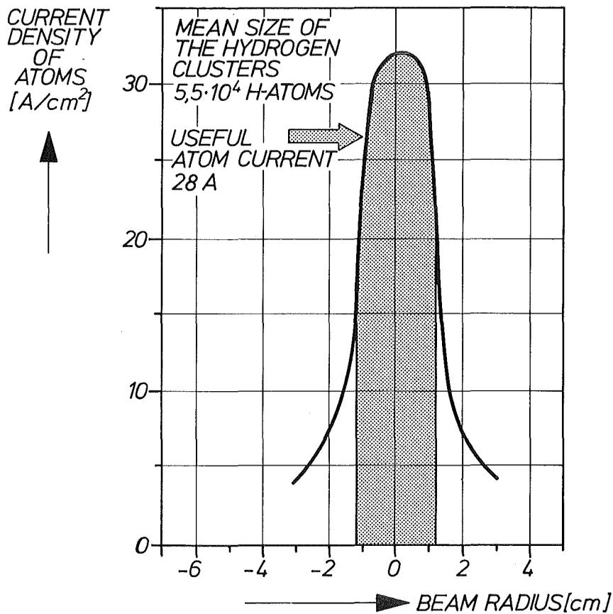
Fig. 3: Intensity profile of a hydrogen cluster beam with an average cluster size of approximately  $5.5 \times 10^4$  H-atoms probably required for ionization.
