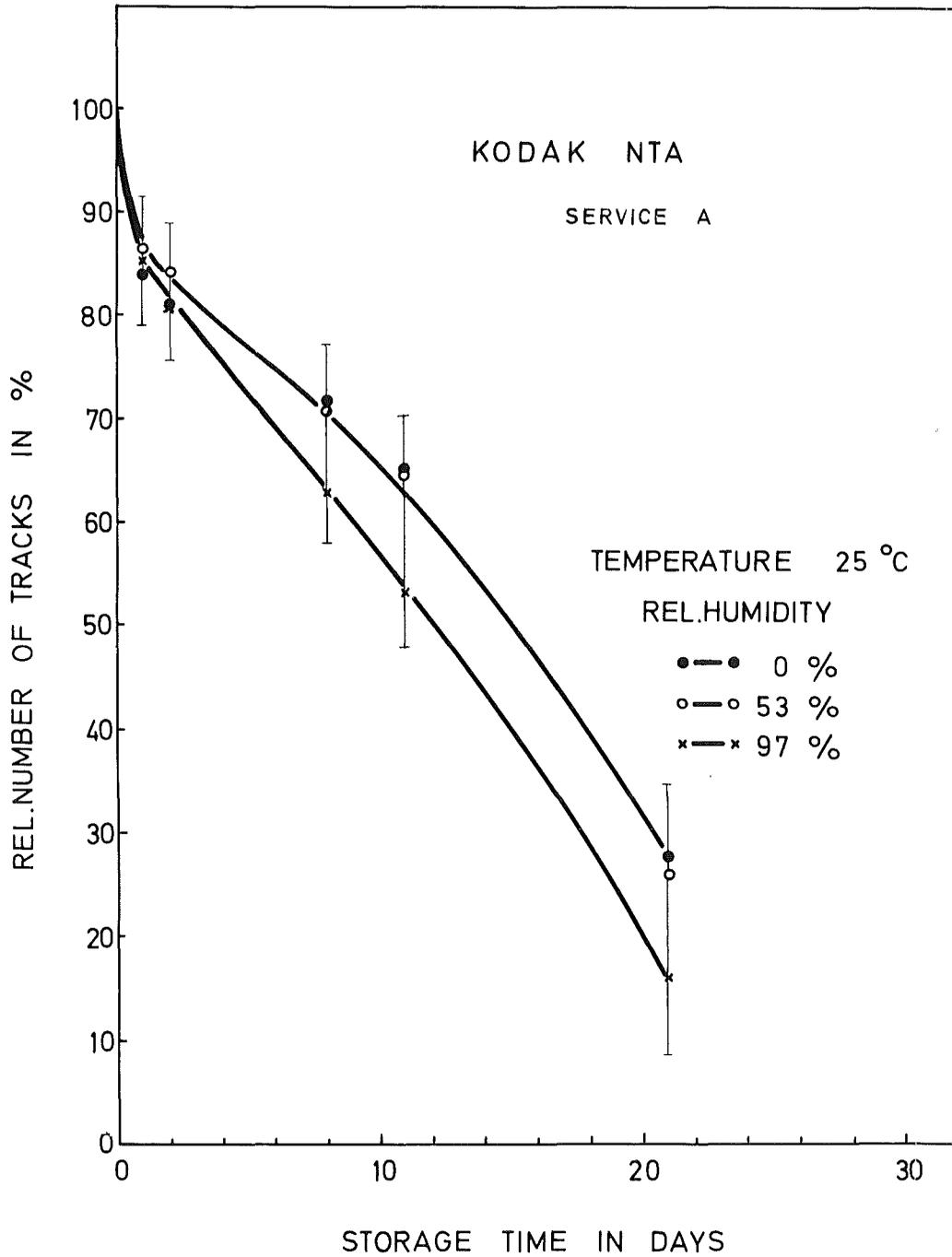
Fig. 5: Relative number of tracks vs storage time for Kodak NTA, service A, stored at 25°C and different relative humidities.
