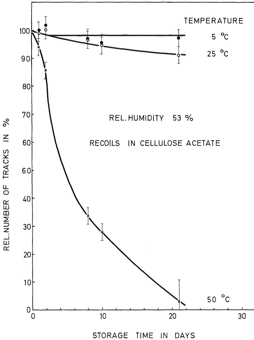
Fig. 24: Fading of recoils in cellulose acetate held at 53 % R.H. and various temperatures
