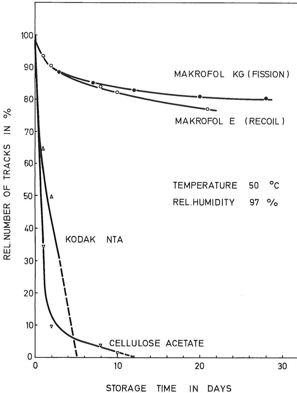
Fig. 36: Relative number of track vs. storage time for Kodak NTA, Makrofol and cellulose acetate , stored at 50°C and 97 % R.H.
