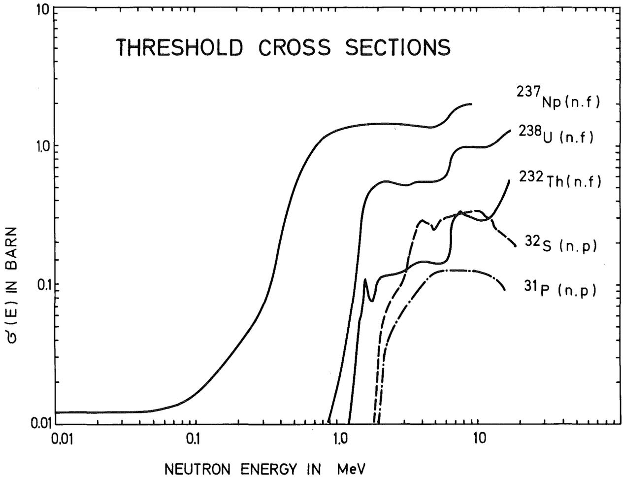
Fig. 3: Energy dependence of neutron cross sections for threshold reactions
