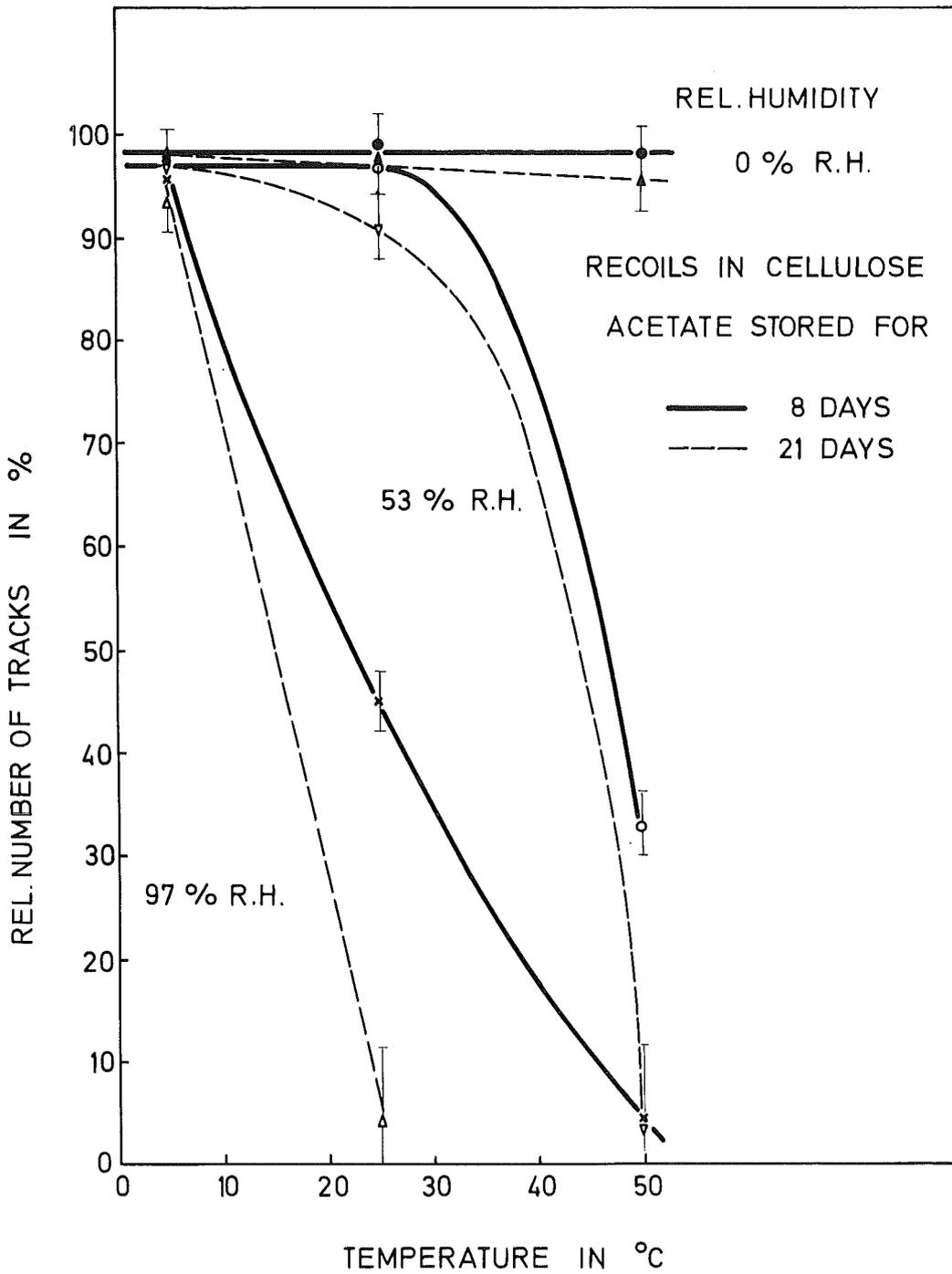
Fig. 27: Relative number of tracks vs. temperature for recoils in cellulose acetate stored for 8 and 21 days at different relative humidities.
