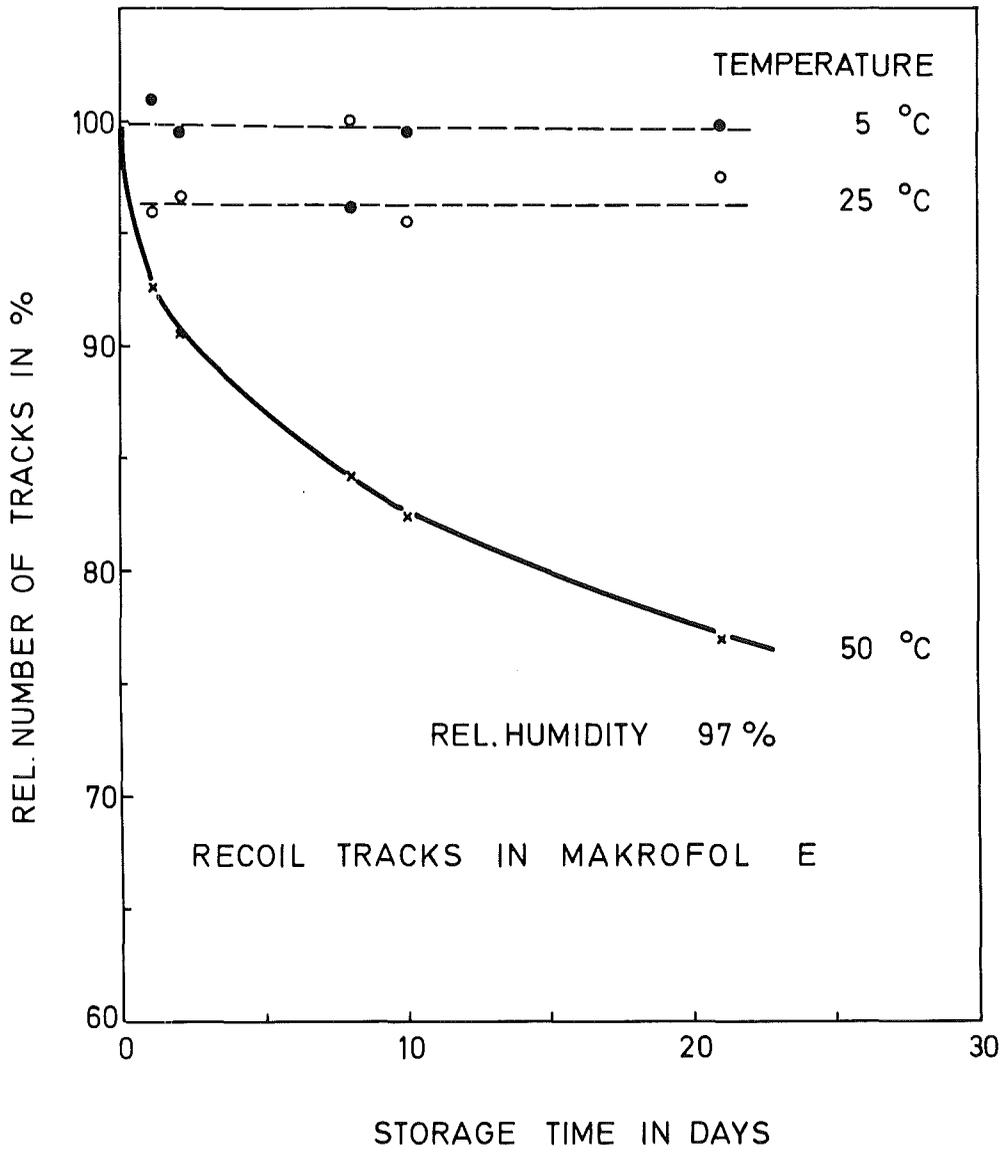
Fig. 28: Variation of the relative number of tracks with storage time for recoils in Makrofol E stored at 97 % R.H. and different temperatures
