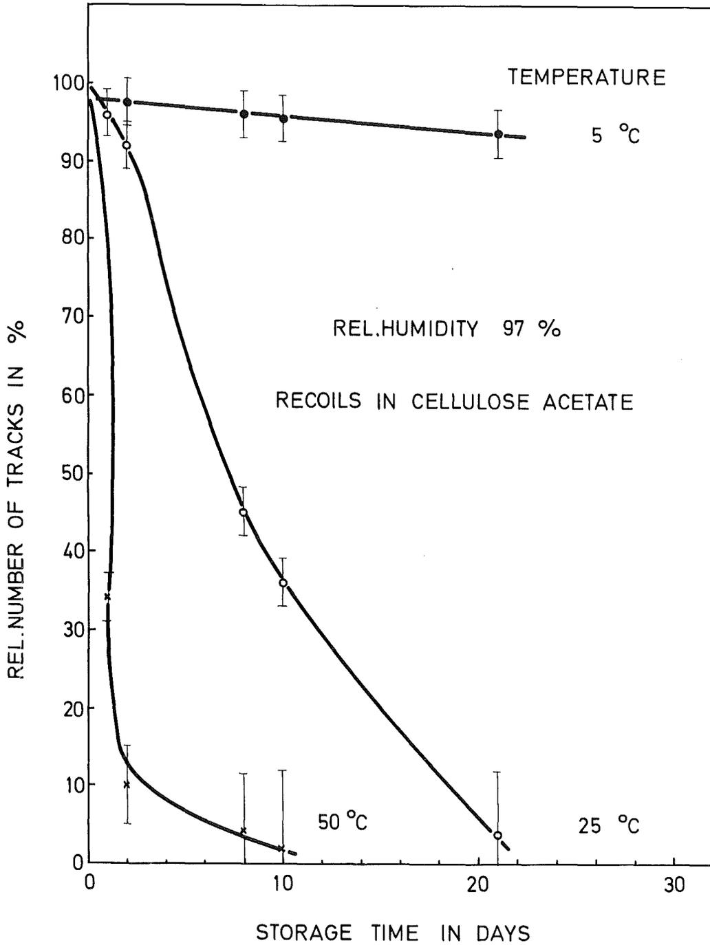
Fig. 25: Fading of recoils in cellulose acetate, held at 97 % R.H. and various temperatures
