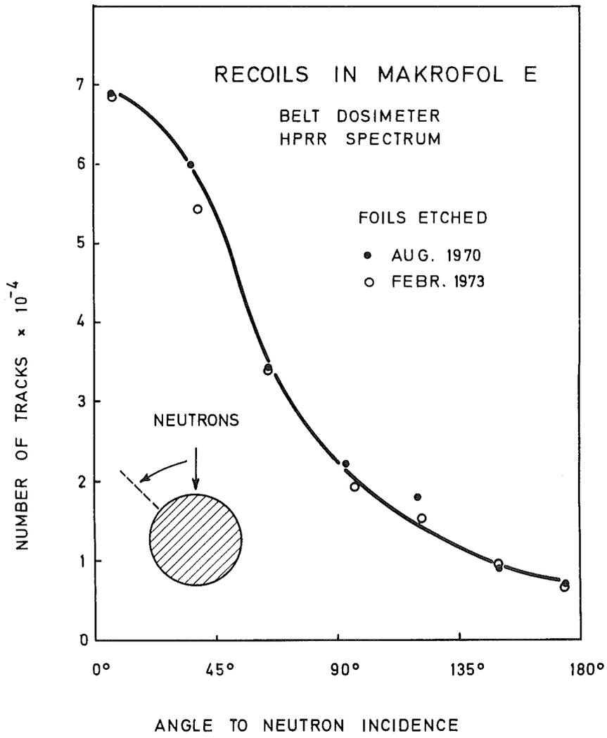
Fig. 32: Number of track as a function of angle to neutron incidence for recoils in Makrofol E
