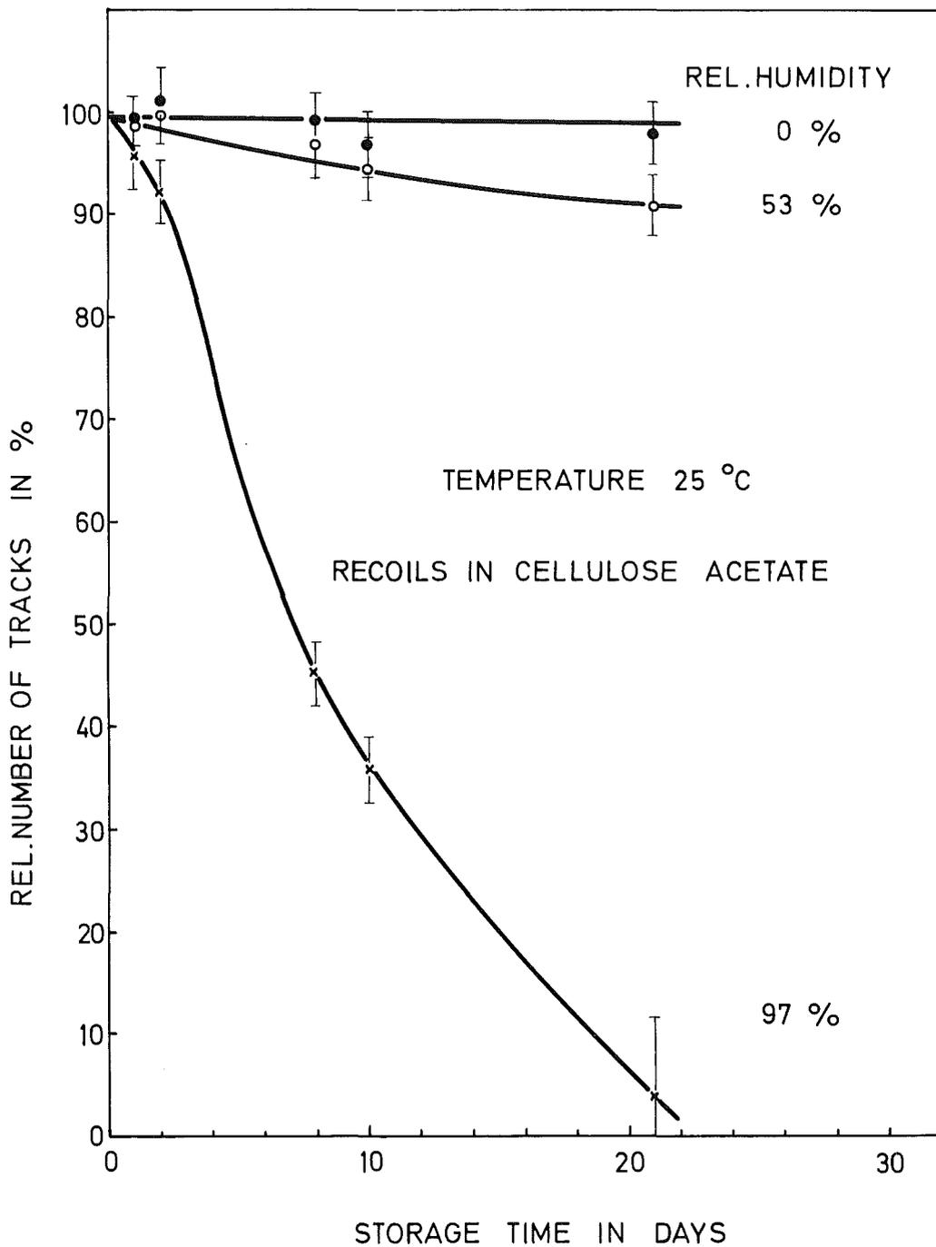
Fig. 21: Relative number of tracks as a function of storage time for neutron-induced recoils in cellulose acetate at 25°C and different relative humidities.
