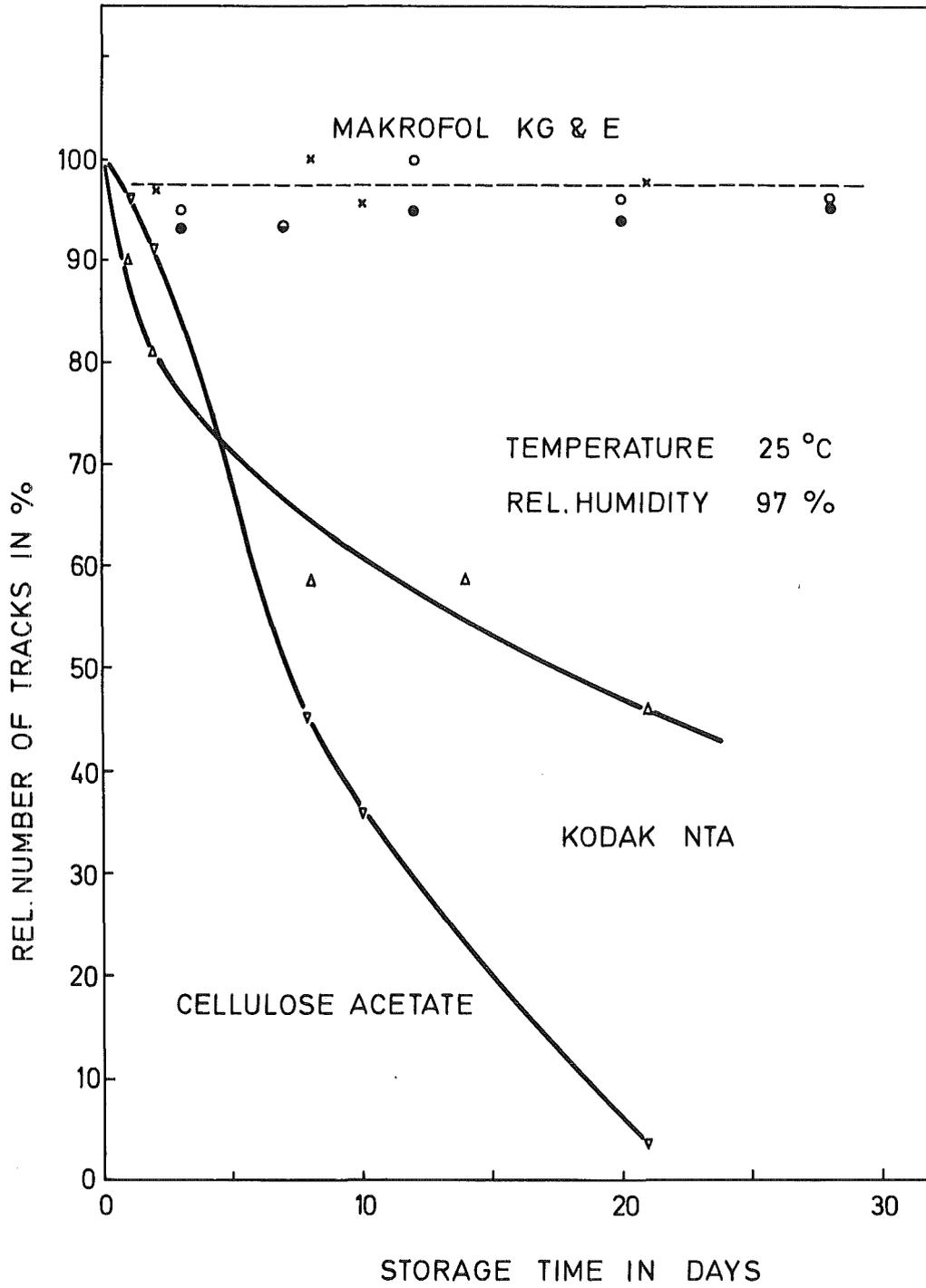
Fig. 34: Latent fading in Kodak NTA, Makrofol and cellulose acetate, stored at 25°C and 97 % R.H.
