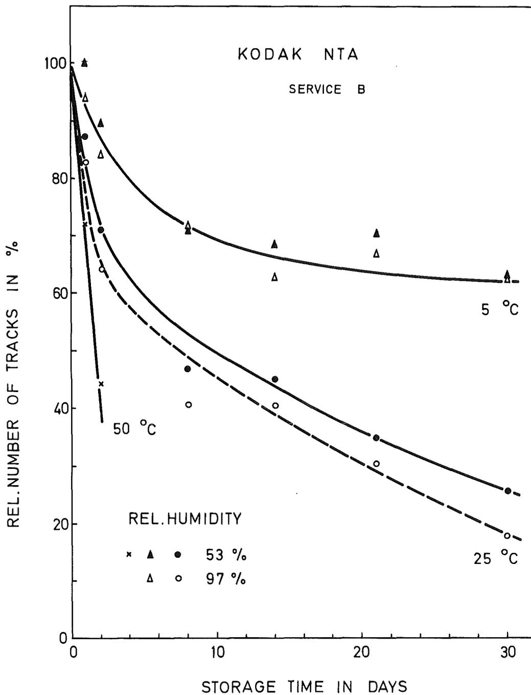
Fig. 8: Relative number of tracks as a function of storage time for Kodak NTA, service B, stored at various temperatures and humidities.
