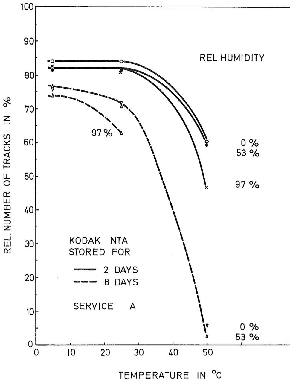
Fig. 14: Latent track fading in Kodak NTA, service A, as a function of temperature, films stored for 2 and 8 days at different relative humidities.
