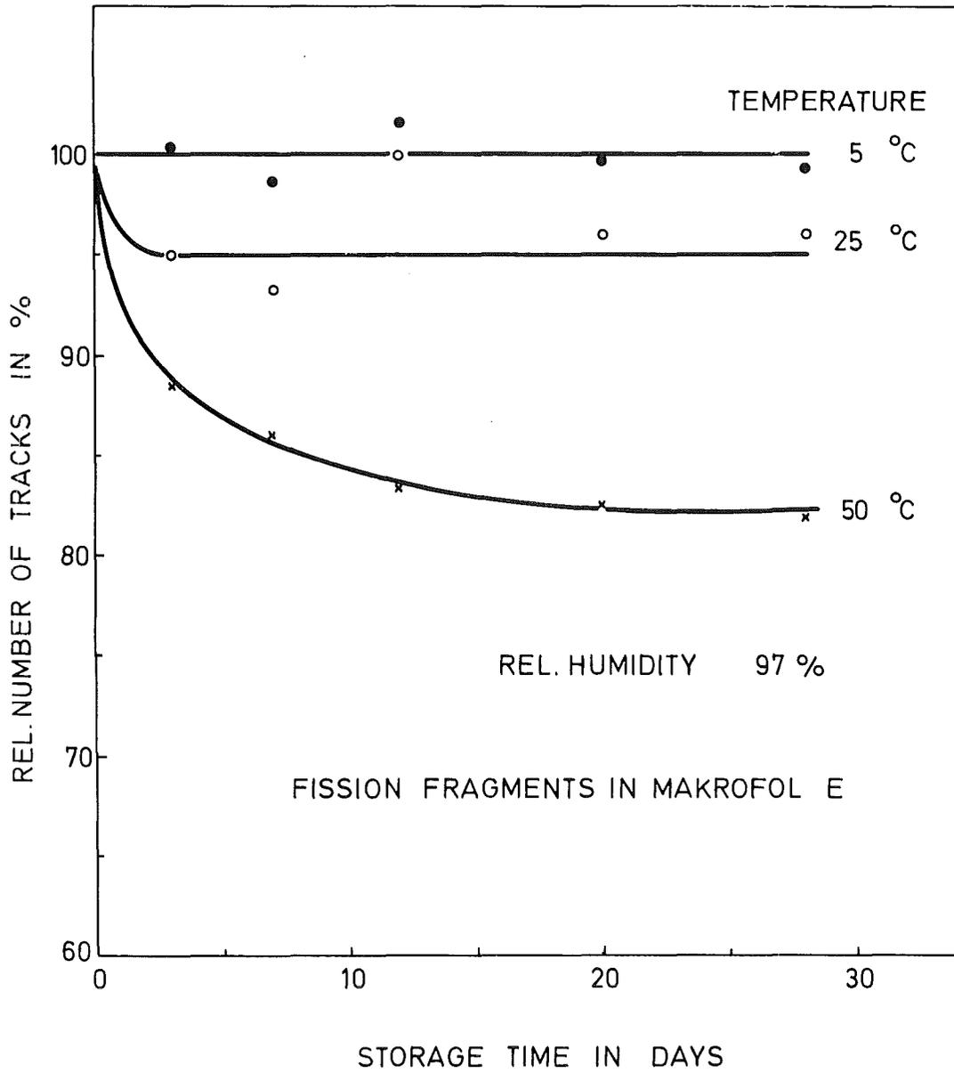
Fig. 16: Relative number of track as a function of storage time for fission fragments in Makrofol E stored at 97 % R.H. and different temperatures
