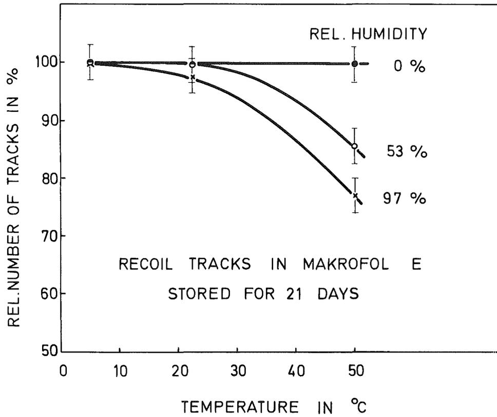
Fig. 31: Relative number of tracks vs. temperature for recoils in Makrofol E stored for 21 days at different relative humidities.
