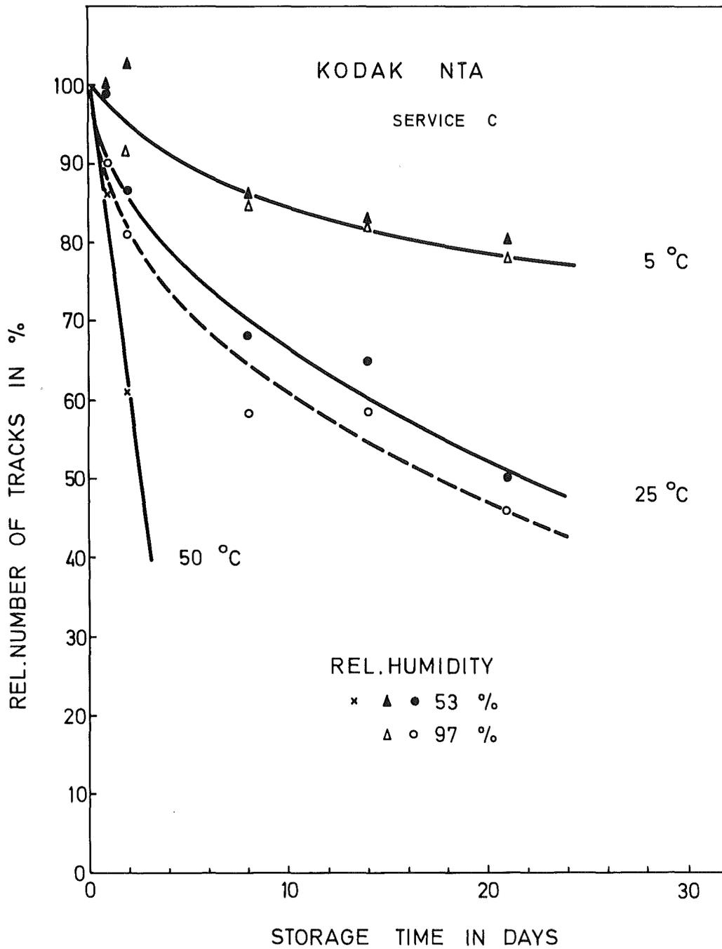
Fig. 9: Variation of the relative number of tracks with storage time for Kodak NTA, service C, for different temperatures and humidities.
