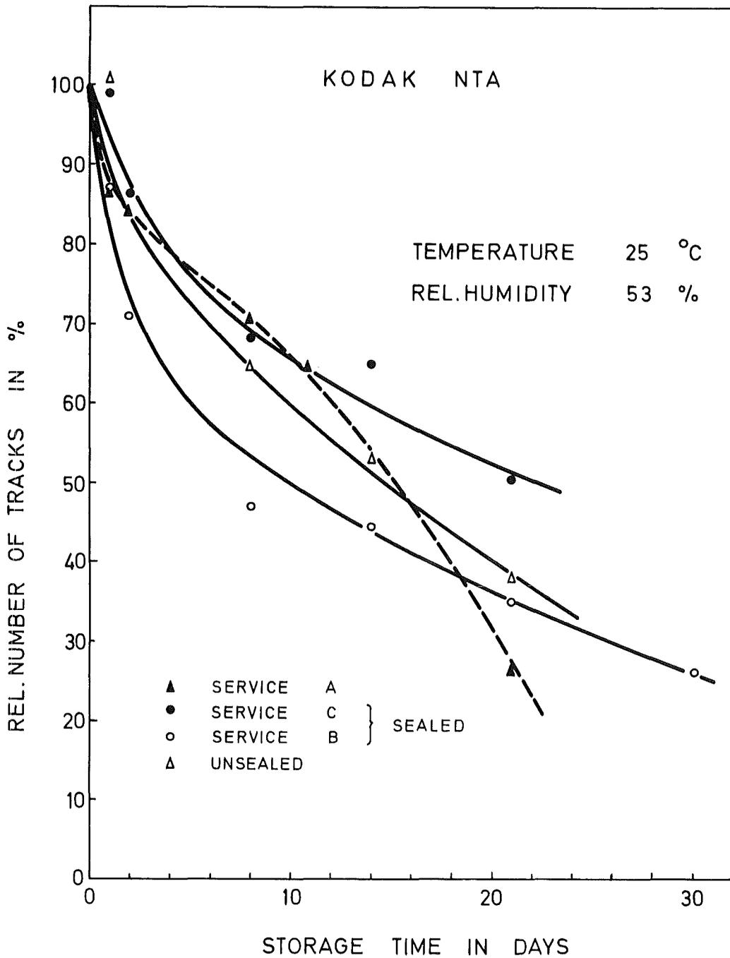
Fig. 12: Comparison of track fading in Kodak NTA from different services for films stored at 25°C and 53 % R.H.
