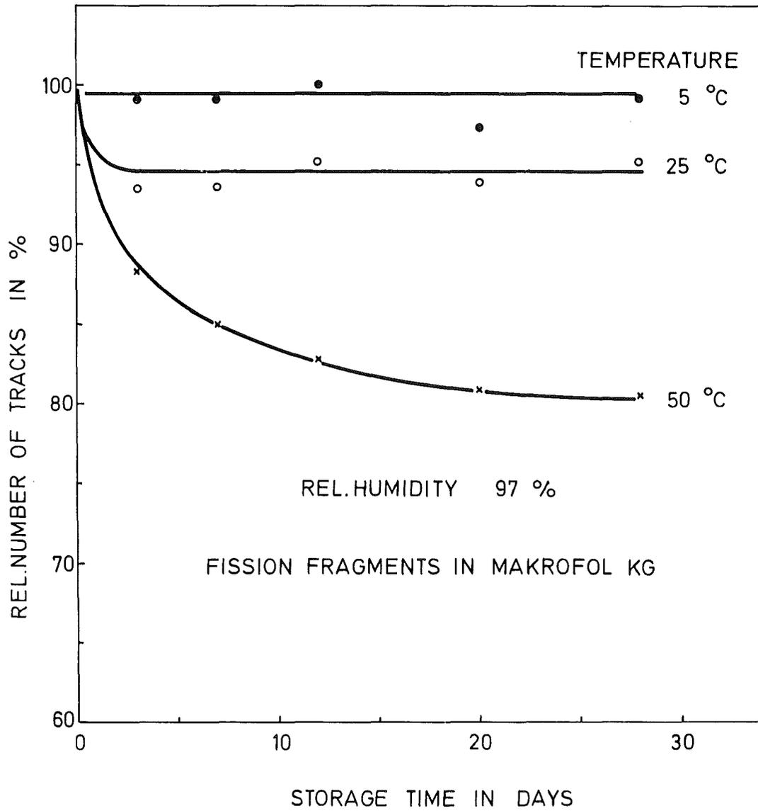
Fig. 18: Latent track fading in Makrofol KG stored at 97 % R.H. and different temperatures
