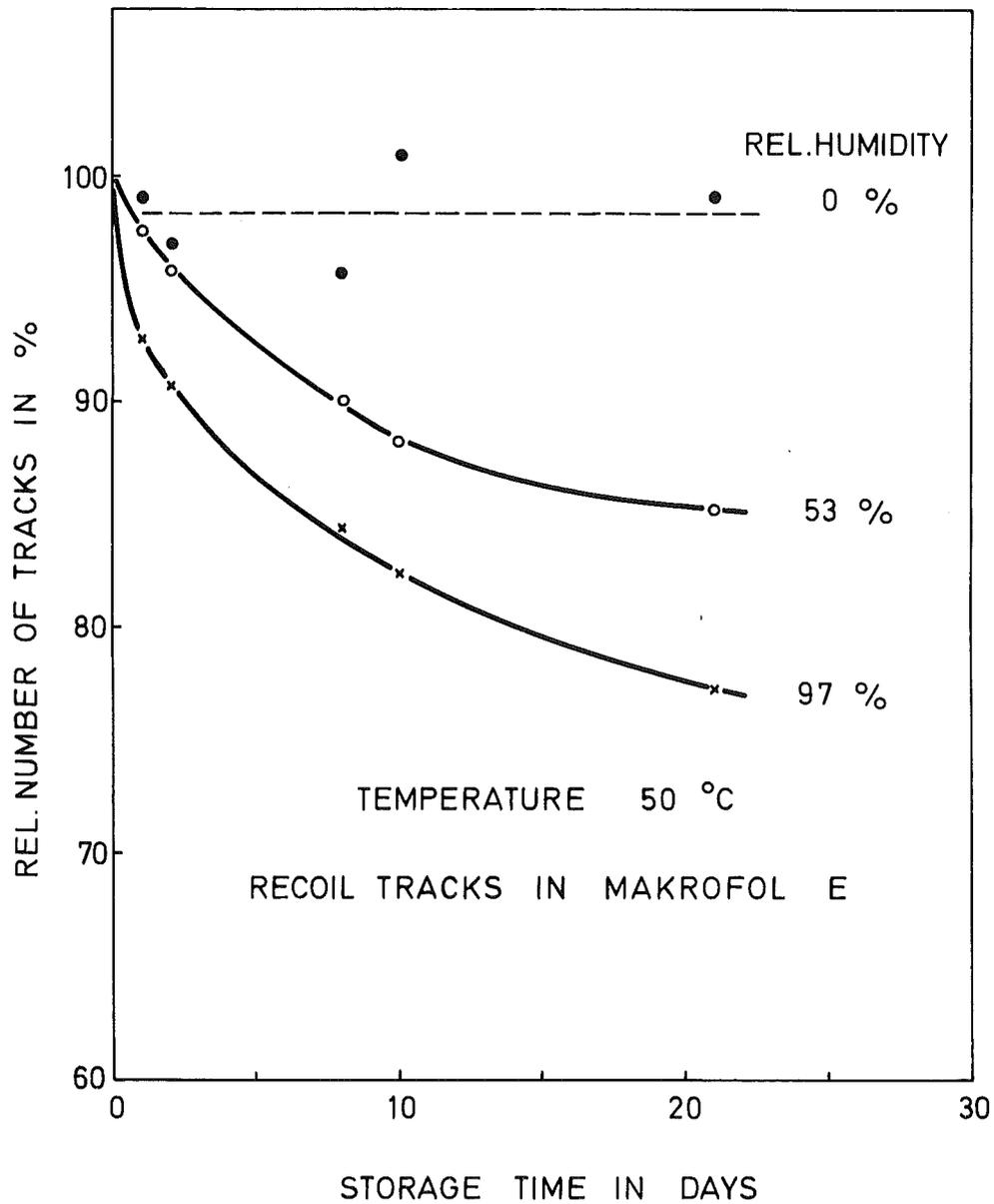
Fig. 29: Variation of the relative number of tracks with storage time for recoils in Makrofol E stored at 50°C and different relative humidities.
