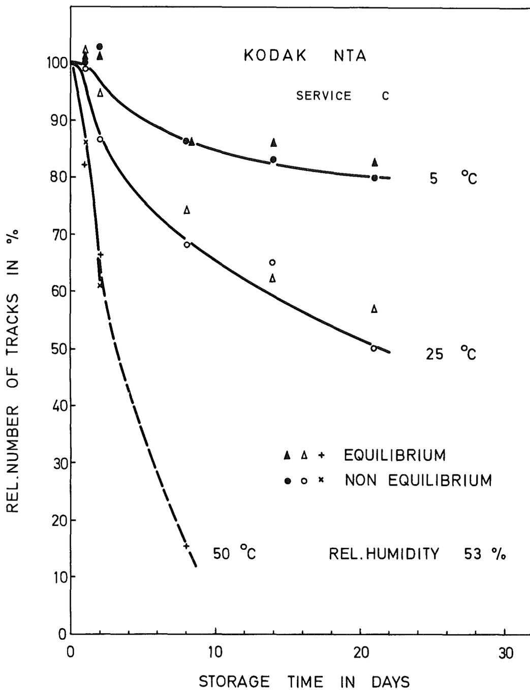
Fig. 11: Fading of latent tracks in Kodak NTA, service C, at 53 % R.H. and different temperatures for 1 week equilibrated and for nonequilibrated films
