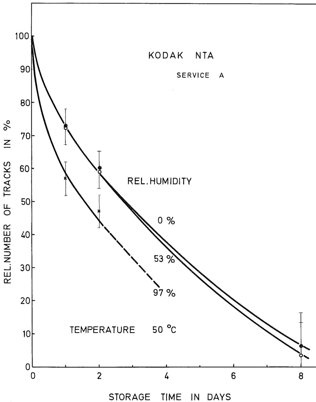
Fig. 6: Relative number of tracks vs. storage time, Kodak NTA, service A, held at 50°C and various relative humidities.
