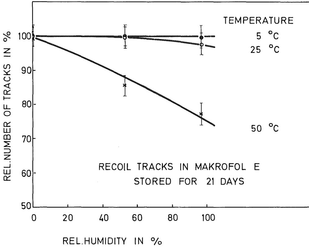
Fig. 30: Relative number of tracks vs. relative humidity for recoils in Makrofol E stored for 21 days at different temperatures
