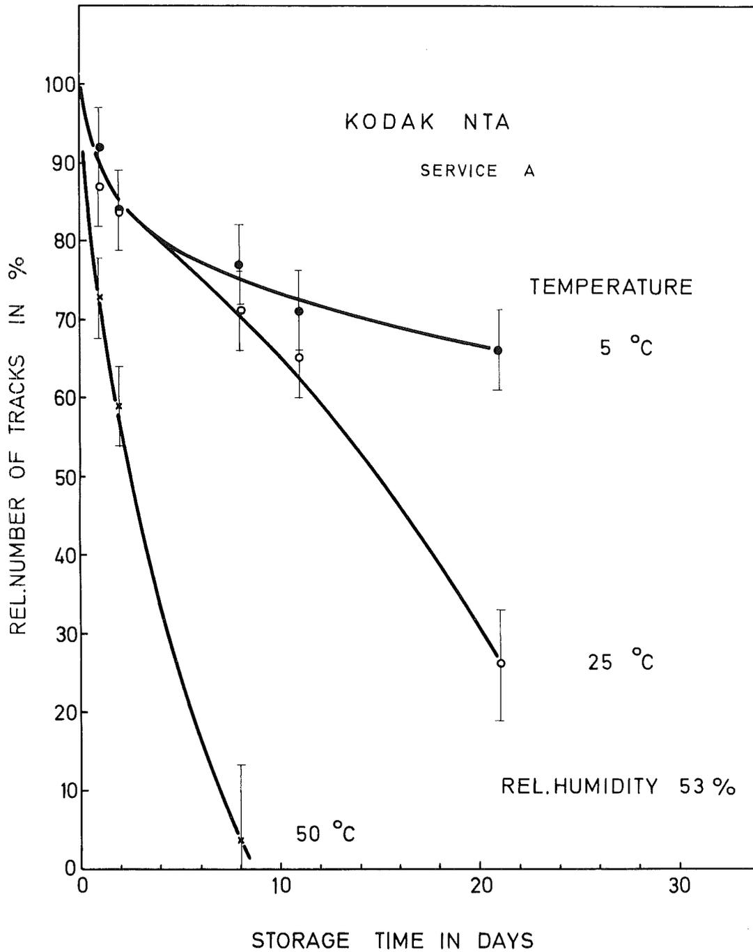
Fig. 7: Kodak NTA from service A stored at 53 % R.H. and different temperatures
