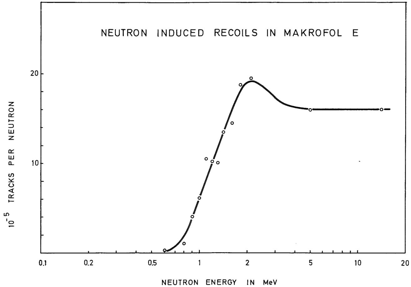
Fig. 2: Energy dependence of neutron induced recoils
