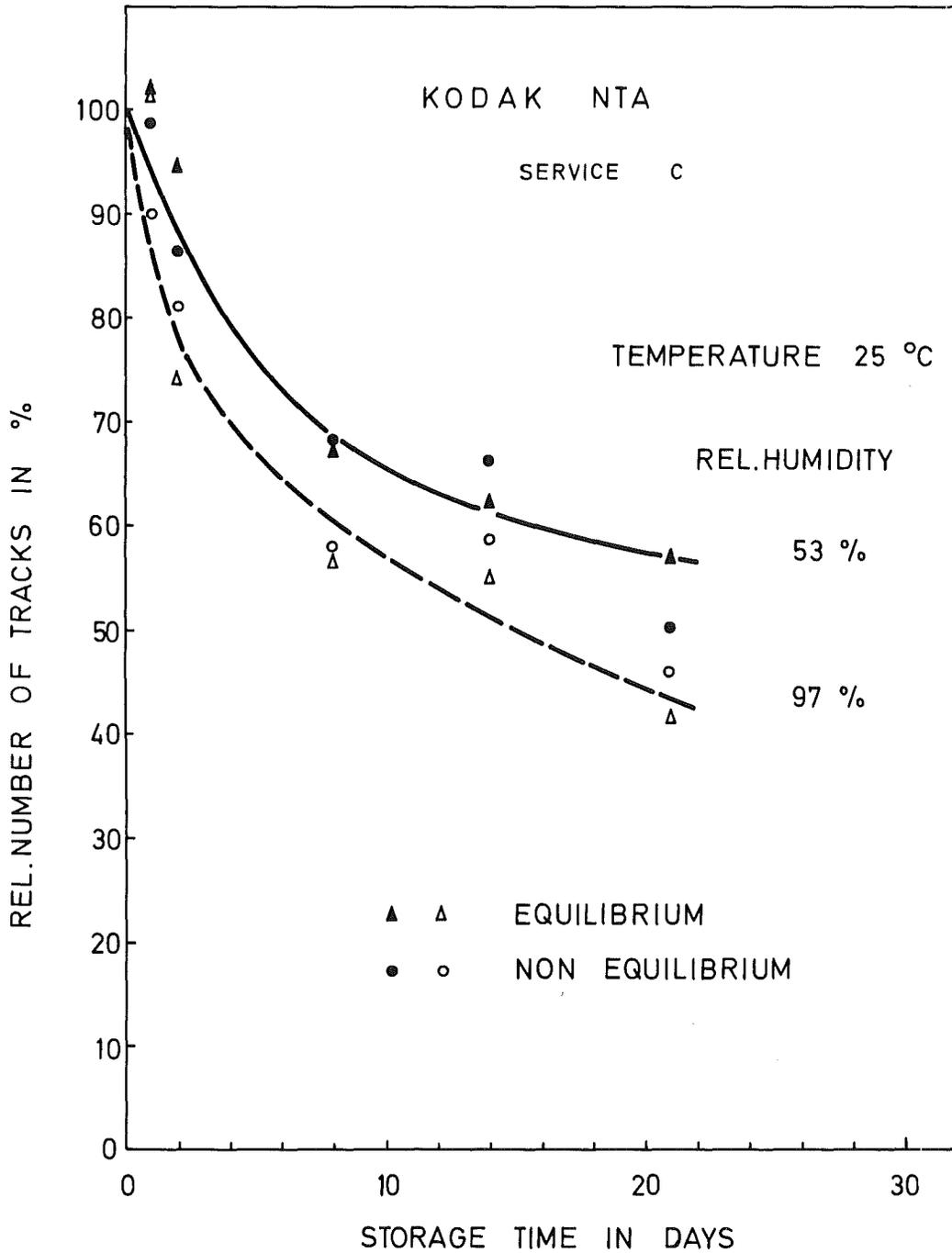
Fig. 10: Latent track fading in Kodak NTA from service C, stored at 25°C and 53 % and 97 % R.H. for films equilibrated for 1 week prior to exposure and for nonequilibrated films
