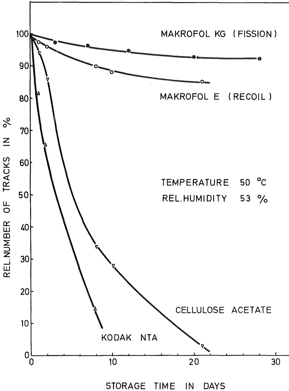
Fig. 35: Relative number of tracks as a function of storage time for Kodak NTA, Makrofol and cellulose acetate, stored at 50°C and 53 % R.H.
