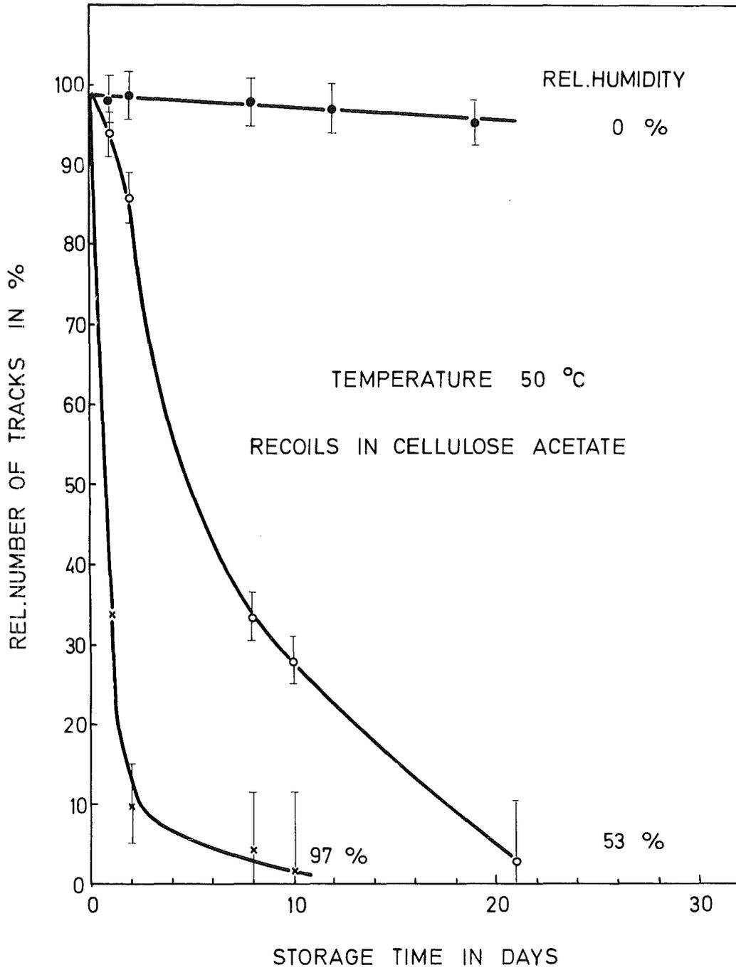
Fig. 22: Latent track fading for neutron induced recoils in cellulose acetate at 50°C and various relative humidities.
