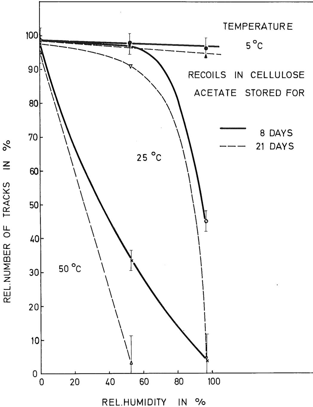
Fig. 26: Relative number of tracks vs. relative humidity for recoils in cellulose acetate stored for 8 and 21 days at different temperatures
