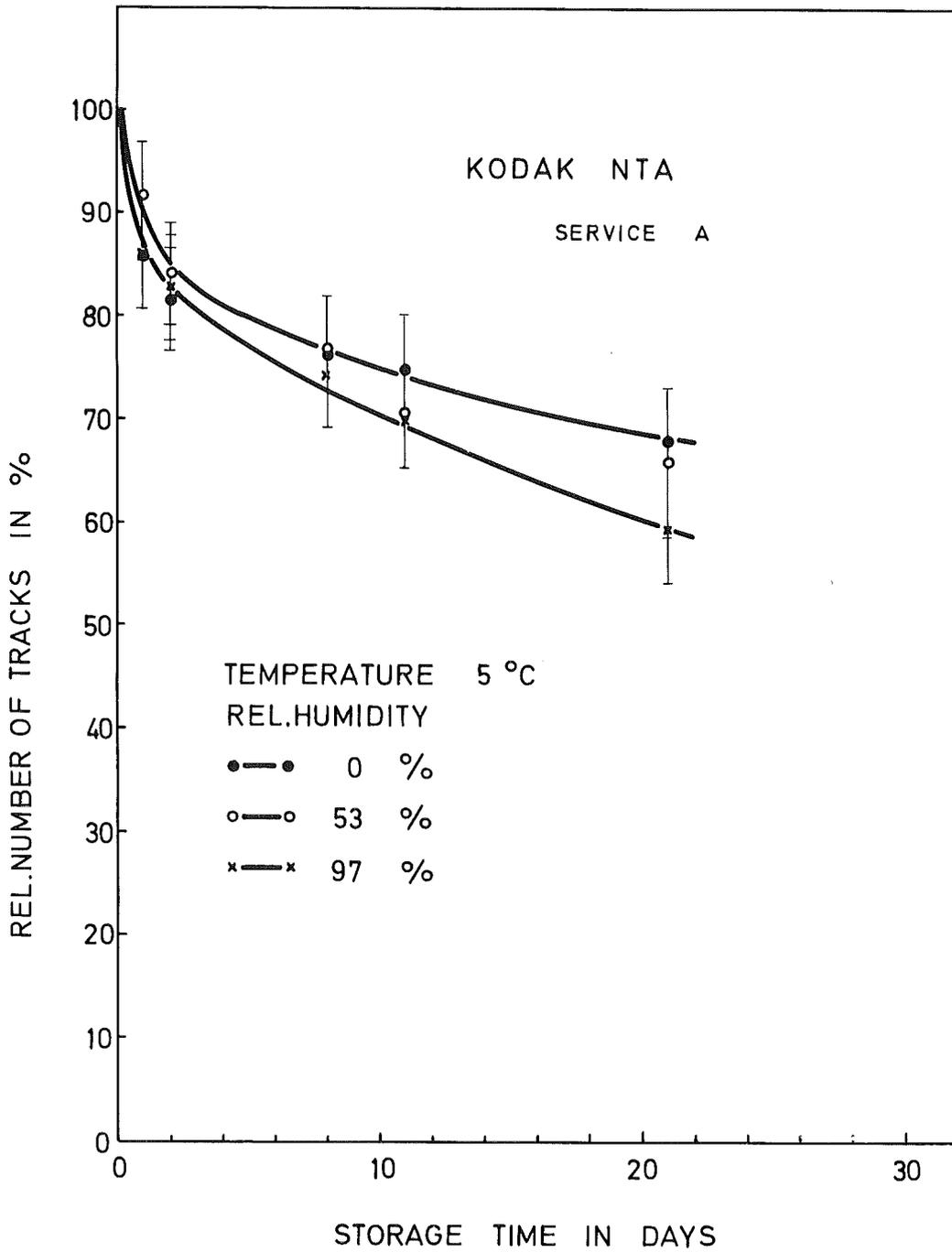
Fig. 4: Variation of the relative number of tracks with storage time for Kodak NTA from service A, stored at 25°C and different relative humidities.
