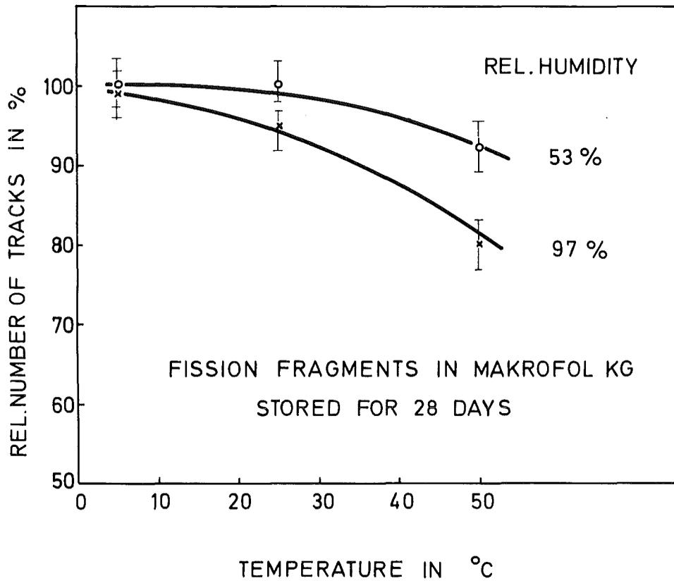
Fig. 20: Relative number of tracks vs. temperatures for fission fragments in Makrofol KG stored for 28 days at different relative humidities.
