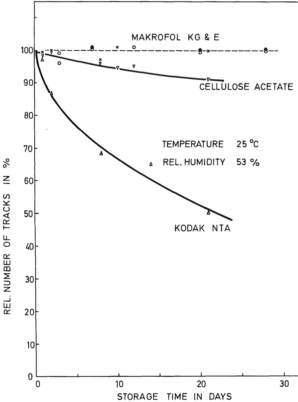
Fig. 33: Comparison of latent fading in Kodak NTA, Makrofol and cellulose acetate, held at 25°C and 53 % R.H.
