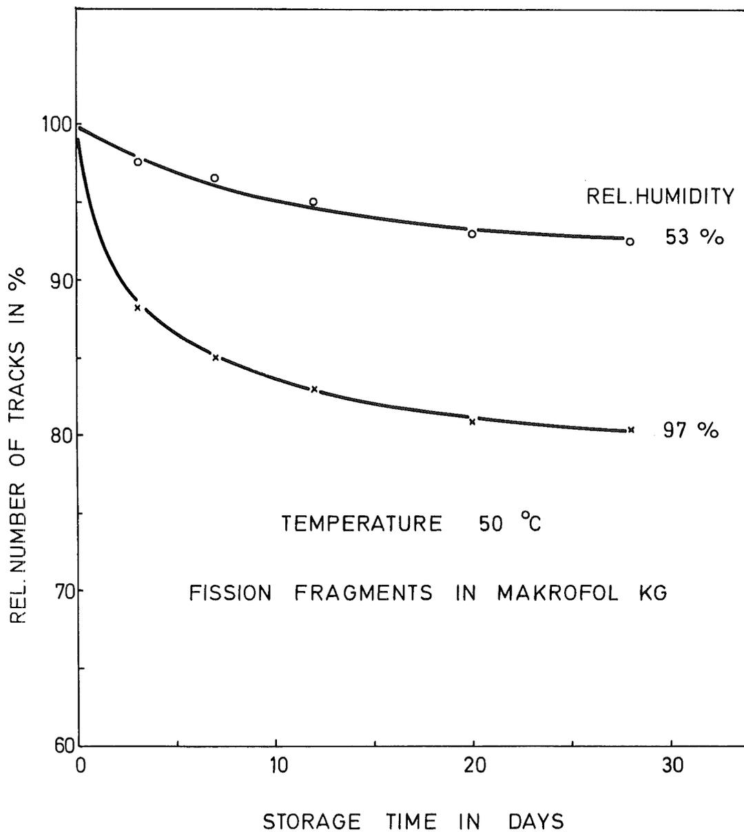
Fig. 19: Latent track fading in Makrofol KG held at 50°C and different relative humidities.
