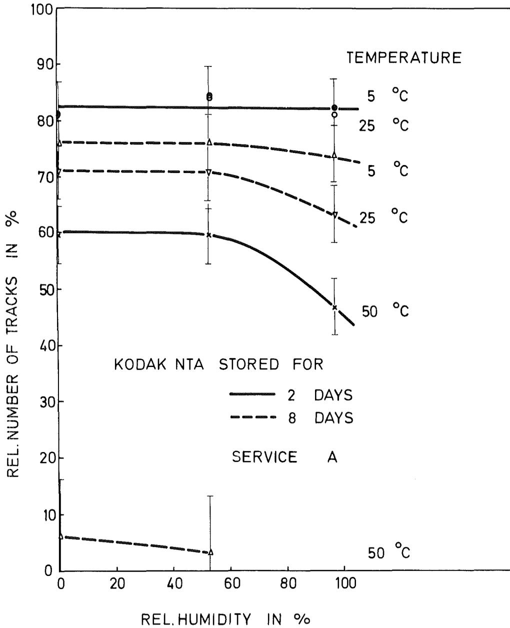
Fig. 15: Latent track fading in NTA, service A, with relative humidity. Films stored at different temperatures for 2 and 8 days.
