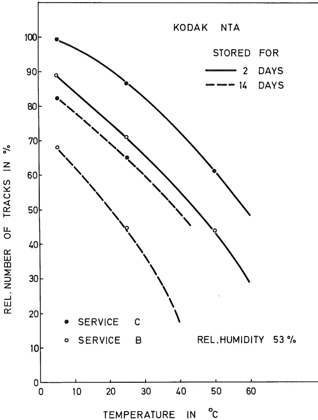
Fig. 13: Relative number of tracks vs. temperature for Kodak NTA from services B and C stored for 2 and 14 days at different relative humidities.
