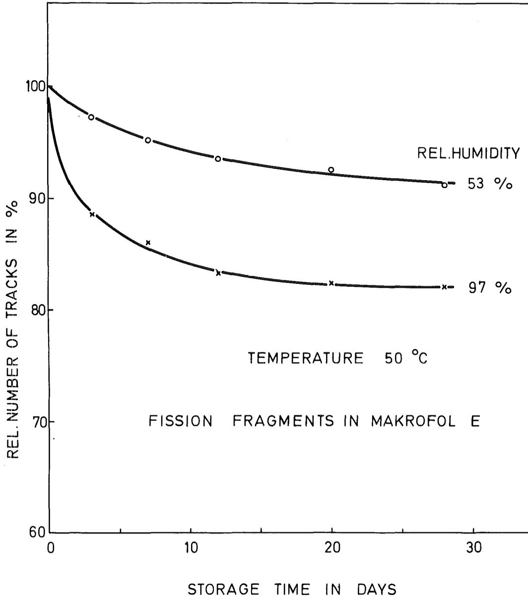
Fig. 17: Relative number of track as a function of storage time for fission fragments in Makrofol E stored at 50°C and different relative humidities.
