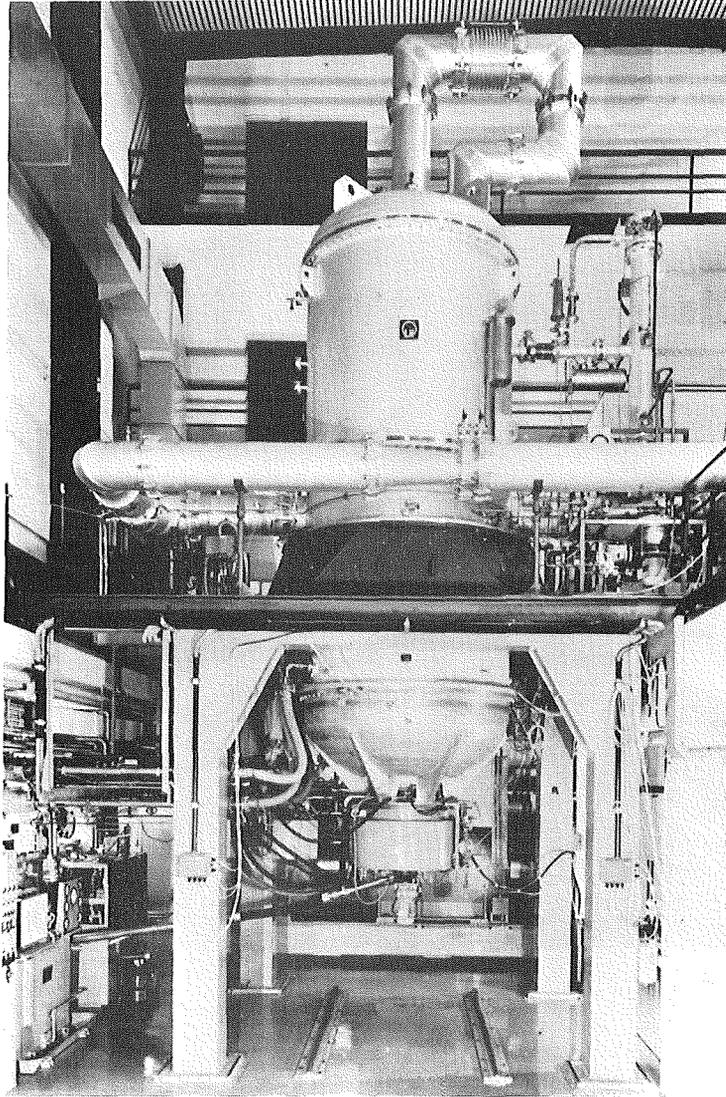
Fig. 6: View of the prototype separative stage.
