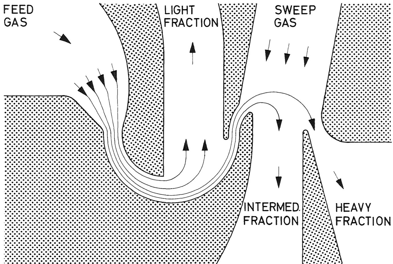
Fig. 11: Advanced separation nozzle system. The heavy fraction of the first nozzle is deflected in the second nozzle by a sweep gas.
