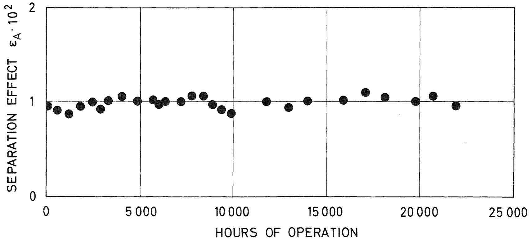
Fig. 3: Life test of a commercial separation element.
