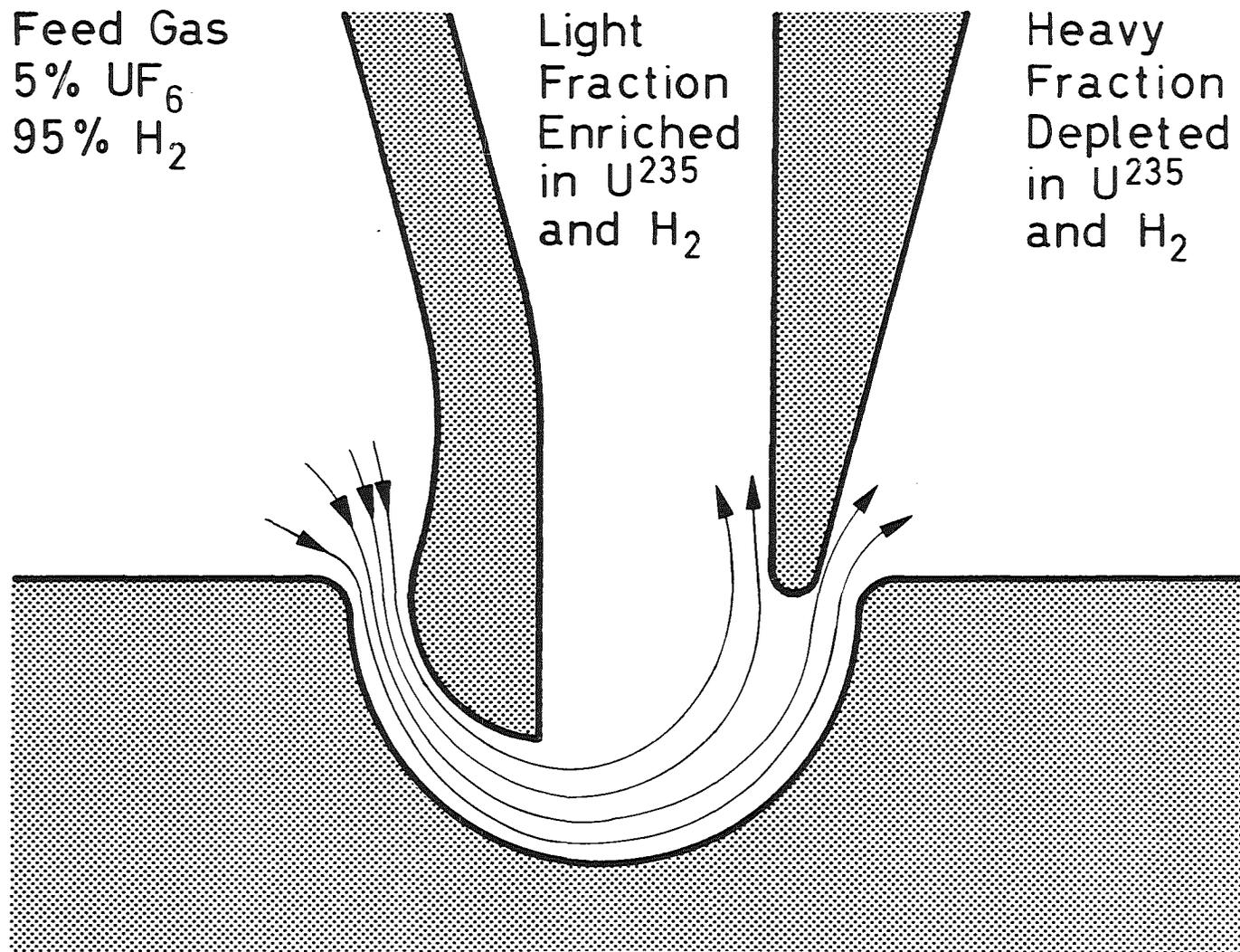
Fig. 1: Cross-section of the separation nozzle system used to date in the commercial implementation of the separation nozzle process.
