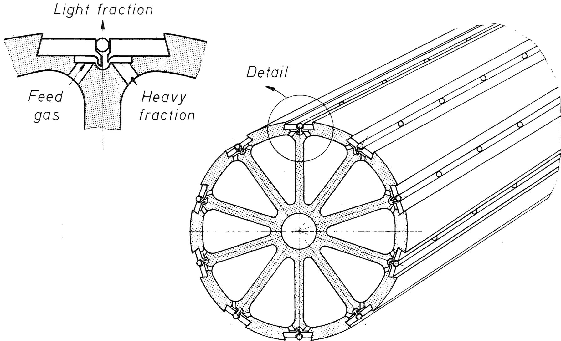
Fig. 2: Separation element tube with 10 separating slits manufactured in a commercial fabrication process.
