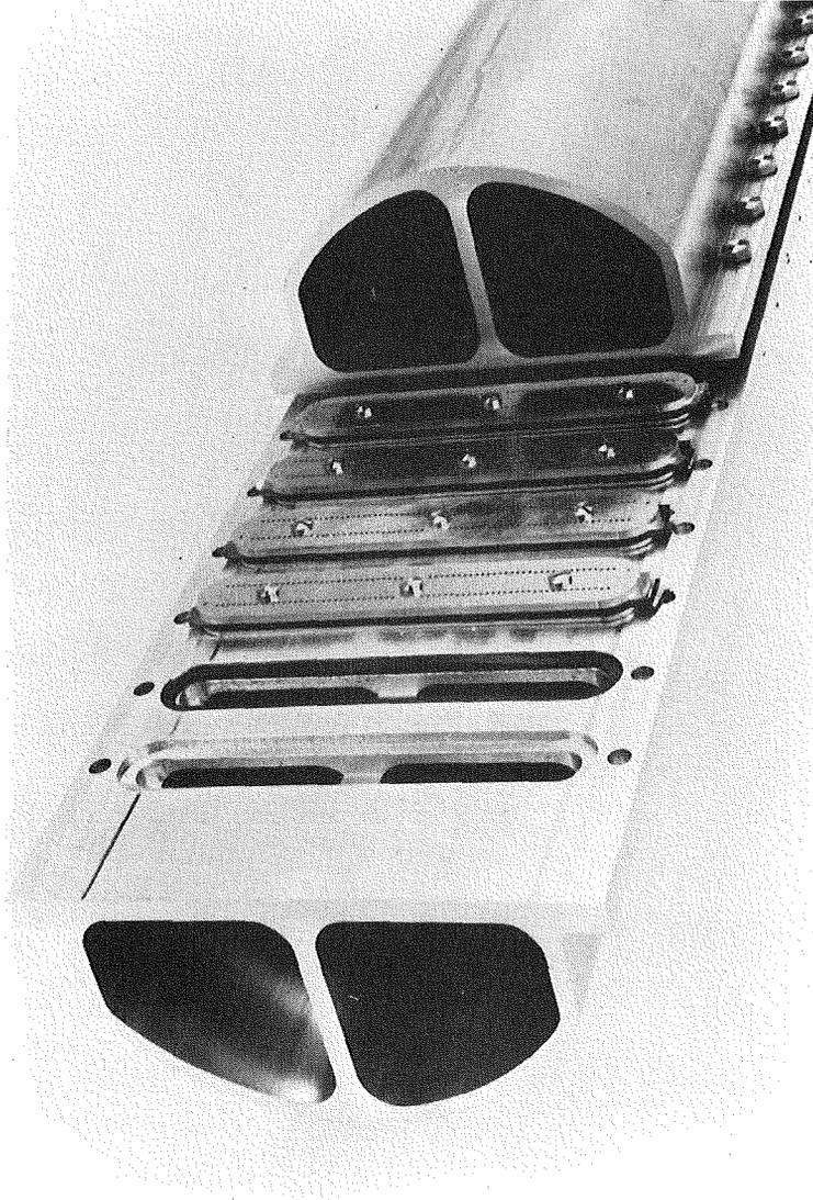
Fig. 14: Separation element tube with photo-etched separation nozzles.
