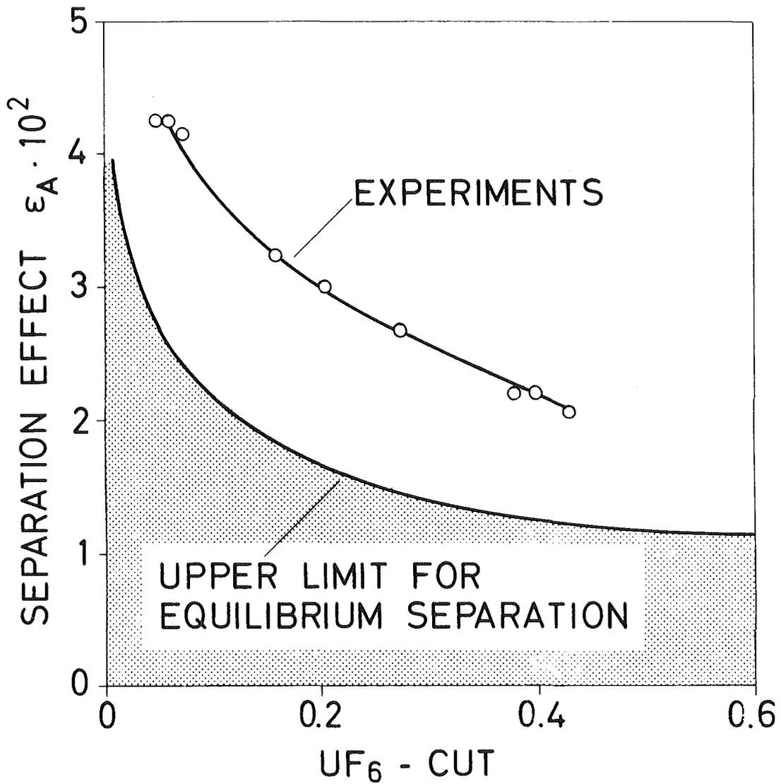
Fig. 10: The upper curves indicates the experimentally determined relation between the separation effect  $\epsilon_A$  and the  $UF_6$ -cut  $\mathcal{S}$  (mixture of  $UF_6/H_2$  with 1.6 mole-%  $UF_6$ ; expansion ratio 8). The lower curve gives the upper limit for equilibrium separation calculated for infinite flow velocity.
