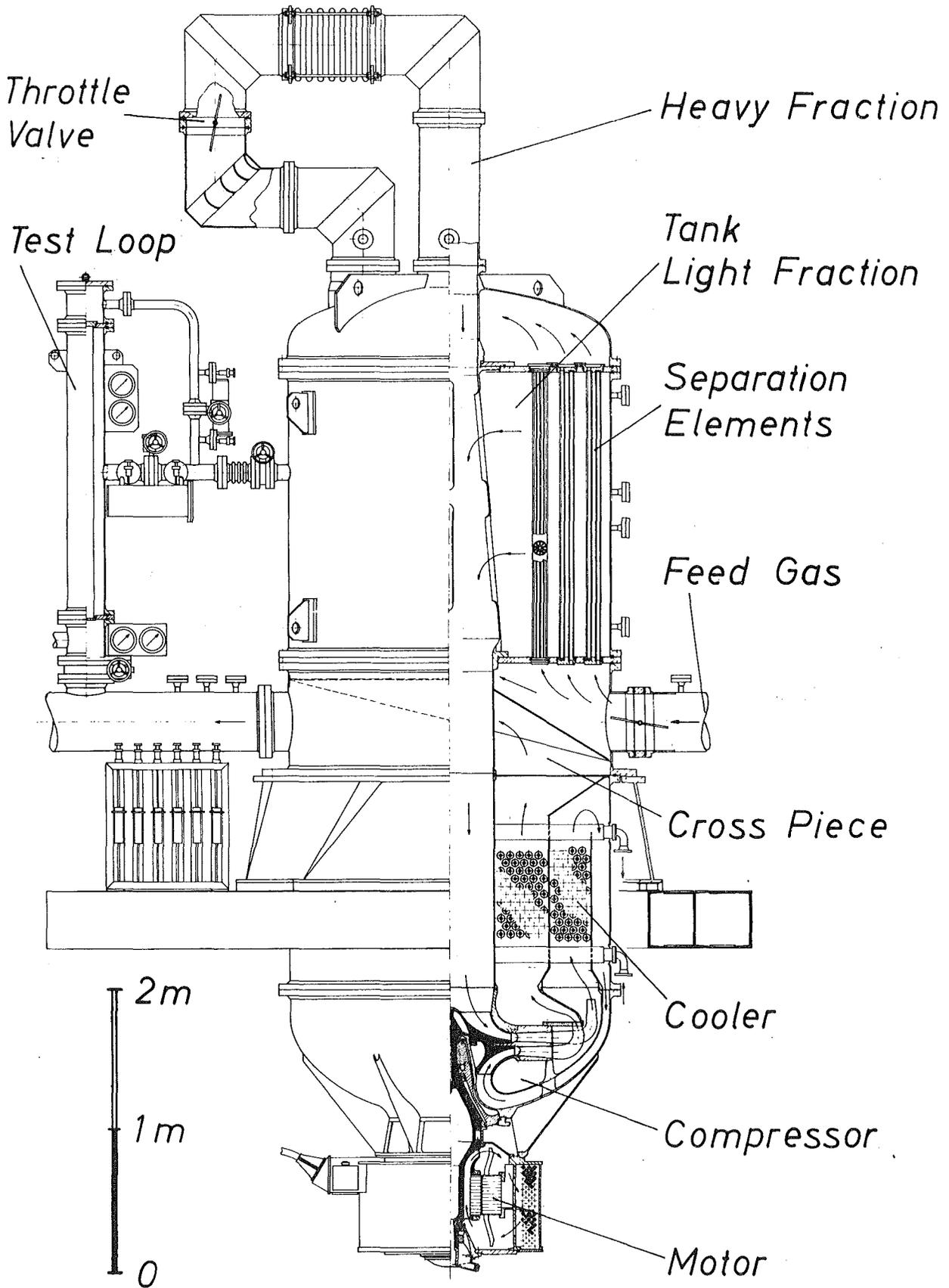
Fig. 5: Cross-section of the prototype separative stage.
