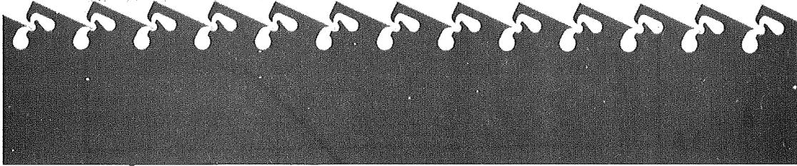
Fig. 13a: Metal foil with separation nozzle structures applied by means of photo-etching.
