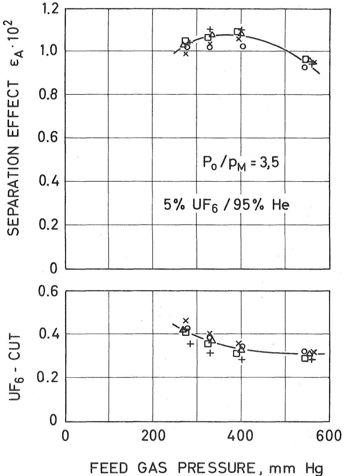
Fig. 4: Results of separation experiments in 5 separation element tubes of 2 m length with 20 m slit-length each.
