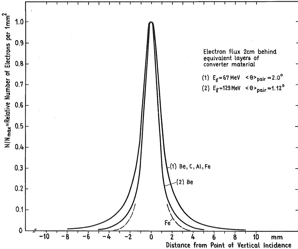
Fig. 4: Distribution of electrons hitting a detector plane 2 cm behind the surfaces of  $\gamma$ -converters with an efficiency  $\eta = 0.07$ . The quanta are moving vertically onto the converter. The whole figure shows rotational symmetry around the momentum axis of the quanta. Curve 1: quanta from  $\pi^0$  decay, curve 2: quanta from radiative capture.
