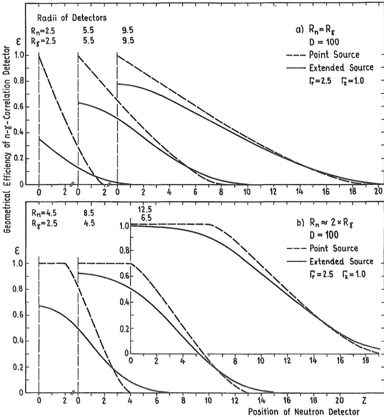
Fig. 8: Geometrical efficiency  $\epsilon$  of a detector pair for neutrons and  $\gamma$ -quanta as a function of the position of the gamma detector. The parameters are the source extension and the detector size.
