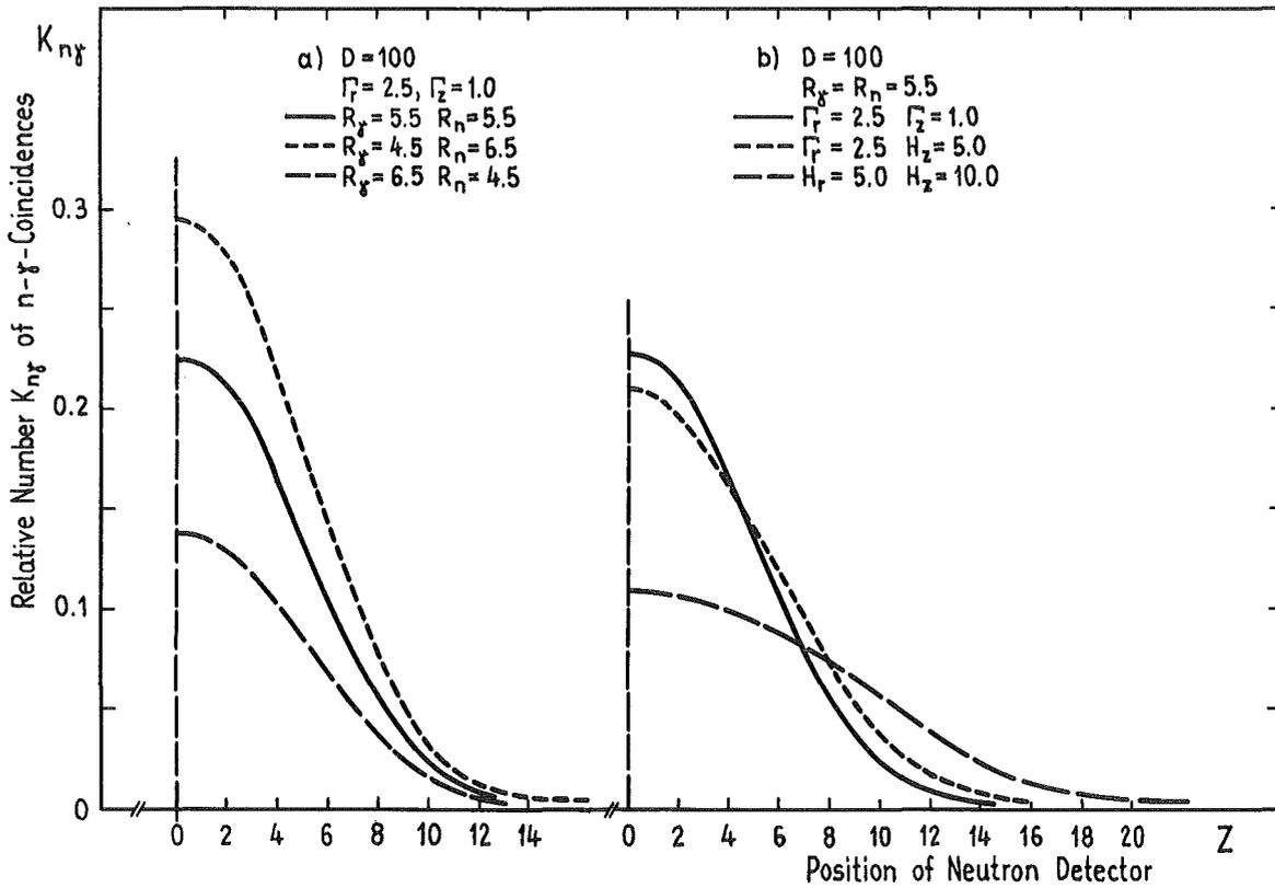
Fig. 10: Relative number of coincidences as a function of the position of the neutron detector calculated by means of Monte-Carlo methods.
