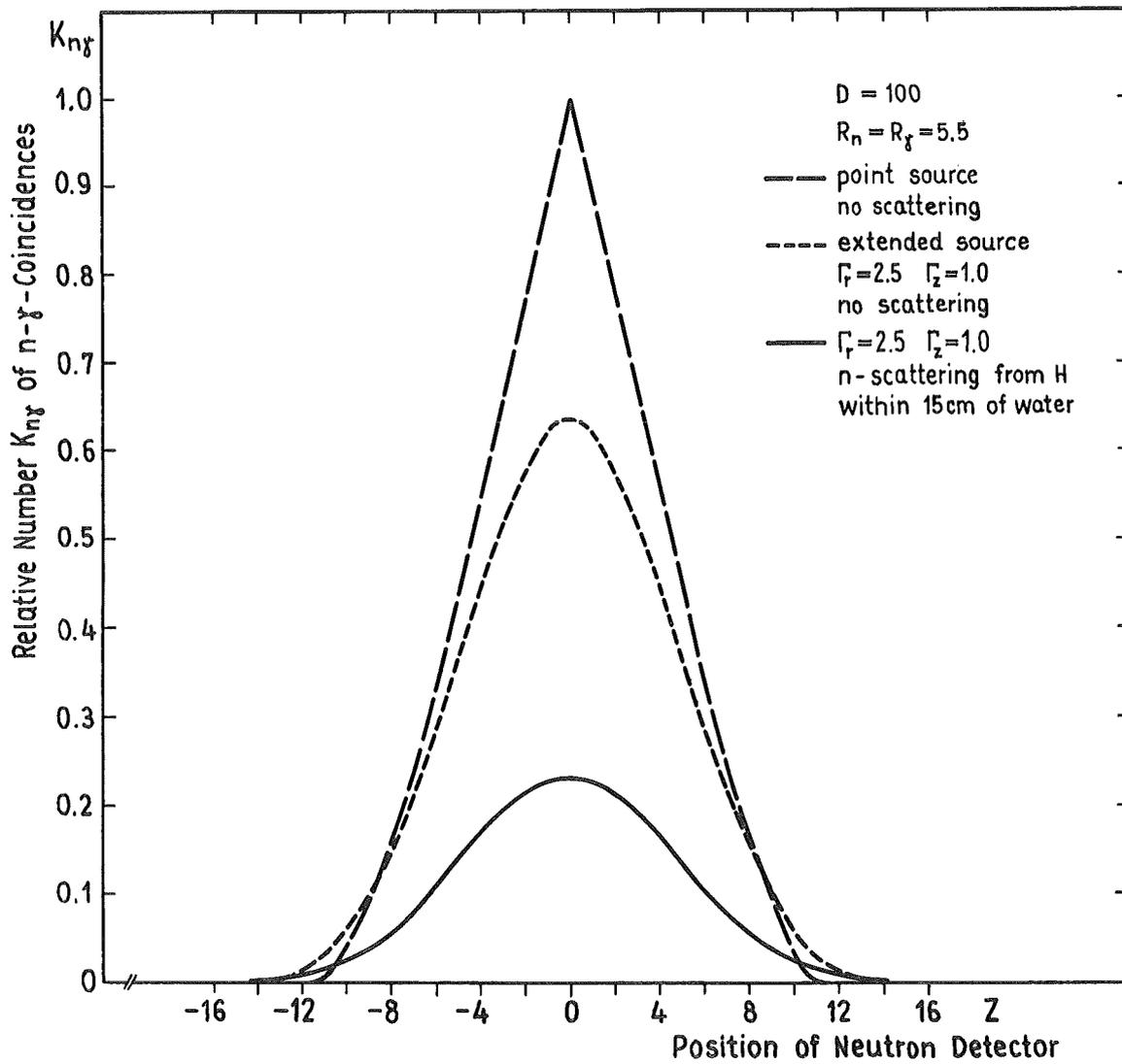
Fig. 9: Relative number of coincidences as a function of the position of the neutron detector calculated using Monte-Carlo methods. Neutron scattering from hydrogen within the water phantom has been taken into account.
