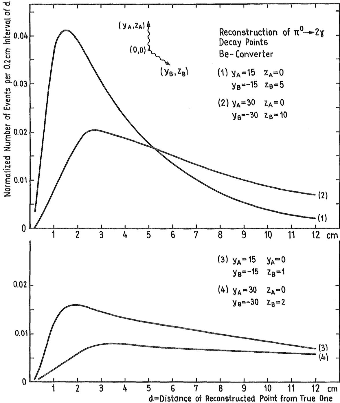
Fig. 6: Distribution of distances of the reconstructed decay points from the true point as a function of the detector geometry and the angle between the two gamma quanta. For curves (1) and (2), the angle between the quanta is fixed to  $162^\circ$ , for curves (3) and (4) the angle is  $176^\circ$ . The relative probability of decay quanta showing these angles can be taken from fig. 2 (A shift of 15 cm should be taken into account for  $z_B$ ).
