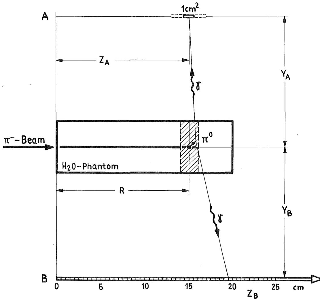
Fig. 1: Schematic setup for topography using the charge exchange reaction. A and B are two parallel planes of detector elements. They are cut vertical to their surface and parallel to the incoming beam.
