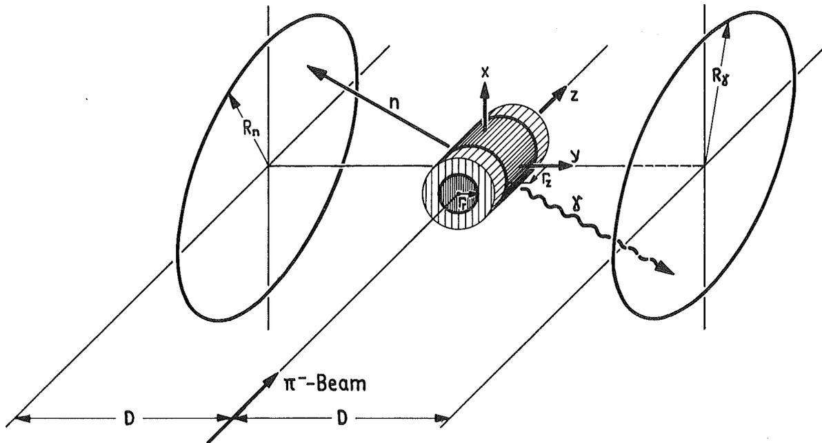
Fig. 7: Schematic geometry for range monitoring using  $\pi^-$  radiative capture from protons at rest. The beam extension is chosen axially symmetric and the stopping interval is distributed around  $z = 0$ .  $\Gamma_r$  and  $\Gamma_z$  are the standard deviations in the Gaussian distribution functions accepted for the radial extension and the stopping interval of the beam.
