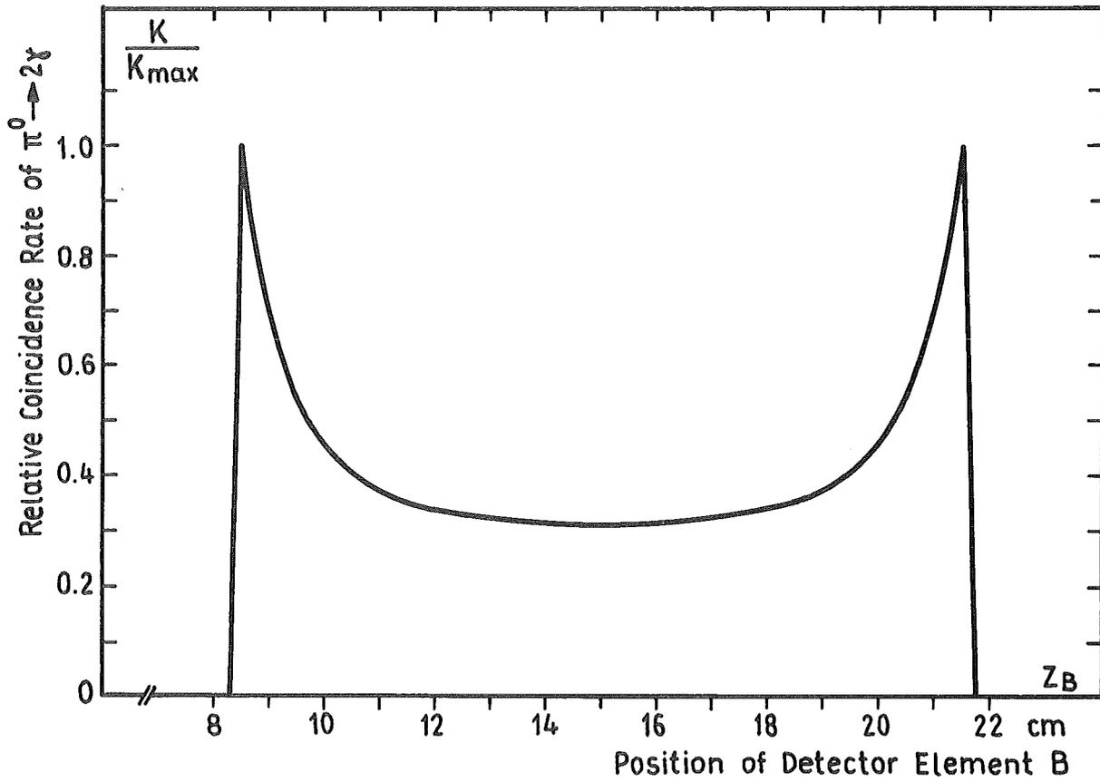
Fig. 2: Distribution of  $\gamma\gamma$ -coincidences  $K$  from  $\pi^0$ -decay. One detector element is fixed at  $y_A (= -y_B) = 15$  cm;  $z_A = 15$  cm. All particles  $\pi^0$  are generated from protons at rest and emitted isotropically from the point  $y = 0$ ;  $z = R = 15$  cm.
