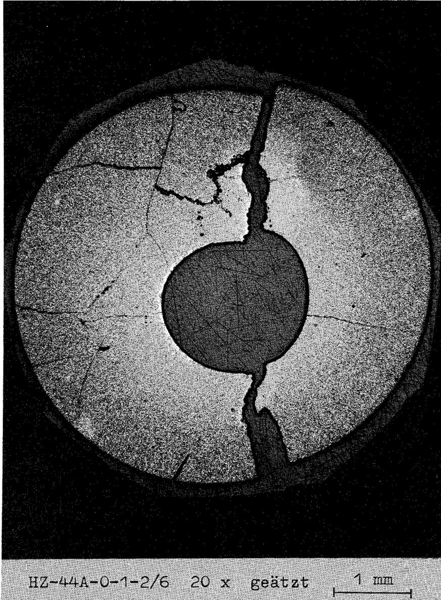
Fig. 10 Pellet cut after the TOP-experiment E5
