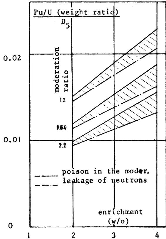
Fig. 14. Calculated Pu/U/U-235 depletion vs initial fuel enrichments with different reactivity control methods and moderation ratios for different PWR fuels. (from ref. 23)
