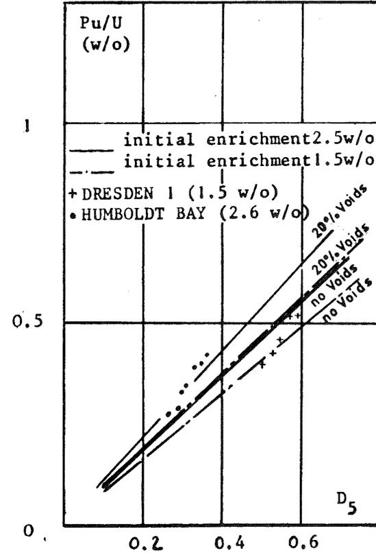
Fig. 15. Calculated Pu/U ratio vs U-235 depletion for different BWR fuels and different void contents of the moderator: comparison with experimental data (from ref. 23)
