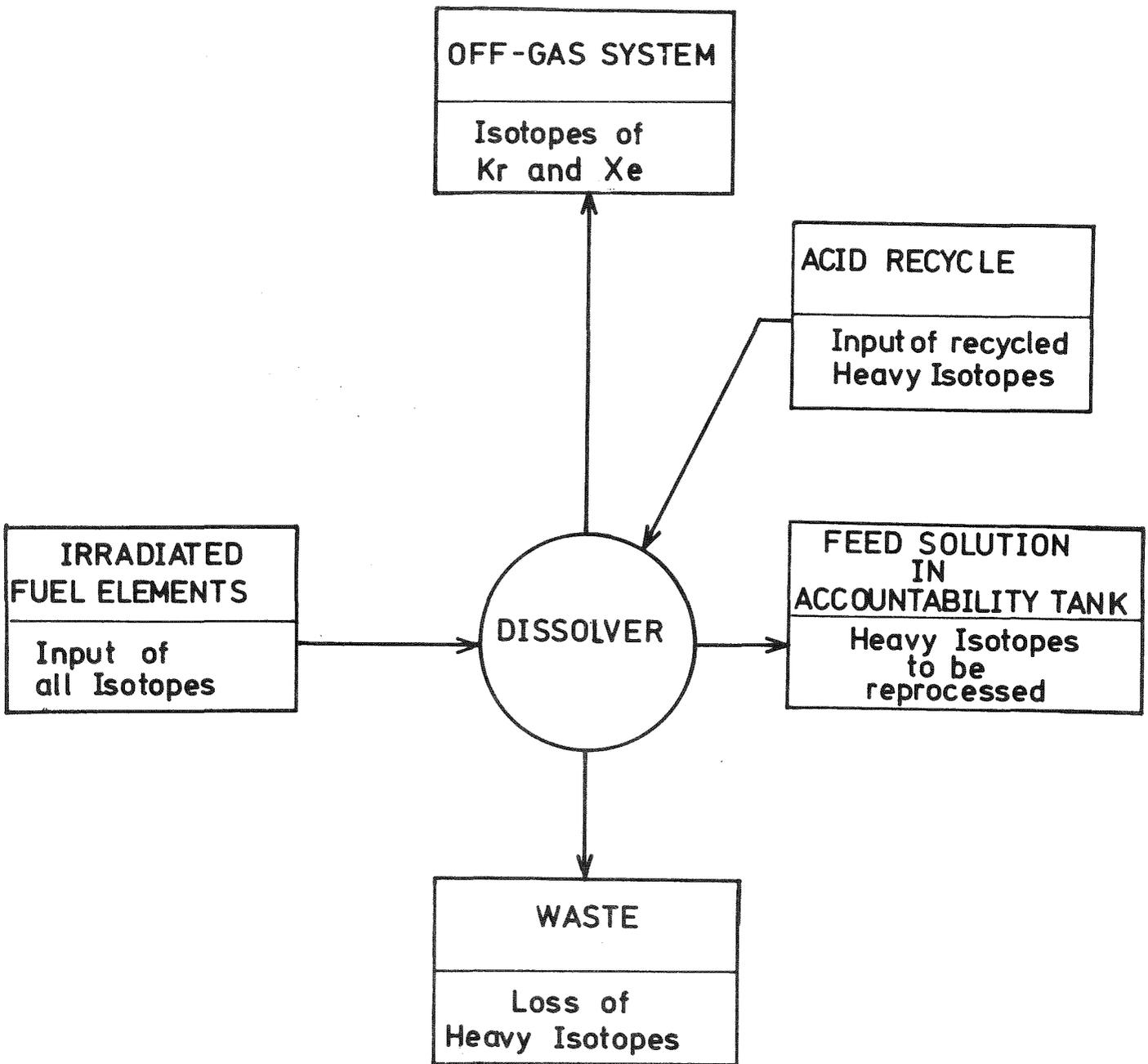
Fig.20 Relevant Steps for Isotopic Correlations around the dissolver of a reprocessing Plant ( Ref.9 )
