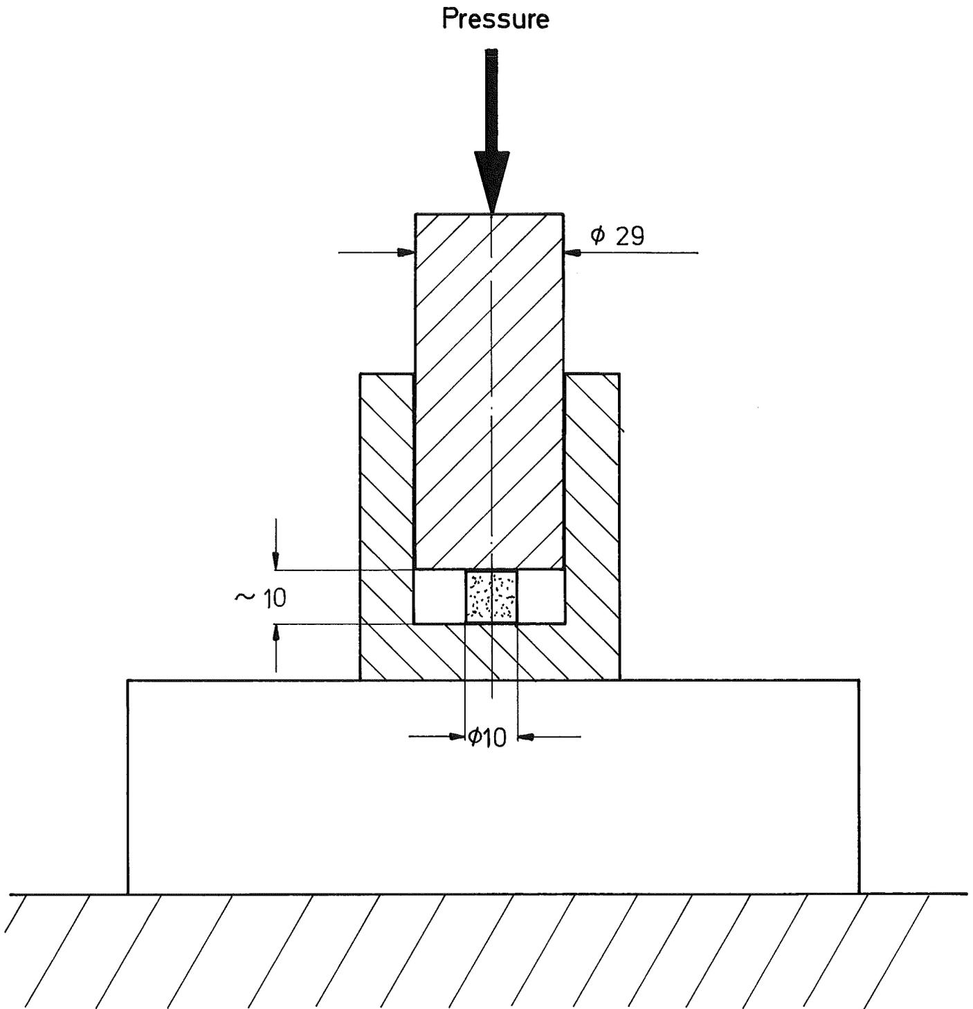
Testing Device for Mechanical Stability
