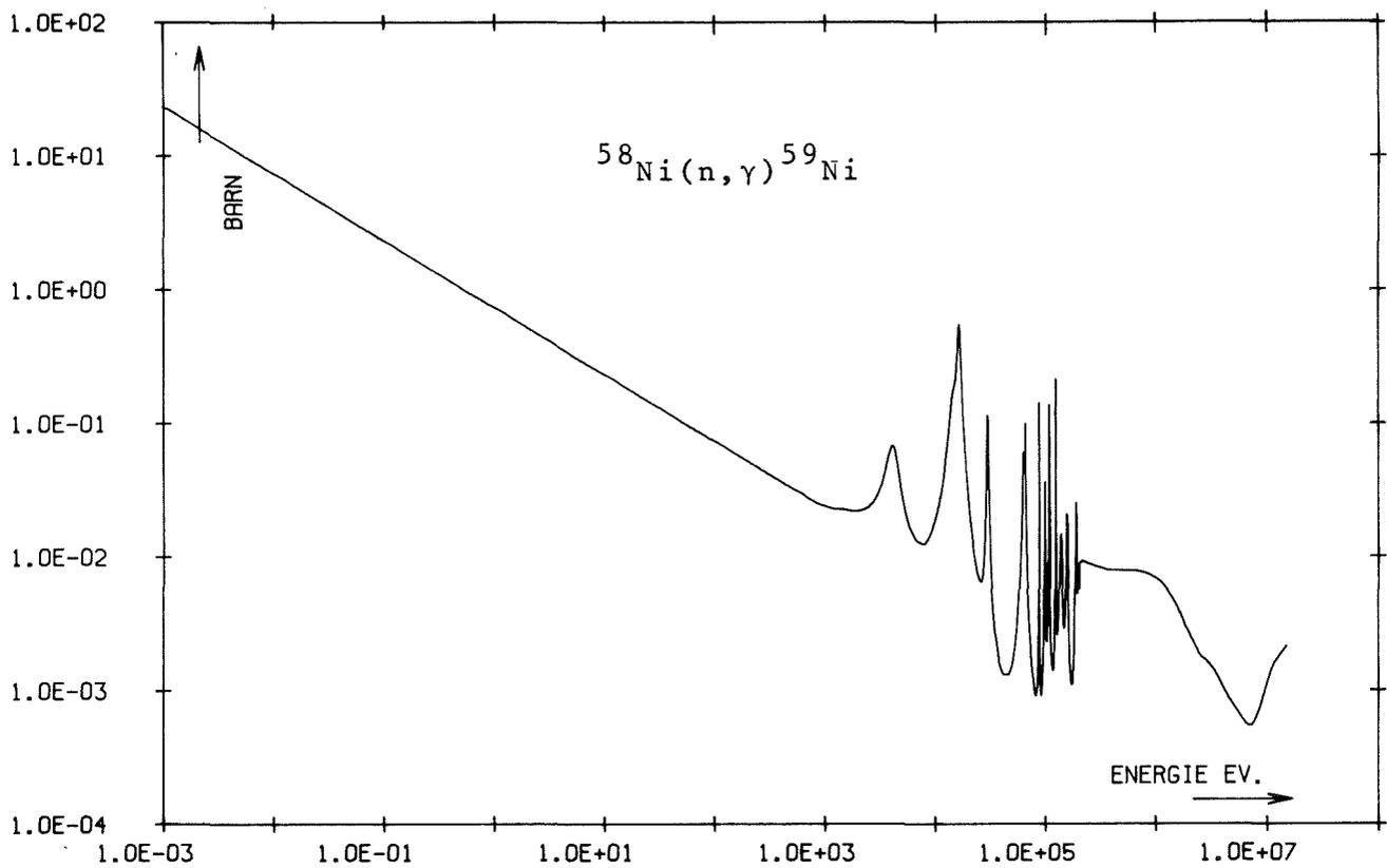
Fig. 5: Cross sections for the process  $^{58}\text{Ni}(n, \gamma)^{59}\text{Ni}(n, \alpha)^{56}\text{Fe}$
