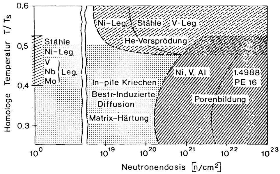
Fig. 1: Important radiation damages as function of neutron dose and temperature
