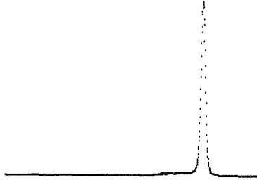
Fig. 1. Photomultiplier and electronic test for internal phase width showing that photomultiplier PM2 has a slightly better time resolution than PM1.
