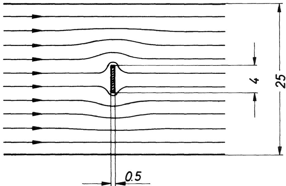
Fig. 8 Flow characteristics of electric current in the vicinity of a thermocouple
