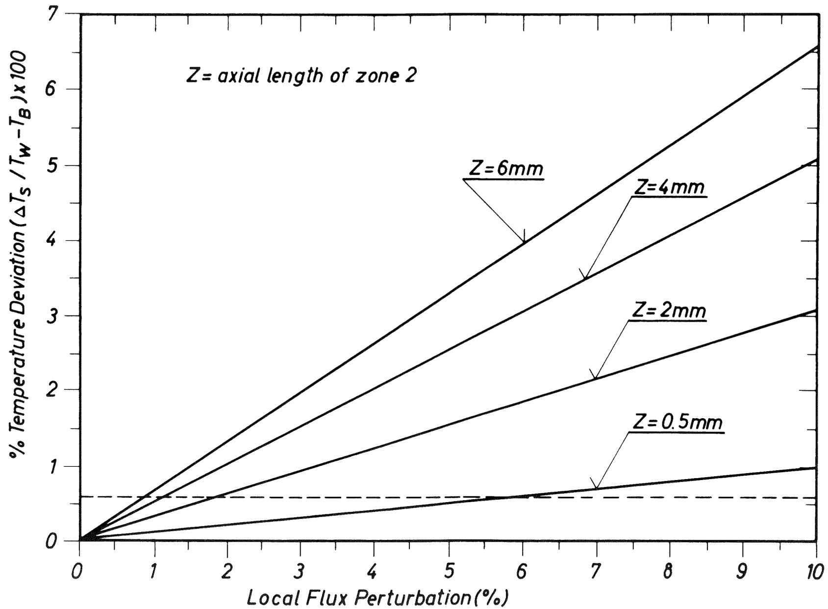
Fig. 9 Local Flux Perturbation VS Resulting Surface Temperature Deviation for BR-2 Rod.
