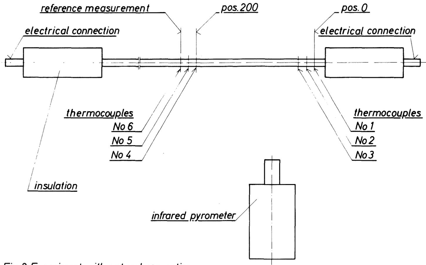
Fig.2 Experiment with natural convection
