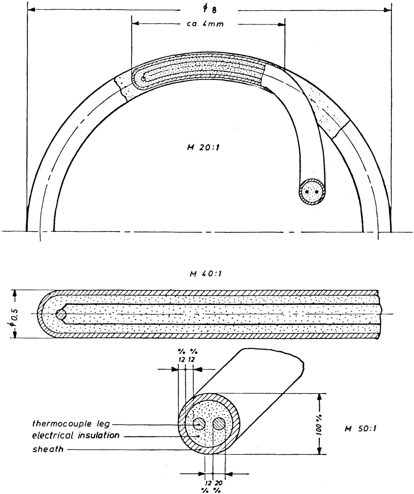
Fig. 1: Thermocouple installation in a BR-2 heater rod
