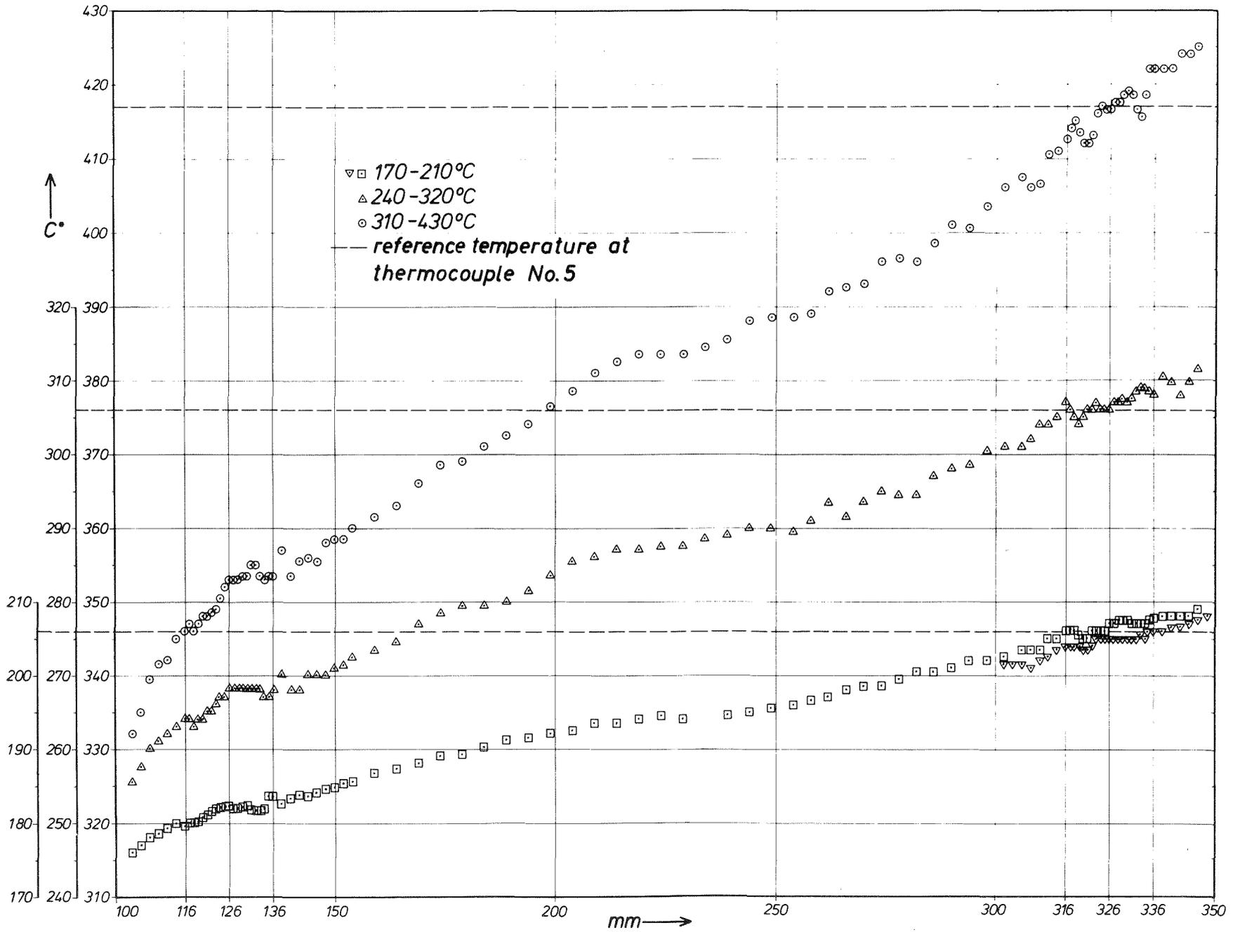
Fig. 6: Pyrometer reading along test rod for experiments with forced convection cooling
