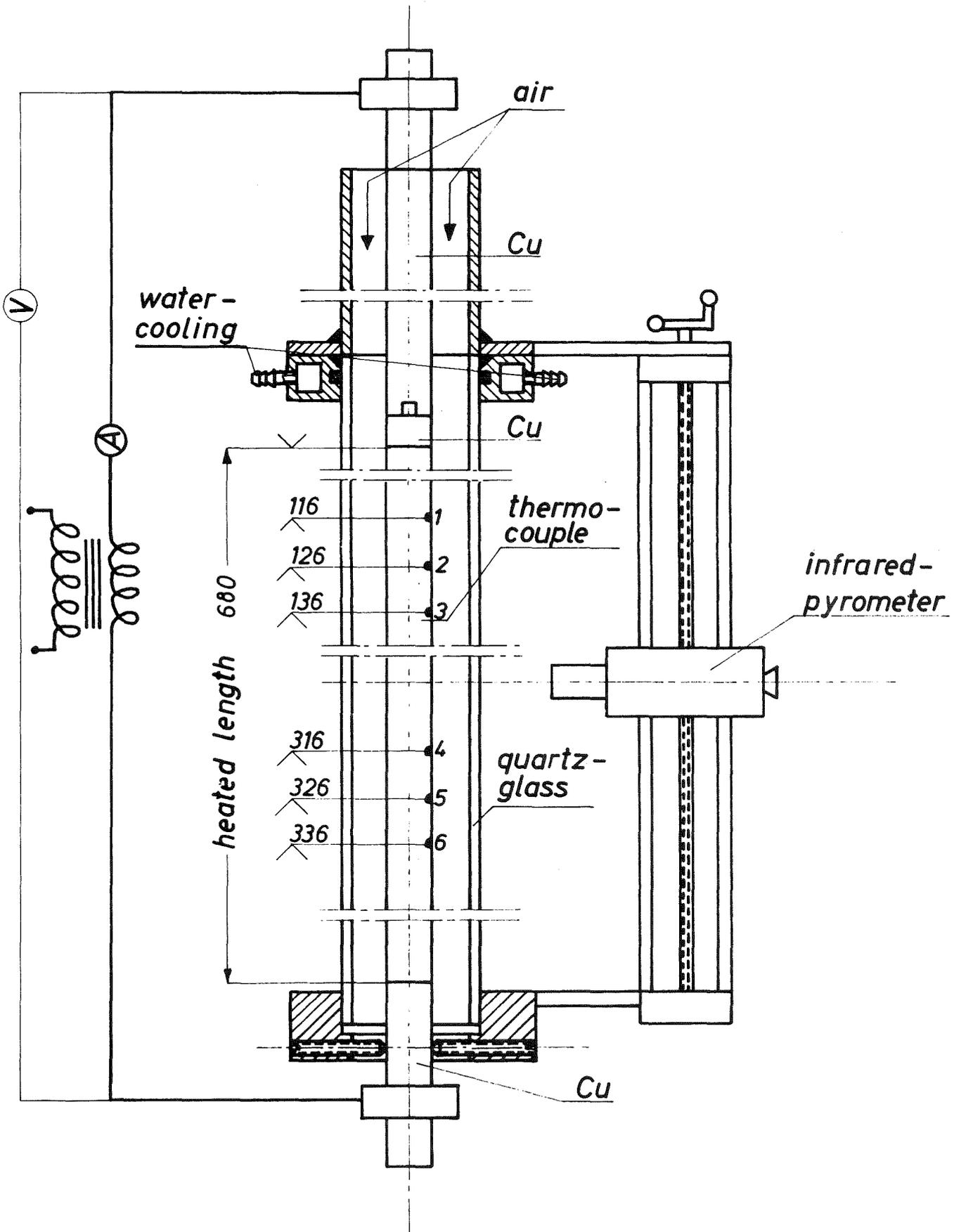
Fig. 5: Test rig for experiment with forced convection cooling
