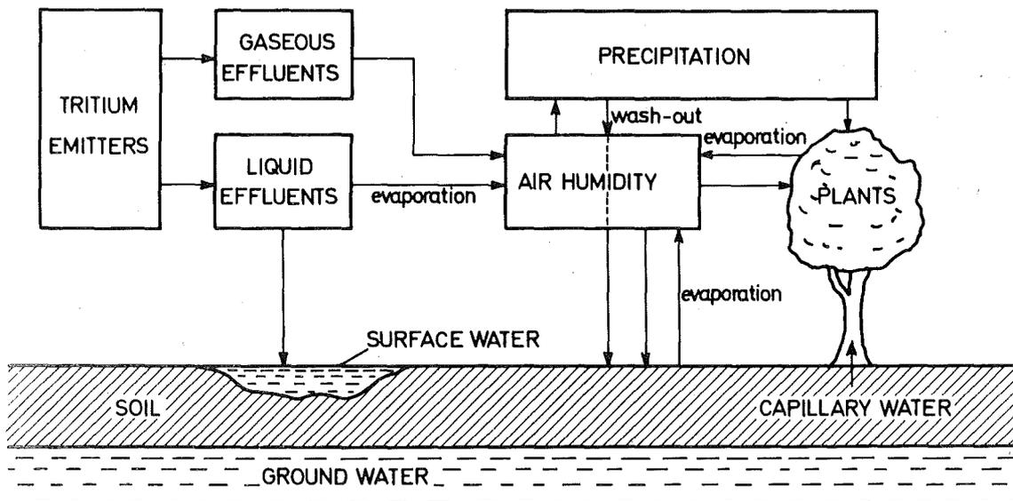
Fig. 20 Simplified model of the transport of tritium in the environment
