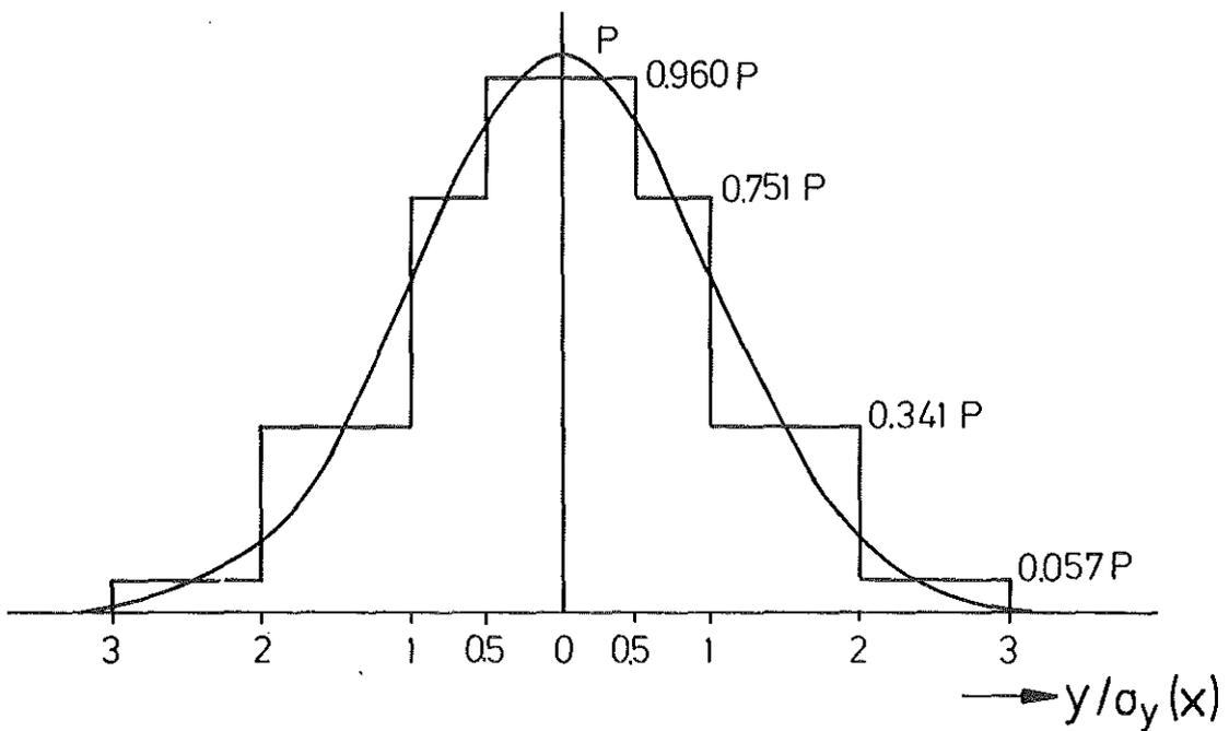
Figure 2: Cross-Plume Concentration Model Used in Phase A of German RSS
