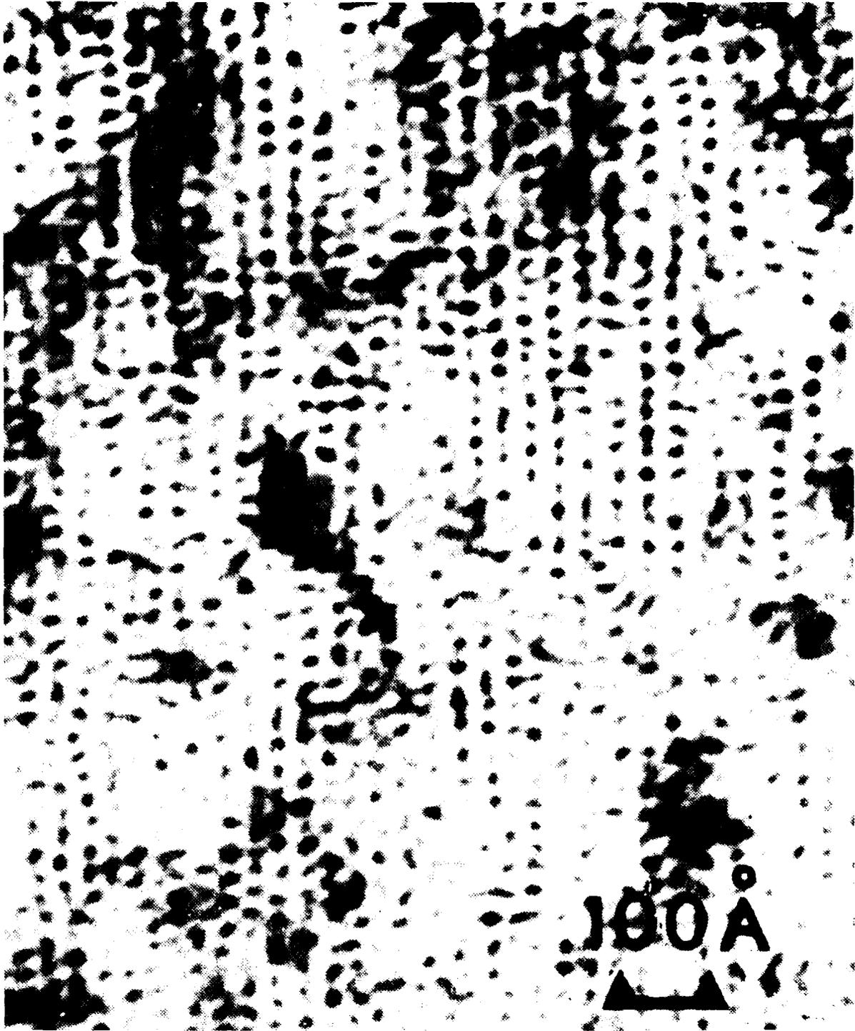
Fig.27. Electron micrograph illustrating the alignment of helium bubbles in molybdenum irradiated at  $300^{\circ}\text{C}$  with  $2.3 \times 10^{17}$  40 keV helium ions  $\text{cm}^{-2}$ . The orientation is close to (001).
