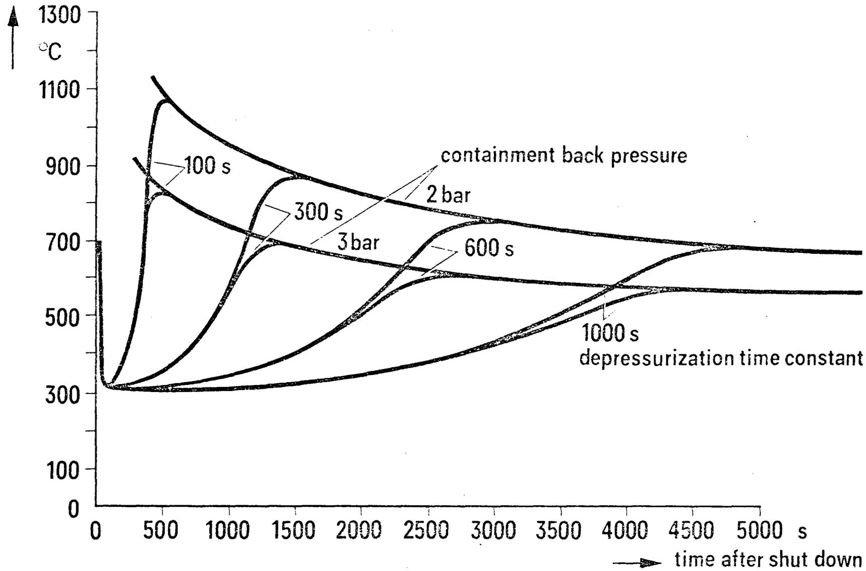
Fig.5: Peak cladding temperatures after depressurization accident (GSB-1)
