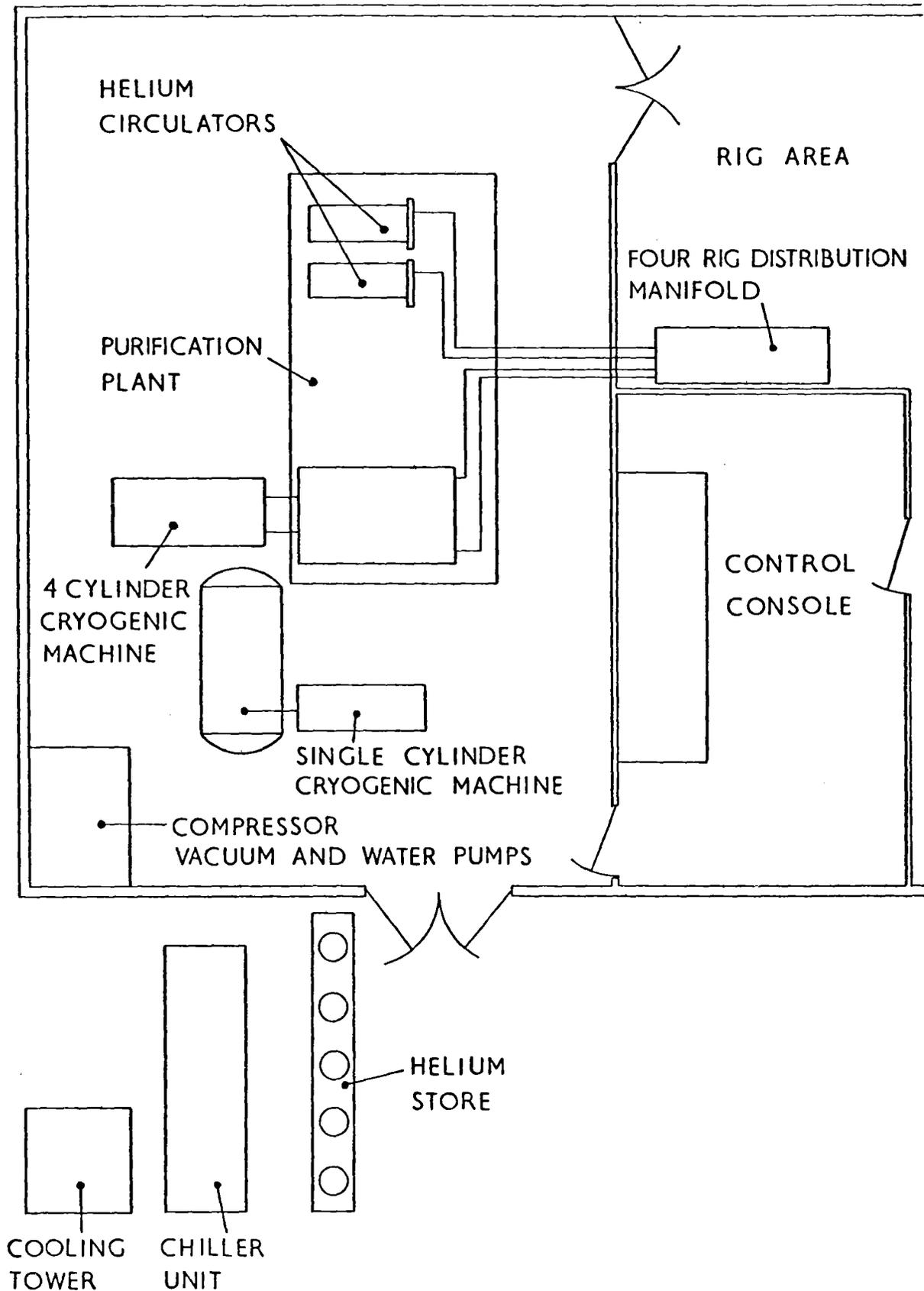
DIAGRAM OF NPC HELIUM TEST LOOP PLANT ROOM
