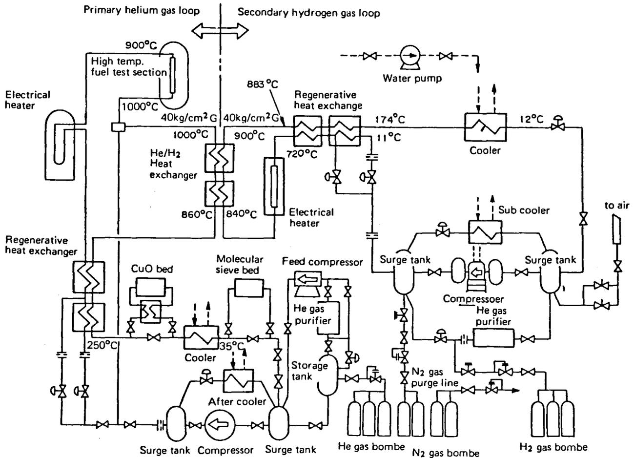
Design parameters of hydrogen gas loop
