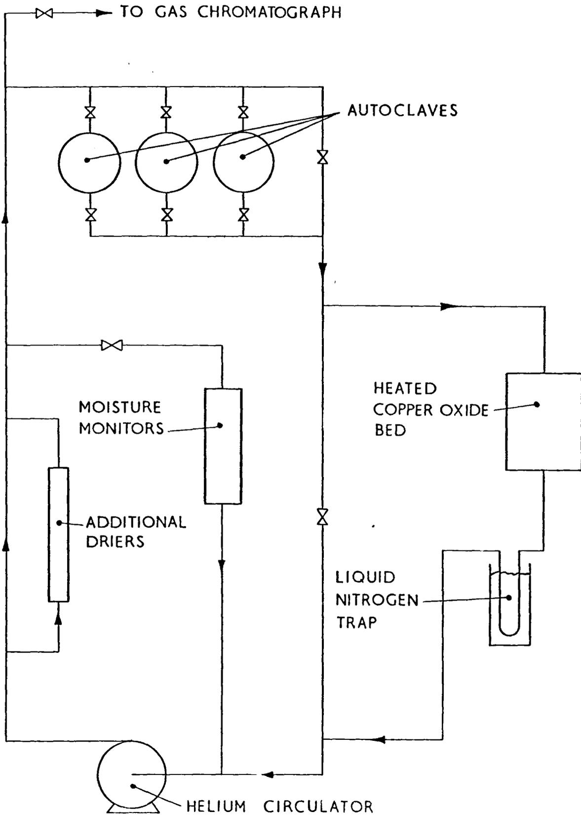
DIAGRAM OF NPC HIGH PRESSURE LOOP
