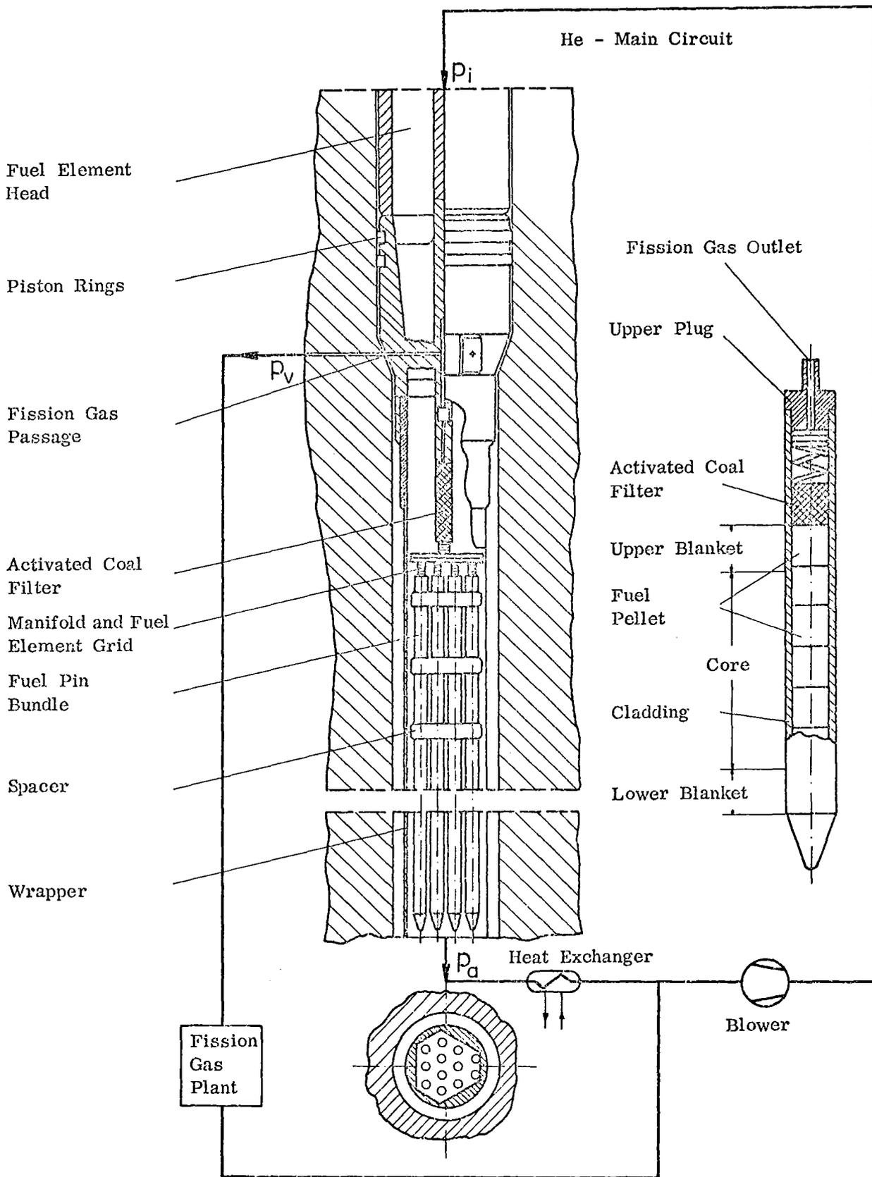
Fig.3: Test fuel element (schematic) for the BR2 irradiation experiment
