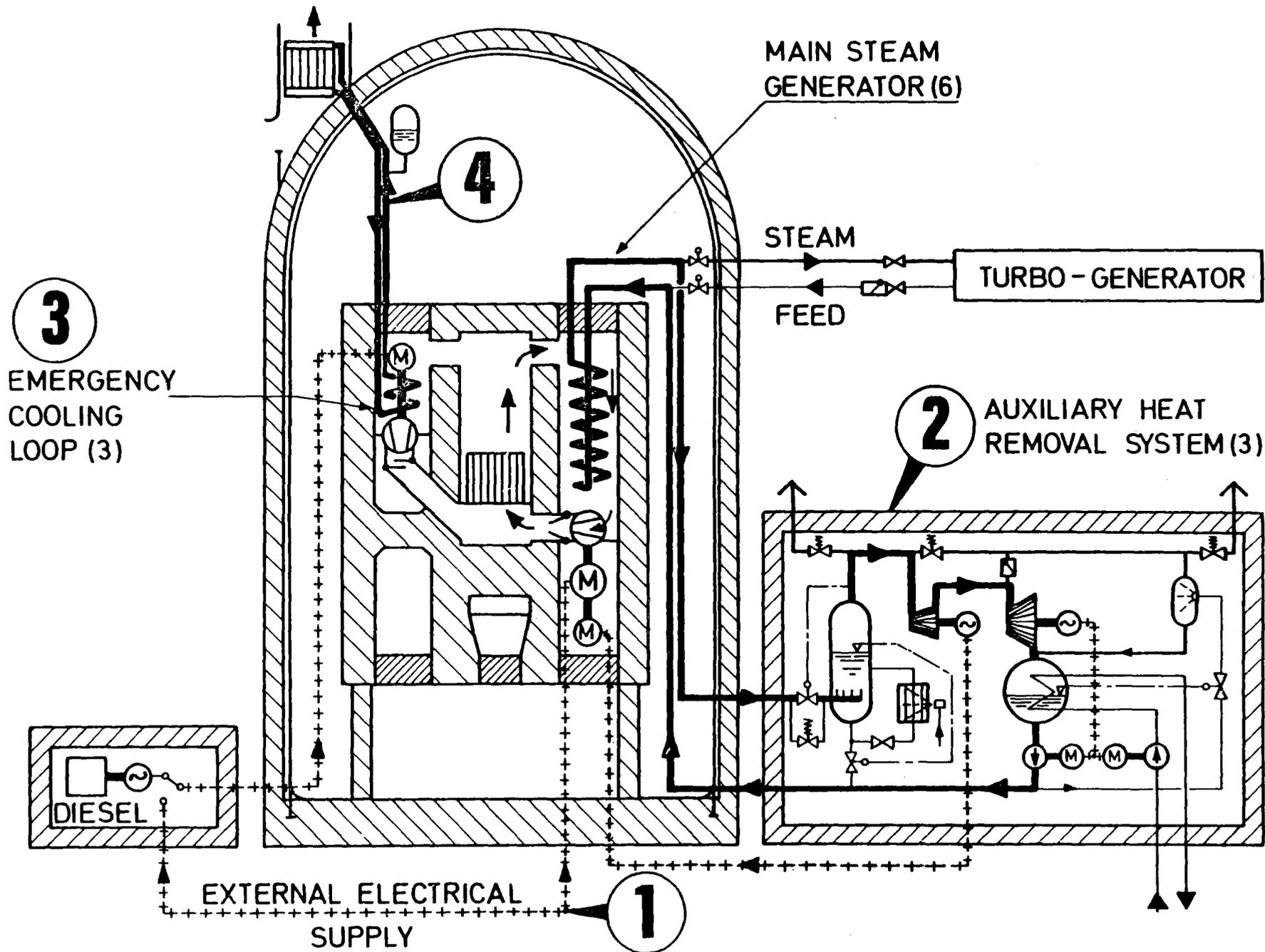
Fig. 2: GBR4 - Emergency Cooling System
