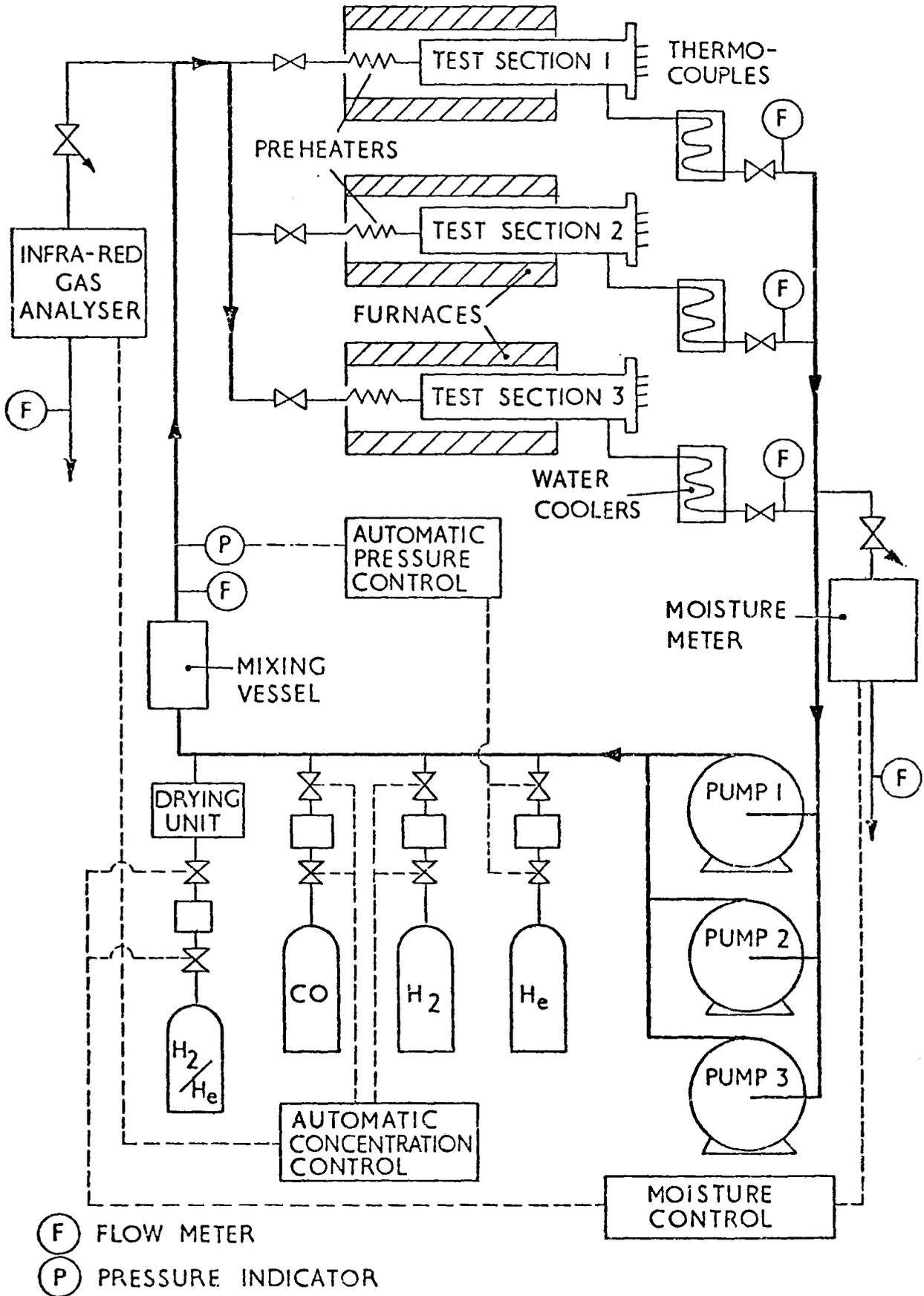
DIAGRAM OF HELIUM CORROSION TEST FACILITY (LOOP 3)
