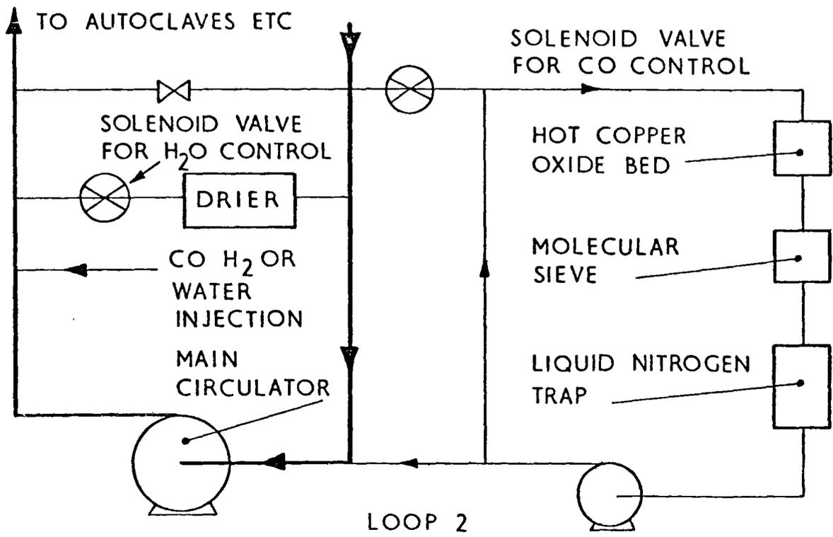
FLOW DIAGRAMS OF NPC LOW PRESSURE LOOPS
