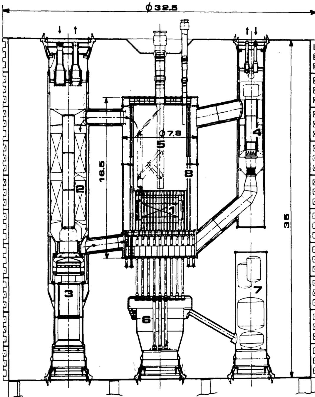
Fig.1: GBR 4 Nuclear Steam Supply System - Vertical section.
