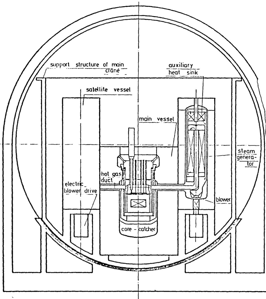
Fig. 6: General Arrangement GCFR 1200
