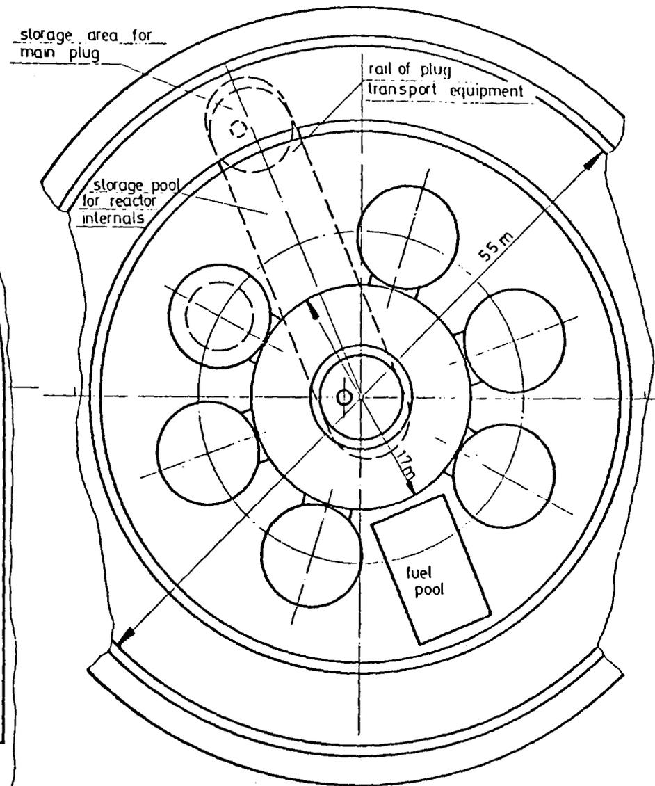
Fig. 7: PCRV General Arrangement Plan View
