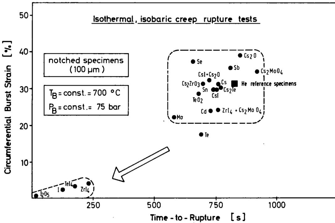
Fig.3: Effect of simulated fission products on the burst strain and time-to-failure of notched Zircaloy-4 tube specimens (100 μm deep internal notches) in isobaric creep rupture tests at 700°C in He.
