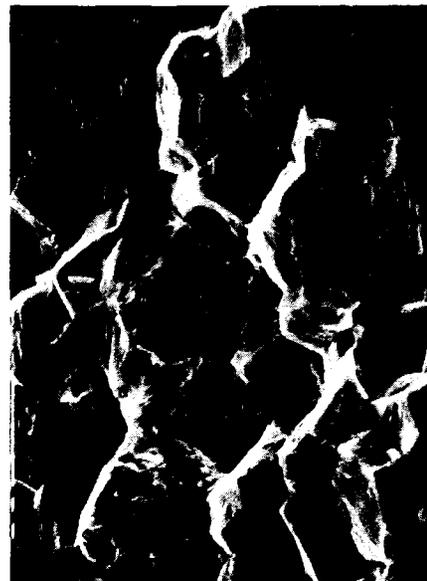
intergranular fracture surface
