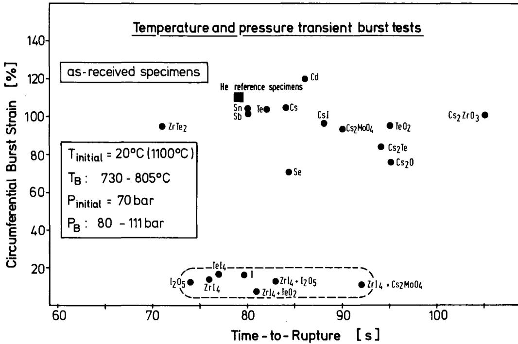
Fig.1: Effect of simulated fission products on the burst strain and time-to-failure of as-received Zircaloy-4 tubing in temperature and pressure transient burst tests in He.
