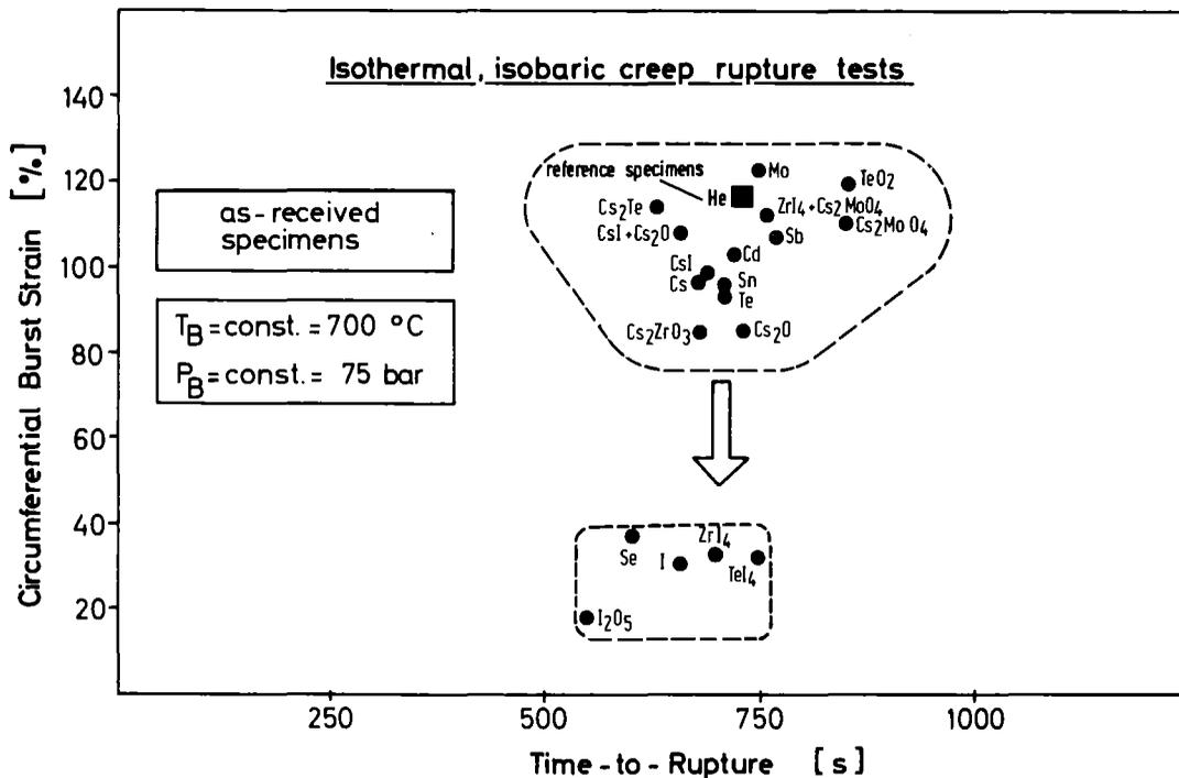
Fig.2: Effect of simulated fission products on the burst strain and time-to-failure of as-received Zircaloy-4 tubing in isobaric creep rupture tests at 700°C in He.
