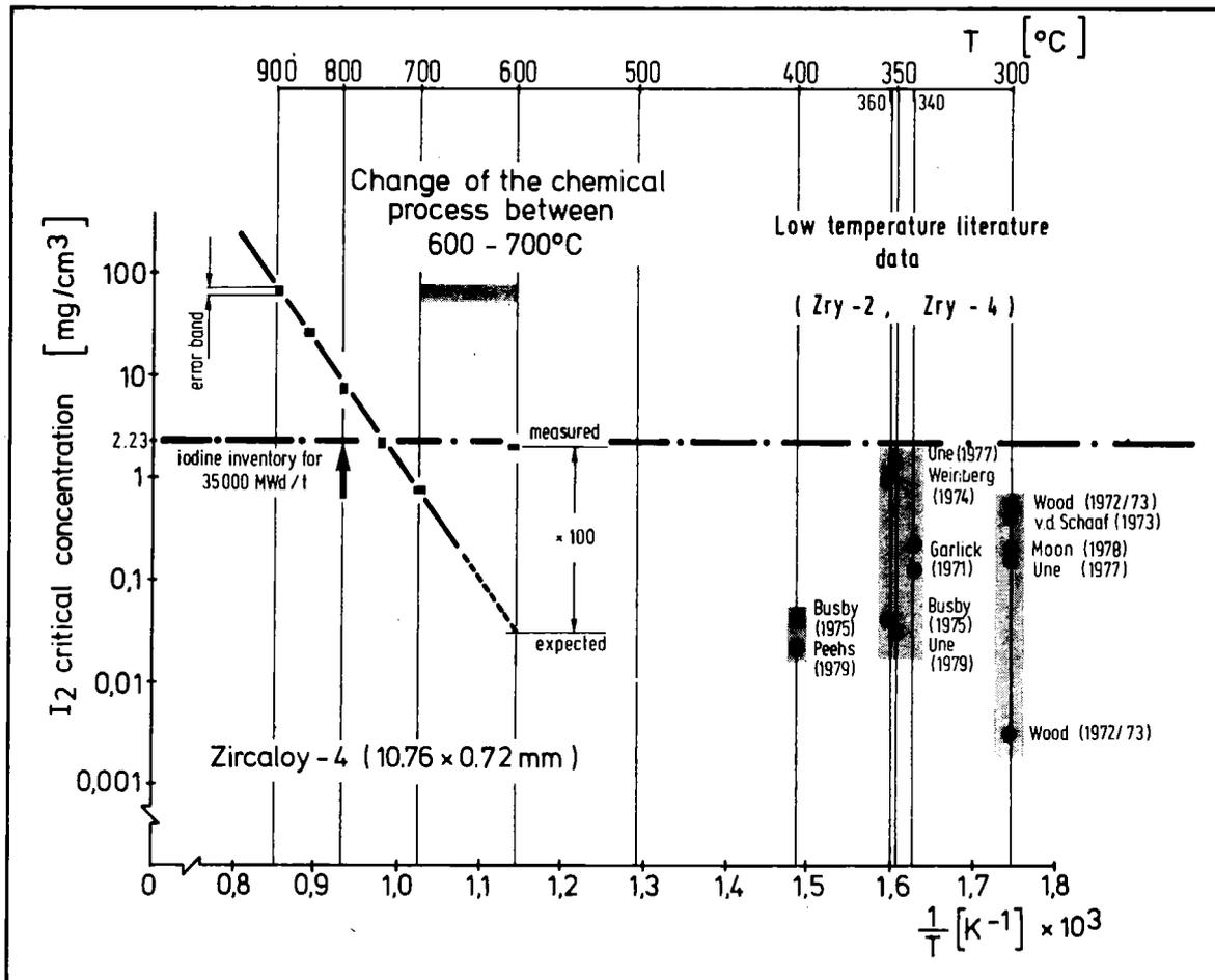
Fig.5: Critical iodine concentration which results in stress corrosion cracking of as-received Zircaloy-4 tubing as a function of temperature.
