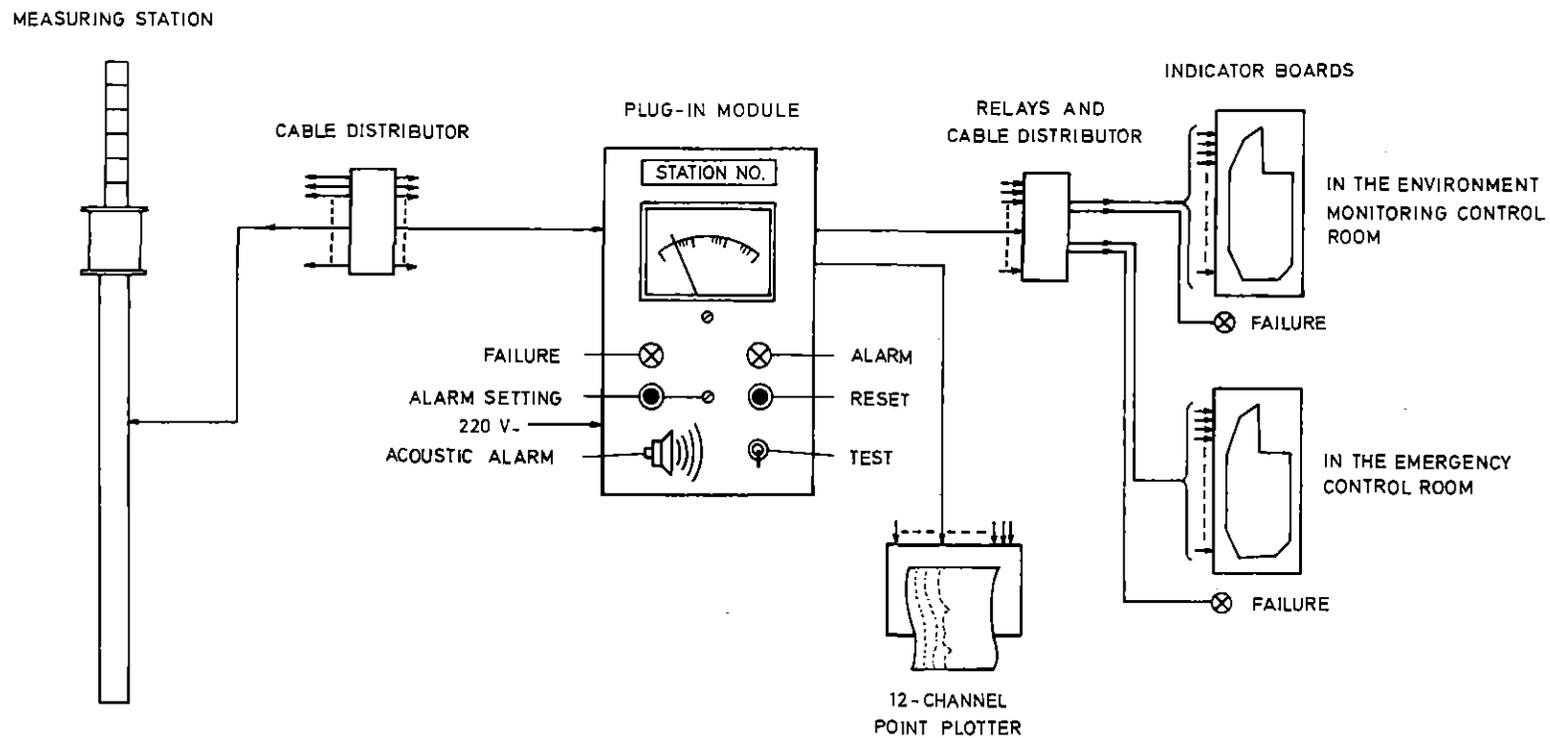
Fig. 5: Block Diagram of the GM-Counting Tube Monitoring System
