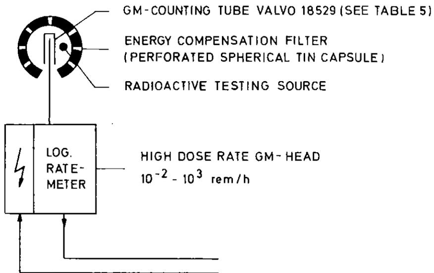
Fig. 6: Measuring stations for Low und High Dose Rates
