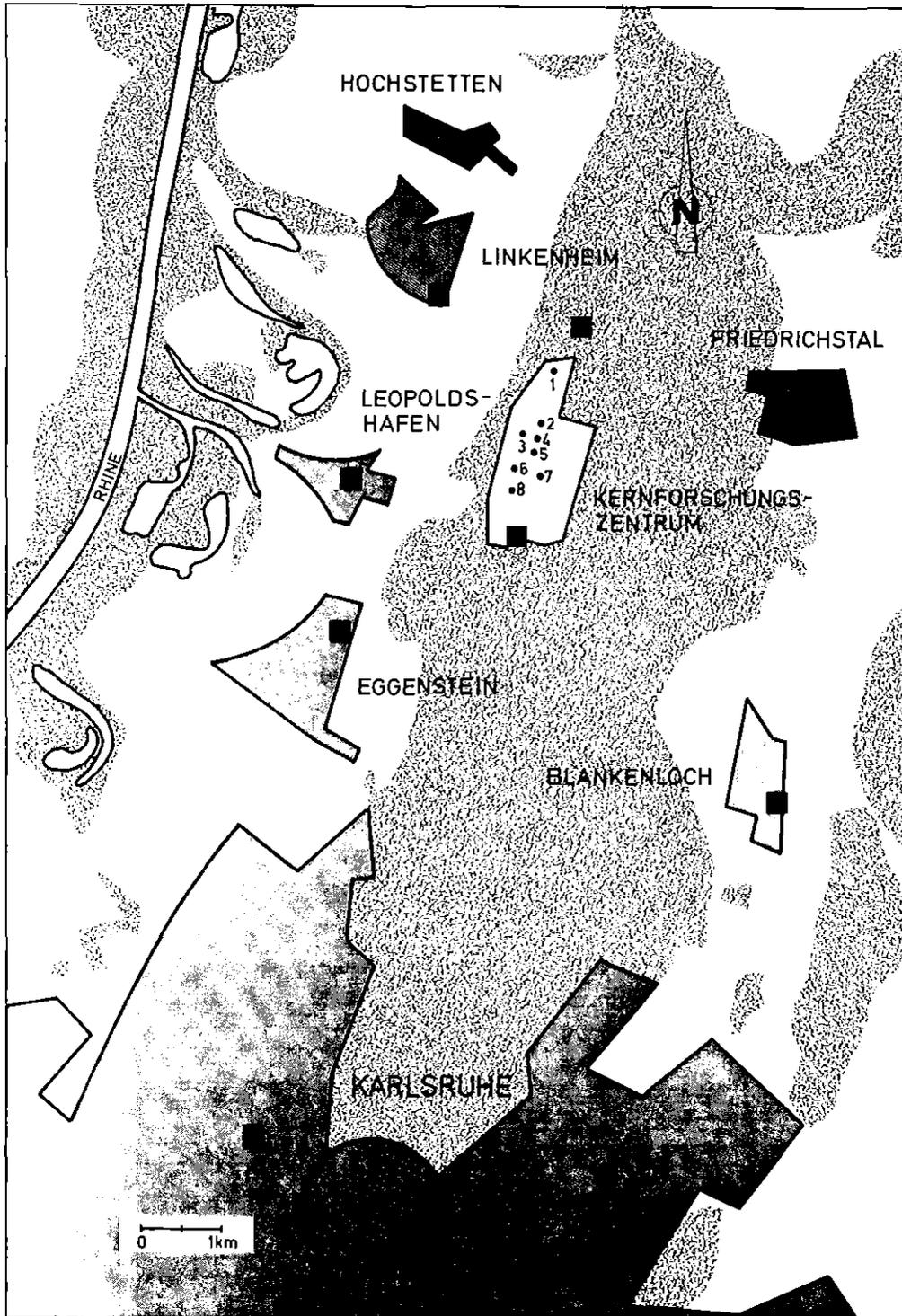
Fig. 1: Map of the measuring points for on-line environmental monitoring. The numerated points within the KfK plant area designate significant emitters of radioactive materials (1: Reprocessing Plant WAK; 2: Reactor MZFR (50 MW<sub>e1</sub>); 3: Compact sodium-cooled Reactor KNK (20 MW<sub>e1</sub>); 4: Institute for Hot Chemistry IHCh; 5: Hot Cells HZ; 6: Incineration Plant FERAB; 7: Research Reactor FR-2 (44 MW<sub>th</sub>); 8: Cyclotron)
