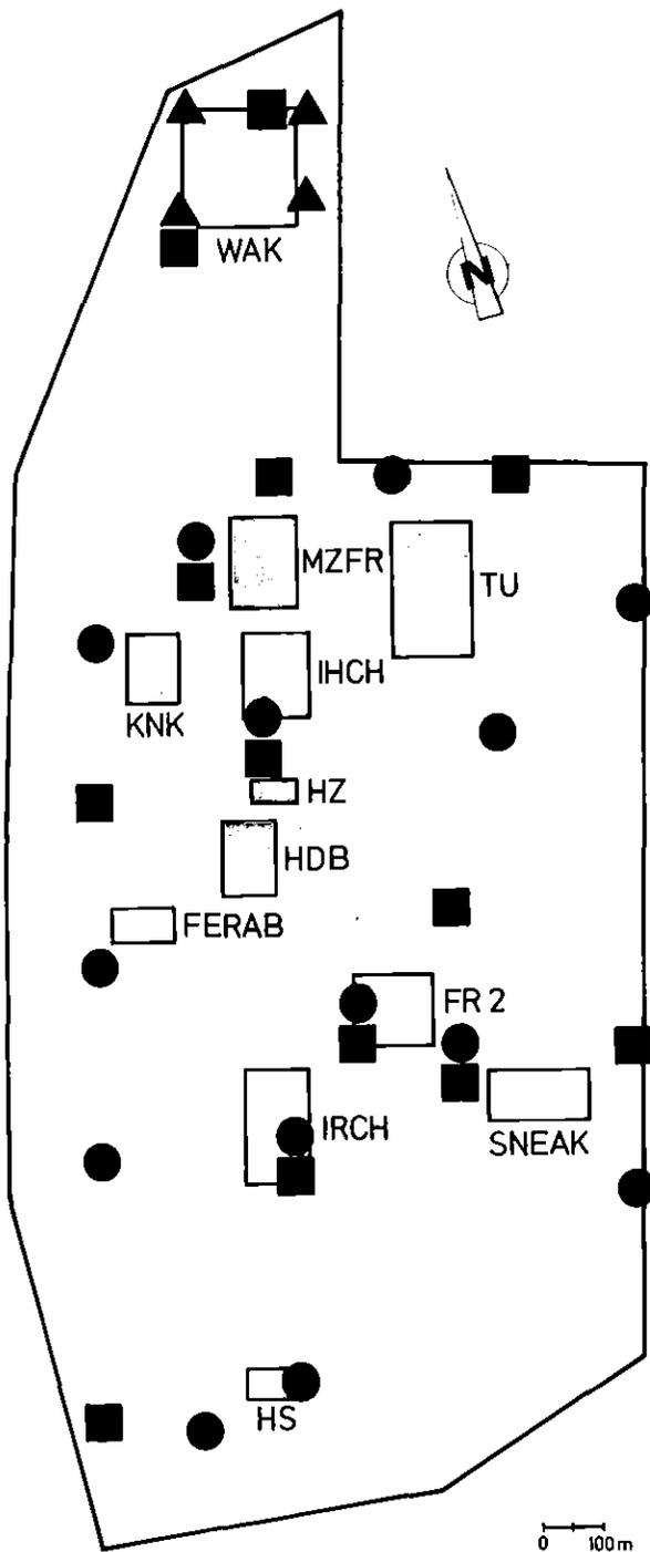
Fig. 2: Map of the measuring points of the Counter Monitor System for monitoring the KfK plant area.
