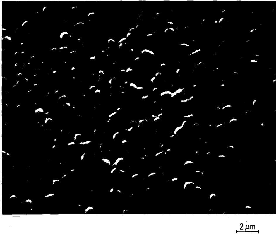
Figure 4: Nb<sub>3</sub>Sn - layer on a Nb substrate (3h, 1050°C)
