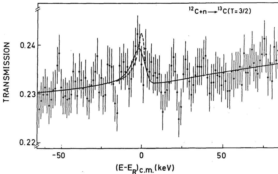
Fig. 4 Measured neutron transmission and best fit curve (solid line) for the first  $^{13}\text{C}$  ( $T=3/2$ ) resonance (preliminary)
