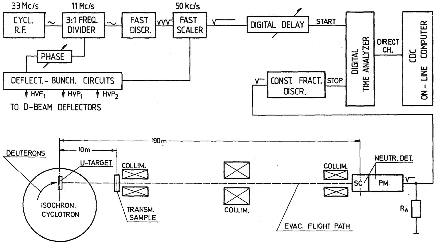
Fig. 1 Schematic diagram of the time-of-flight set-up. For clarity details of the KfK deflection-bunching system and the complete set of logic circuits are not shown
