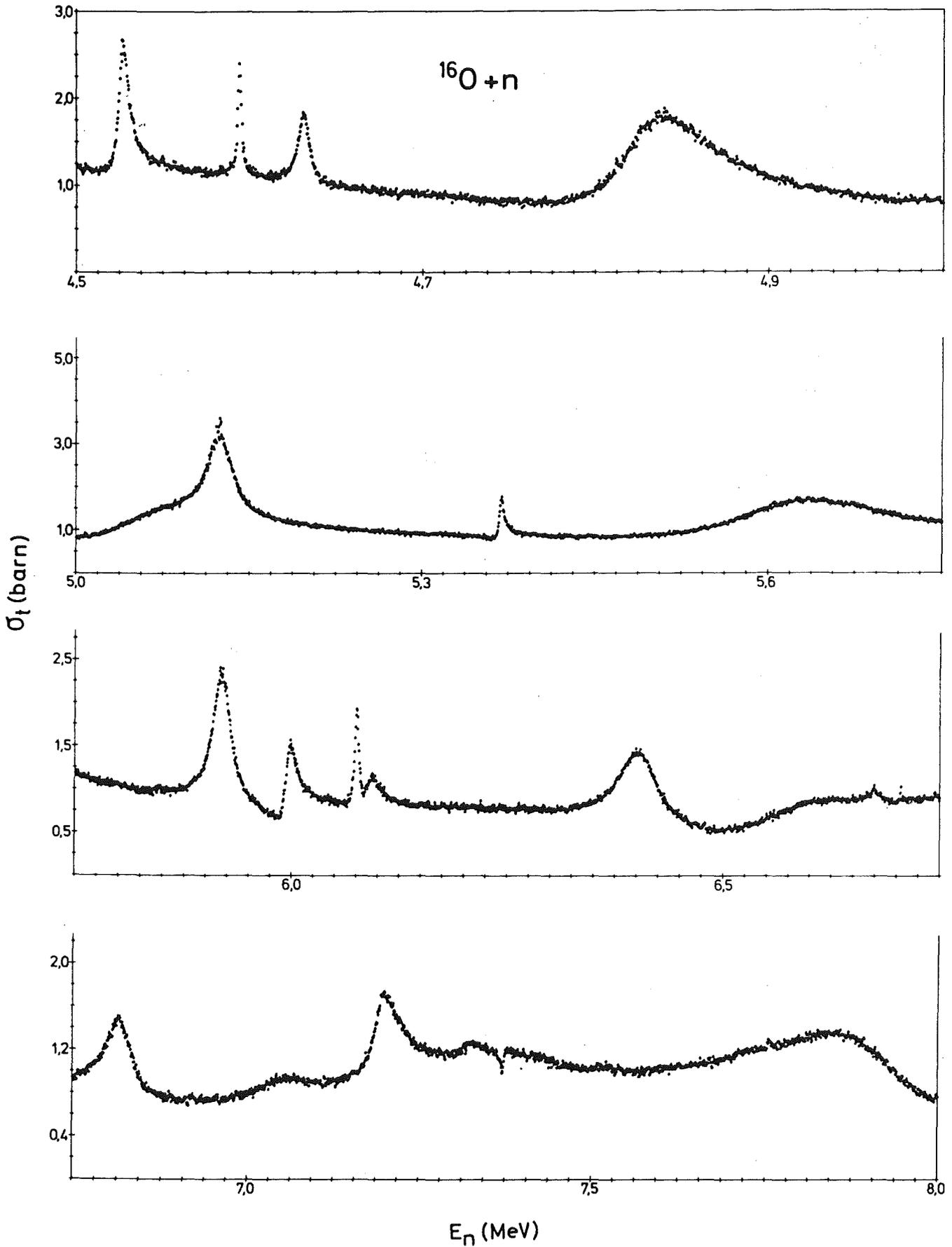
Fig. 2 Total neutron cross section between 4.5 and 8 MeV. These data are an example of the experimental results obtained for C and O between 3 and 30 MeV
