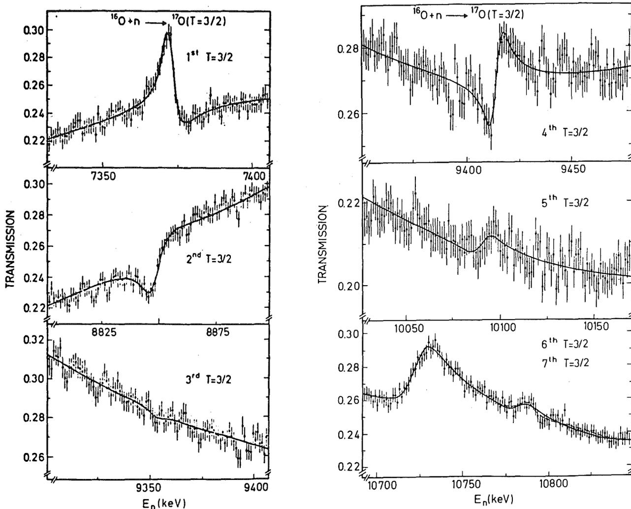
Fig. 3 Measured neutron transmission and best fit curves (solid lines) from our resonance analyses for the first seven  $^{17}\text{O}$  ( $T=3/2$ ) resonances
