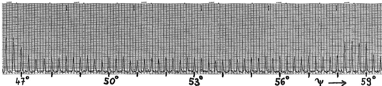
Fig. 3 Diverse  $\omega$ -scans (fixed  $\omega$ -scan range  $\Delta\Omega=1.2^\circ$ ) for different  $\psi$ -values out of the Umweganregung - free region
