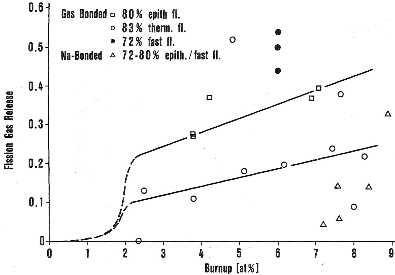
Fig. 8 Fission gas release in carbide fuel pins versus burnup
