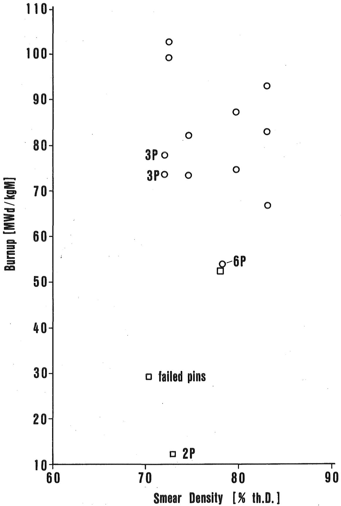
Fig. 2 Burnup of Na-bonded pins versus smear density
