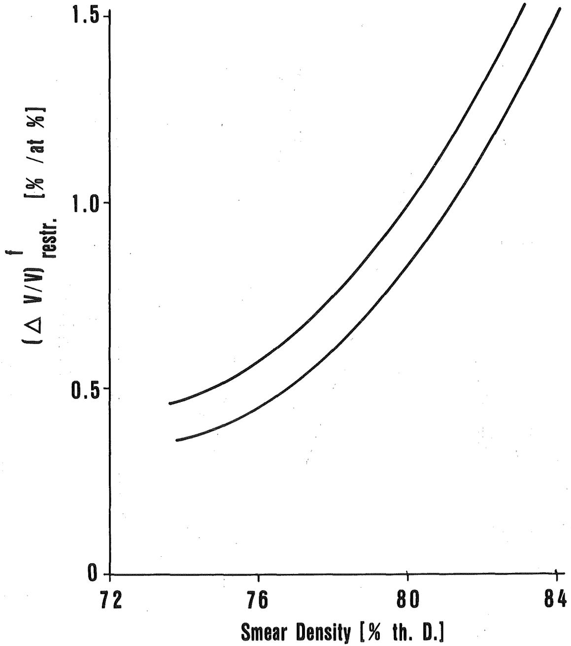
Fig. 7 Restraint carbide swelling rates versus smear density
