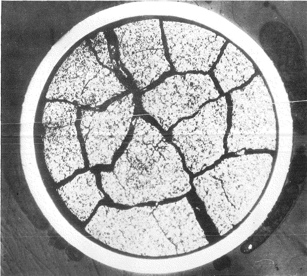
Fig. 12 Cracking pattern in a Na-bonded fuel pin
