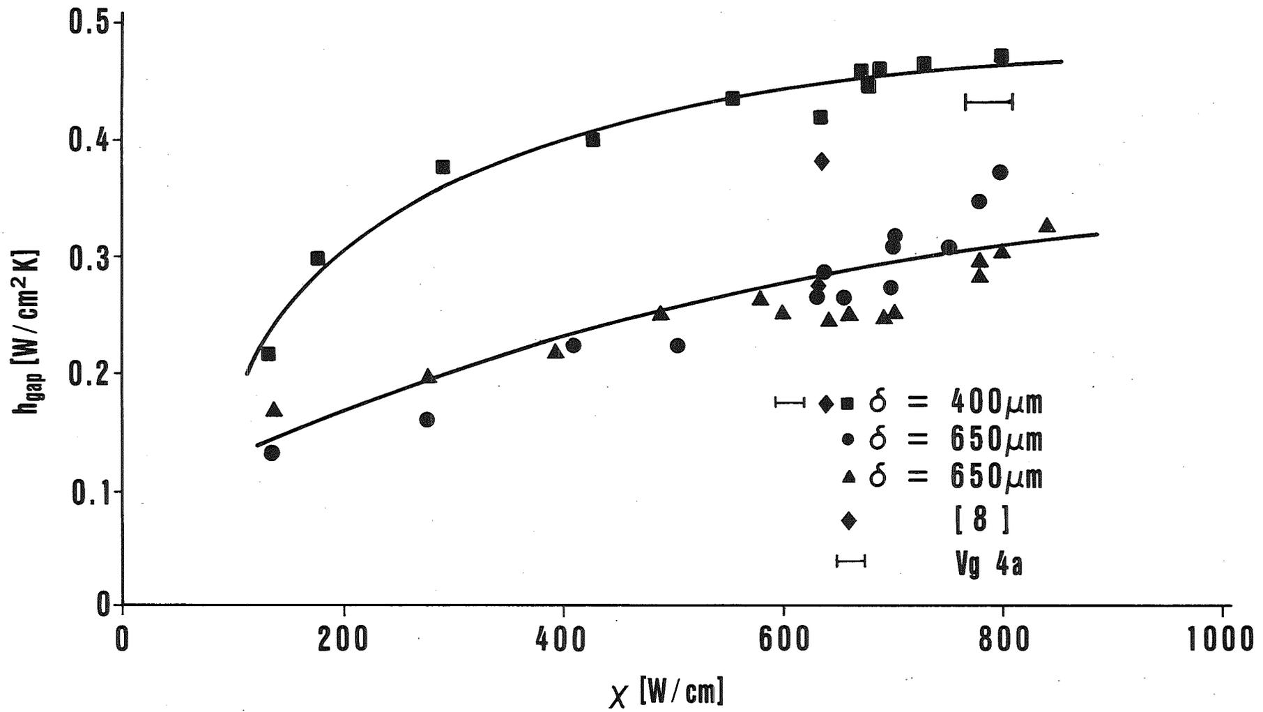
Fig. 4 Experimental heat transfer coefficients of He-bonded pins at BOL
