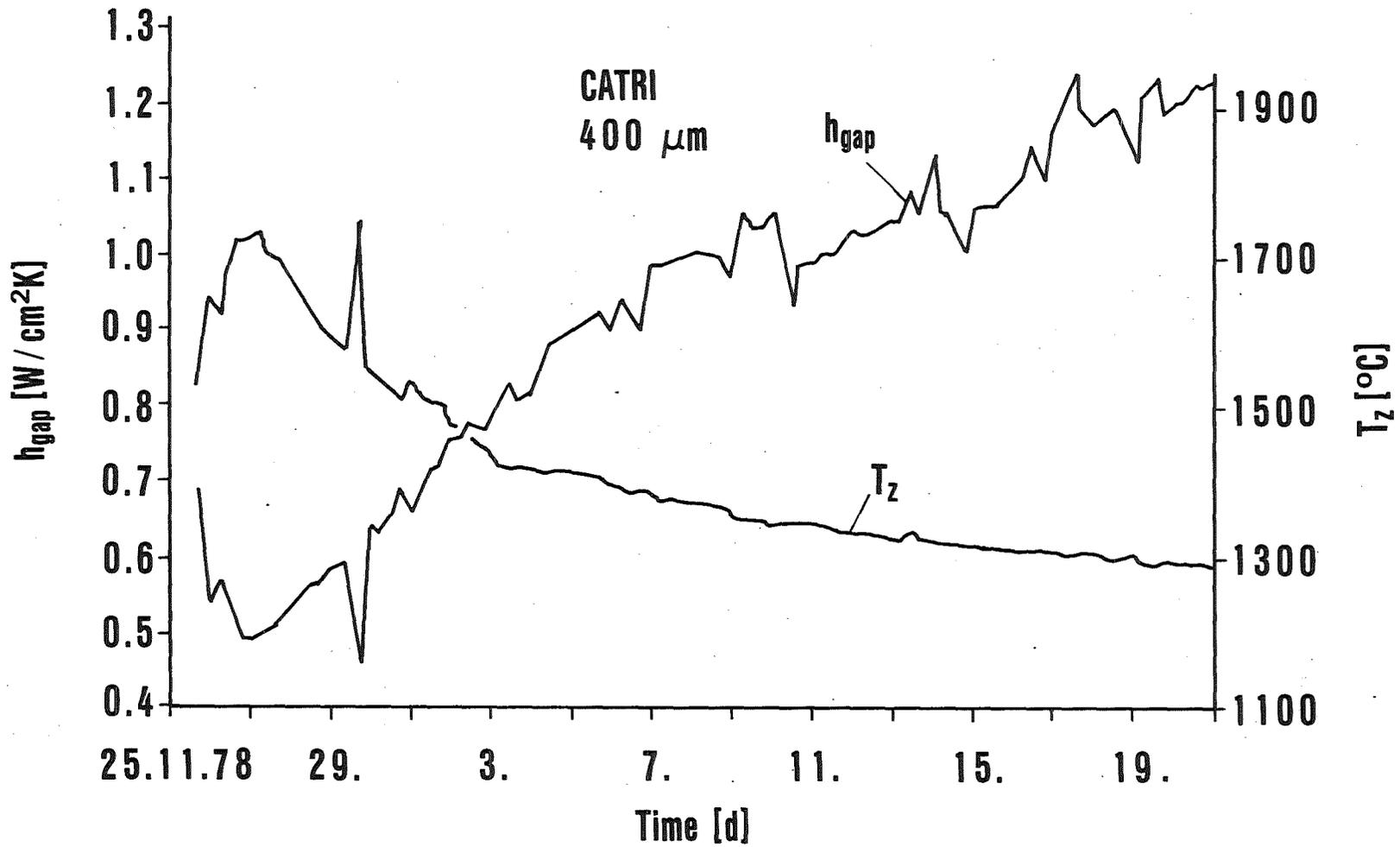
Fig. 5 Fuel centerline temperatures and gap coefficients at BOL of CATRI
