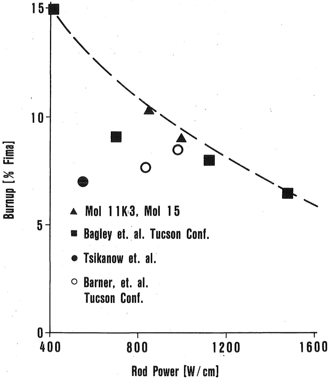
Fig. 3 Burnup of Na-bonded fuel pins versus rod power
