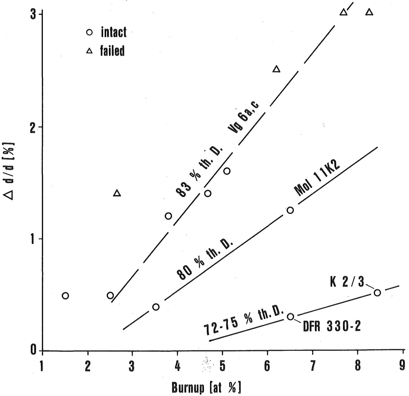
Fig. 6 Mechanical strain of gas-bonded carbide fuel pins versus burnup
