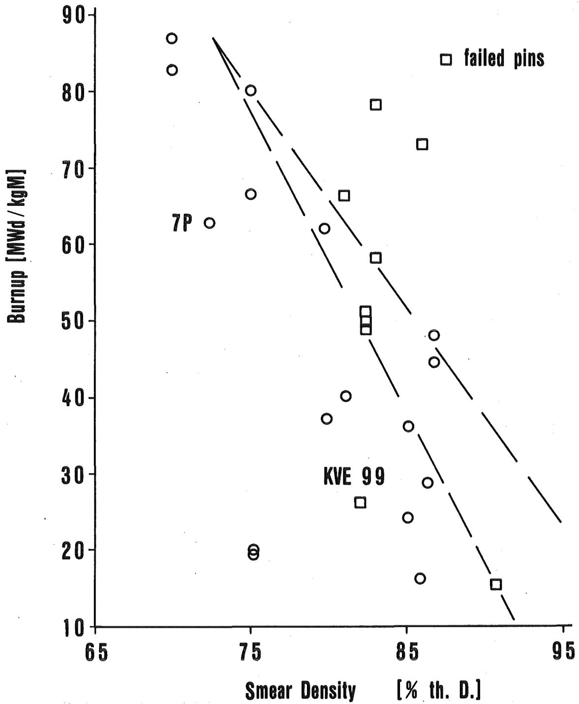
Fig. 1 Burnup of He-bonded pins versus smear density
