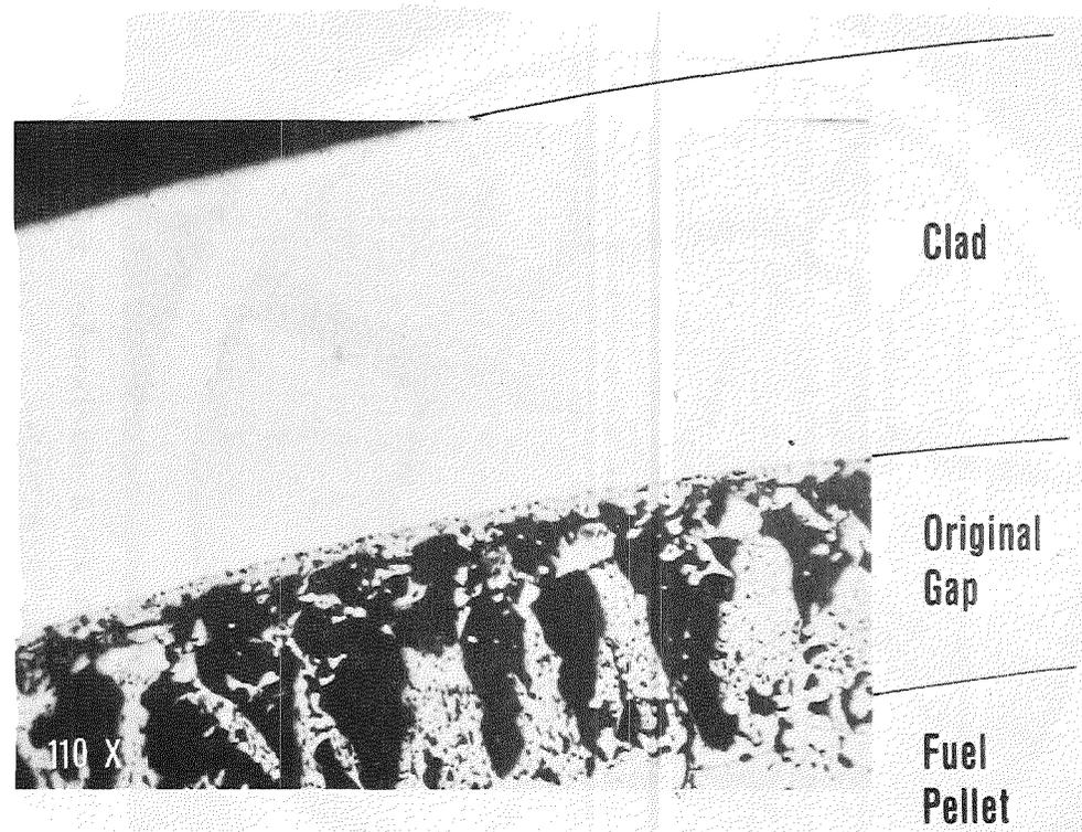
Fig. 11 Formation of a grid-like structure in a large fuel/clad gap
