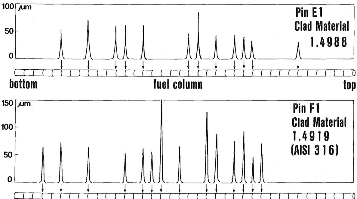
Fig. 13 Local strain peaks in Na-bonded fuel pins
