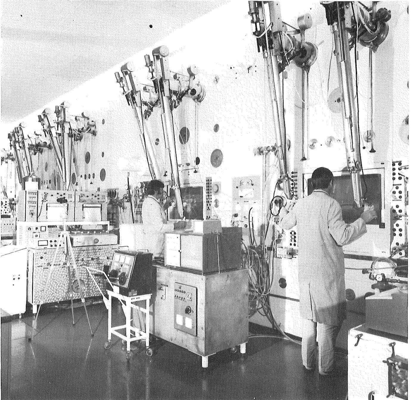
Fig. 12 Operating Area of a Hot Cell Plant, with Slave Arms of Mechanical Master-Slave Manipulators and Shielding Windows Installed in Concrete Shielding Walls
