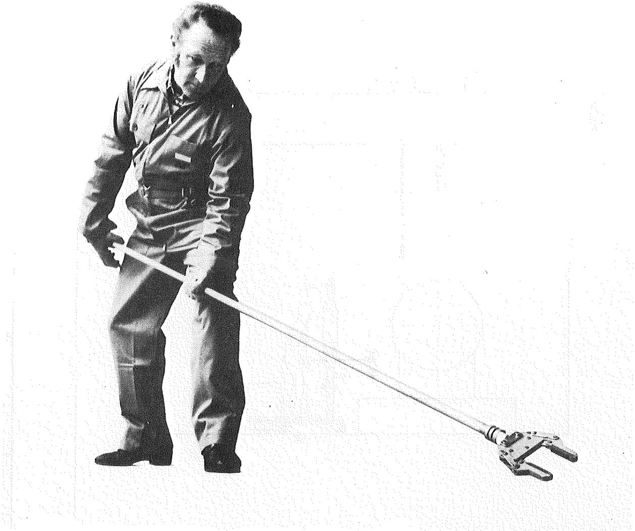
Fig. 10 Portable Remotely Handled Tong
