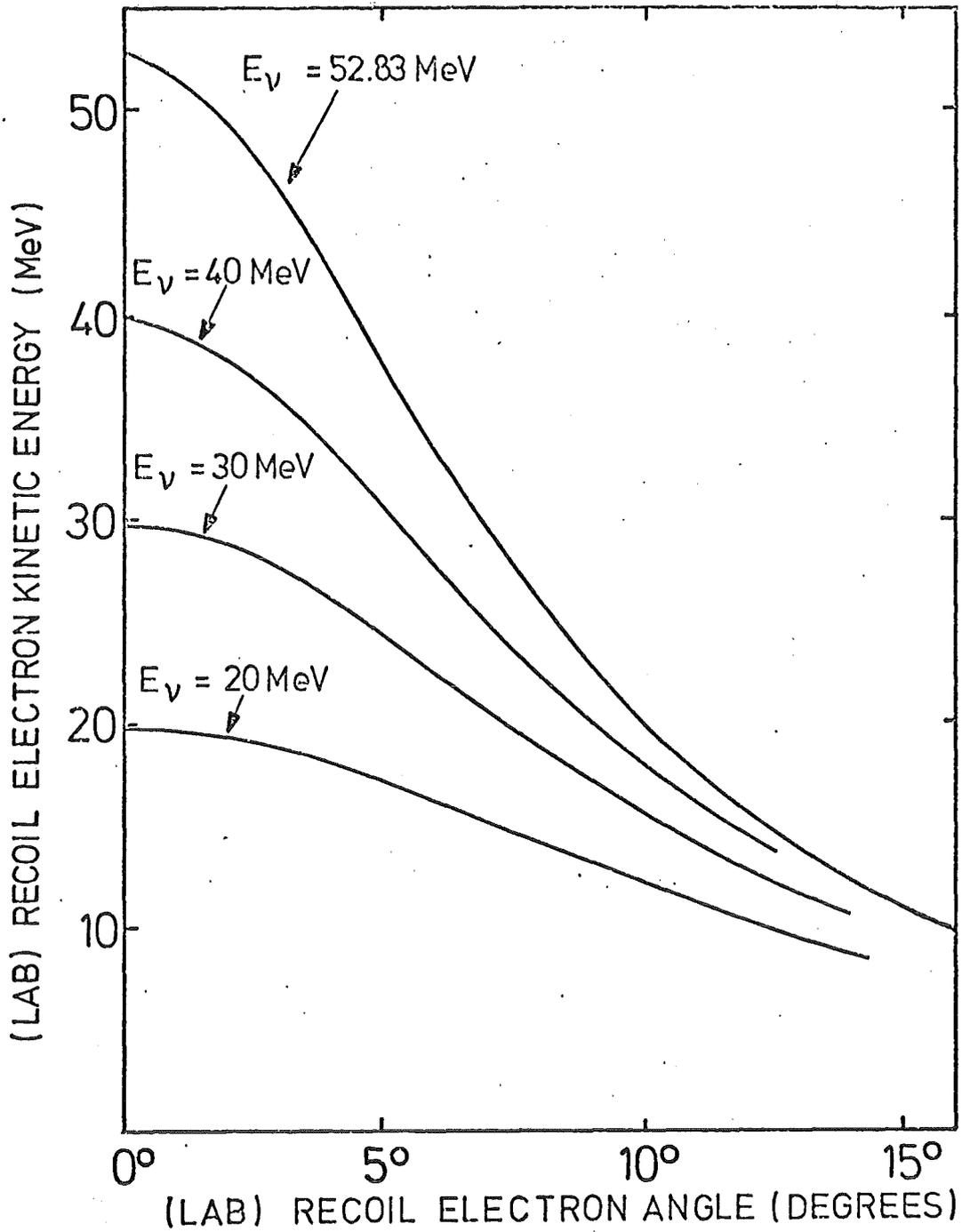
Fig. 9 : Angular dependence of the energy of the recoil electrons from  $\nu$ - $e^-$  elastic scattering for various neutrino energies
