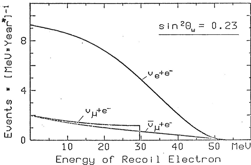
Fig.14: Energy dependent countrate for  $\nu$ -e-scattering expected in a 50 ton liquid Argon detector at 18 m distance from the  $\nu$ -source
