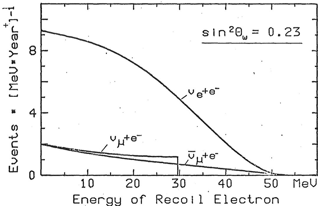
Fig.8: Energy dependent count rate for  $\nu$ - $e^-$ -scattering expected in a 50 ton liquid Argon detector at 18 m distance from the  $\nu$ -source.
