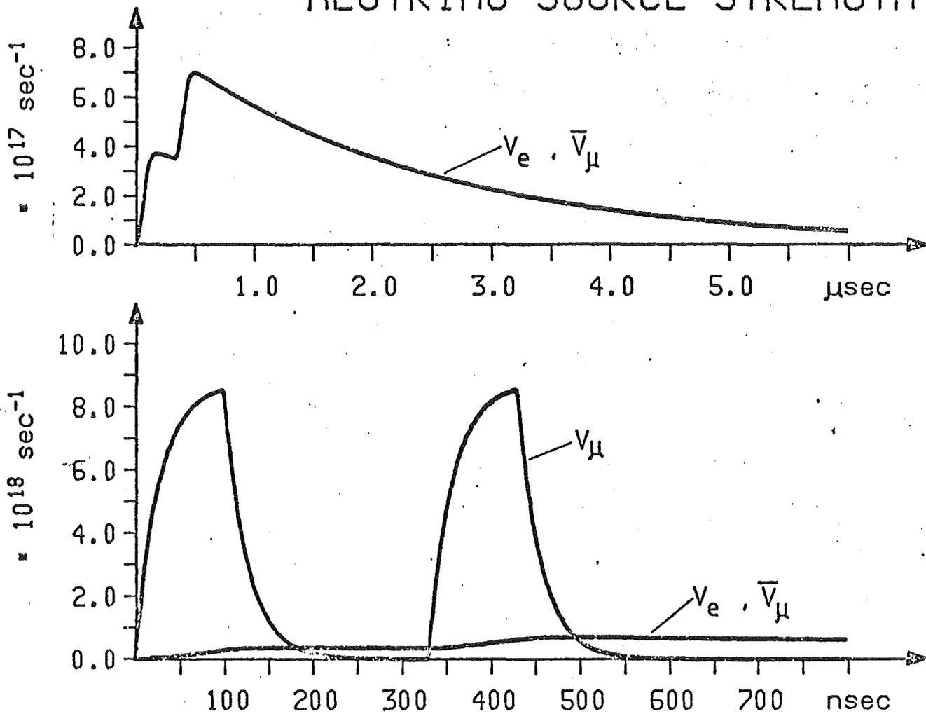
Fig. 4: Time dependence of the neutrino source strengths at the SNS spallation neutron source ( $t_p = 100 \text{ nsec}$ ;  $\Delta t_p = 330 \text{ nsec}$ ;  $\bar{I}_p = 200 \mu\text{A}$ ;  $f = 50 \text{ Hz}$ )
