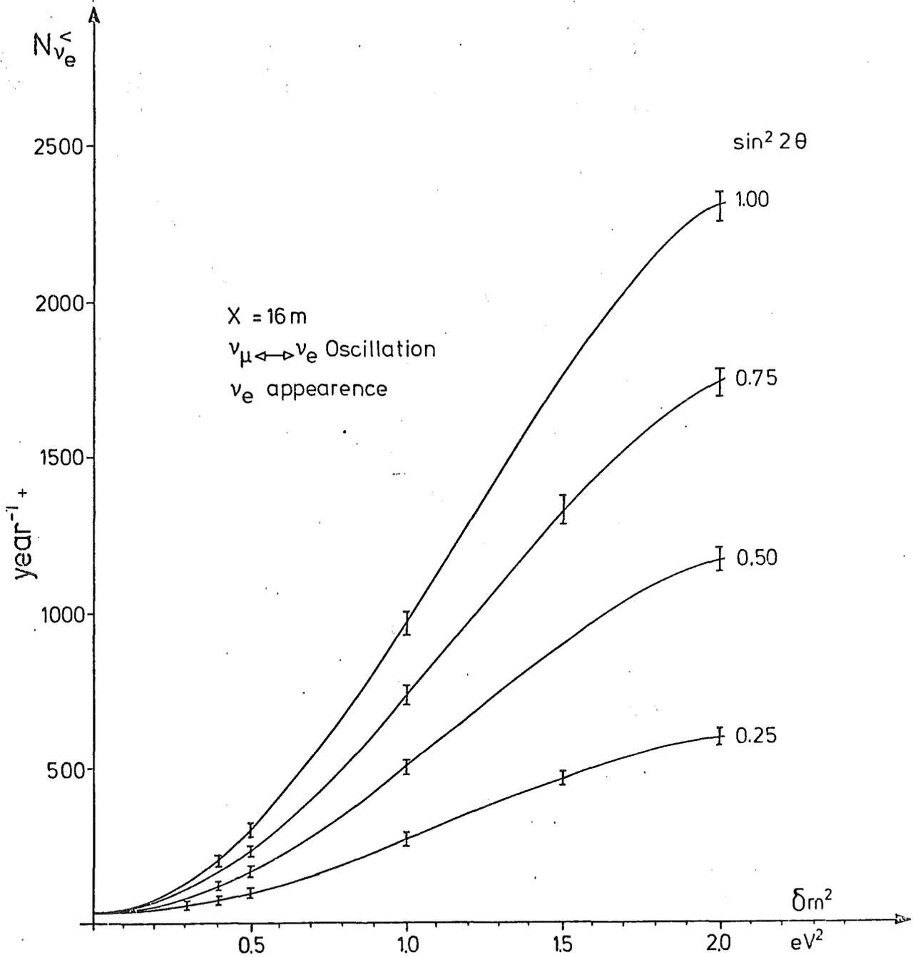
Fig.10: Expected counting rates from electron neutrinos during beam on time
