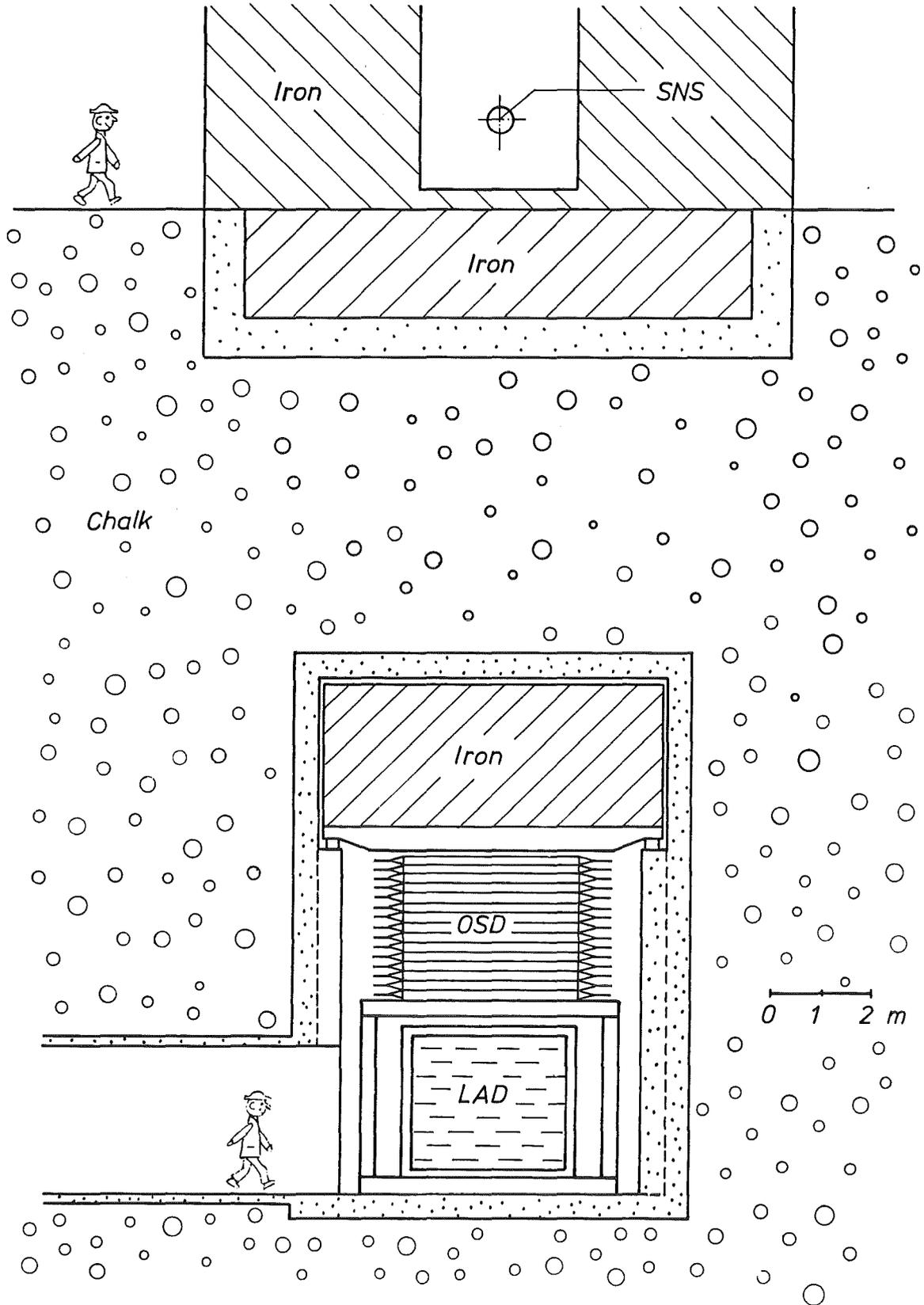
Fig.7: Schematic view of the proposed neutrino cave in the chalk below the Spallation Neutron Source SNS.(see also fig. 7a)
