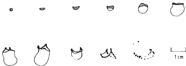
FIG. 12.6 Breakup of a water drop in an air stream moving downwards relative to a particle. traced from photographs by Lane (L6).
