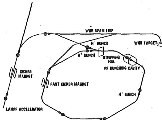
Fig. 8: Schematic drawing of the Proton Storage Ring (PSR), a planned extension to the WNR facility [19]. In the short pulse mode of operation 1 ns pulses with  $7.2 \times 10^{13}$  protons/second will be produced at repetition rates of up to 720 Hz.
