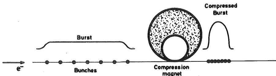
Fig. 7: Principle of a pulse compression system studied for use with the GELINA fast neutron source. The  $360^\circ$  bending magnet is expected to provide bunching after acceleration with a pulse compression factor of three [25].
