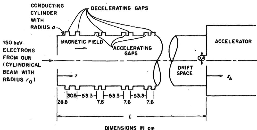
Fig. 6: Schematic diagram of the ORELA prebuncher used in a study for short pulse compression. The ultimate goal is to compress a 15 ns long pulse into a 3 ns pulse with essentially no loss in beam power [24].
