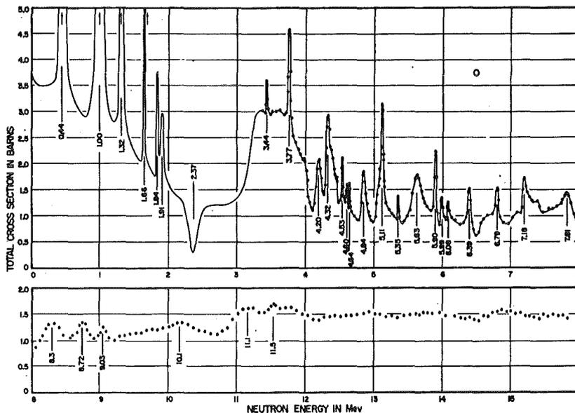
Fig. 2: The total neutron cross section of oxygen from Ref. 7. The neutron energy spread is about 20 keV up to 7 MeV and above this energy about 45 keV.
