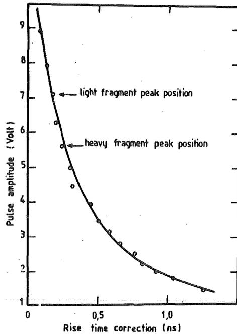
Fig. 10: Example of the time shift occurring on the discriminator pulse as a function of the pulse height for a 6 cm<sup>2</sup> silicon surface barrier fission detector [40].
