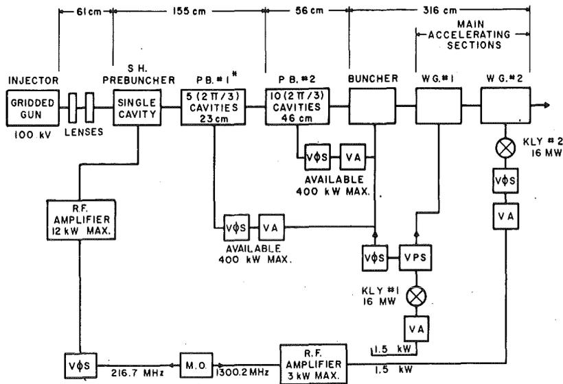
Fig. 9: Dimensional layout of the ANL electron linac. To achieve 30 ps beam bunches a subharmonic (SH) prebuncher was added with the original components being axially repositioned.
