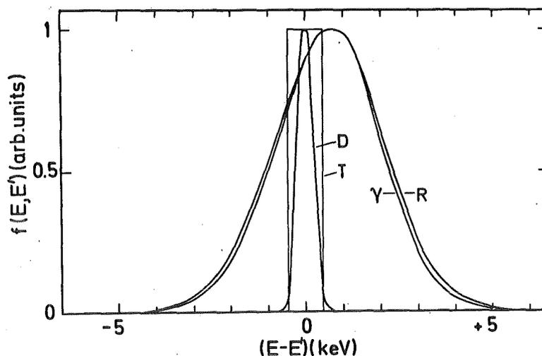
Fig. 3: Total effective energy resolution function at  $E_n = 7.4$  MeV for the KfK high-resolution transmission measurement on 0 [6].  $\gamma$  is the combined contribution from neutron pulse duration and detector response. D represents the Doppler broadening contribution and T the combined source and detector thickness contribution. The slight displacement between the two sets of curves reflects the difference between centroid and adopted nominal reference channel.
