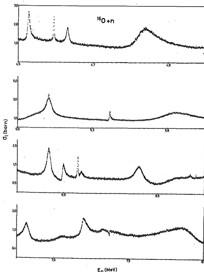
Fig. 5: Total neutron cross section of oxygen measured at the KfK cyclotron with a spectrometer resolution of 0.005 ns/m [6]. High resolution data were measured over the extended energy range from 3 to 30 MeV.
