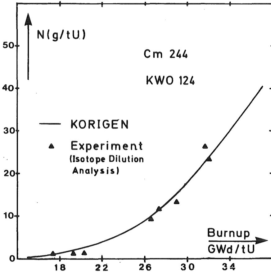
Fig. 10  $^{244}\text{Cm}$  concentration in the spent fuel of KWO
