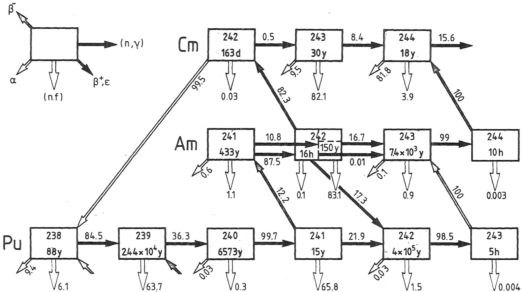
Fig.2 ISOTOPE PRODUCTION IN A THERMAL REACTOR ( $\phi_{th} = 10^{13} \text{ n/cm}^2 \cdot \text{sec}$ )
