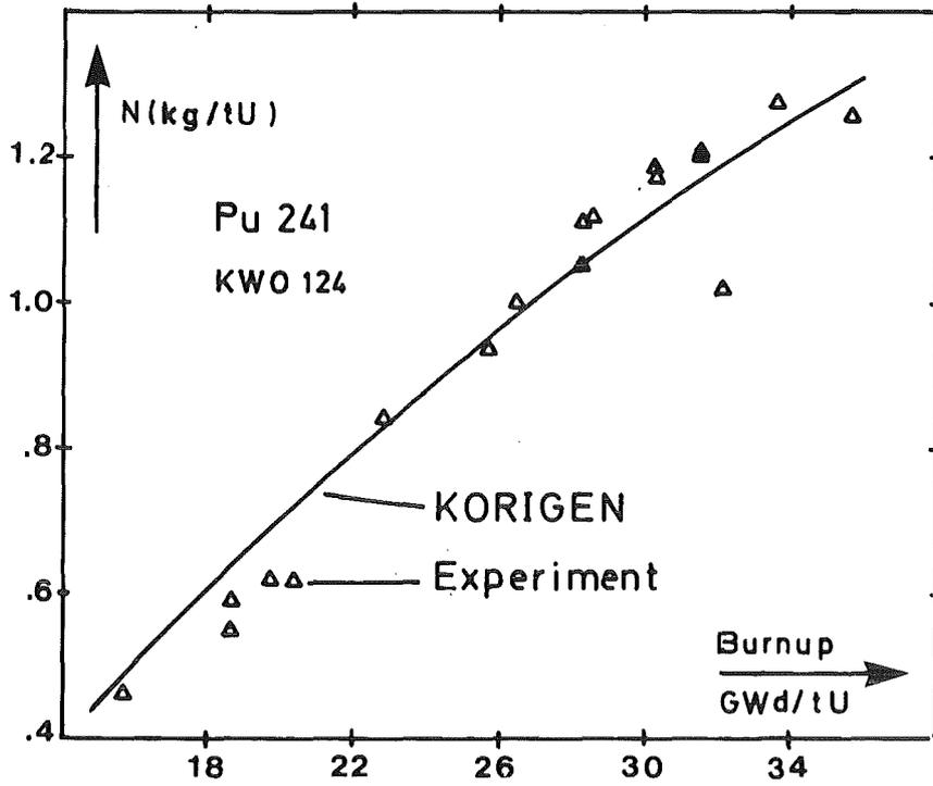
Fig. 5  $^{241}\text{Pu}$  concentration in the spent fuel of the PW reactor KWO
