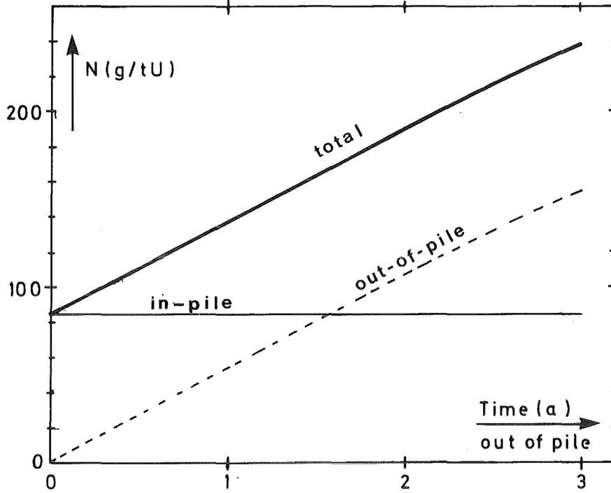
Fig. 7 Out of pile accumulation of  $^{241}\text{Am}$  in spent fuel
