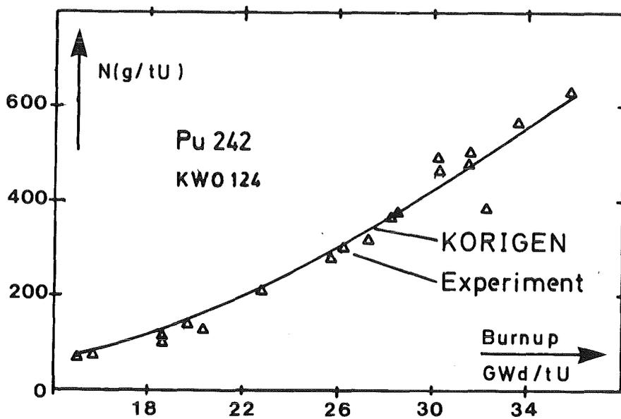
Fig. 6  $^{242}\text{Pu}$  concentration in the spent fuel of the PW reactor KWO
