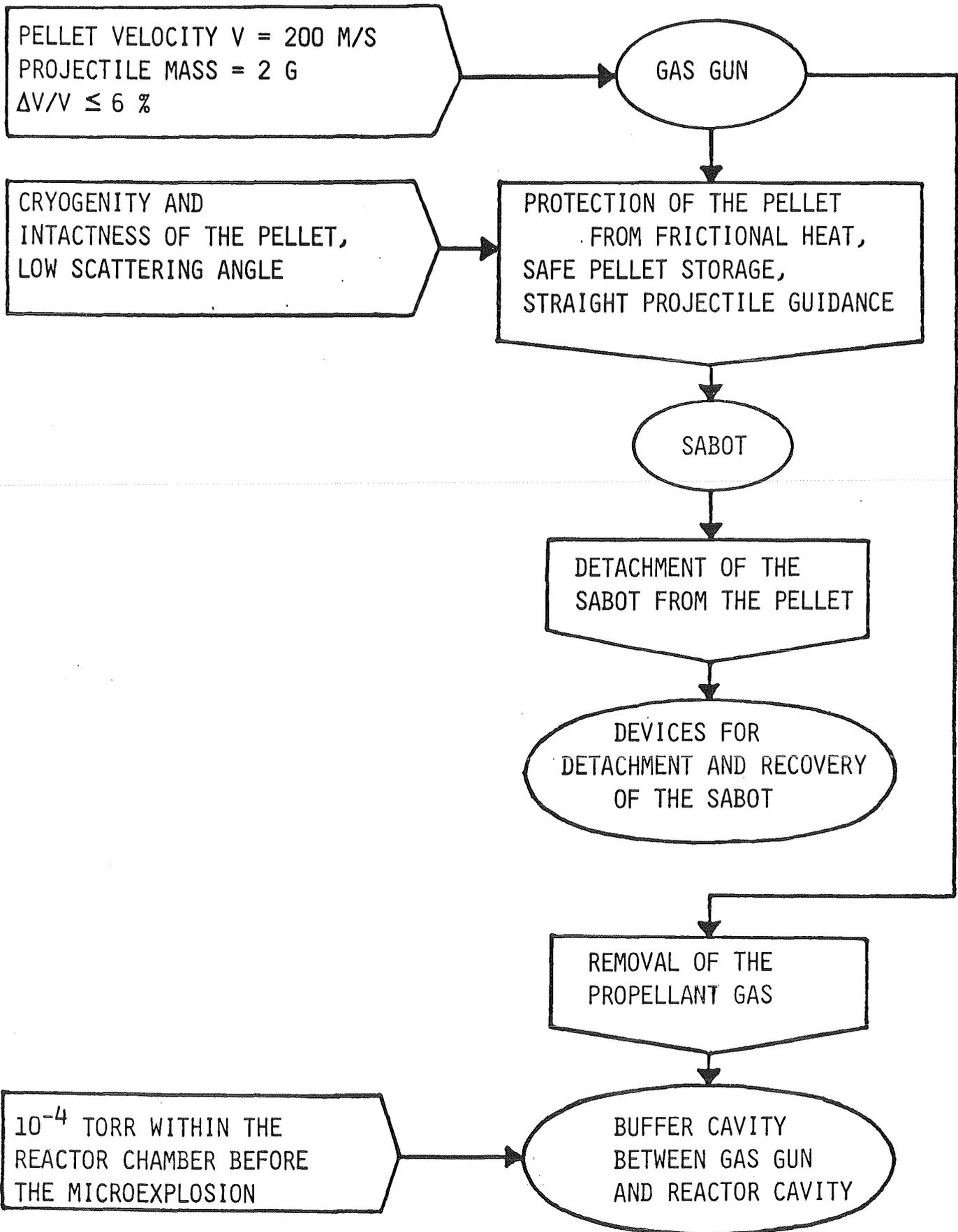
Fig. 5: Basic Requirements , System Components and Technical Tasks for a pneumatic pellet injection system for HIBALL / 1 /.
