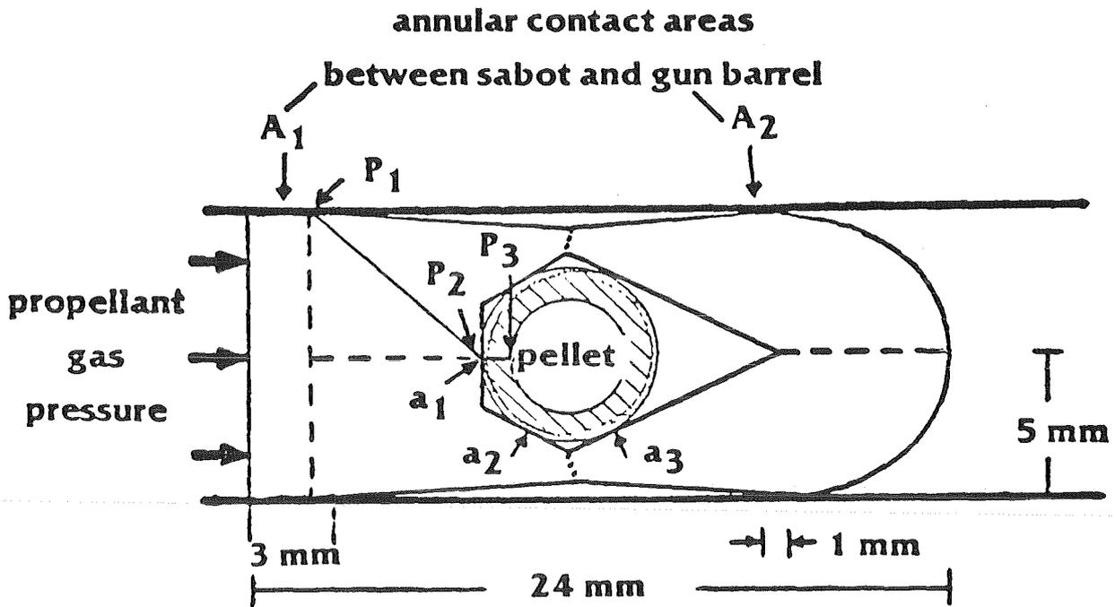
Fig. 1: Reference design of the sabot for a pneumatic pellet injection system for HIBALL; ... and ---: alternative possibilities of sabot division.
