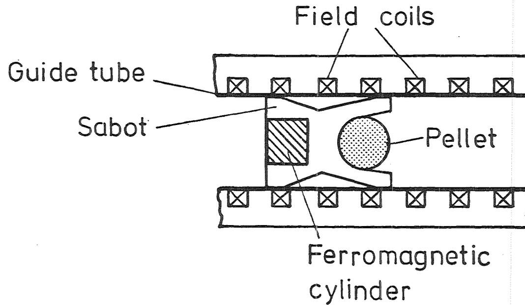
Fig. 6: Scheme of a magnetic linear accelerator for pellet injection into inertial confinement fusion reactor chambers.
