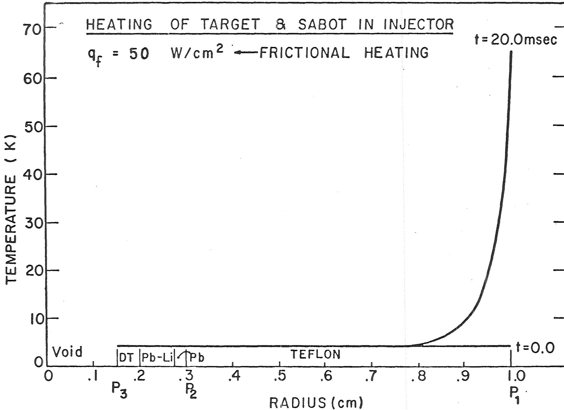
Fig. 2: Temperature distribution for pellet and sabot along  $\overline{P_1 P_2 P_3}$  (see Fig. 1) from frictional heating during acceleration / 6 /.
