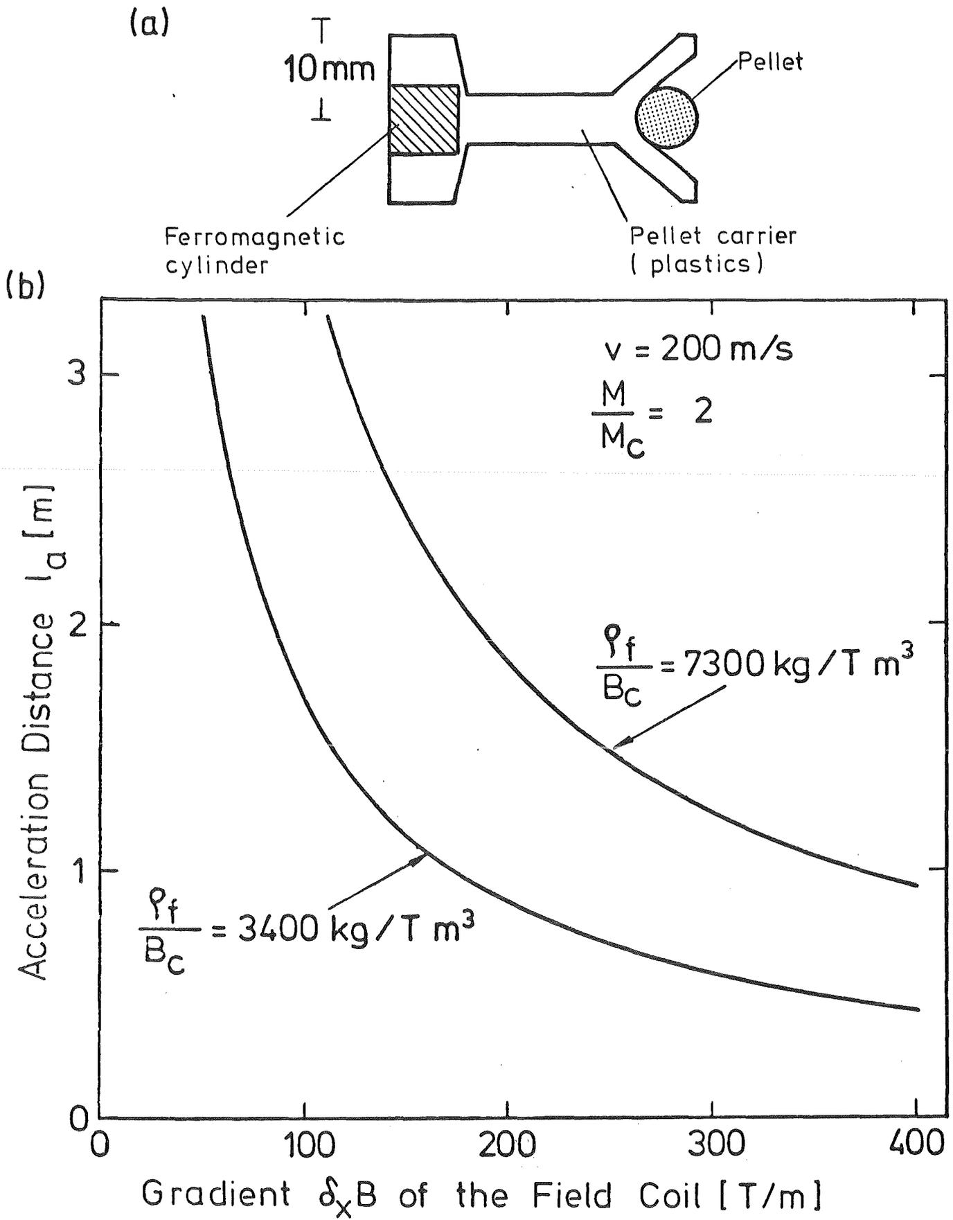
Fig. 7: Pellet acceleration by a magnetic linear accelerator:
