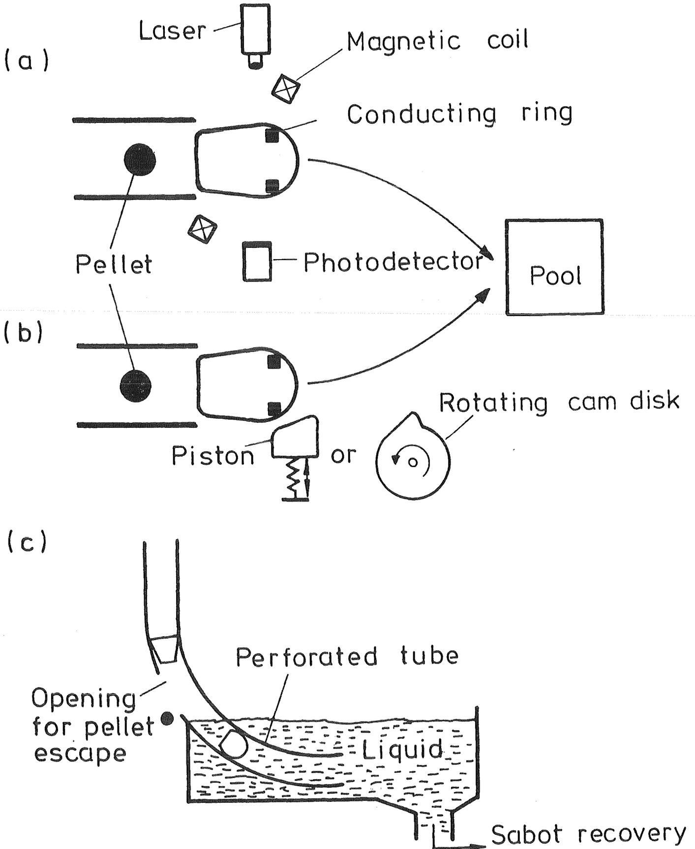
Fig. 4: Concepts for the deflection and the recovery of the sabot (not to scale), (a) Electromagnetically, (b, c) Mechanically
