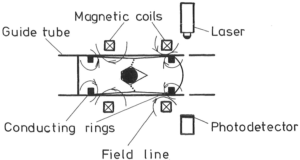
Fig. 3: Concept of detachment of the sabot from the pellet for a transversal division of the sabot; ... boundary of the sabot parts.
