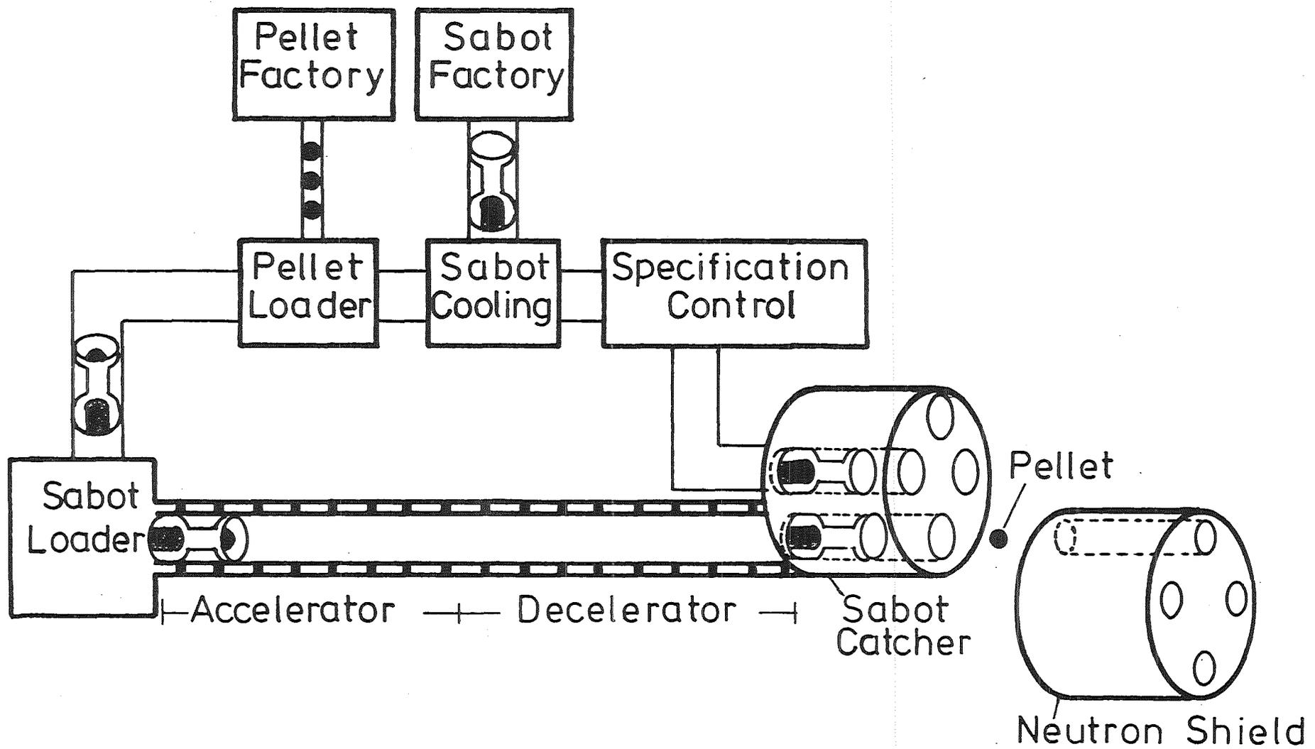
Fig. 8: Scheme of an electromagnetic pellet injection system
