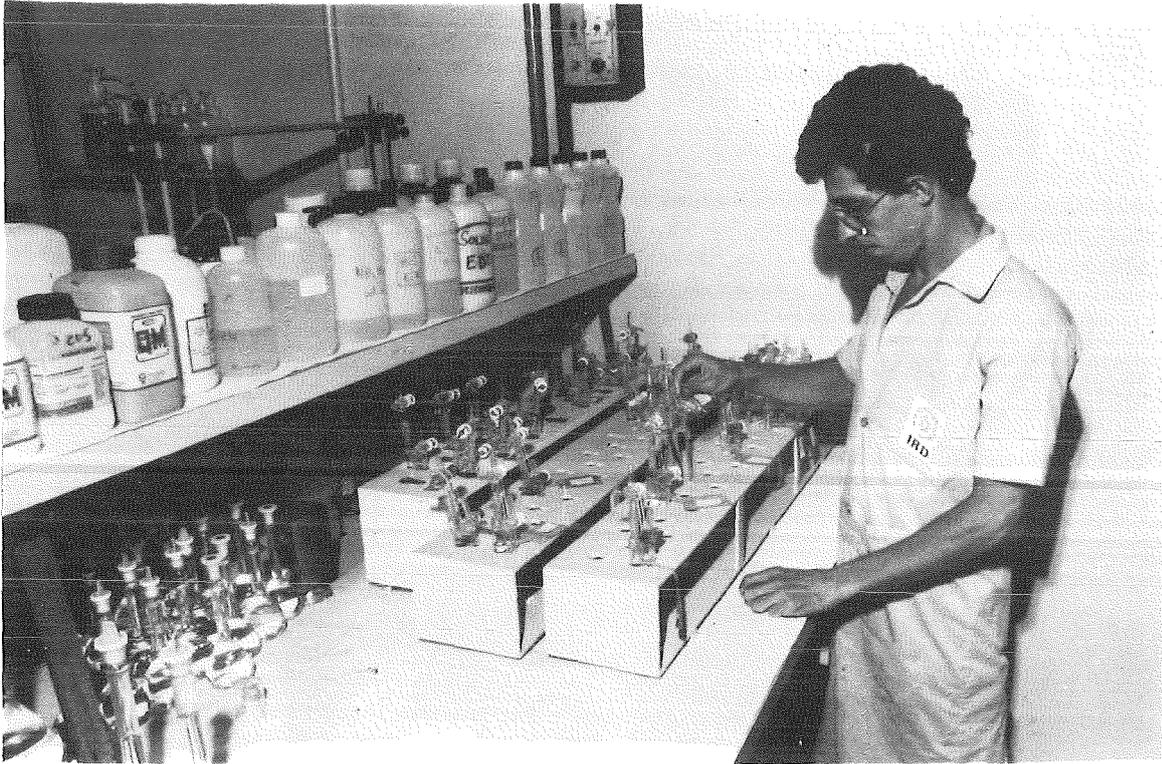
Fig. 2: Determination of radium by the radon emanation method (DEPRA/IRD).
