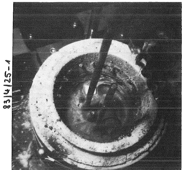
Fig. 6 Upper photo: Series "3 tubes", crucible before and after reaction, tube inlet and WRe thermocouple
