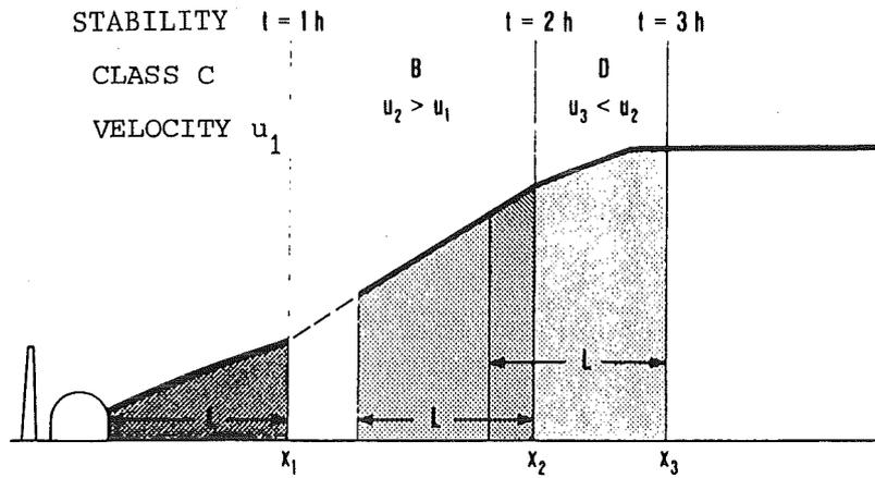
Fig. 3: Side view of the activity plume.
