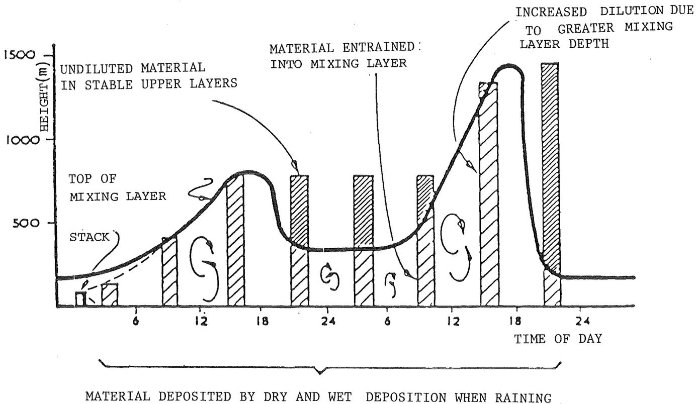
Fig. 5: Vertical dispersion of the plume.
