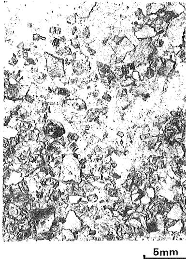
Fig. 9 Fuel Rod Fragments after Flooding Test. (Test No. 15, 220 cal/g·UO<sub>2</sub>, in Air, Water Injected)
