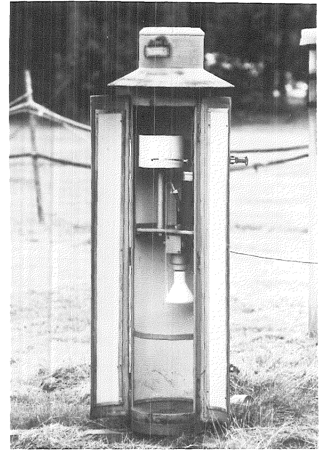
Fig. 8: Rainfall measuring instrument
