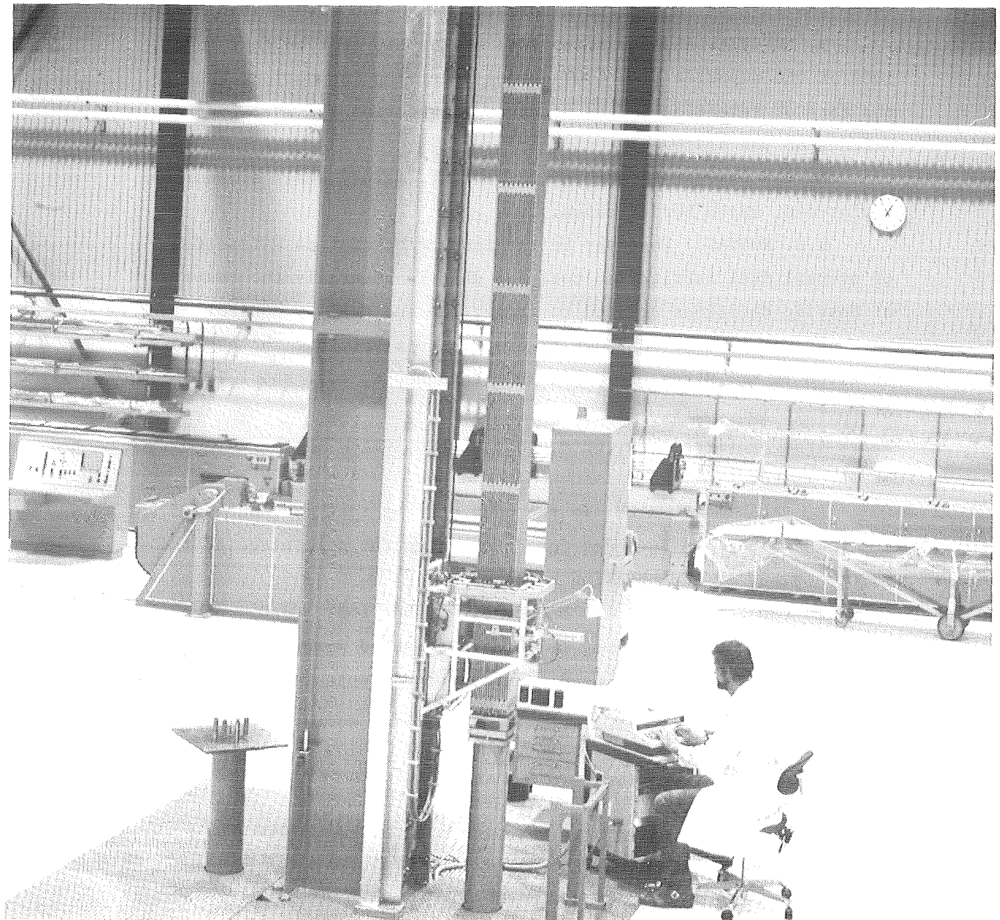
Fig. 14. PWR assembly inspection machine
