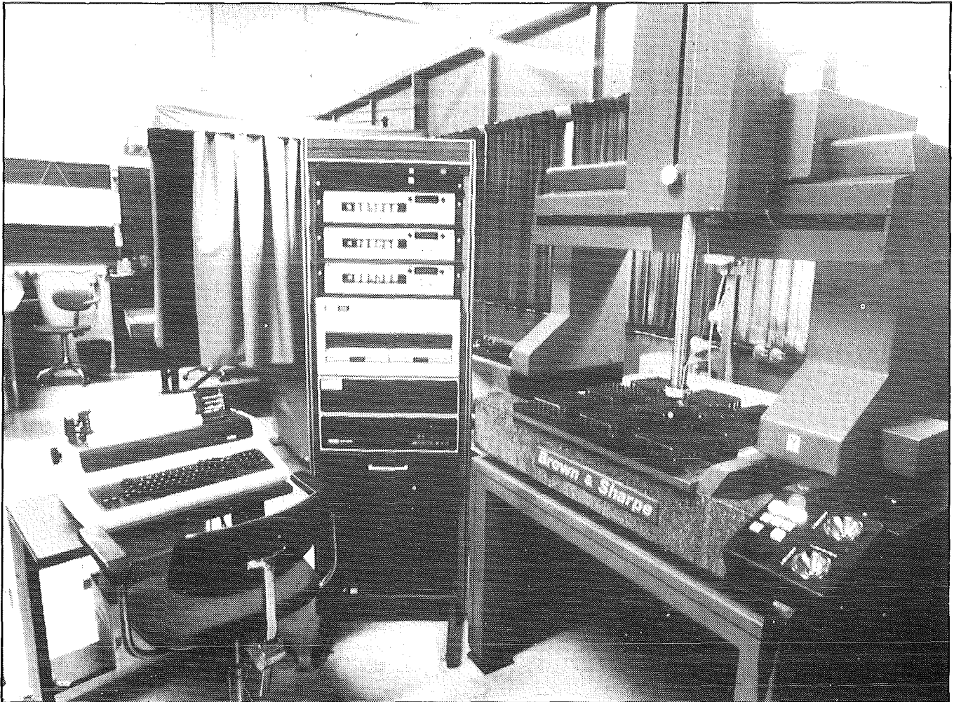
Fig. 13. Inspection of spacer grids in the coordinate measuring machine
