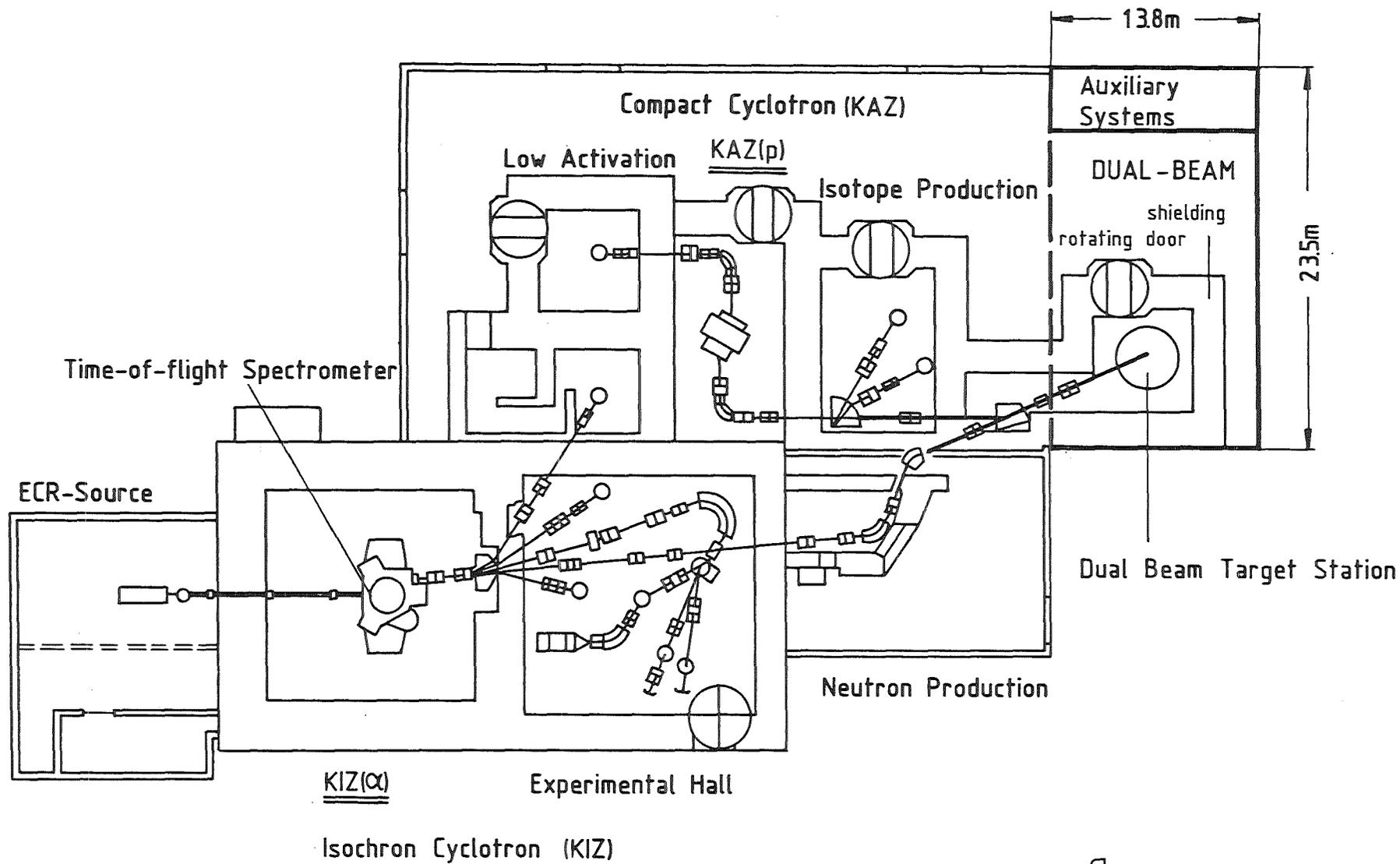
Fig. 2 a Karlsruhe Cyclotron Plot Plan
