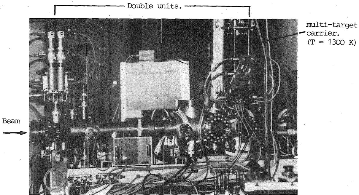
UHV irradiation chamber and different beam diagnostic components.
