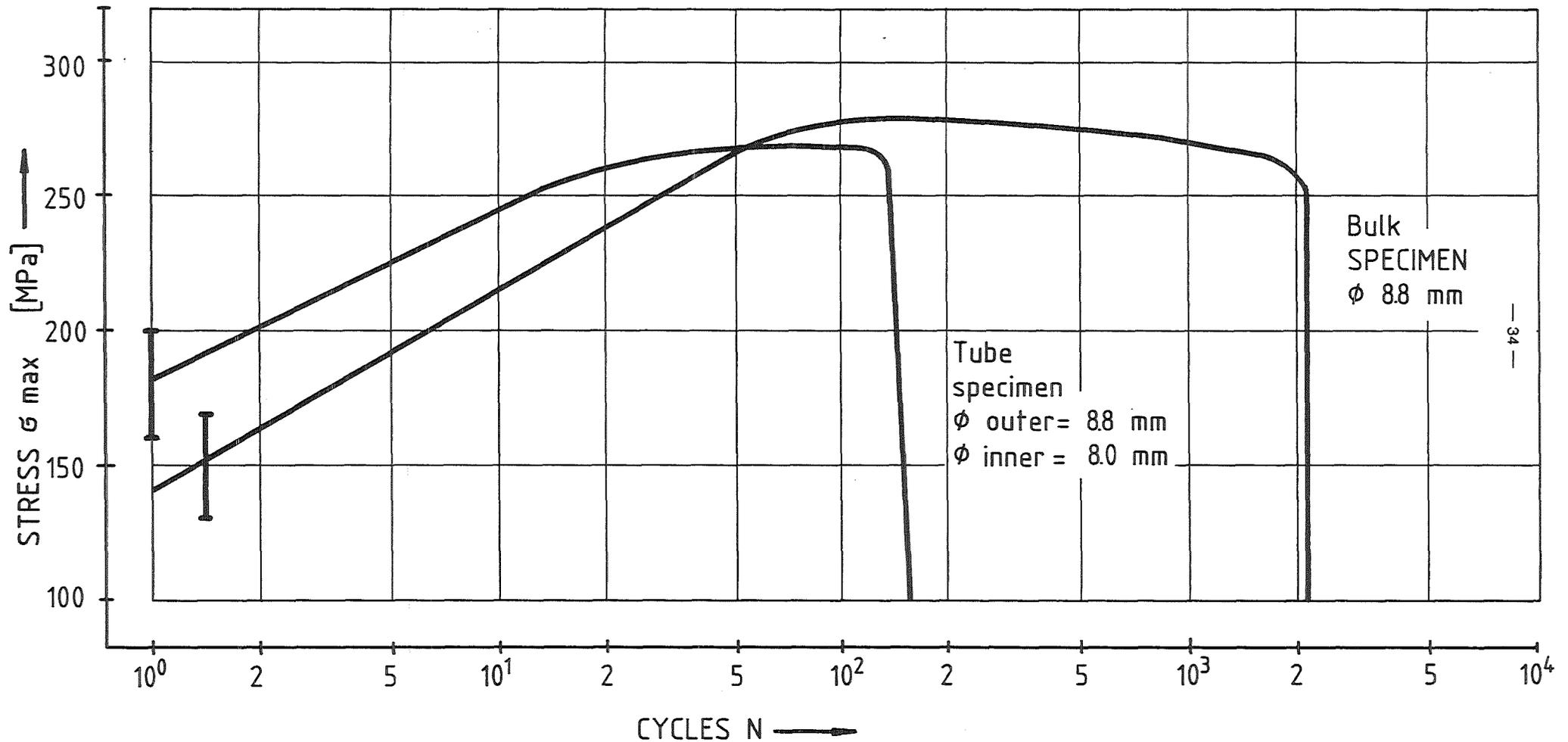
Fig. 6 Comparison of the low-cycle behaviour (LCF) of 14948 ss at 823 K for a bulk specimen and a tube specimen of 0.4mm wall thickness
