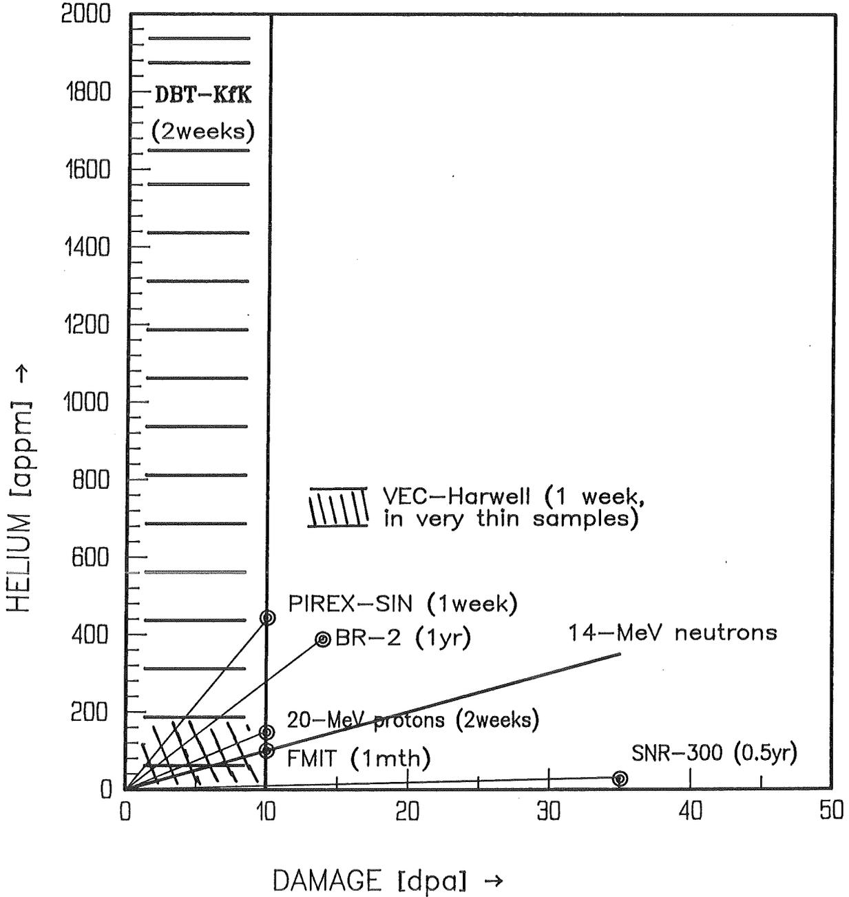
Fig.1 Facility comparison in terms of the production of damage and helium for stainless steel.
