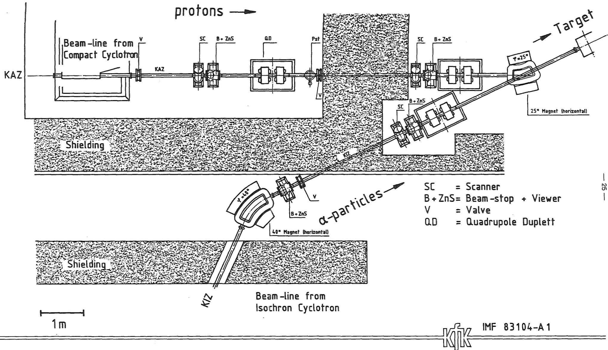
Fig. 2b Top view of the two beam-lines and the required diagnostic components
