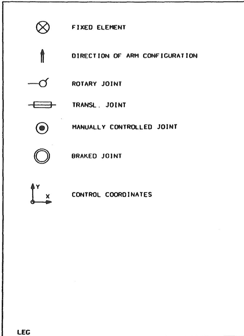
Figure 12. Boom kinematic symbols
