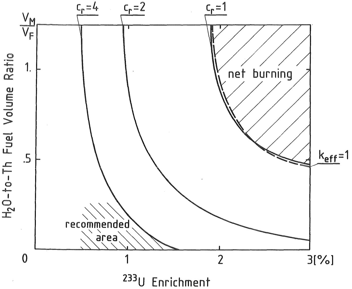
Fig. 4.11a Fissile breeding system parameter phase space
