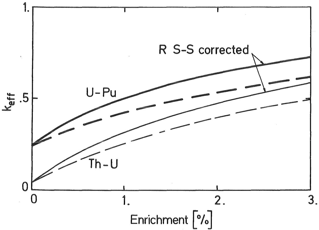
Fig. 4.9c Resonance self-shielding influence on  $k_{eff}$
