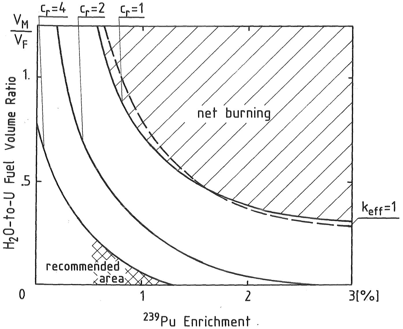
Fig. 4.11b Fissile breeding system parameters phase space U-cycle
