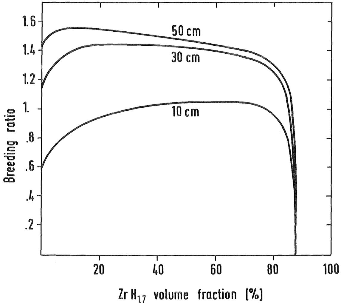
Fig. 3.4 Tritium breeding rate for various thicknesses of Li<sub>17</sub>Pb<sub>83</sub> (90 % <sup>6</sup>Li) breeding zone vs. ZrH<sub>1.7</sub> volume fraction
