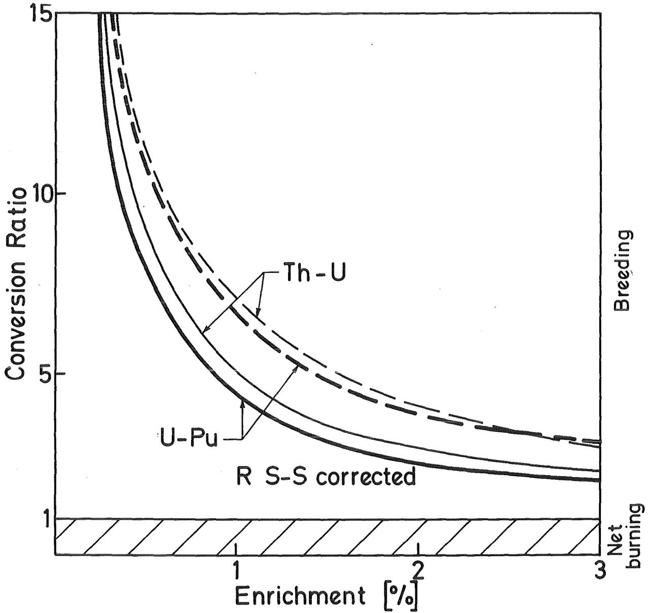
Fig. 4.10c Resonance self-shielding influence on the conversion ratio
