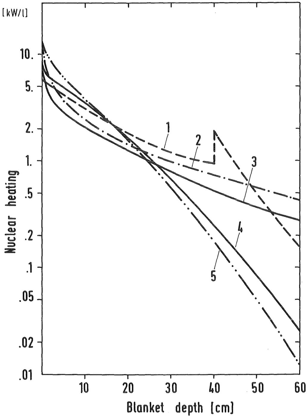
Fig. 3.10a Power density distributions for  $1 \text{ MW/m}^2$  of FW of 14 MeV neutrons (direct FW heating from plasma not considered)
