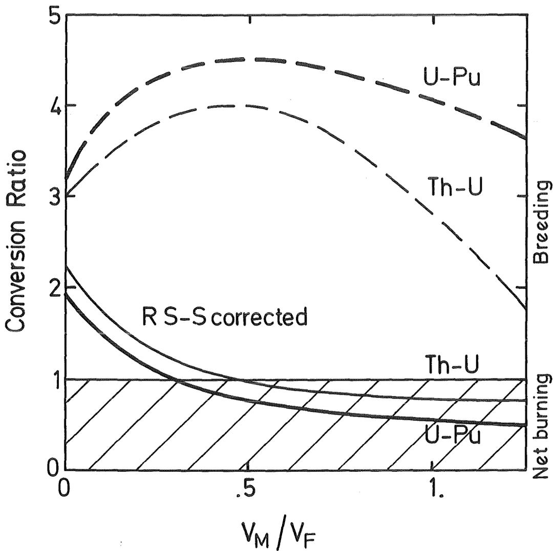
Fig. 4.10a Resonance self-shielding influence on the conversion ratio
