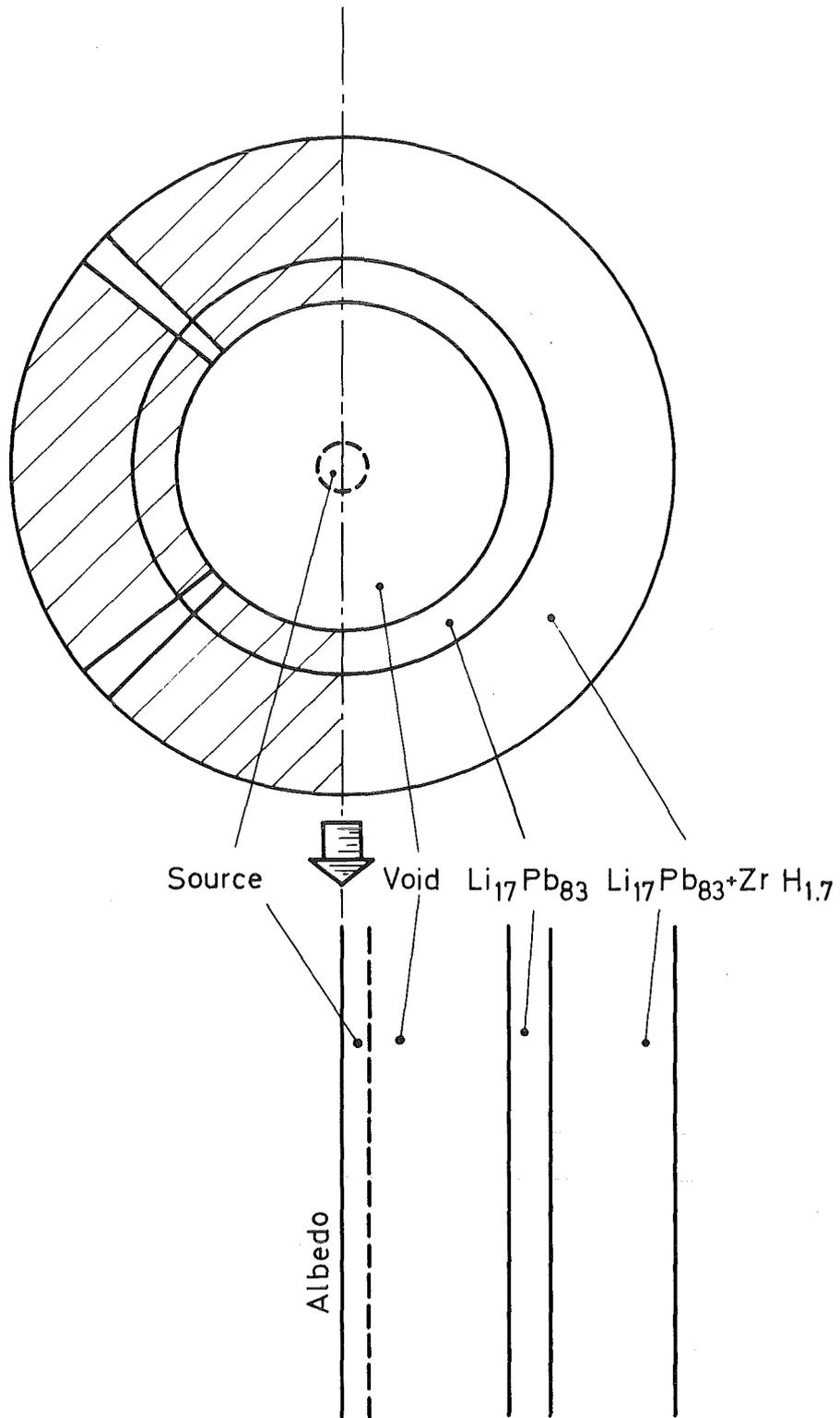
Fig. 2.1a Void streaming estimation with the one-dimensional geometry
