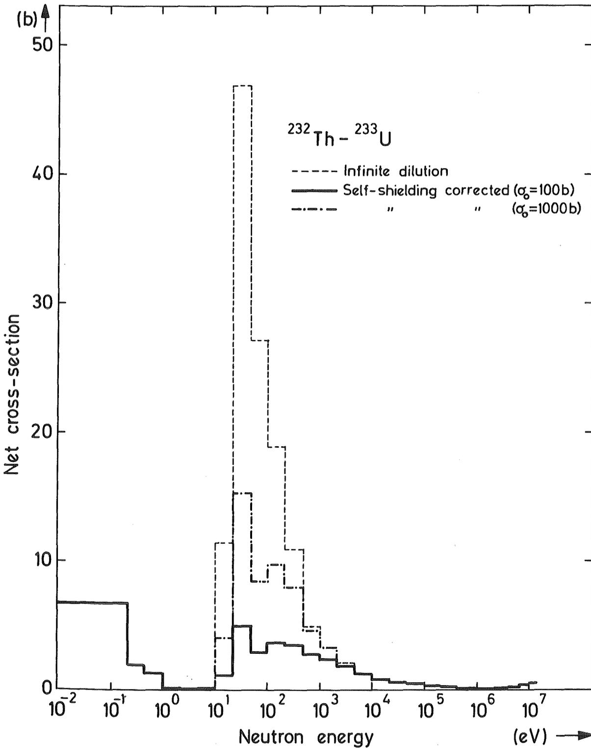
Fig. 4.3a Resonance self-shielding influence on the net fissile breeding cross-section. RSS corrections correspond e.g. to homogeneous mixtures with fertile-to-Be atomic ratios 1/15 and 1.150 respectively (data based on ref. /6,7,8/.  $\sigma_0$  signifies the total cross-section of the medium per one fertile nucleus of resonance cross-section /8/).
