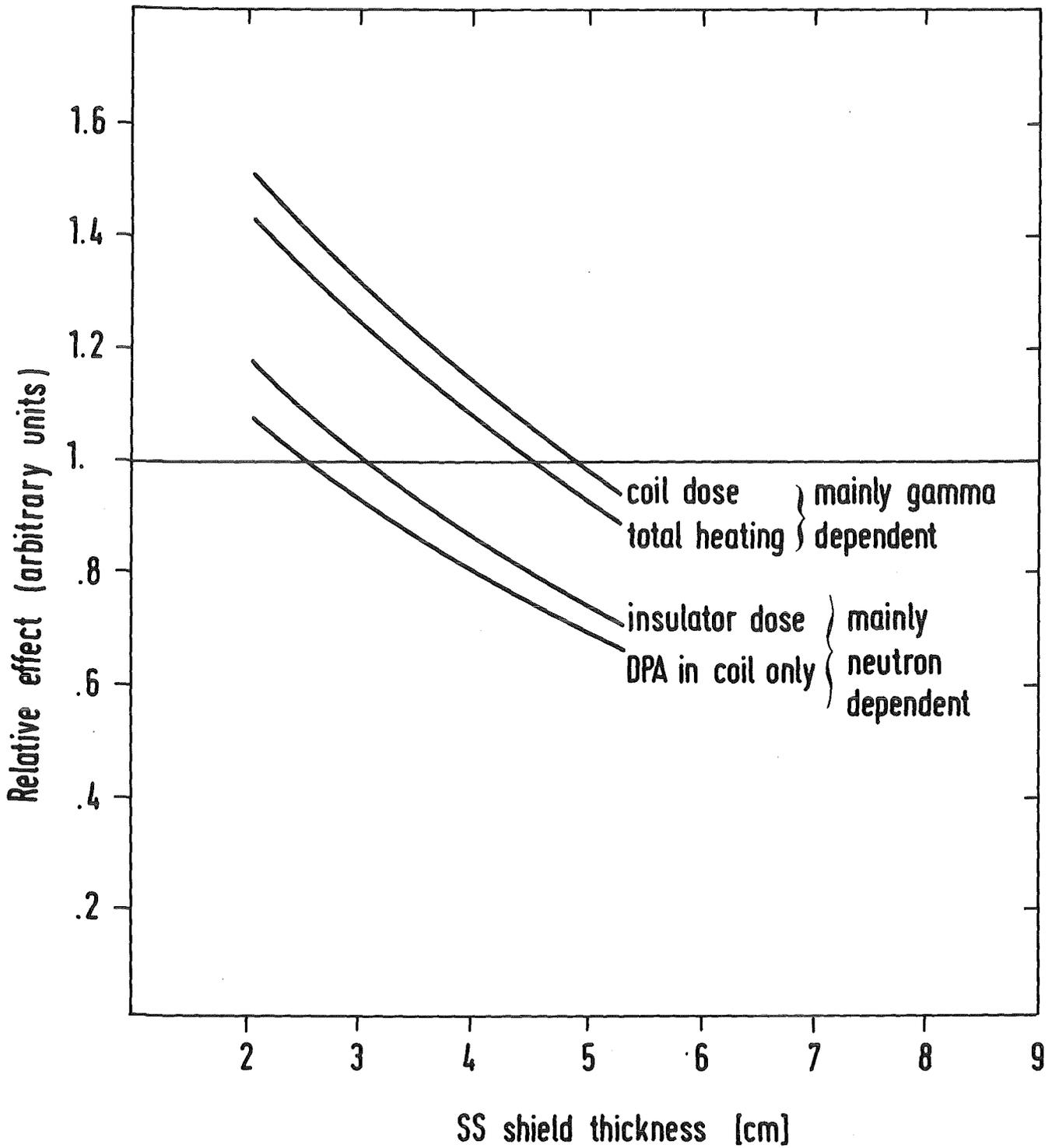
Fig. 3.6 Compensation of weaker radiation attenuation in the 10 cm thick breeding zone by additional steel shield (Breeding medium:  $\text{Li}_{17}\text{Pb}_{83} + \text{ZrH}_{1.7}$ )
