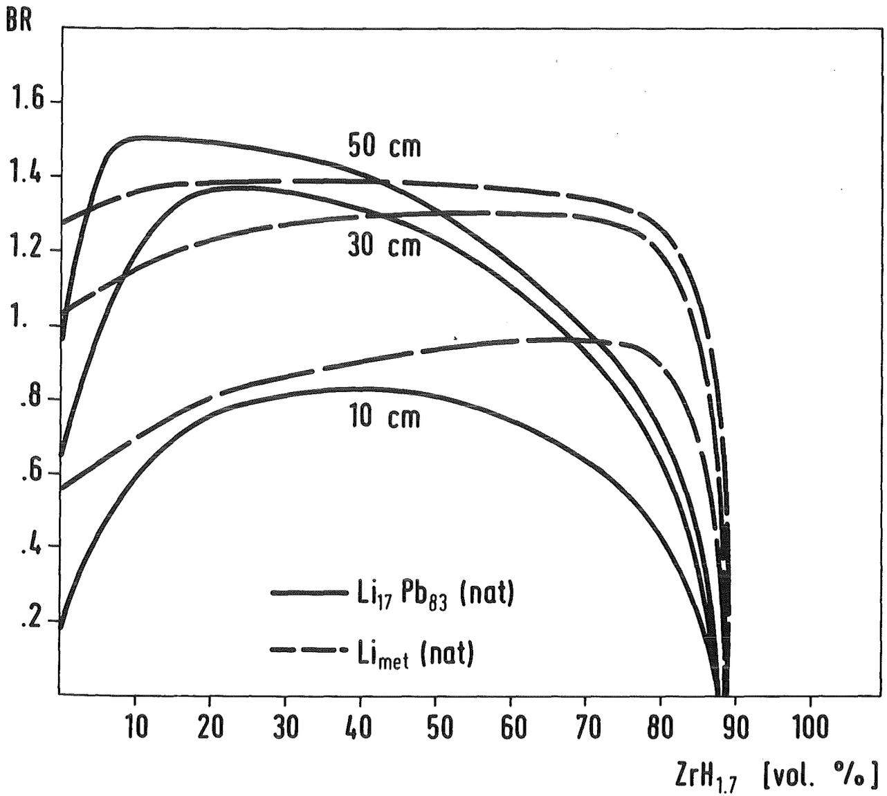
Fig. 3.3 Tritium breeding rate for various breeding zone thicknesses and materials vs.  $ZrH_{1.7}$  volume fraction
