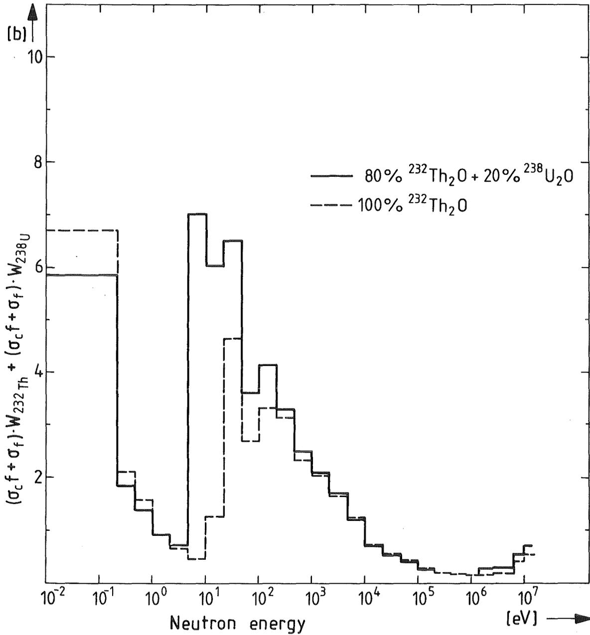
Fig. 4.4 Increase in the effective fissile breeding cross-section for a mixture of fertile materials (self-shielding correction factor  $f$  as for fig. 4.3)
