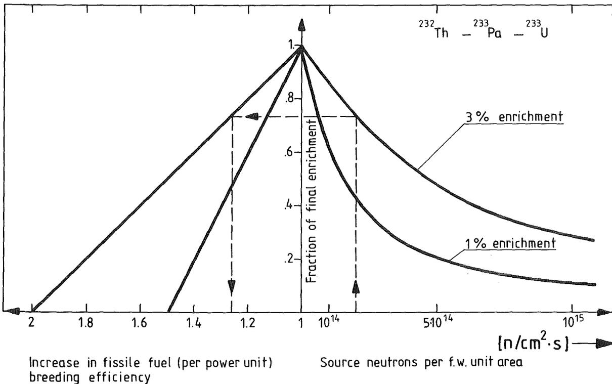
Fig. 4.2a Advantages of rapid enrichment due to delayed fissile build up (200 kg Th 232 per m<sup>2</sup> of the first wall, .6 fissile nuclei/fusion neutron)
