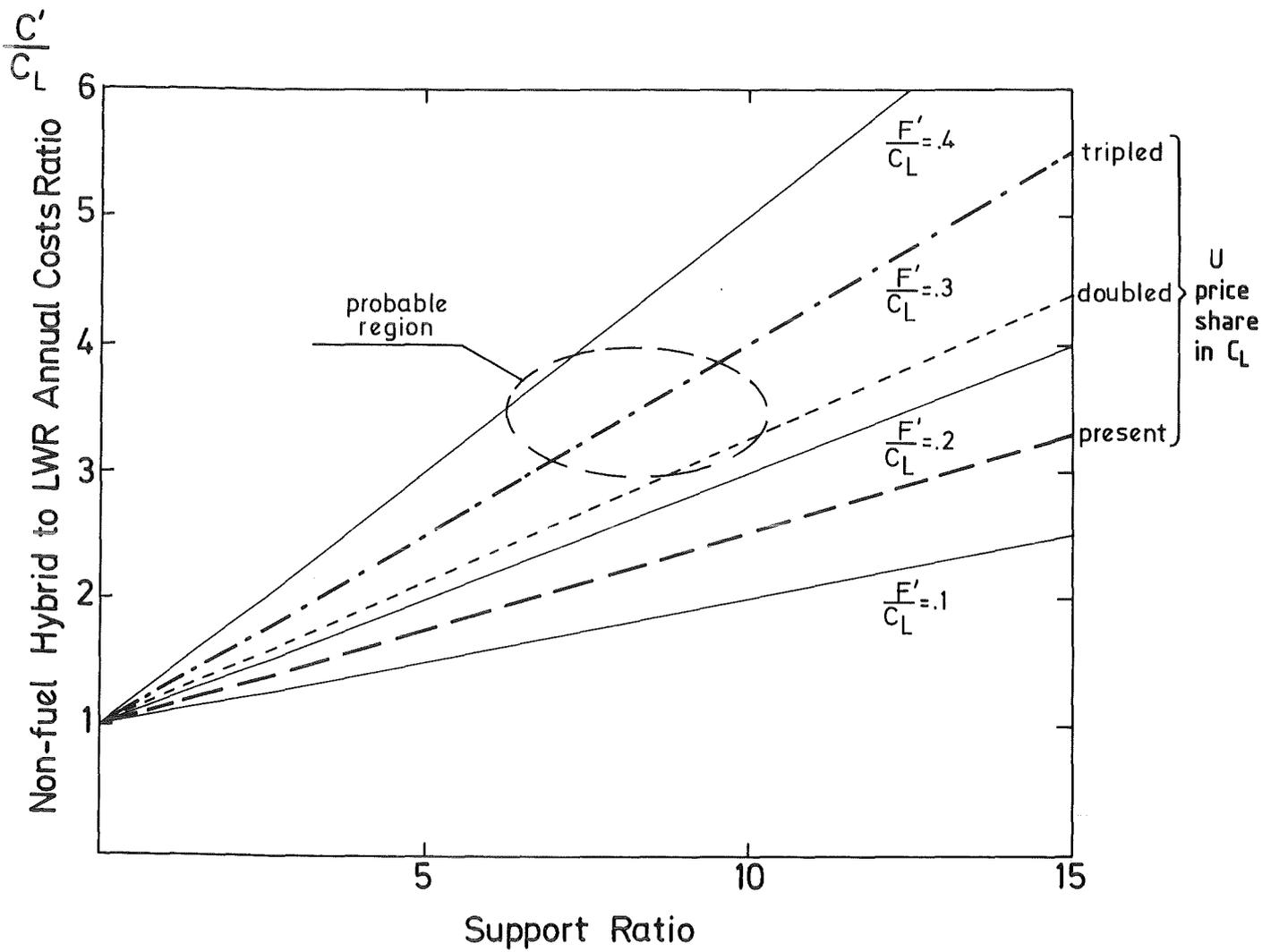
Fig. 1.1a Maximum admissible fissile breeder non-fuel costs as a function of its support ratio for various uranium prices
