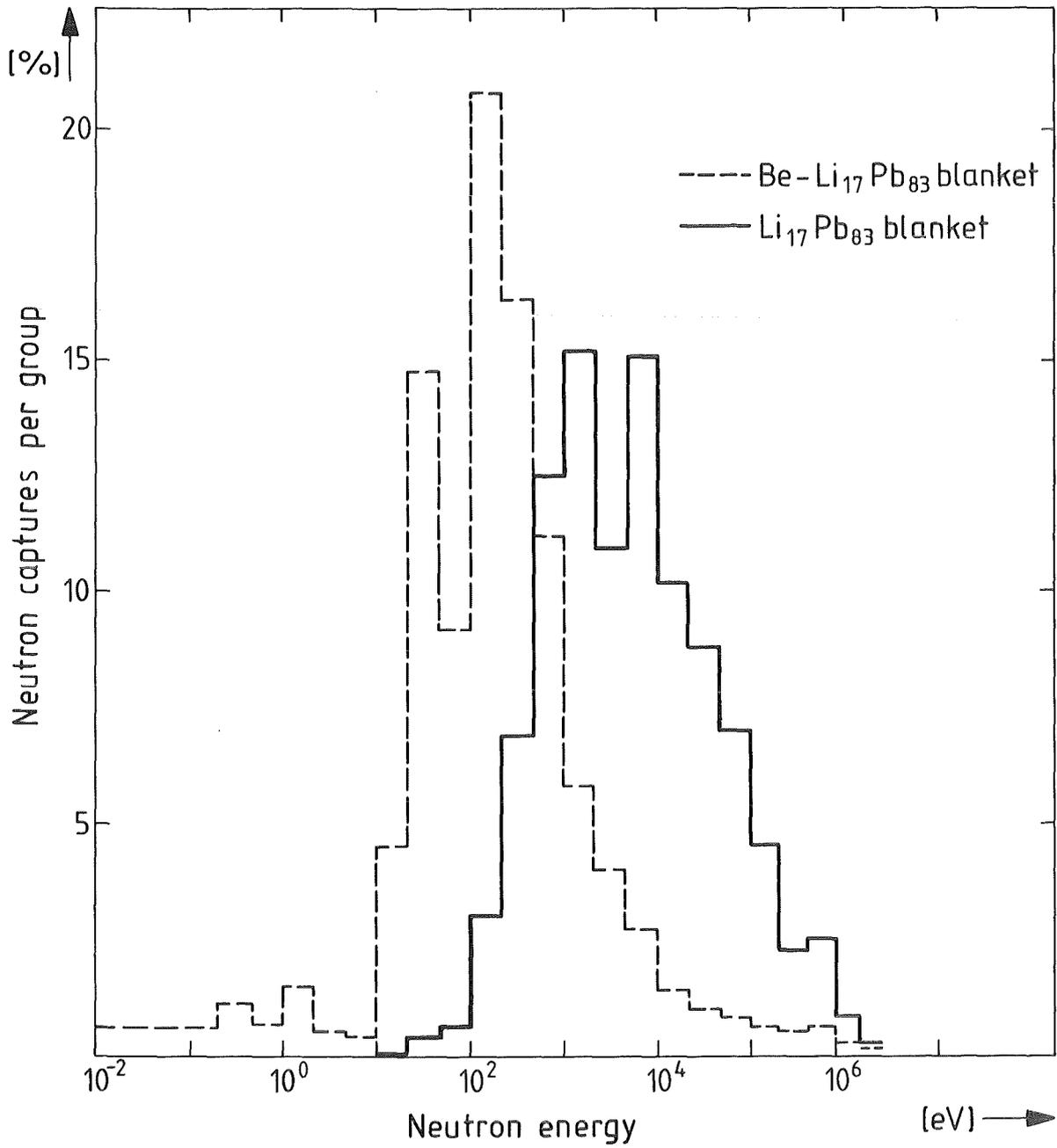
Fig. 4.8 Fissile breeding spectrum for moderated and unmoderated blankets (volume fractions: 66 % Be, 17 % Li<sub>17</sub>Pb<sub>83</sub> (15 % Li 6), 3 % ThO<sub>2</sub>, 4 % SS and 80 % Li<sub>17</sub>Pb<sub>83</sub>, 10 % ThO<sub>2</sub>, 10 % SS respectively)
