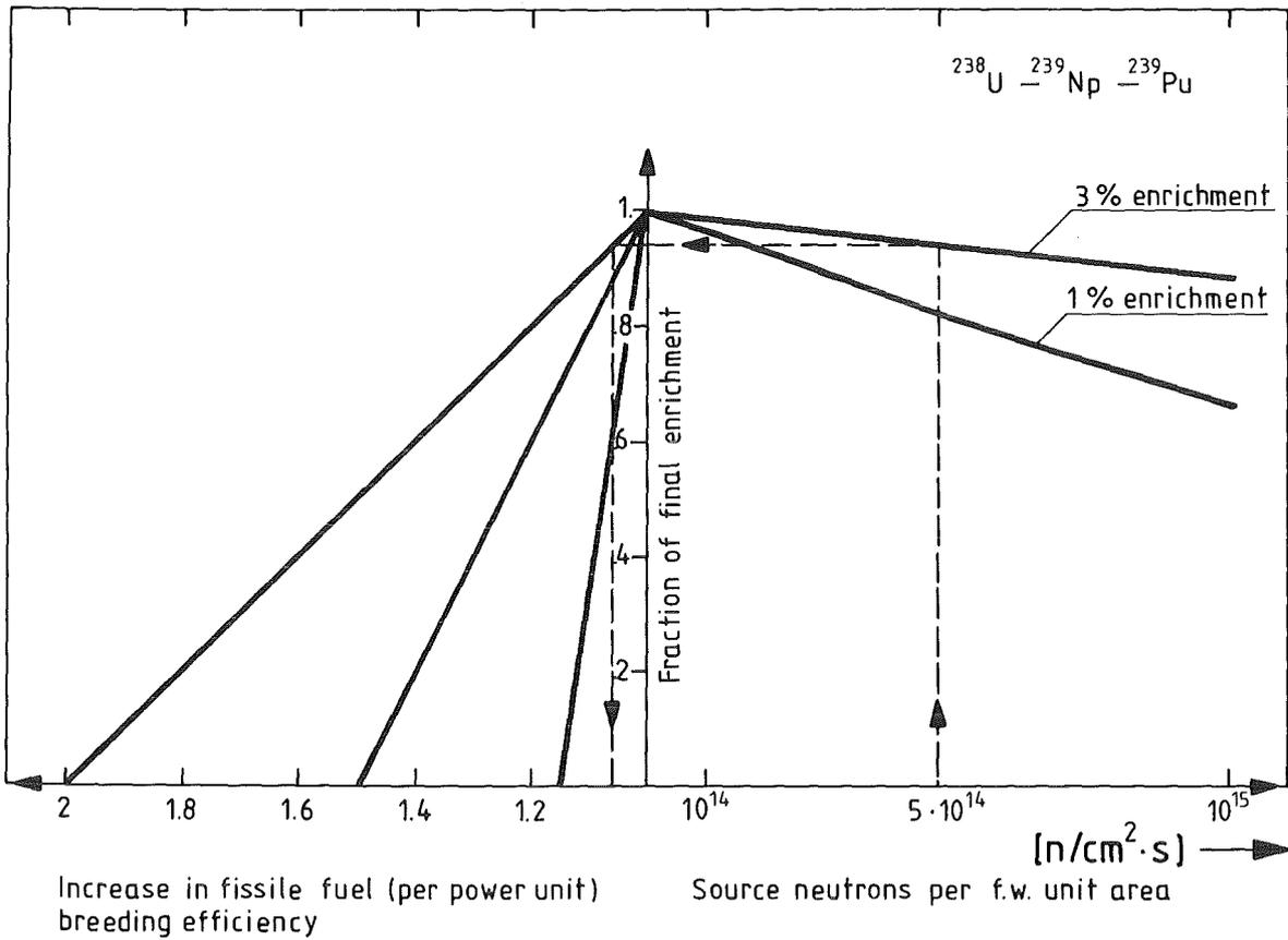
Fig. 4.2b Advantages of rapid enrichment due to delayed fissile build up (200 kg U 238 per m<sup>2</sup> of the first wall, .6 fissile nuclei/fusion neutron)
