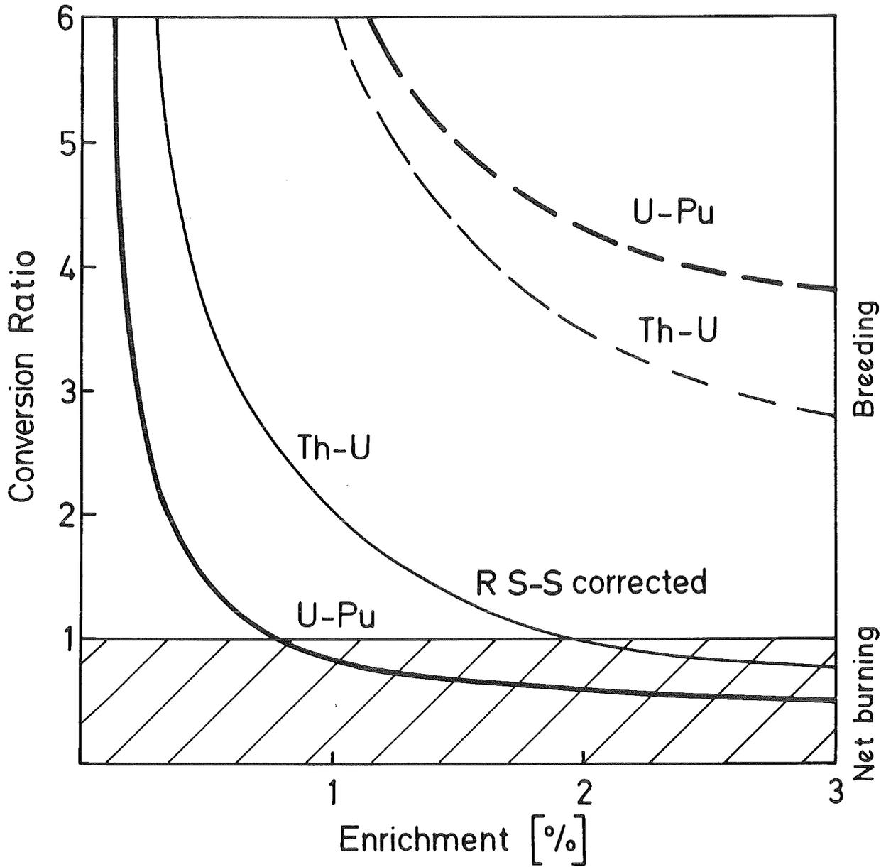
Fig. 4.10b Resonance self-shielding influence on the conversion ratio
