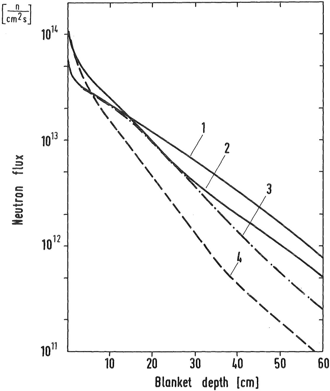
Fig. 3.7 Examples of 14 MeV source neutron flux distributions for various materials and geometries, normalized to 1 MW/m<sup>2</sup> of 14 MeV neutrons
