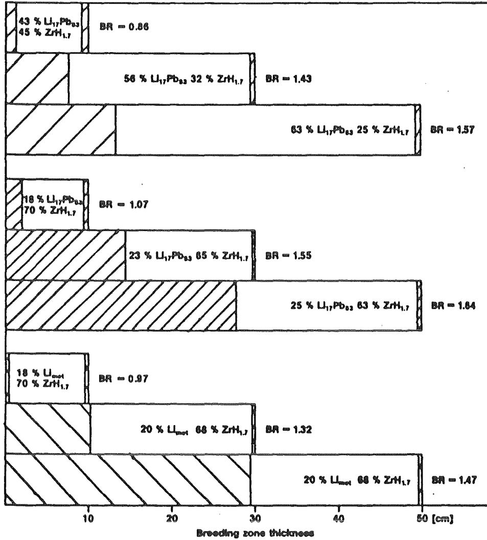
Fig. 3.5. Optimum sandwich structures of the breeding zone for 10 cm, 30 cm and 50 cm blanket thicknesses (in all layers 8 % void, 4 % SS)
