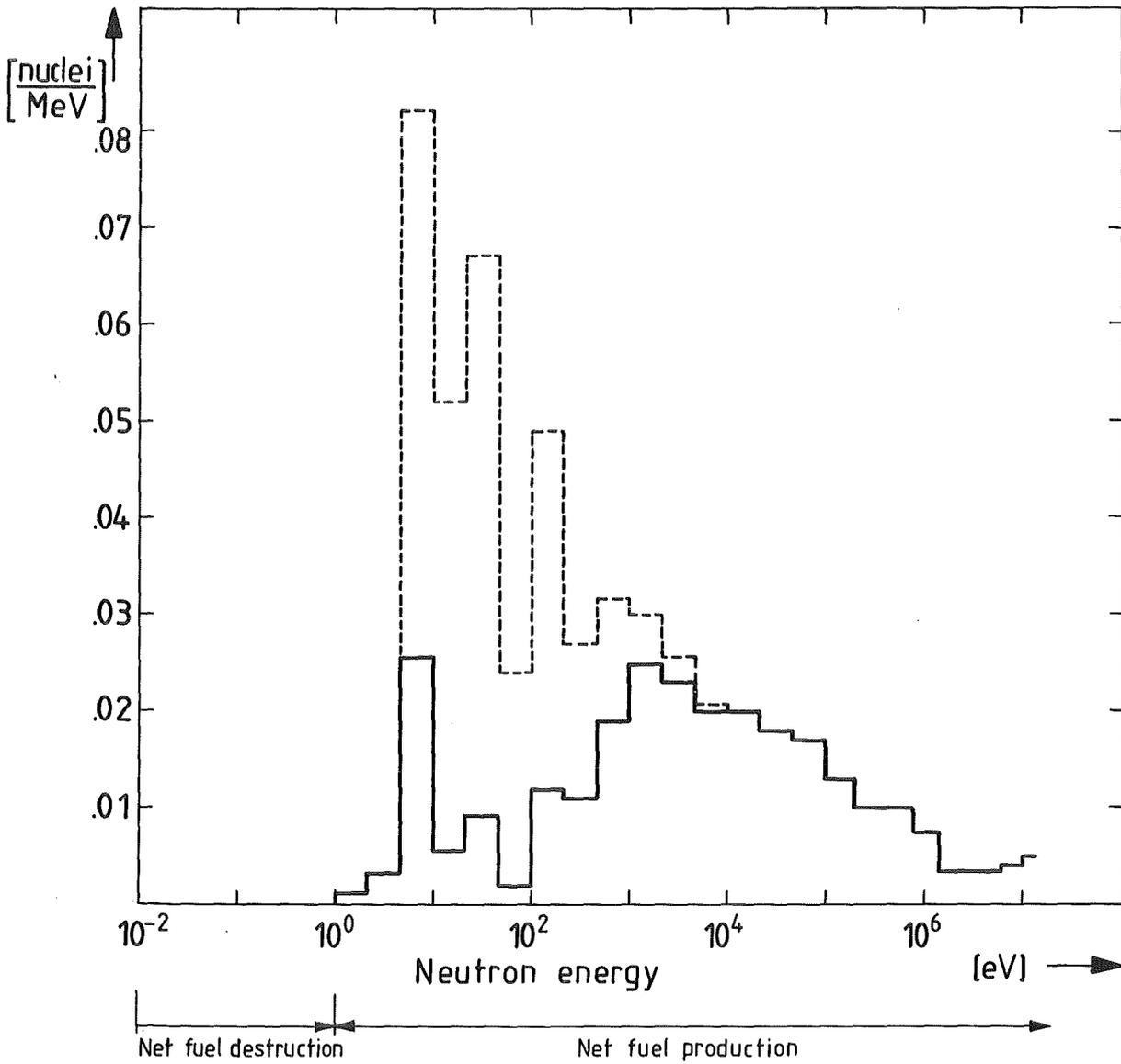
Fig. 4.5b Net fissile breeding per energy released in the fuel (self-shielding correction as for fig. 4.3)
