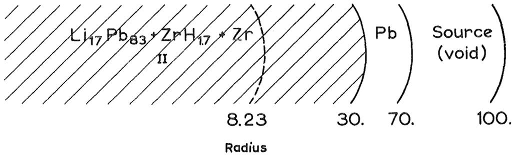
Fig. 2.4 Example of a calculational model for the estimation of non-resonance self-shielding effects in one-dimensional geometry
