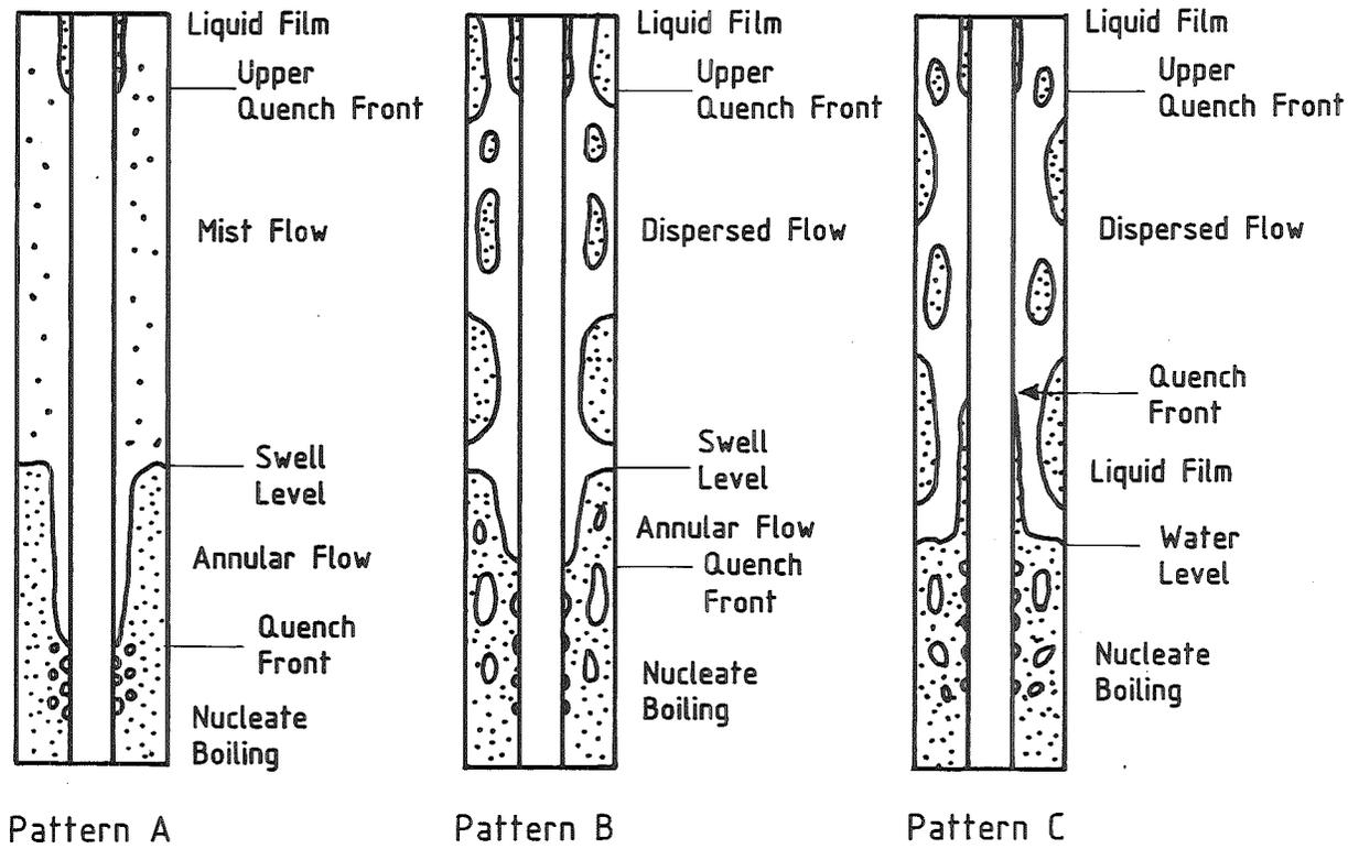
Fig. 17 Comparison of Quench Patterns
