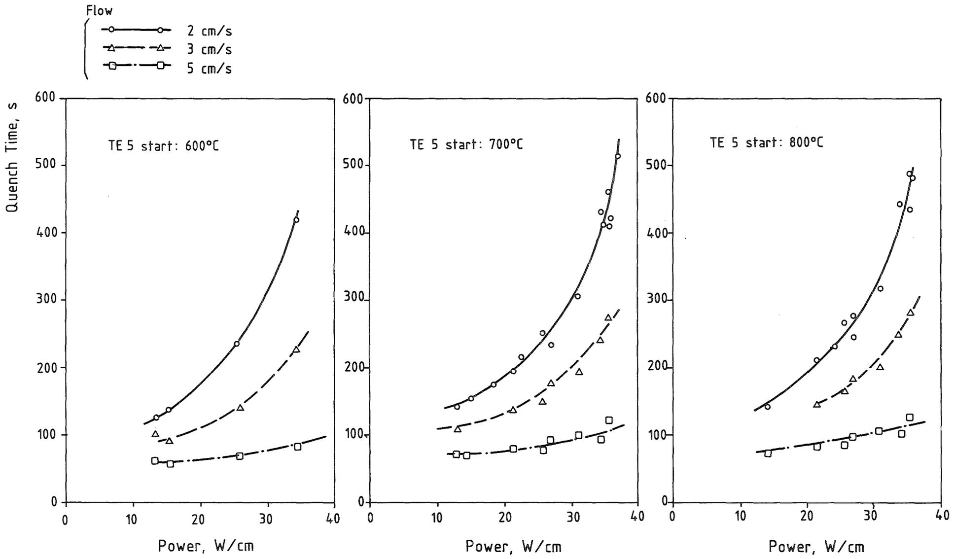
Fig. 10 Quench Times of Whole Rod, Influence of flooding velocity and rod power
