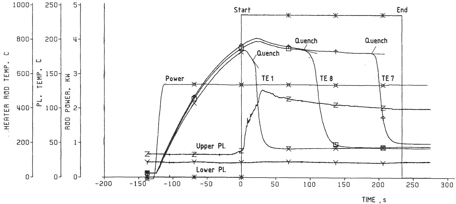
Fig. 6 Heater Rod , Plenum Temperatures and Power
