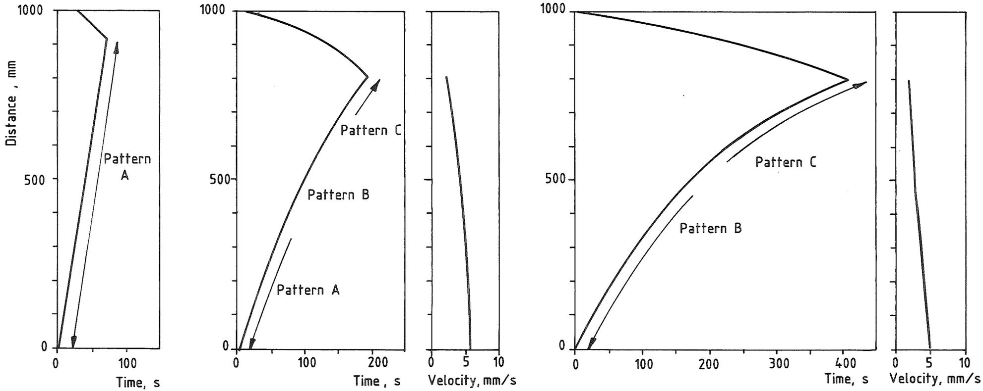
Fig. 18 Quench Front Progressions and Quench Front Velocities - Comparison of Quench Pattern
