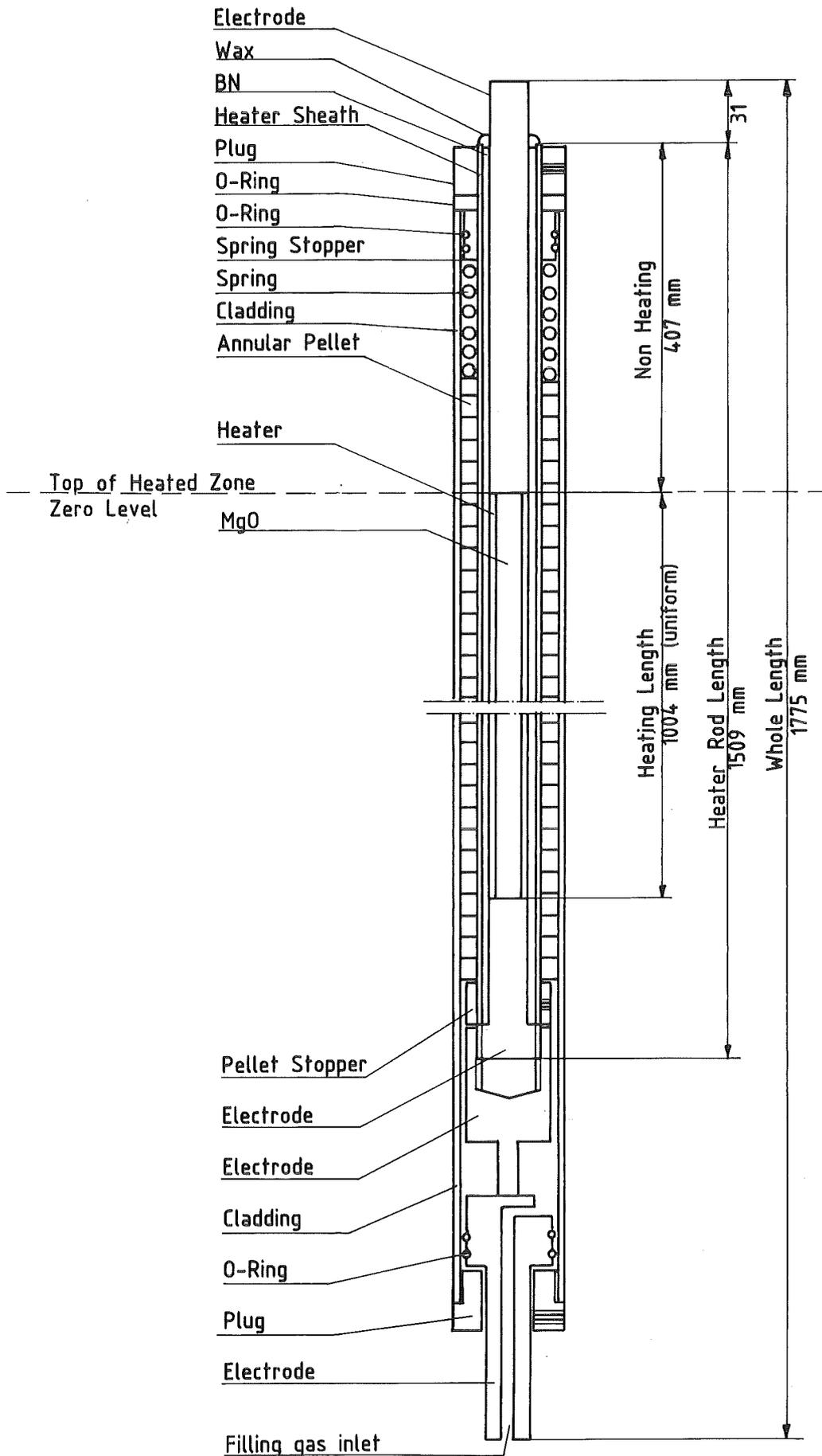
Fig. 2 Longitudinal Cross Section of SEFLEX-E Fuel Rod Simulator
