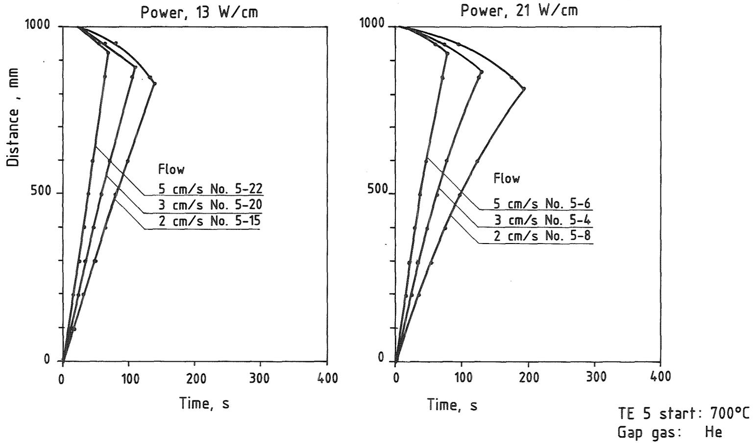
Fig. 13 Quench Front Progressions-Influence of Flooding Velocity
