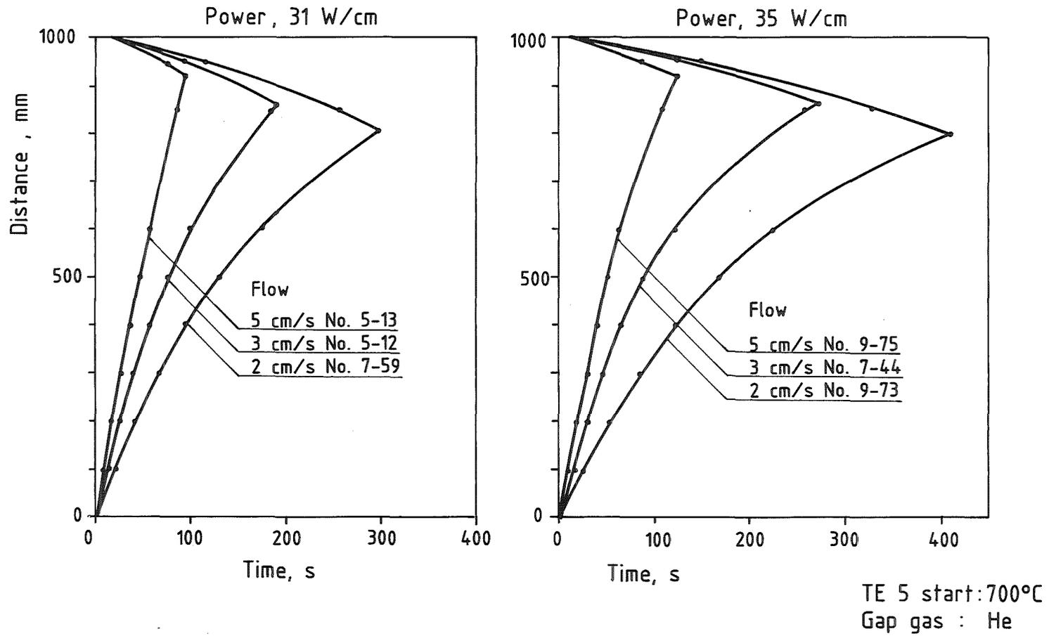
Fig. 14 Quench Front Progressions-Influence of Flooding Velocity
