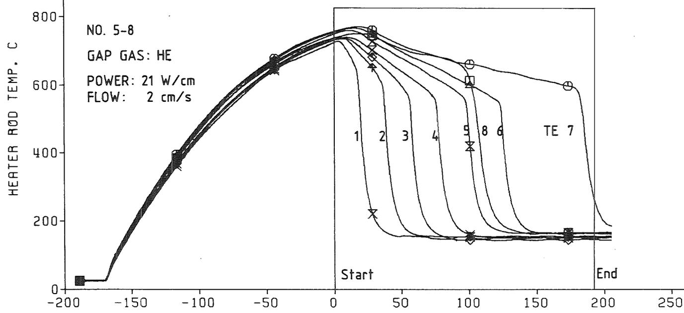
Fig. 19 Heater Rod Temperatures- Influence of Gap gas
