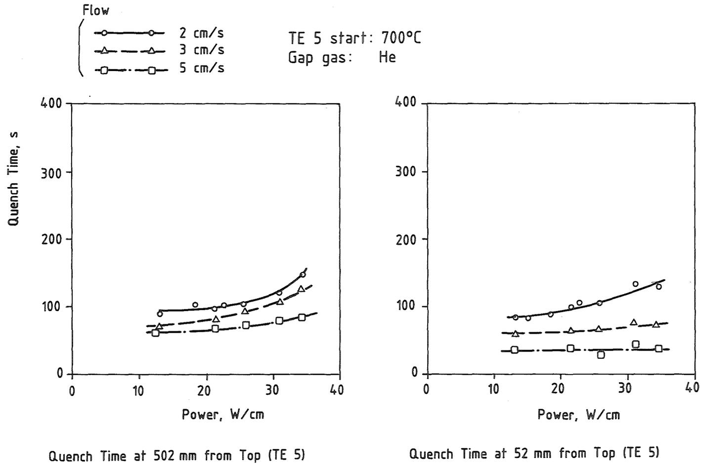
Fig. 11 Quench Times at 502mm, 52mm from Top, Influence of flooding velocity and rod power
