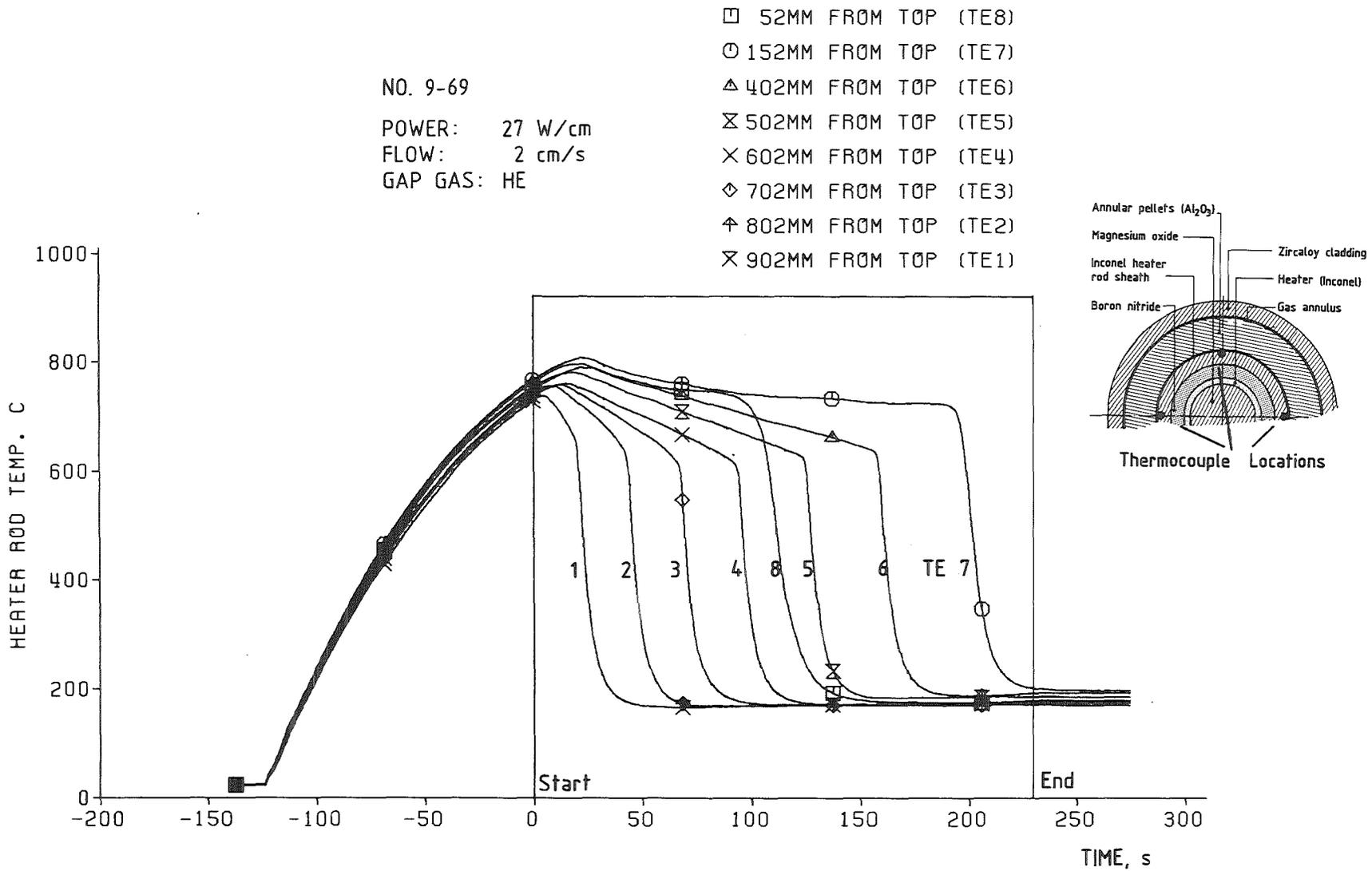
Fig. 5 Heater Rod Temperatures
