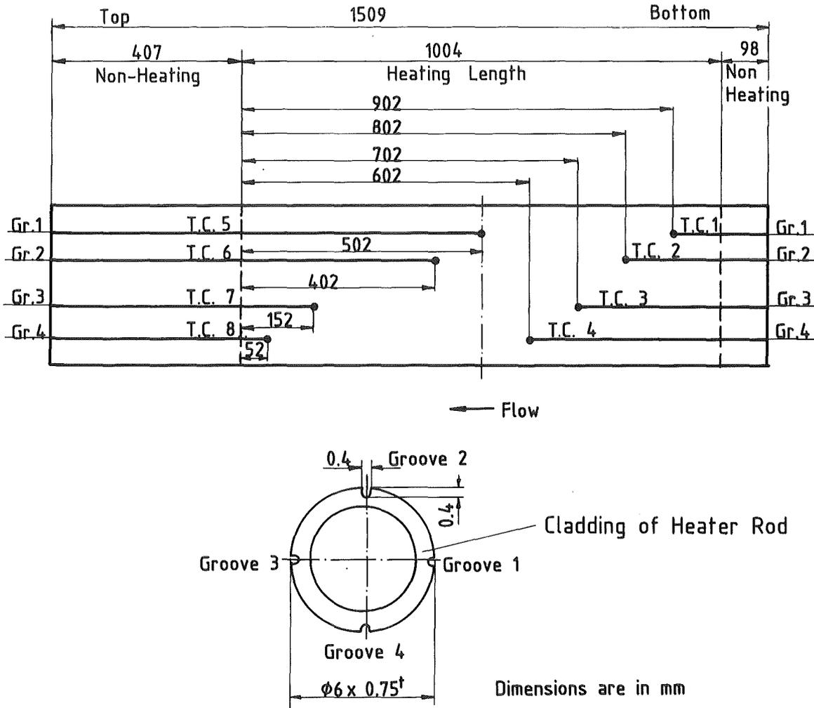
Fig. 4 Positions of Thermocouples of the internal SEFLEX-E Heater Rod
