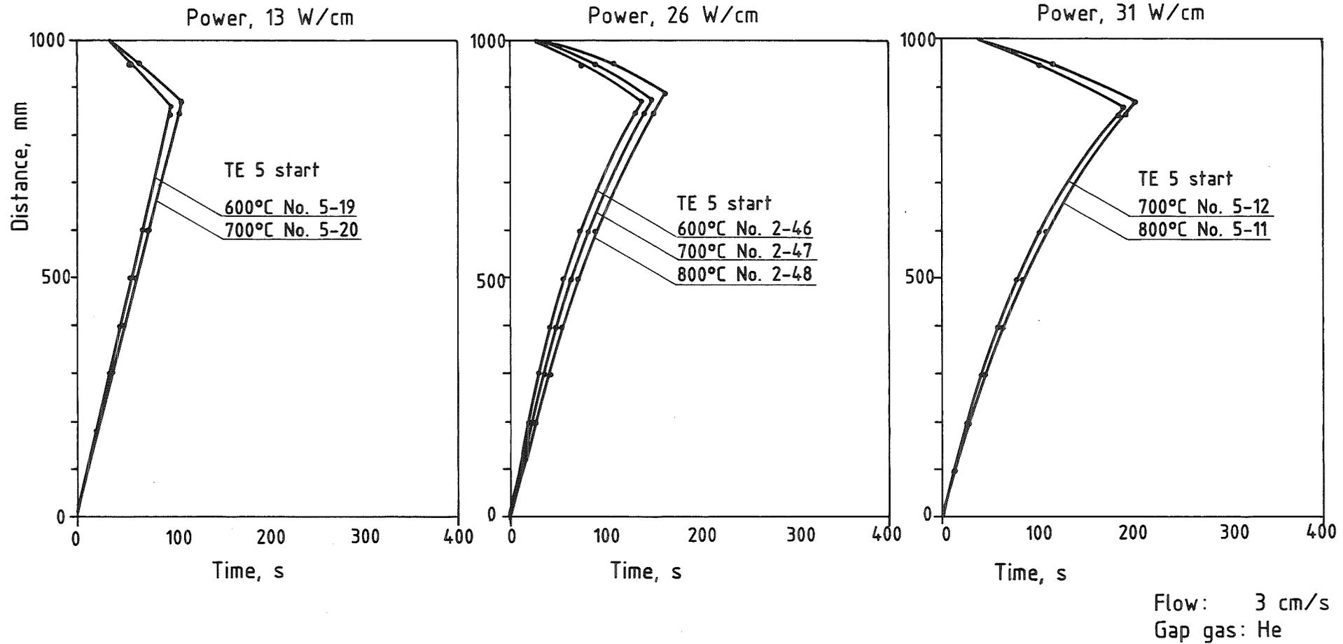
Fig. 16 Quench Front Progressions-Influence of Initial Rod Temperature
