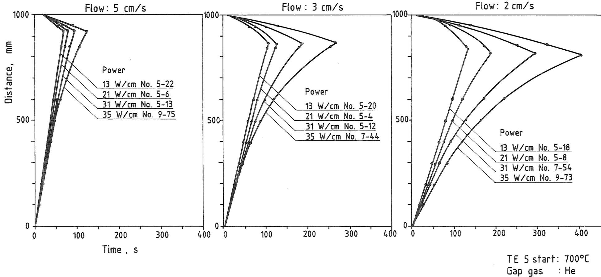
Fig. 9 Influence of flooding velocity and rod power on quench front progression
