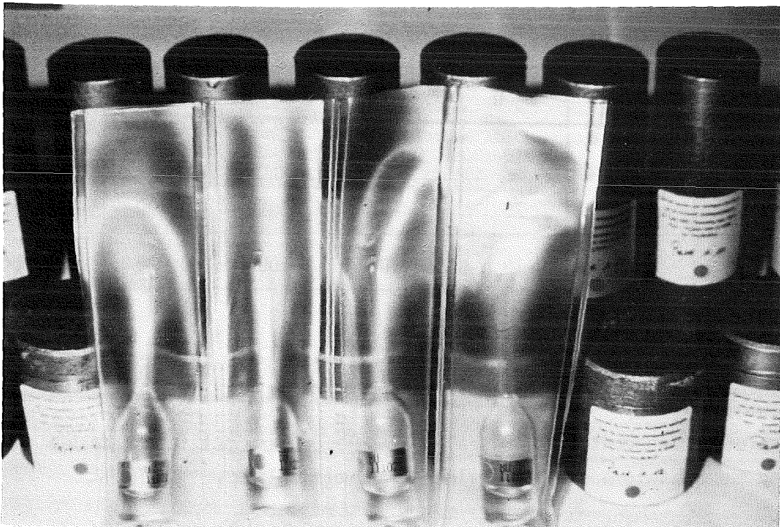
Photogr. 3.1: Liquid test samples in sealed glass ampoules as well as lead container
